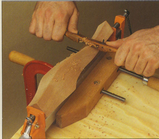
The cabriole leg harkens back to the time-honored art of shaping wood with hand tools. Here, the leg's unmistakable contours are revealed and smoothed by a spokeshave, traditional cousin of the hand plane.
