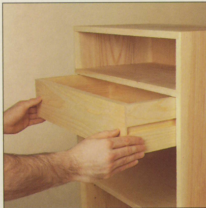
A side-mounted drawer is slid into a carcass for test-fitting. A lipped front conceals the runners and grooves when the drawer is closed.
