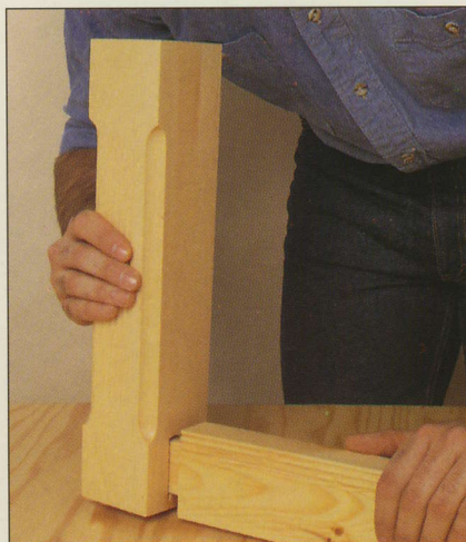
The tenon at the end of a rail fits snugly in a mortise cut out of a square leg, creating a sturdy, long-lasting joint.
