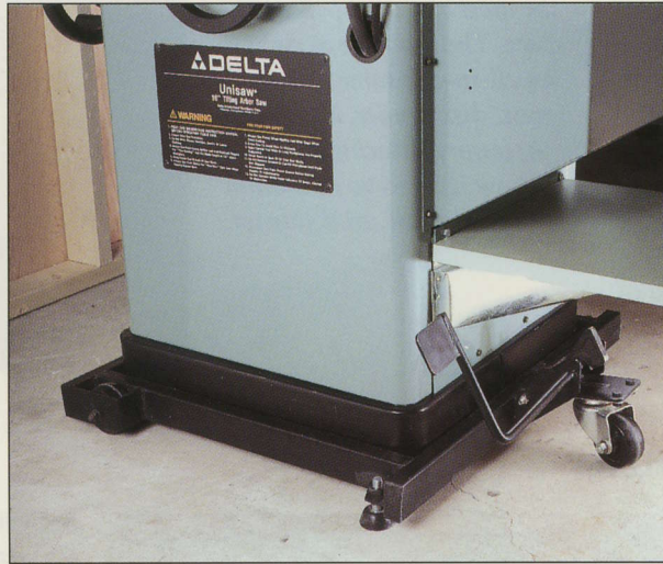
Even in spacious shops, tools occasionally need to be moved around; in small shops, reassigning floor space may be a part of every project. A wheeled base can make a 10-inch table saw, like the one pictured here, easy to reposition.
