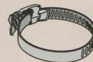
Hose clamp Slotted metal band and screw used to join two lengths of duct or hose
