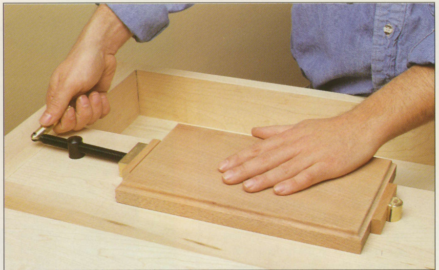
This bench dog features a threaded screw that converts it into a miniature tail vise. Used in conjunction with other bench dogs, it excels at clamping small or irregular work, like the panel shown above.
