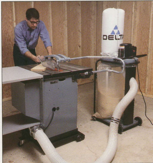
Most of the wood chips and sawdust generated by this 10-inch table saw are captured by a portable dust collection system. Often neglected in the past, dust collection has become a central concern of many safety-conscious woodworkers in planning the layout of their shops.
