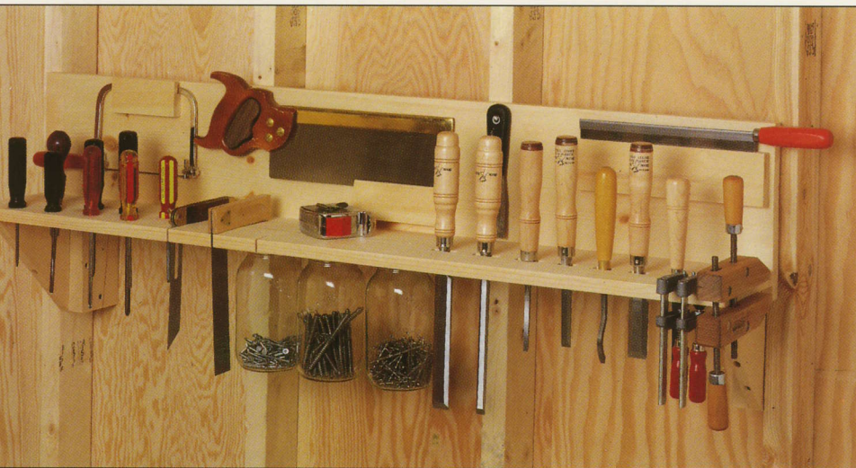
Shelves are an ideal tool storage option. This shop-built unit features grooves and cleats custom-cut to hang a panoply of tools in full view over a workbench.
