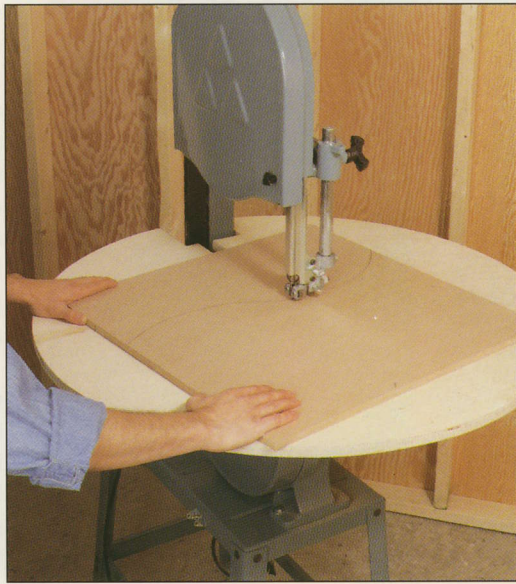
Better control produces better results. Secured to a band saw's original table, a shop-made extension table keeps a large hardboard sheet level during a curved cut.
