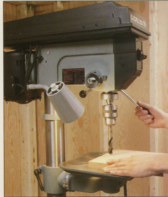
A clamp-on lamp can shed all the light you need to work safely at a tool. Mounted on a drill press, this lamp's flexible neck aims a 40-watt bulb directly at the machine's work table.
