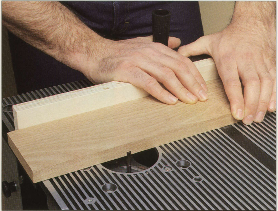
Mounted upside down in a specially designed table, a router cuts a dado. Attaching a backup board to the miter gauge helps keep the work square to the bit and reduces tearout.
