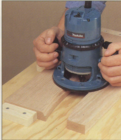
A support board secured alongside a workpiece during an edge-forming operation keeps the router steady. For contour cuts, use the waste piece that remains after sawing the curve.
