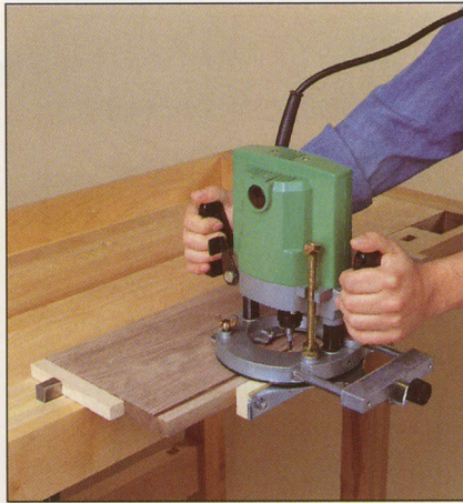
A straight bit carves a groove in a board. Riding an edge guide along the board produces a cut parallel to the edge.
