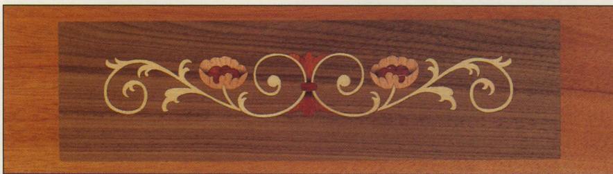
A marquetry inlay, formed from a pattern of dyed wood set in a veneer, graces a mahogany board. The inlay was glued into a routed recess.
