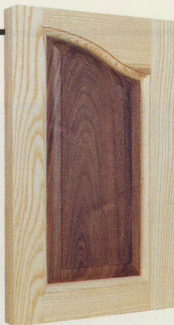
This frame-and-panel door features a sturdy frame of rails and stiles encasing a decorative floating panel. The contrast between the walnut panel and ash frame makes this door all the more striking.
