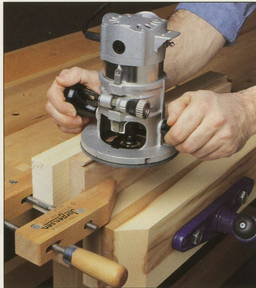
Keeping a router from wobbling as it is fed along the edge of a workpiece to cut a profile into the face can be a tricky operation. A support board clamped to the stock can help keep the tool steady.
