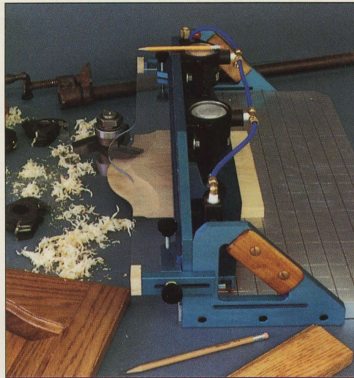
The shaper is a common sight in production shops, where it is unequaled for constructing cabinet doors. The panel-raising jig shown above allows arched top rails and arched raised panels to be shaped quickly, safely, and accurately.
