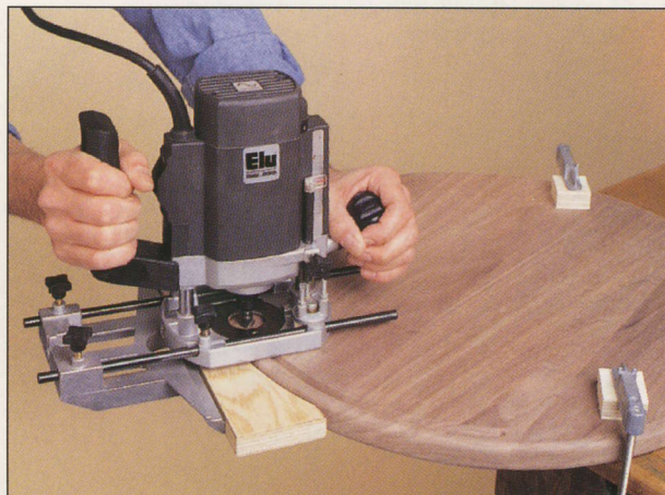
A core box bit carves a circular groove near the edge of a walnut tabletop. To ensure that this decorative cut follows the arc of the workpiece, a curved extension is fastened to a commercial edge guide to ride along the edge of the stock.
