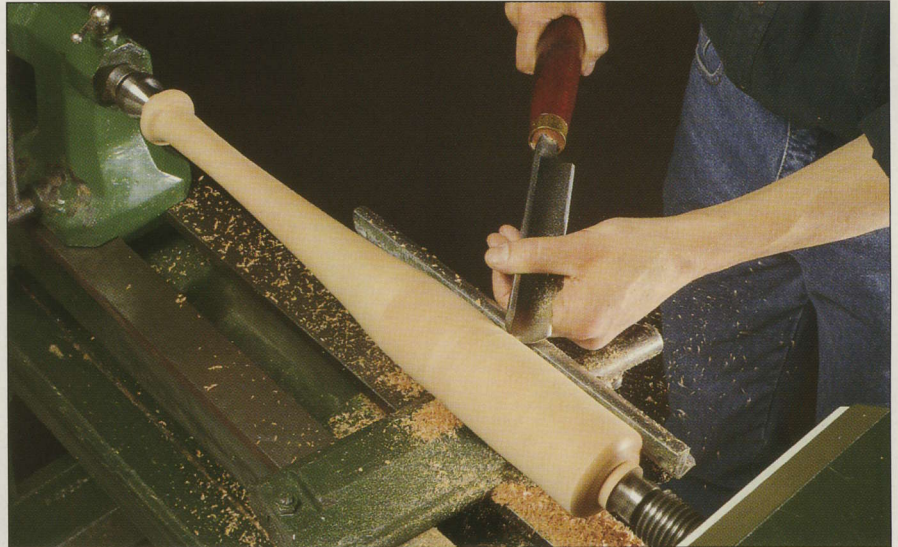
Because it is spinning at high speeds, a blank mounted between centers provides the turner with an immediate and continual visual check of a project's progress. In the photo above, a roughing gouge brings a small baseball bat to its final shape.
