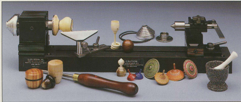
Developed by Seattle wood turner Bonnie Klein, the Klein Design Miniature Lathe shown above is used for producing small-scale turnings. Used by amateur and professional turners alike, the lathe is driven by a ¼-horsepower motor. A sampling of Klein's colorful boxes and spinning tops are displayed in the foreground.
