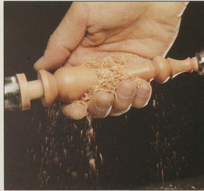
The simplest and most natural finish for a spindle turning is often the one closest at hand. In the photo above, a cherry finial is being rubbed with a palm-full of wood shavings. Natural oils from the shavings will impart a warm, burnished glow to the wood.
