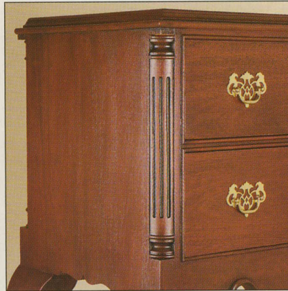
Quarter columns add a visual framework to fine furniture such as the Queen Anne chest of drawers shown above. The columns are made from a single blank sawn in four, then glued up, turned on the lathe, and pried apart.
