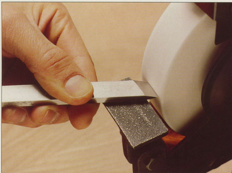
The grinder is a multipurpose tool for the wood turner. Here, the nicked cutting edge of a skew chisel is squared before grinding the bevel.
