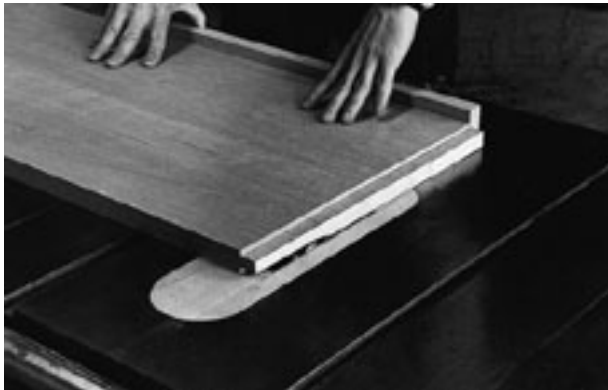
7 Rip and crosscut the headboard stock oversize. Cut joining plate slots in the stock, then glue and clamp the stock.
