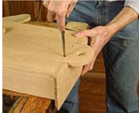
The back is screwed only near the center. The edges are then nailed into place, allowing for seasonal movement.
