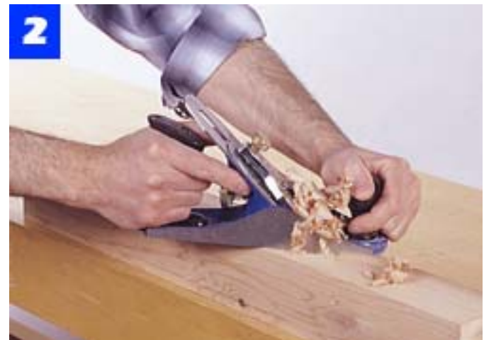
Clamp a table leg to a benchtop and remove saw marks with a hand plane. To make a smooth cut, push the plane at an angle.
