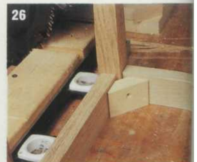
26 Glue the skirts to the legs, and the braces to the skirts. If the corner braces don't set squarely against the skirts, place and draw up the cable screws lightly to hold the braces in place. Tighten the band clamp.
