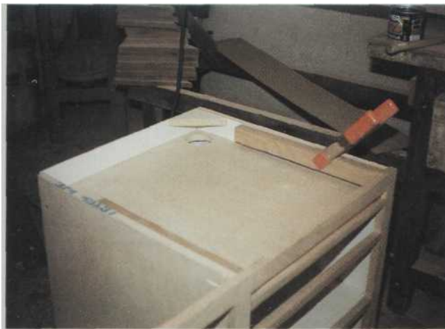
4 The drawer assembly (R & S) being held in place with squeeze clamps.
