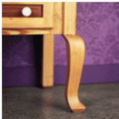
Creative cabriole legs cut from a template refine the vanity's stance and give it a furniture-like appeal
