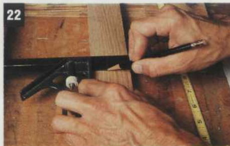
22 Measure an 11½" length on the 1" x 2" x 48" skirt piece. Square the mark and cut. Repeat for the remaining three skirt pieces. Now's the time to check the skirts and legs for blade burn, and sand the faces if needed.
