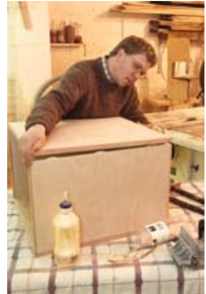
During the second stage of cabinet assembly, laying the cabinet on its side keeps you from fighting with gravity. The cabinet comes together relatively easily, and the alignment is a snap thanks to the biscuits.
