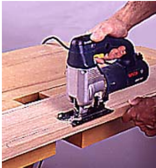
5--Cut the upper base to size and bore a 9/16-in. hole through its centerpoint. Attach it with glue and screws.
