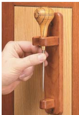
Scratch awl. An open hole traps the handle of this awl. And to protect your hands (and other tools), the point sits in a base.
