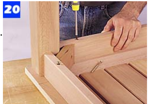
Attach the tabletop to the base with several screws. Drive each screw into its matching counterbored hole the apron.
