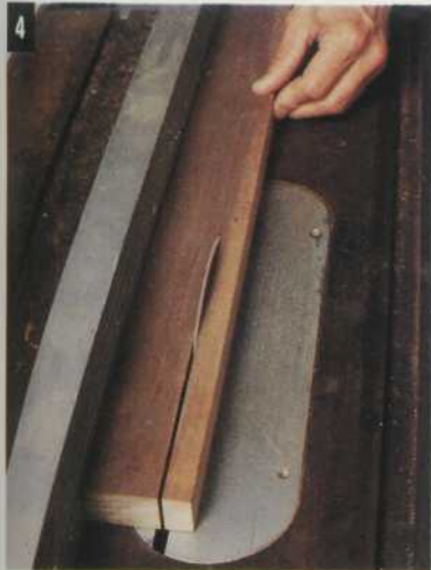
4 Rip the walnut into 1 3/4" strips and cut them into four 18" lengths.
