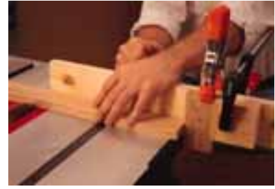
Here I'm cutting the A2 piece with one of the spacers in place. To cut the A3 piece, use two of the spacer blocks.
