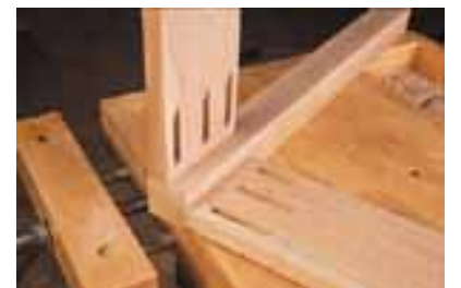
Pocket screws aren't my first choice for building dining tables, but for a small occasional table, it'll work.
