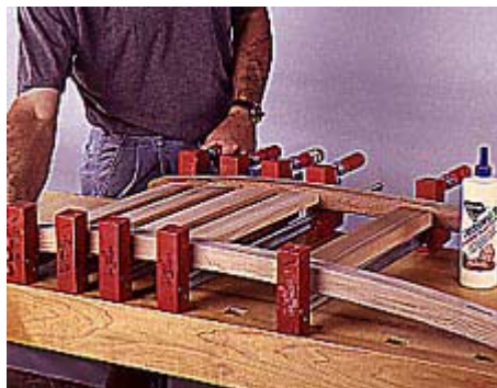
17 Glue and clamp together two side stretchers with a cross stretcher. Check the assembly for square.
