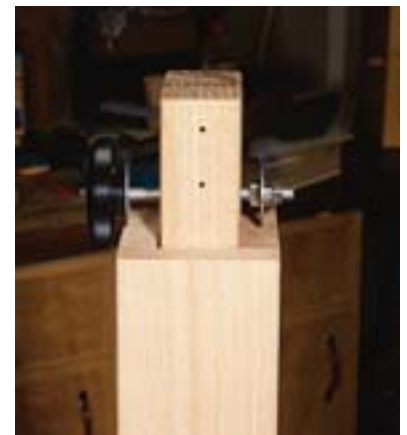
Some simple hardware from your local home center store allows you to lock the post solidly, but quickly loosen the post and readjust for any height. The hardware is shown at right, resting on top of the
