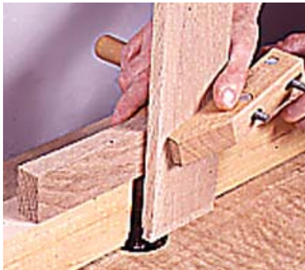
13--Rout slots in the drawer face for the drawer sides with a dovetail bit. Use a square U-shaped jig to guide the router.
