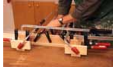
Here I'm clamping the E and D pieces together. Use spacers on the ends of the D parts to hold them in place against your gluing jig.
