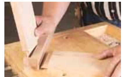
Mitered mortise-and-tenon joinery is common on tables with thin legs or when your set back is deeper than normal.
