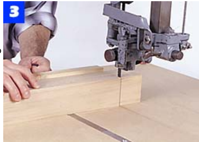
Crosscut the legs on the band saw. Here, a shopmade crosscutting table and a miter gauge are used to make the cut.
