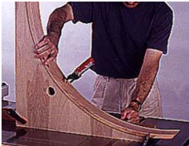
5 Clamp the laminate strips at either end to keep them from shifting. Apply pressure with equally spaced clamps.
