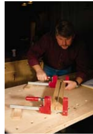
To form the post, the rough piece is ripped into three pieces, the center piece is cut to form two small blocks, and then the whole thing is glued back together.
