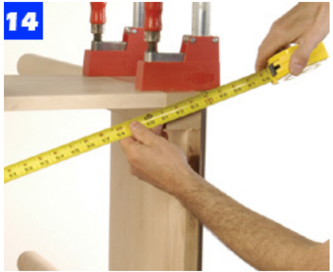
Complete the table base by joining the back subassembly to the sides and partitions. Then check for square.
