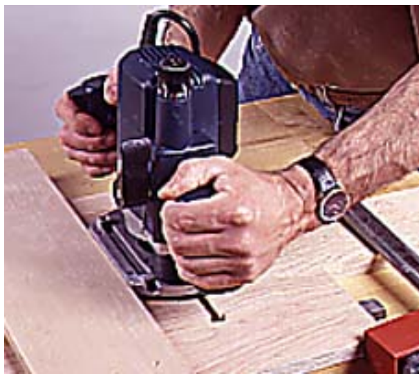
13--Rout slots in the drawer face for the drawer sides with a dovetail bit. Use a square U-shaped jig to guide the router.
