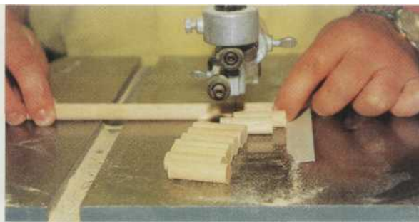
9 1 1/2" dowels, cut on the band saw, help make the joint stronger.
