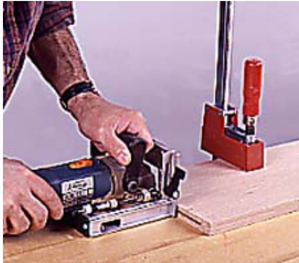
5--Clamp the bottom shelf securely to a workbench. Then use a plate joiner to cut joining slots in both ends of the shelf.
