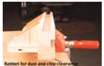
ROCK SOLID The fence is made of a sturdy, stable hardwood. Cut a groove the length of the top and face of the fence. The grooves support T-slot tracks, which can be used for stops, hold-downs and other accessories.
