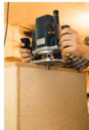
Go slowly while rounding over the edges, as the cherry can tear out and splinter if a cut is rushed. The roundover is key to the smooth, clean feel of the piece.
