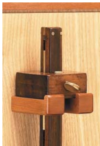
Marking gauge. For this marking gauge, a notched block supports the head, and a small lip keeps the tool from sliding off.
