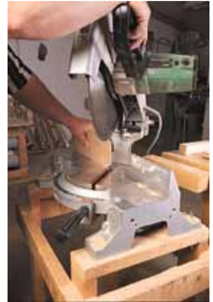
When you have to use mitered mortise-and-tenon joinery, don't get too worked up about the fit of the miter. You don't want the miter too tight.
