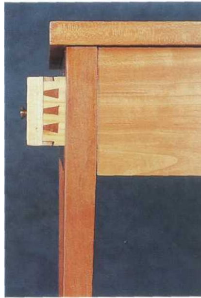
This close-up of the drawer side shows the cock bead inlay around the drawer.
