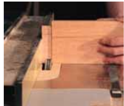
Cut 1/2" shoulders on each side of the aprons.
