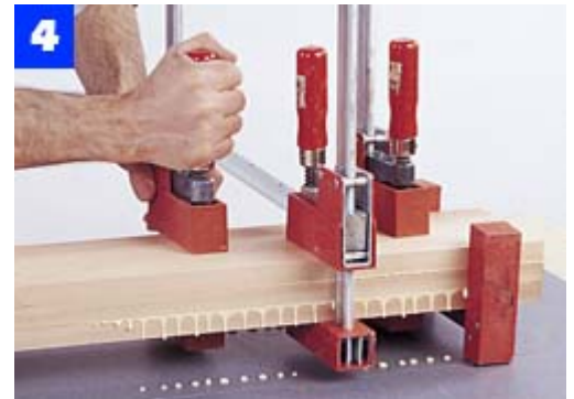
For the bench legs, spread glue on 3/4-in.-thick stock. Lay disposable material under the pieces and clamp them together.
