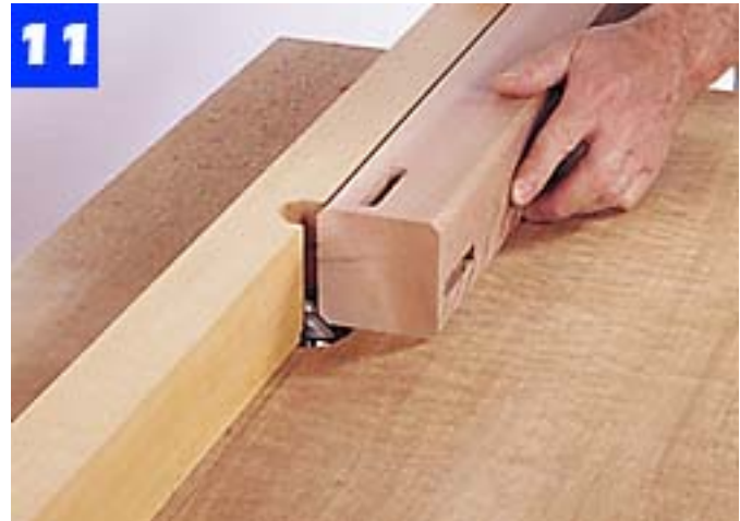
Use a chamfer bit in the router table to cut the chamfer on all four edges of the legs for the benches and table.
