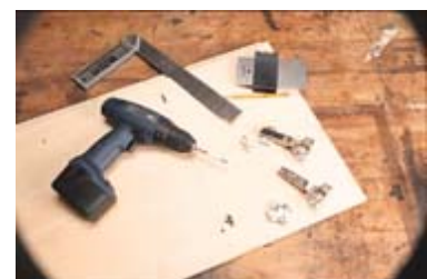
SHELF PIN SETUP • Before assembly it's best to mark and drill the locations for the shelf pins, and to lay out and mount the base plates for the hinges. As always, a little masking tape on the drill bit makes a handy depth stop.
