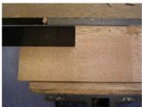
And checking flatness along length of two faces to be joined.
