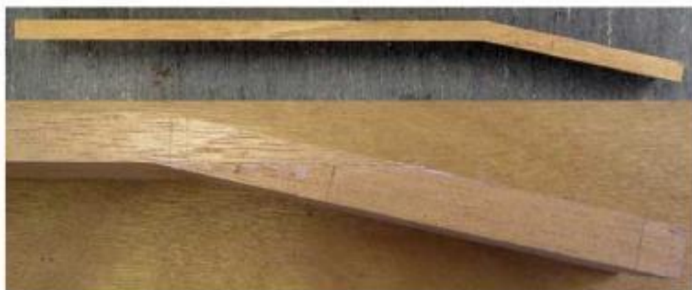
Neck Scarf Joint Completed.
