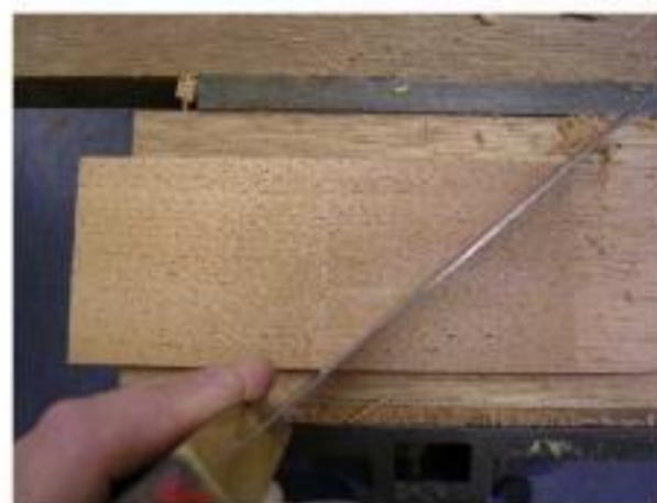
Checking both separate faces of the scarf joint from corner to corner.
