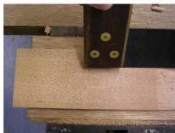
And checking flatness along length of two faces to be joined.
