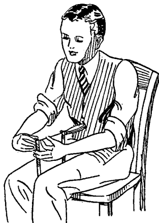
Fig. 2.—How to fix the sawblade.
