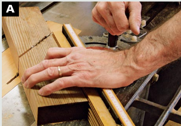
CUT THE ANGLE Use the miter gauge to cut angles on 2x4 stock.
