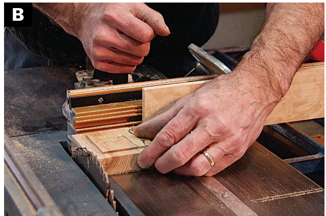
CUT THE TOP TO SHAPE To cut the top to a more interesting shape, angle the tablesaw blade to 9 degrees. Leave enough edge on the sides of the lid to follow the fence during each cut.
