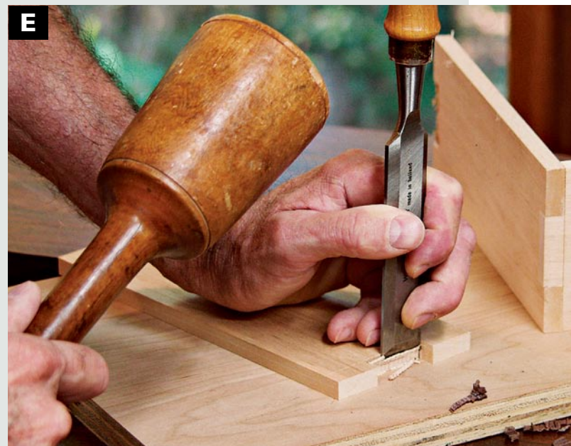
CLEAN UP THE CUT As in cutting this joint by hand, set a wide chisel in the marking-gauge line to clean up the cut. Cut in first from the inside face of the stock, then flip the stock over and cut from the other side.
