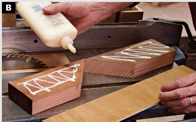
GLUE UP THE JIG Arrange the angled pieces to make a cradle, then add glue to attach the back.
