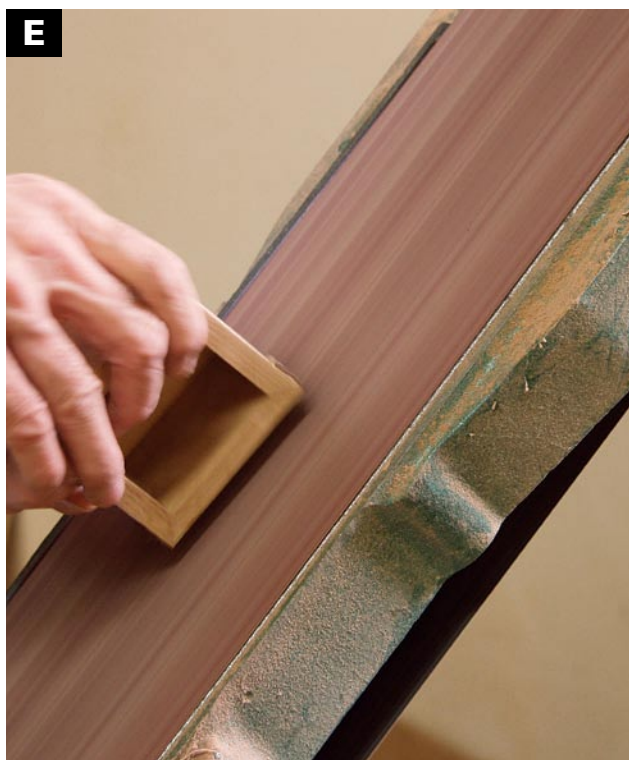
E SAND THE KEYS FLUSH WITH SIDES Use a stationary belt sander to sand the keys flush with the surrounding box sides. Sanding by hand is a little slower, but it works as well.
