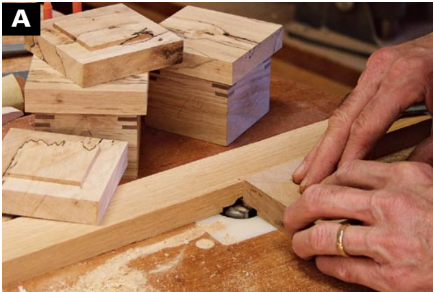
FIT THE TOP Use the router table and a straight bit to rabbet the lid. Rout the end grain first so that the routing of the side grain will remove any tearout resulting from the first cuts.
