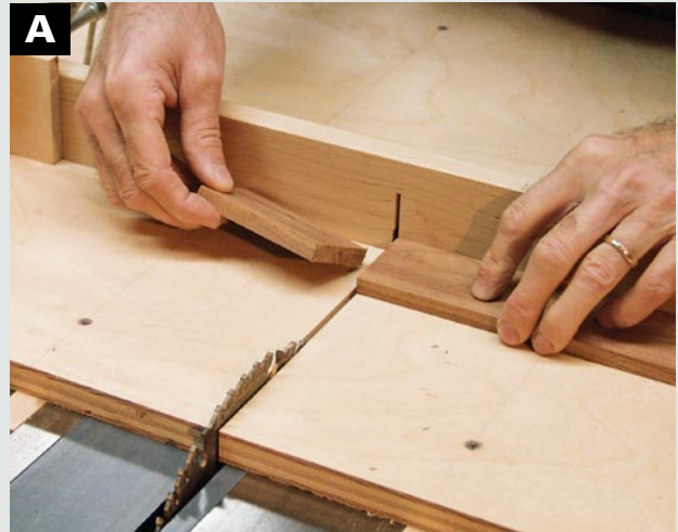
SLEDS ARE SAFER Sleds allow you to pull small parts safely away from the blade before removing them.
