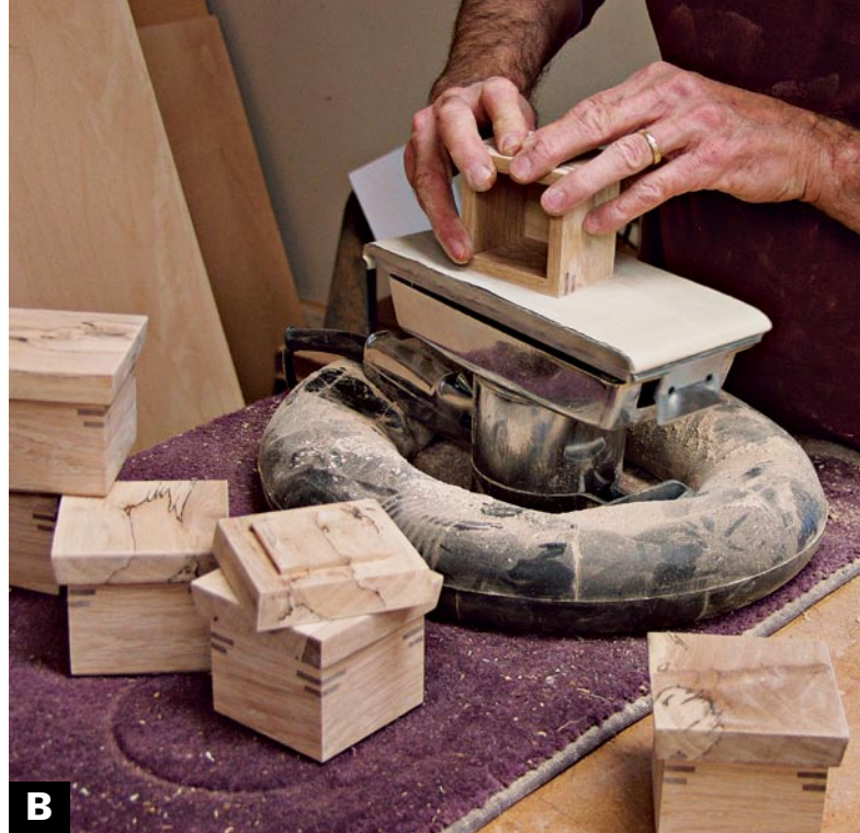
B SAND TO 320 GRIT An inverted half-sheet sander clamped to the workbench is used to smooth small boxes in a short amount of time.
