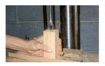
The hole for the leg on the Mook Yan Jong, must be slanted at a 14° slope. To achieve this, your pilot hole must be made using a wooden guide. One can easily be made by drilling a hole with the boring bit into the end of a 3"x 2"x 2" block of wood.
