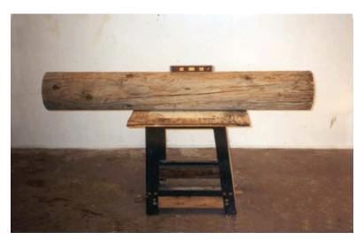
Lay the body horizontally. It is important whenever drilling a hole, to be sure that the body is level.
