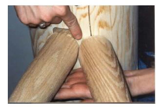
Notice that the 2-1/2" diameter on the top two arms prevents them from being inserted all the way in. It seems as though the holes were too close together. That is not the case. It is necessary to sand some excess material off where the arms meet, so that they fit in the holes at the same time, and so that there is some play between them.
