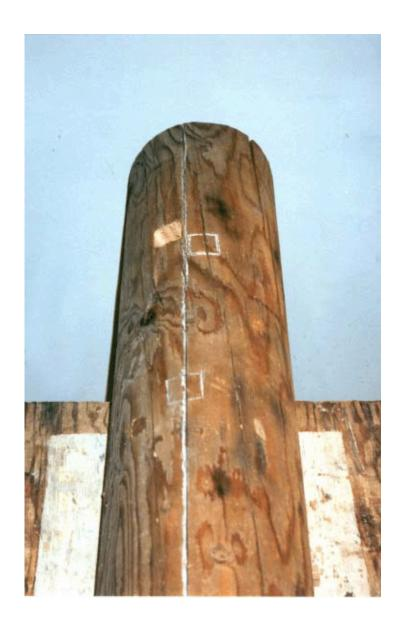
Be aware that since there is no distance between the bottom of the first armhole, and the top of the second, the two holes will literally meet in the middle of the dummy, creating a diamond shaped passage from one hole to the other.
