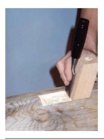
With a pilot hole drilled, chiseling out the rest of the hole is much like chiseling the armholes, except one must be careful to create this hole with the 14° angle. The wooden guide you created is useful in this process. Use the guide by laying it on the surface of the body, at the top of the leg hole and begin chiseling out the hole.
