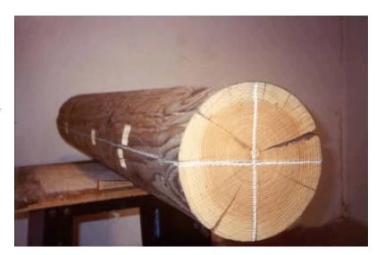
Mark the holes as shown on the plans at the back of this book. Be sure that the holes are off centered and toward the back of the dummy. You cannot, however, use a 1-1/2" boring bit. You'll have to go with a smaller one. Drill a pilot hole and chisel out the corners as you did with all the previous holes.
