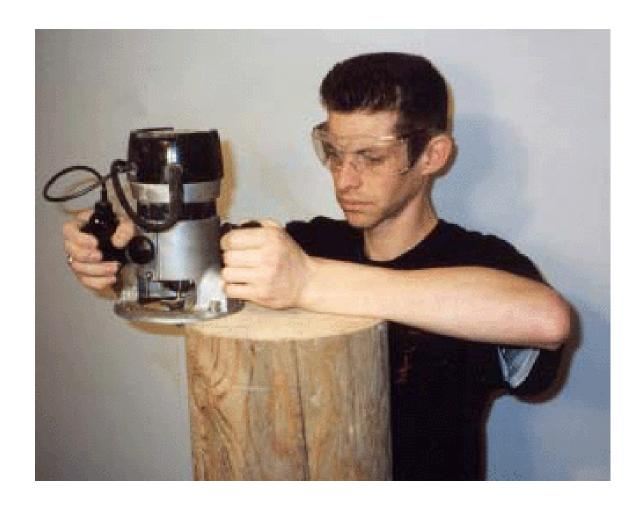
You are now just about finished building the body, and the only thing left to do is to use a router to round off the edges on the top and the bottom of the dummy. Sanding them down instead works just as well, but it takes somewhat longer.
