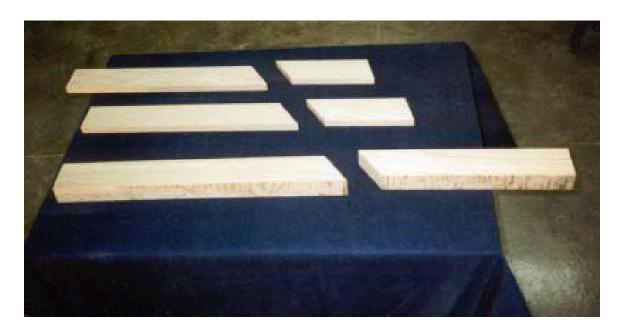
Start with two 3/4" thick boards, and a  $1 \frac{1}{2}$ " board. The thicker board will also be longer. Refer to the plans to determine the length of the boards. Cut them at a  $45^{\circ}$  angle.
