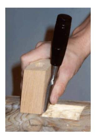
Then move the guide to the bottom of the hole and use the back edge of the guide, begin chiseling out the bottom of the leg hole. This process will help you start the leg hole at the correct angle.
