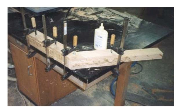
Next, simply laminate the leg in the configuration as shown on the pictures. Use plenty of wood glue and camp the leg tightly. Let dry the entire assembly dry completely.
