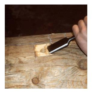
Next, Begin to carefully chisel the square shape of the hole and continue chiseling down all the way through the body.
