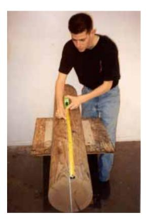
Using these lines as the main guides, draw where the holes for the three arms and the leg will be, as shown on the plans.
