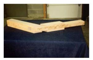
The two above photos show different views of how the joint will come together. The photos show a disjointed fit, in order to illustrate the individual board. Note that the boards alternate at the joint. This layering process can just as easily be done in four layers if using only 3/4" thick boards, just keep consistent with the concept of layering the leg.
