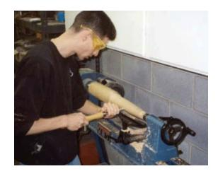
Stop often and check your progress by measuring the diameter with calipers. When the lathe work is finished, take the arm and cut off the excess wood on the tapered side.
