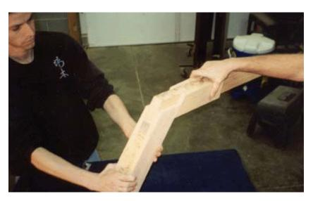
The photo at the left illustrates the leg and how it comes together. All that has to happen now is to slidethe two lower outside pieces up into place
