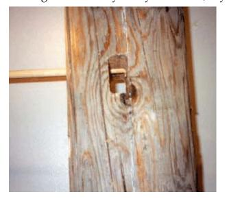
crosspiece, you should see about half of your dowel hole is invading the hole for the crosspiece. Then, insert and glue a 5/8" dowel into the hole you drilled, use a coping saw to cut off the excess, so that the dowel is flush with the body. The process is the same for the bottom dowel hole.
