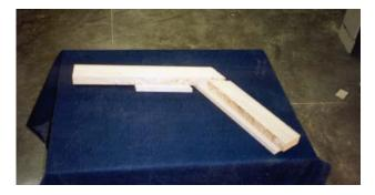
Now assemble the leg pieces into place. When done correctly, you will have the leg in its entirety placed together without glue as shown below.
