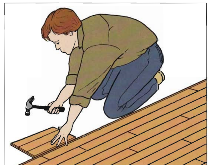
4. Tap the joint tight along the entire run of planking with a hammer and block made from scrap flooring.
