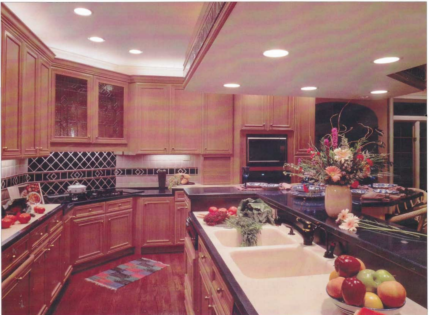
An abundance of recessed canister lights, cove accent lighting, and under-counter task lighting enhances this room's design and function.
