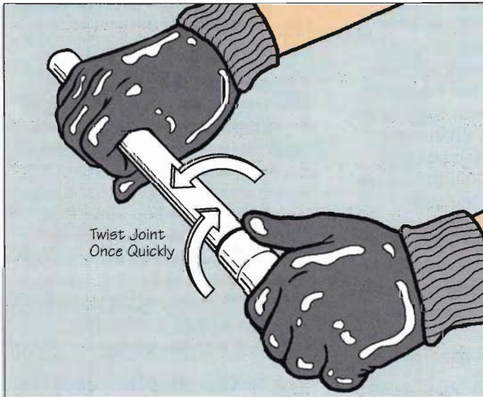
5. Insert the pipe into the fitting, and twist one-quarter turn. Hold the pieces together for 10 seconds.
