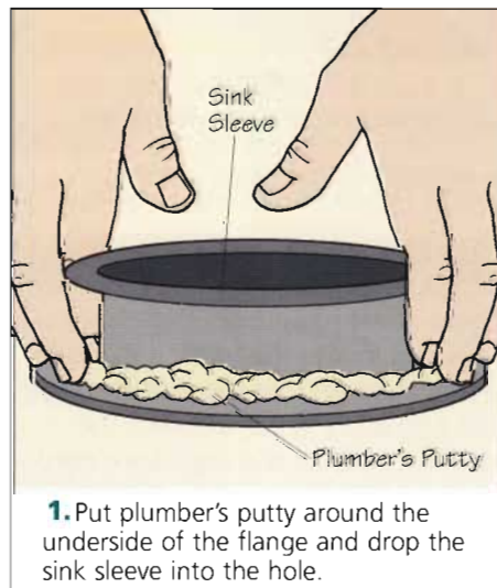
Waste-Disposal Units. A batch-feed disposer, controlled by a wall switch, is the safest and most efficient to use. It's installed on a sink with hardware that includes a sink flange, gasket, and mounting rings, and connected to the sink's drainpipe through the discharge tube.
