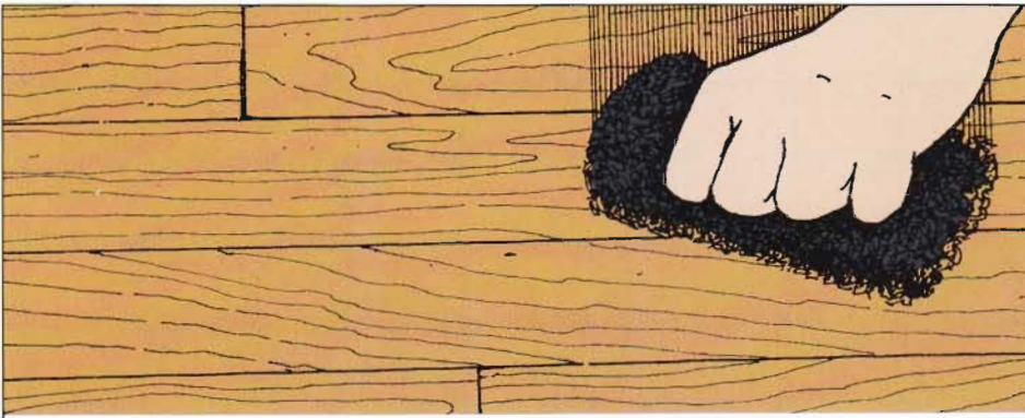
Applying the Filler. Steel wool or burlap will force filler into pores of wood. Rub across grain to force filler in; rub with grain to remove any excess.
