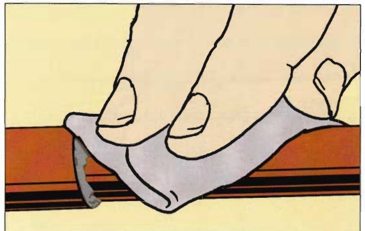
5. Wipe the pipe with a wet rag to cool it, then check for leaks. Stop leaks with more solder; if that doesn't work, redo the joint.
