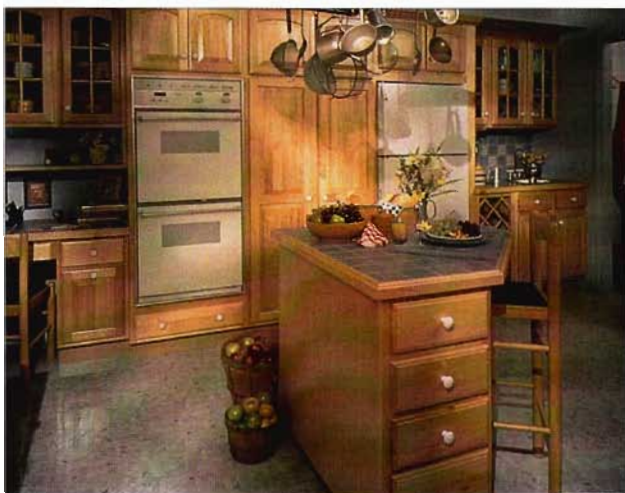
Wall units allow two ovens in the space of one and give equal access to standing and wheelchair cooks.
