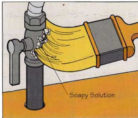
Hook Up a Gas Range. Bend the flexible connector but don't crimp it. Turn on the gas. Test all connections by brushing them with soapy water.
