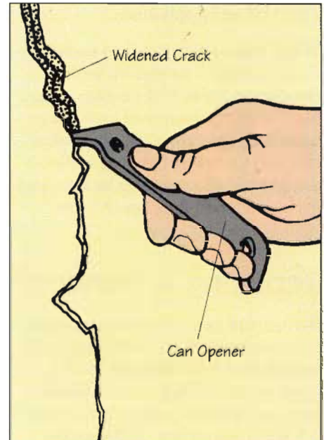
1. Widen hairline plaster cracks with a sharp tool to make a base that will hold the filler.
