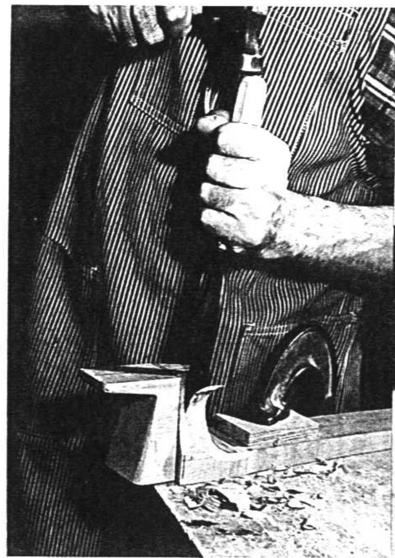
Fig. 59 Rough shaping with gouge
