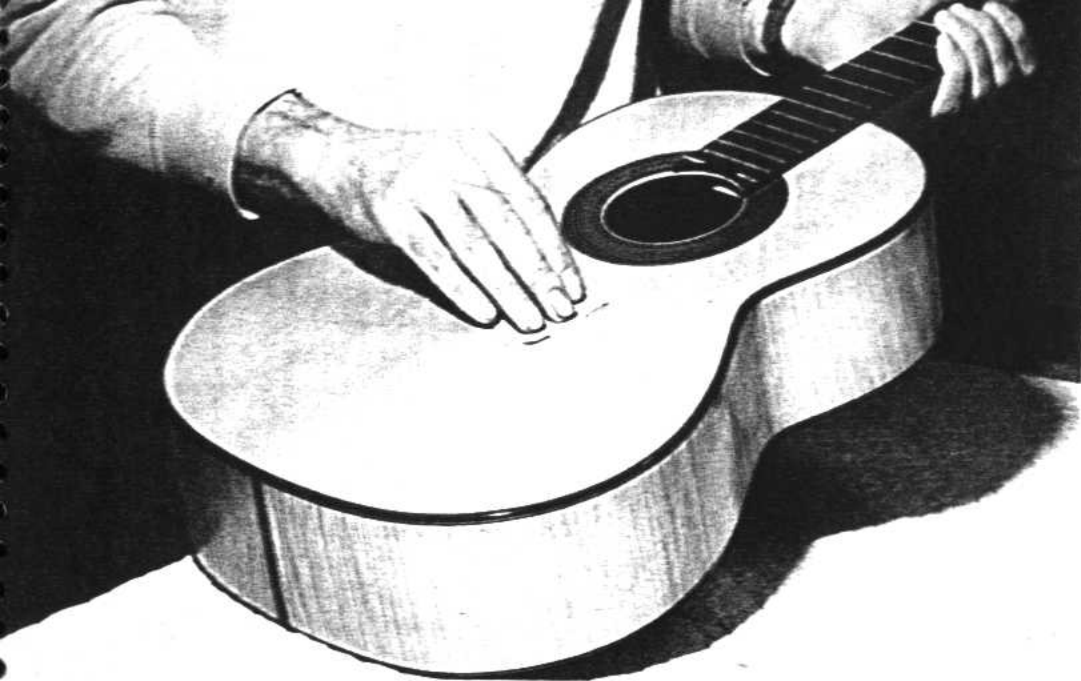
Fig. 124 Final sanding of back
