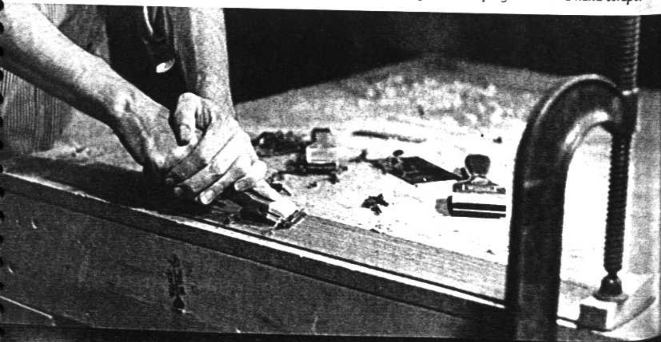
Fig. 34 Scraping side with a hand scraper
