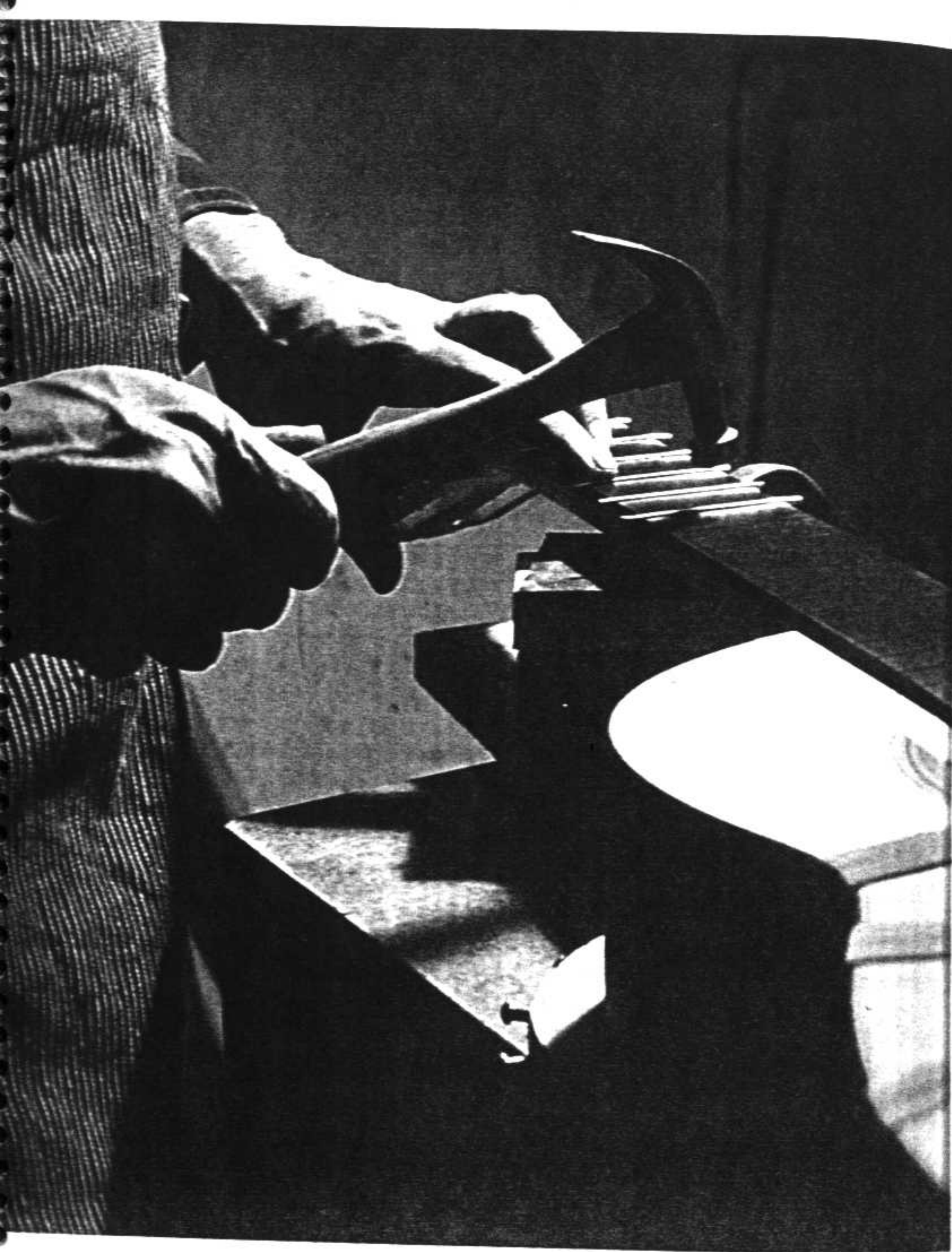
Fig. 99 Hammering in frets over neck support
