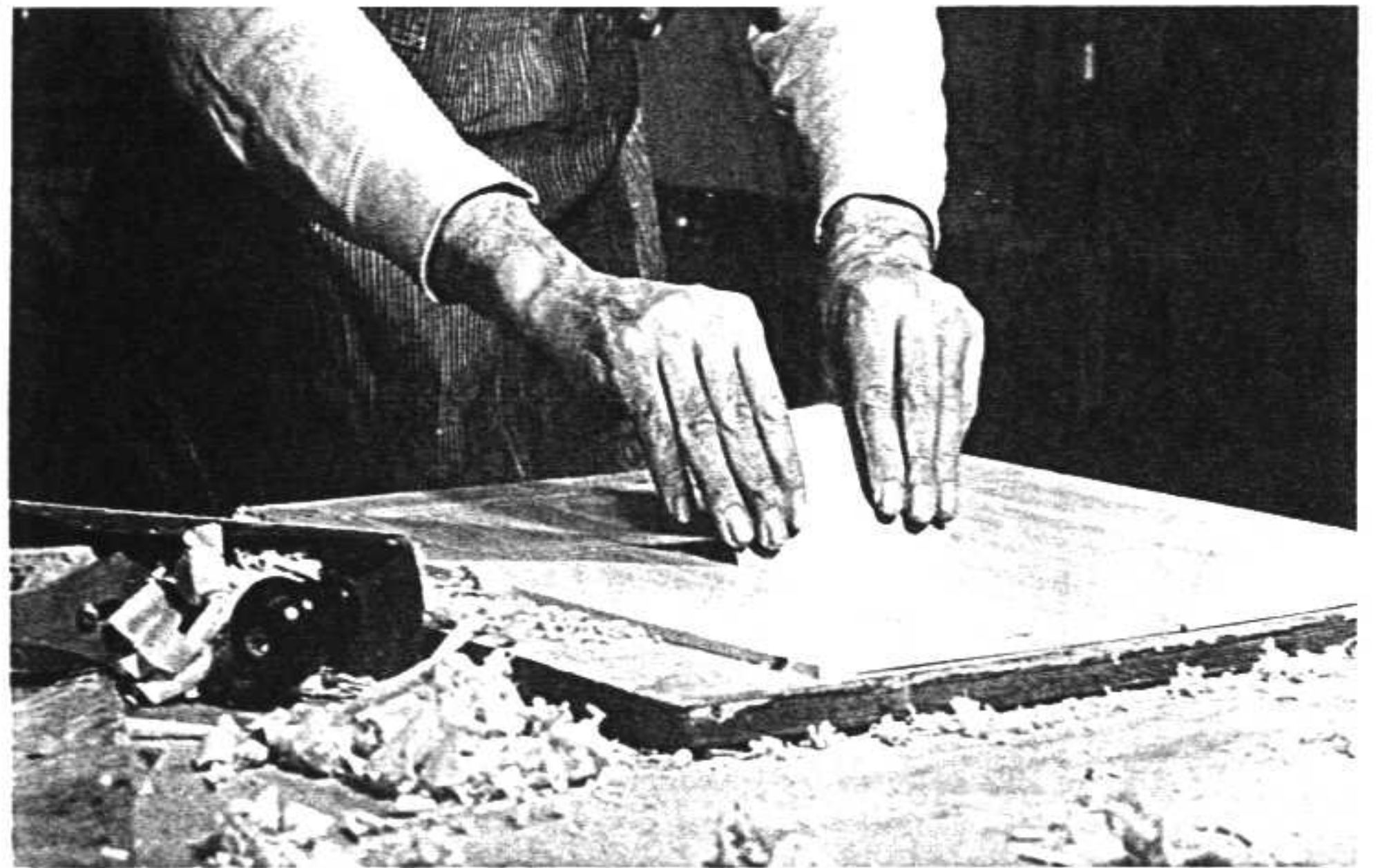
Fig. 36 Final leveling with scraper blade
