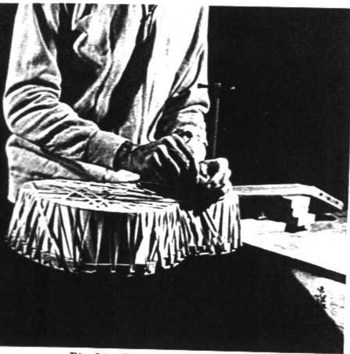
Fig. 84 Clamping glued top
