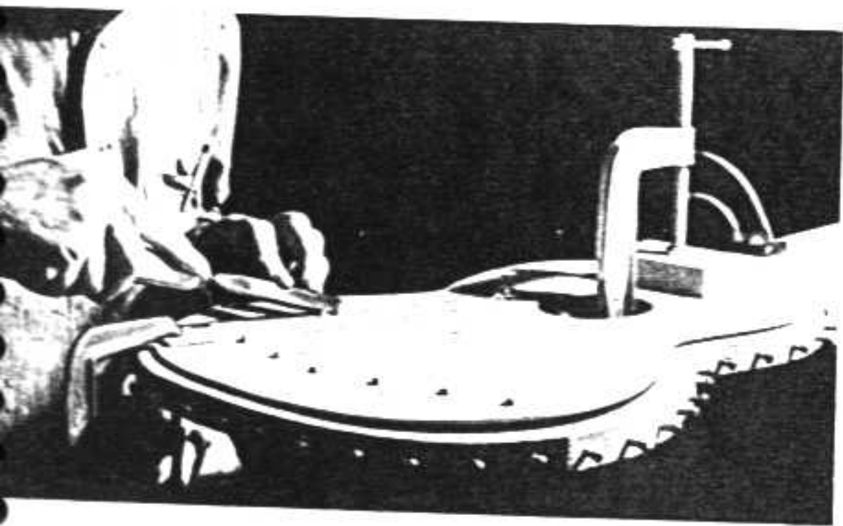
Fig. 78 Chiseling braces to shape
