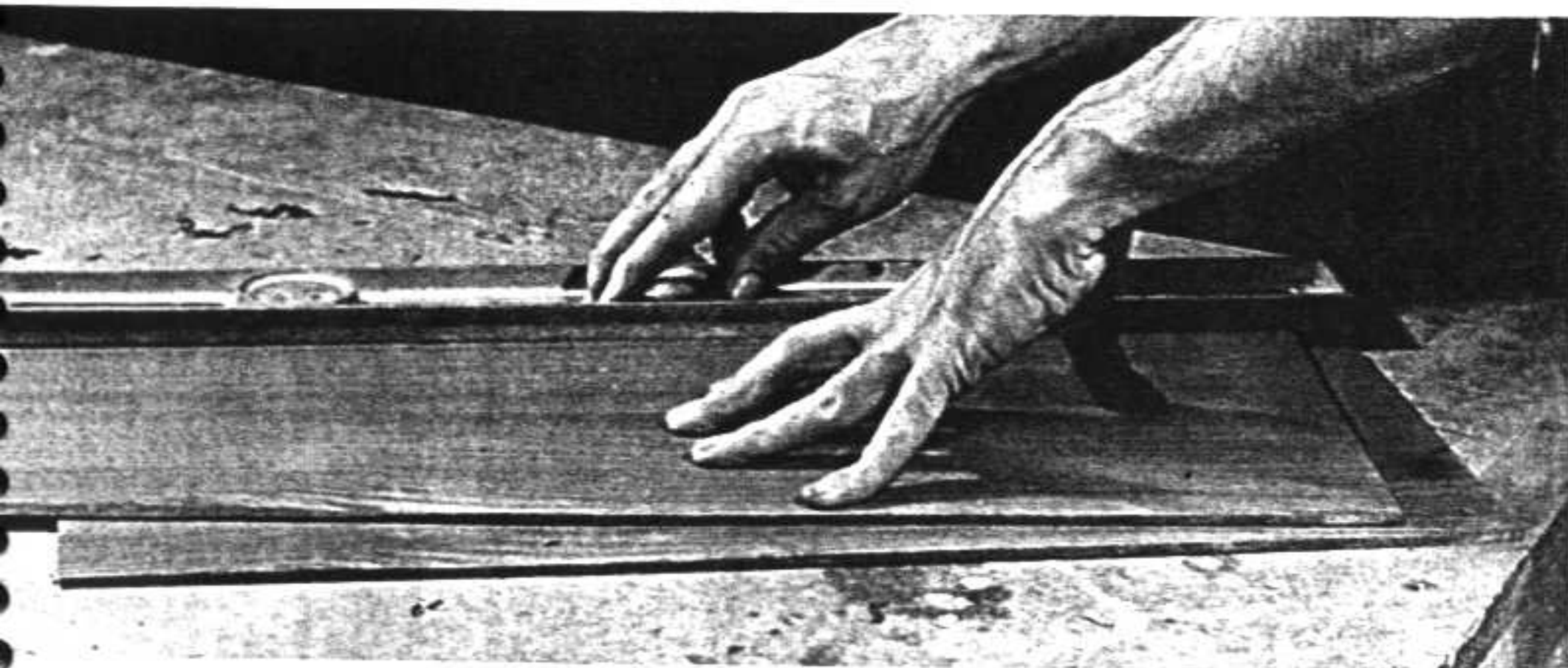
Fig. 37 Sanding edges with level faced with sandpaper
