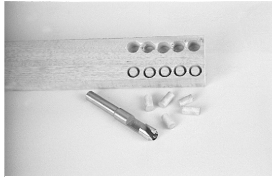
Figure 10.18 Parallel-sided plugs and the cutter used to produce them. Tapered plug cutters produce a very snug fit but in time, as the wood and plug expand and contract in response to fluctuations in RH, the pressure exerted by the taper can cause the plug to become proud of the surface
