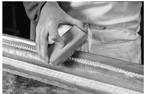
Figure 14.9 Denibbing and buffing dry bole with a stiff brush
