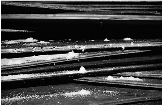
Figure 7.8 Cones of frass produced by the common furniture beetle Anobium punctatum from heavily infested wood
