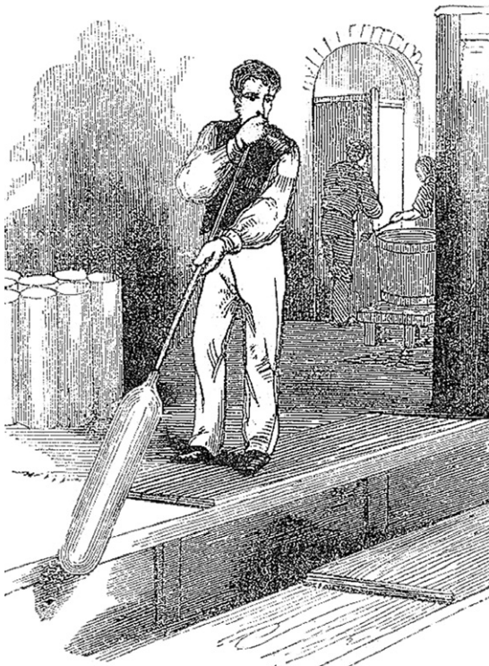
Figure 5.15 Blowing a cylinder for sheet glass. (Illustration from George Dodd (1844–51) British Manufactures , C. Knight and Co., London)
