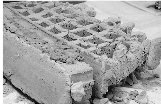
Figure 8.11 Detail of degraded latex rubber cushion for 'Mambo Chair' designed by Michael Inchbald in 1954
