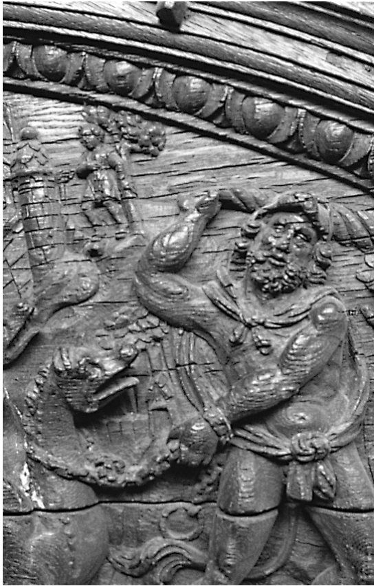
Figure 10.13 Surface checks and splits in a carved oak panel. Such checks may be a result of the use of unseasoned wood or fluctuations in RH
