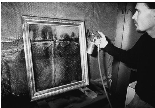
Figure 16.29 Coating and toning of a conserved frame with spray application of cellulose nitrate lacquer
