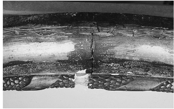
Figure 16.27 Detail of darkened and discoloured brass particle ('bronze') paint on a nineteenth century gilded picture frame
