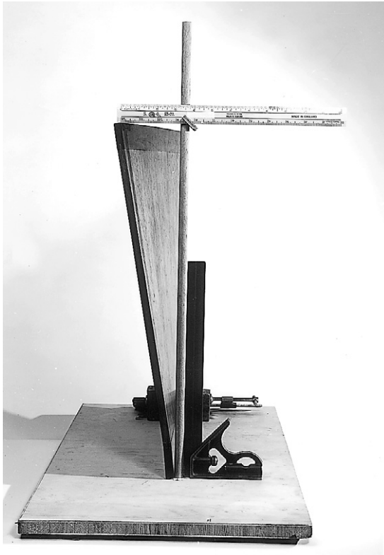
Figure 7.17 Compound warp of approximately 90 mm (3½ in) in a door from a piece of early twentieth-century furniture
