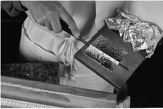
Figure 14.12 Manipulating the gold leaf on the cushion with a gilder's knife
