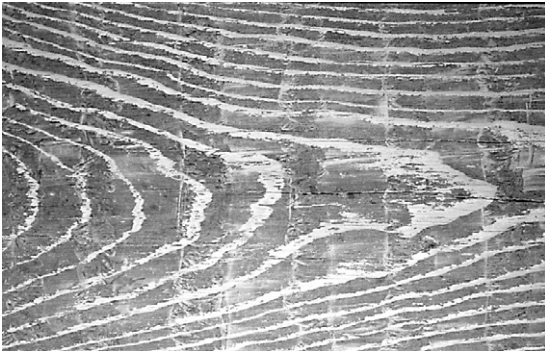
Figure 8.4 Detail of a pine panel from the David Hottenstein House, Berks County, PA, 1783. Woodwork installed as the 'Fraktur Room' at Winterthur Museum in 1952. Poor absorption properties can cause paint loss along the lines of late wood growth, seen here as lighter lines of paint loss contrasting with darker areas where paint remains
