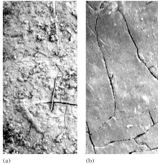
Figure 13.2 Scanning electron microscopy (SEM) photomicrographs of an aged natural resin varnish (a) Before cleaning: accretions darken and obscure the mahogany substrate. (b) After cleaning: accretions have been removed and the original varnish remains intact
