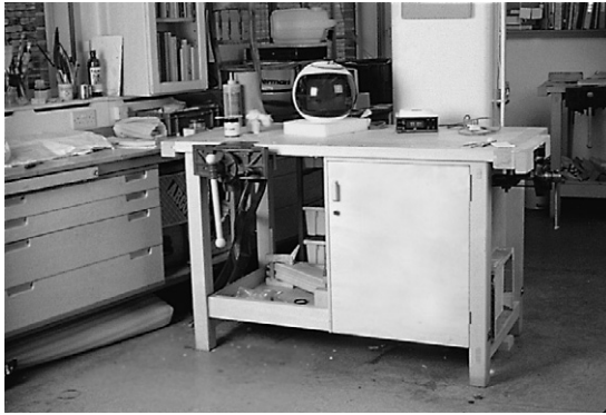
Figure 9.7 A work bench fitted with a pattern maker's vice and end vice
