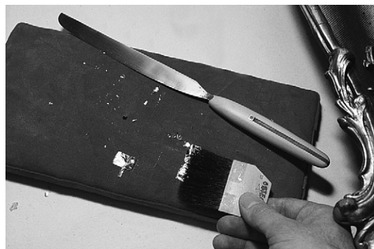
Figure 14.3 A gilder's knife, and a gilder's tip being used to pick up cut gold leaf
