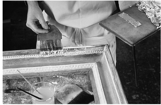
Figure 14.14 Laying gold leaf (water gilding)
