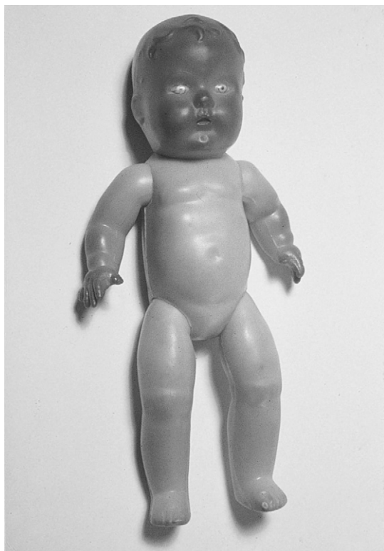
Figure 16.4 PVC doll. Discoloration of the face, arms and legs is a result of photochemical degradation and cannot be removed by cleaning
