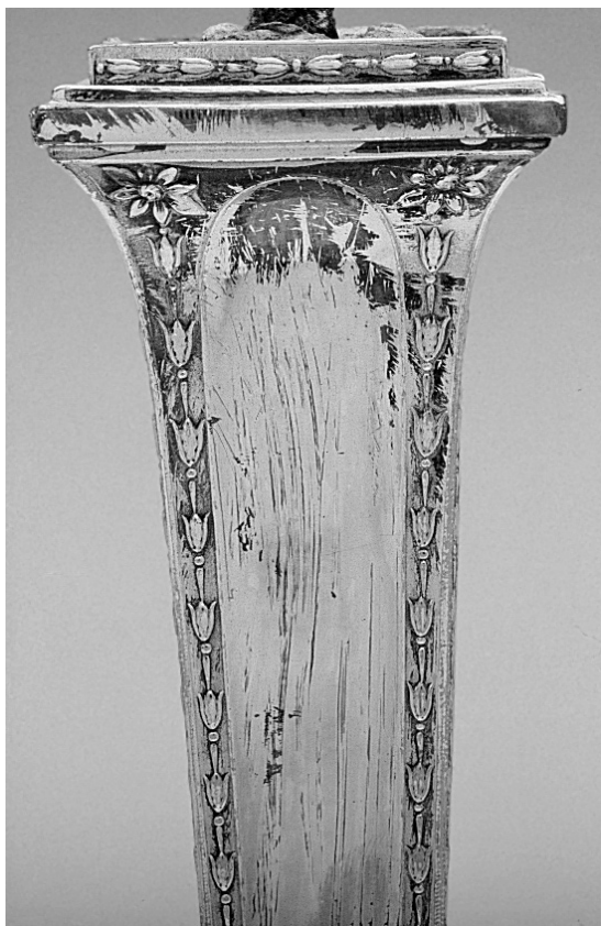
Figure 15.7 An eighteenth century Sheffield silver-plated candlestick. Preferential corrosion has occurred as a result of poor application technique when the object was lacquered
