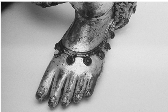
Figure 15.12 Eighteenth century statue of Tara, Nepal (a) Detail of foot before removal of corrosion products. The metal is a gilded copper alloy. Corrosion products from the copper obscure the gilt surface (b) Detail of foot of statue, after cleaning. The gilded surface was revealed by the removal of copper corrosion products. This is the type of alloy that might have been cleaned with ammonia in the past but is now more safely cleaned using chelating agents, followed by rinses of deionized water and acetone
