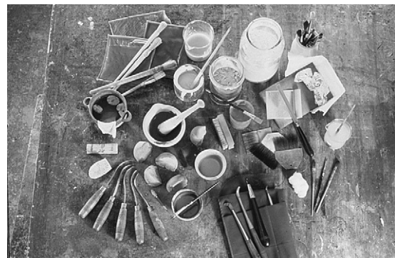
Figure 14.1 A range of tools and materials that may be used in traditional gilding
