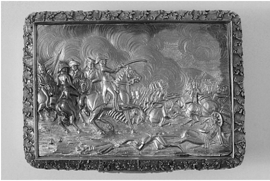
Figure 15.11 A gold snuff box, c.1814. Disfiguring tarnish caused by the corrosion of metals alloyed with the gold
