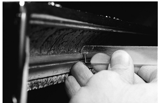
Figure 14.10 Smoothing bole with a Perspex/Plexiglass scraper shaped to fit the profile of the moulding
