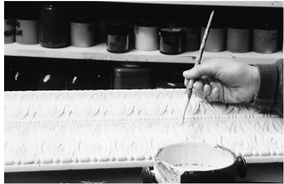
Figure 14.4 Application of gesso to a carved surface
