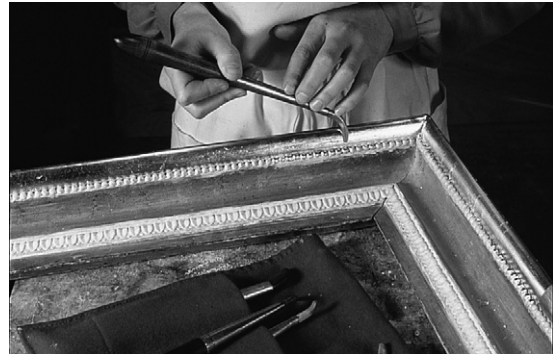
Figure 14.16 Burnishing water gilding using a dog's-tooth agate burnisher
