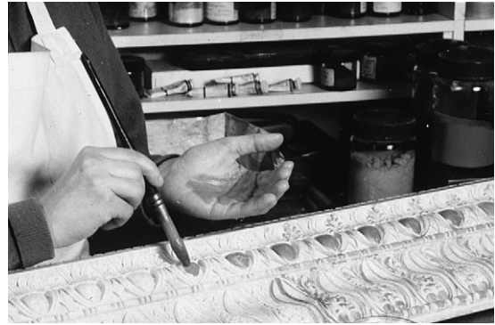
Figure 14.8 Applying a darker bole to highlights of the carved surface
