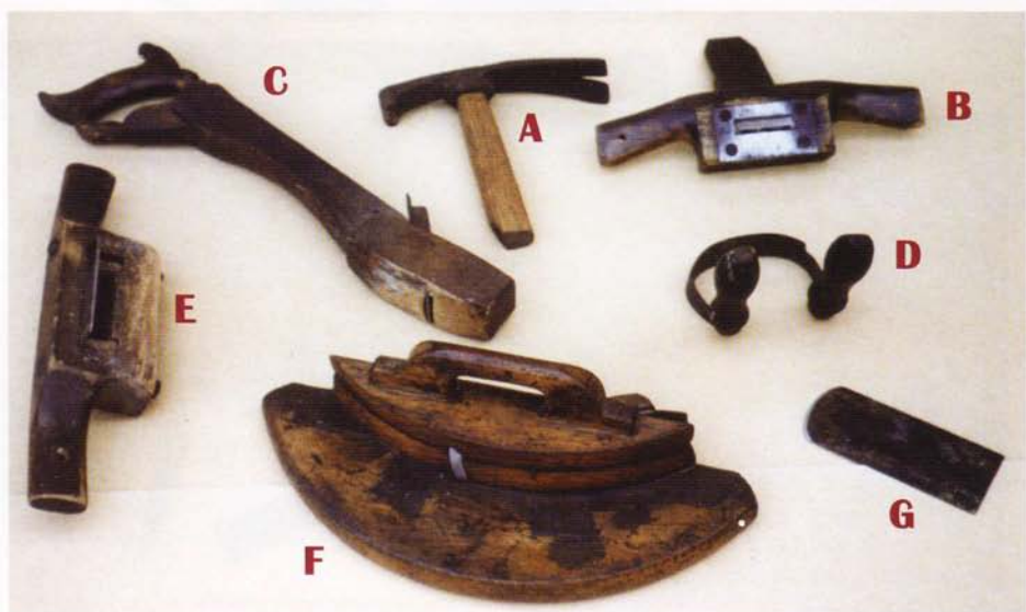
A, dry cooper's adze. B, downright. C, extended stoup plane. D, round shave (smuggling iron). E, buzz. F, herring cooper's flincher. G, scraper.
