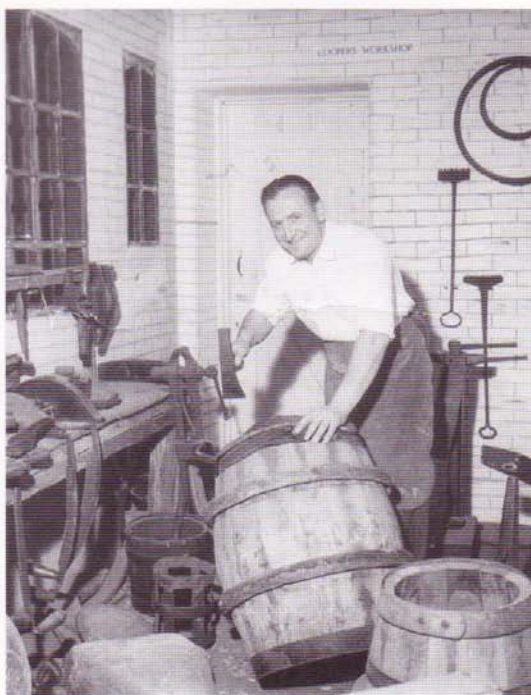
Using an adze to cut the bevel on the top of the staves – chiming the cask.
