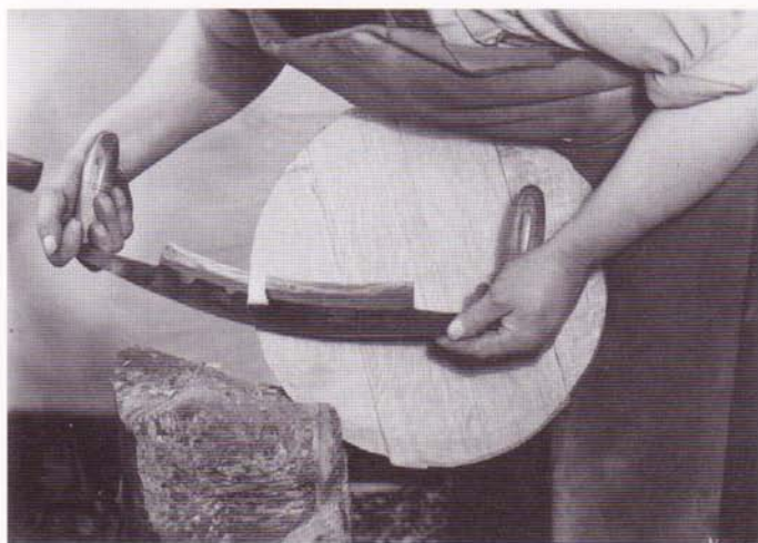
Cutting the outer basil of the head with a heading knife.
