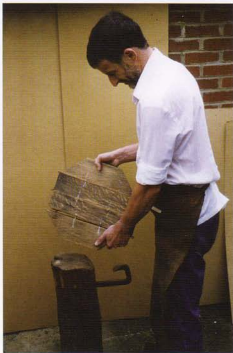
Dowelling together the head. Note the flag in the joint.
