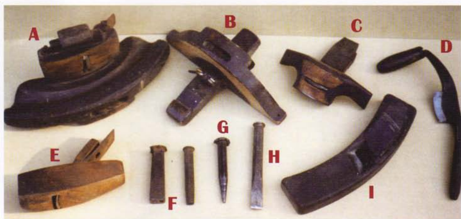
A, chiv. B, croze. C, inside shave. D, jigger. E, stoup plane. F, rivet moulds. G, punch. H, cold chisel. I, topping (or sun) plane.
