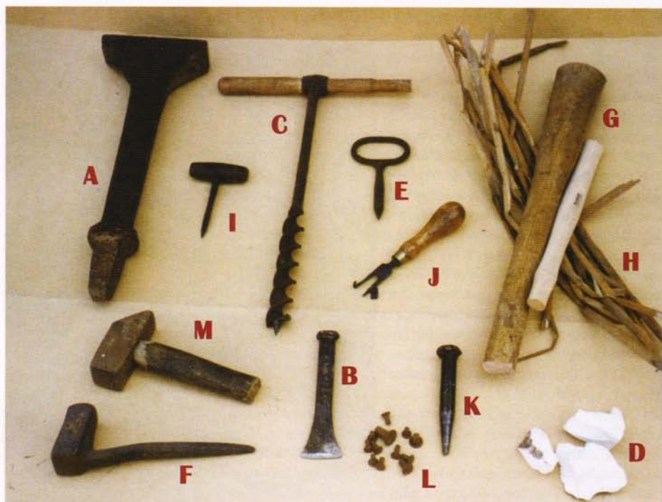
A set of ship's cooper's tools (1861 Admiralty Instructions): A, bick iron; B, bolster or chince; C, bung borer; D, chalk (for helping hoops to stick when being driven); E, heading vice; F, driver; G, helves; H, flag; I, gimlet; J, marking iron (race); K, punch; L, rivets; M, striking hammer.
