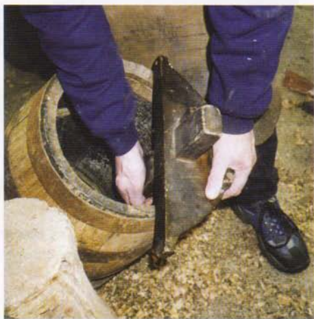
Cutting the groove with a croze.
