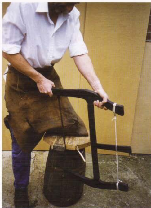
Sawing round the head with a bow saw.
