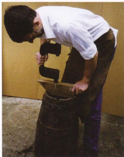
Boring dowel holes on the cant of the head using a dowelling stock.
