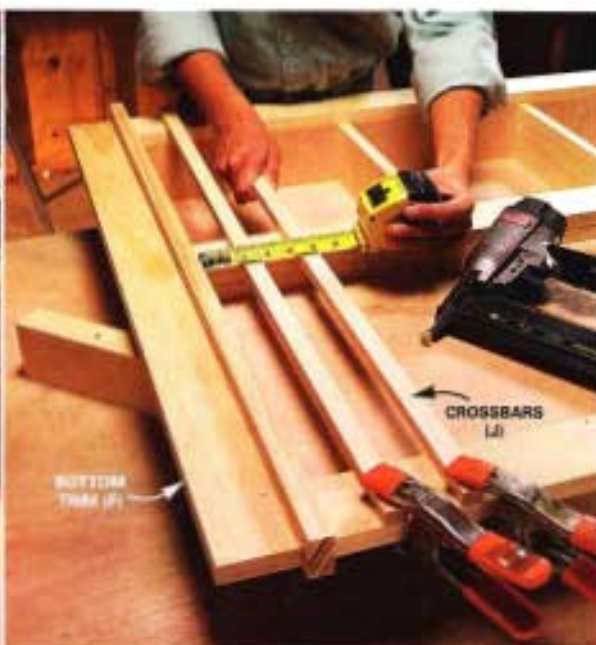
9 Nail on the top and bottom trim (F). Position and clamp the two 1/2-in. x 3/4-in. crossbars (J). Nail with 1-in. brads.
