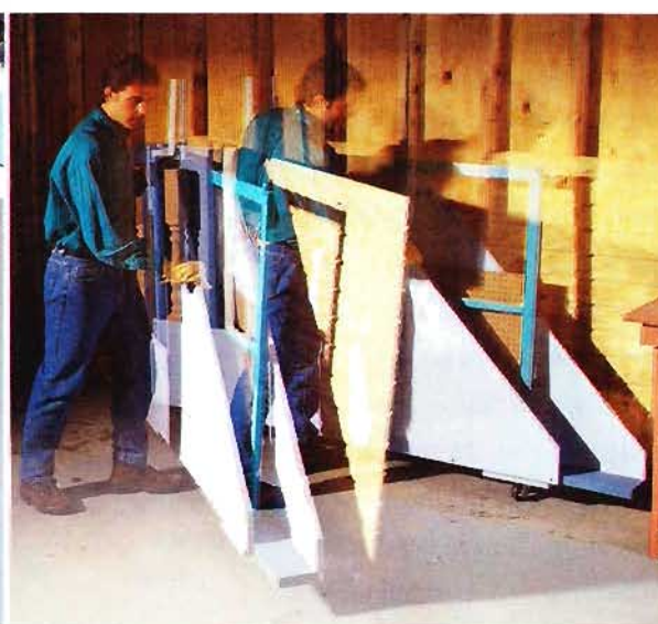
8 Swing the rack out from the wall and load it with plywood, drywall and other big, flat stuff.
