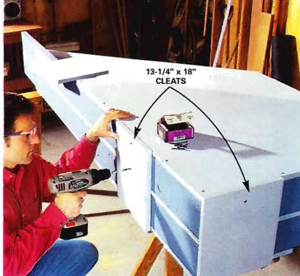
5 Fasten four plywood cleats to the bottom and sides with 2-in. screws to hold the rack together. Use 12 screws per cleat.
