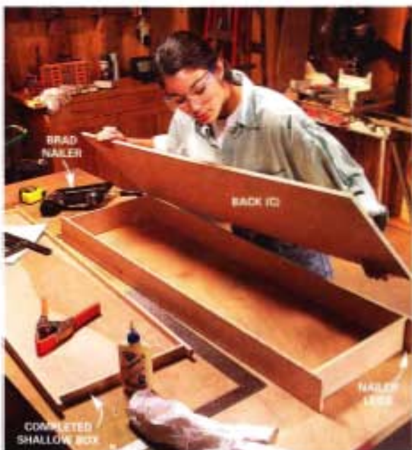
5 Glue and nail the sides, top and bottom first, then glue and nail on the 1/2-in. plywood back (C) to square each box. Wipe off excess glue with a damp rag.
