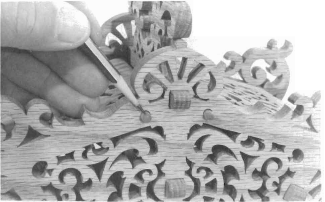
A close-up look at the hinge dowels and the through-mortise and tab construction details.
