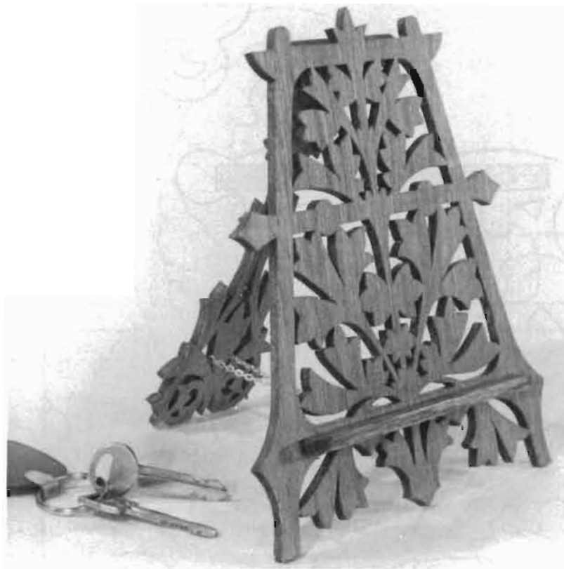
Easel, one of several designs. Make all easels from 1/4"-thick material. Supporting legs or struts can be hinged in several ways. (See the methods of hinging below.)
