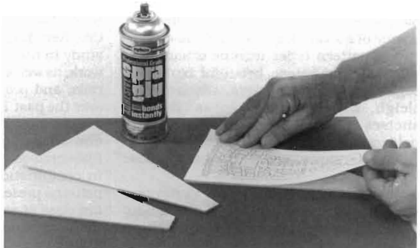
Illus. 3 Pressing down a spray-adhesive-coated copy of the pattern directly onto the wood workpiece blank.
