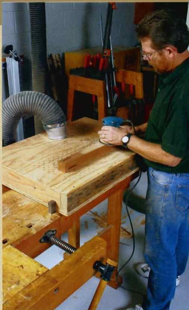
**A DOWNDRAFT TABLE KEEPS IT CLEAN.** The author's sanding table is just a box drilled with holes to suck the dust away. This simple box, made of plywood and 2x4s, hooks up to a dust-collection system or shop vacuum.
