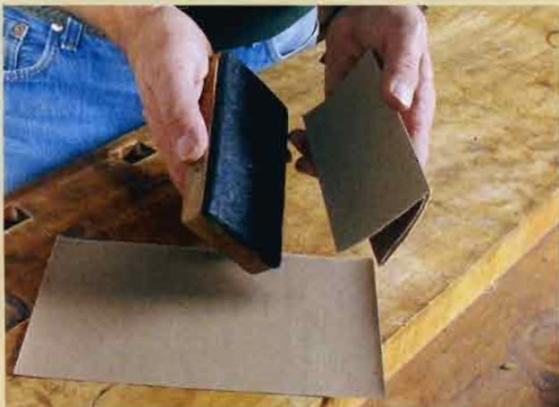
**FOLDED HALF SHEETS FOR A SANDING BLOCK.** Tear paper in half and fold it into thirds, taking care to use every surface before you discard the sheet. Felt on the block evens out the sanding pressure and helps hold the paper in place.
