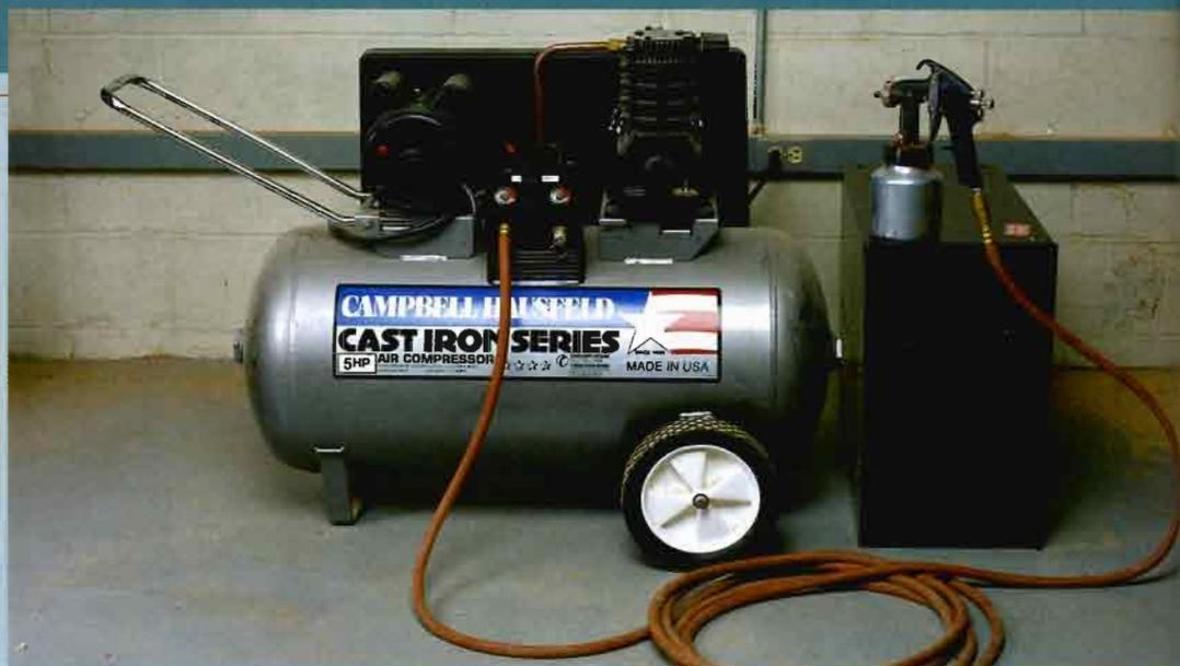
did his own little test when HVLP first hit the market. He painted one cabinet with a traditional, compressor-driven gun and an identical cabinet with an HVLP unit. When he was done, there was three times as much paint left in the HVLP cup. Where was the paint missing from the conventional gun? All over.
