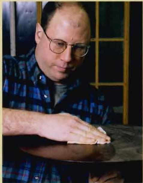
**DON'T USE TACK RAGS TO WIPE OFF DUST.** They can leave chemical residues that will show up as blemishes under a waterborne finish. Use a rag dampened with water.
