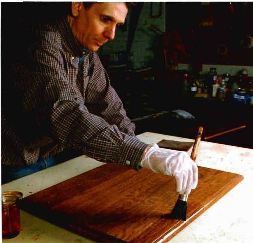
(to make it spray or brush better), but more than that can disrupt the chemical makeup of the finish, which will have a negative effect on how the finish forms a film.
