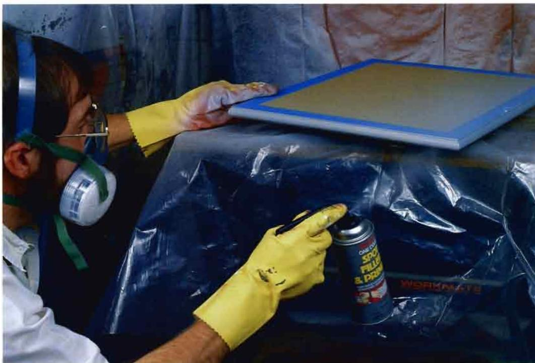
also filled in the knots. No matter how sound they look, knots always have cracks that show through the paint. Knots often contain resins, too, especially in softwoods. So once the filler in the knots had cured (about 30 minutes), I sanded it flush and spot-sealed the knots with shellac just to be safe. Finally, to make the edges of the medium-density fiberboard (MDF) top perfectly smooth, I used some spackle (see sidebar on the facing page).
