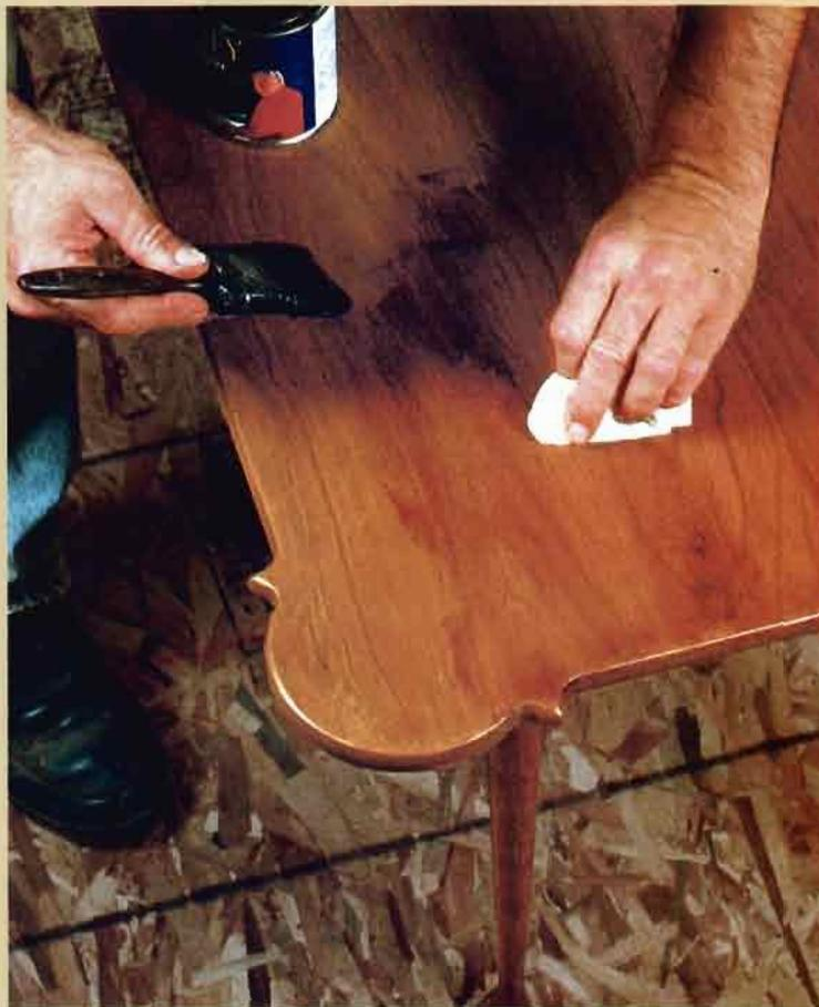
**THE FIRST COAT OF GLAZE.** A brush is used to apply the first glaze coat, a gel stain. The cloth pad allows the author to remove just the right amount of glaze from the surface to get the desired result.
