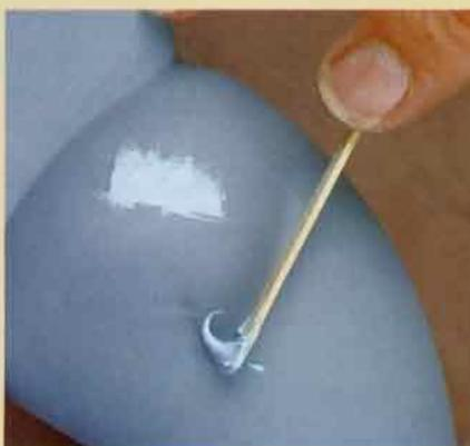
**GLAZING PUTTY SMOOTHS OUT BLEMISHES IN PRIMER.** After Minick primes a leg, he sands it out to reveal tiny surface dents and nicks, which he fills with blue glazing putty. When that's dry, he'll sand, reprime, and then lightly sand again in preparation for paint.
