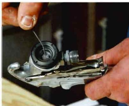
**REMOVE THE AIR CAP AND FLUID NOZZLE.** The inside of the gun is best cleaned with a skinny brush soaked in lacquer thinner.
