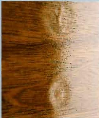
1. Silicone or wax residue from paint stripper or old finish: Wipe surface with mineral spirits; mist coats (let each dry) to trap contaminants.
