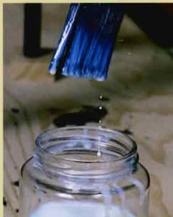
**LET THE EXCESS FINISH DRIP OFF THE BRUSH.** Rubbing the brush against the edge of the container may cause the finish to foam.
