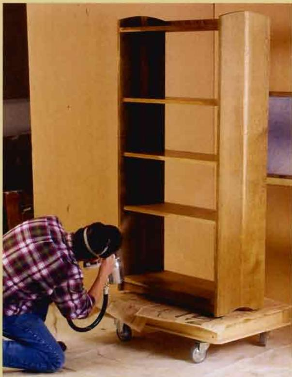
**GET DOWN, AND GET UNDER YOUR CABINET.** Spray the underside of the shelves first (above). Then complete the inside of a cabinet by spraying the sides (right) followed by the tops of the shelves. In this way, the most noticeable surface is sprayed last and won't be affected by overspray.
