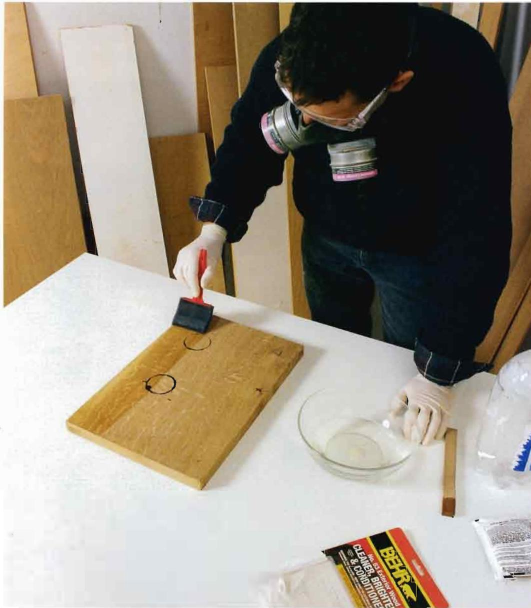
**OXALIC ACID REMOVES THE STAIN** but not the color of the wood. The author used a deck brightener, which has oxalic acid as an active ingredient, on this piece of white oak.
