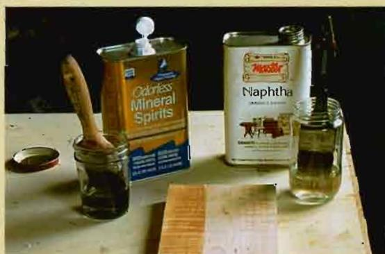
**THE SLOW AND THE FAST.** Mineral spirits and naphtha were simultaneously brushed onto a board. Three minutes later, the naphtha had almost evaporated, while the mineral spirits was still wet.
