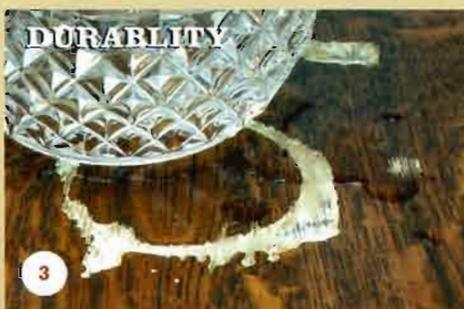
redissolve in the solvent originally used to thin them. Except for the pure oils, reactive finishes tend to hold up better to heat and chemicals.
