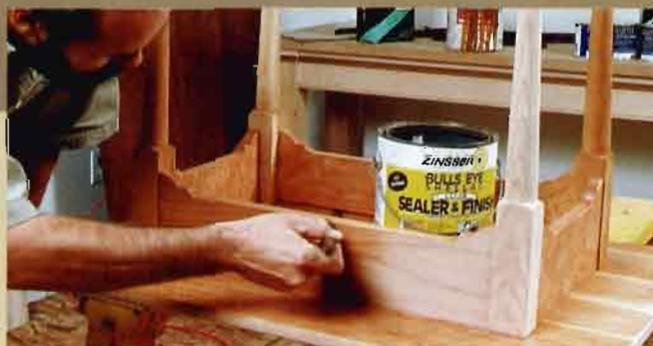
**BRUSH ON SHELLAC.** A washcoat of thinned shellac added before the stain helps control blotching.
