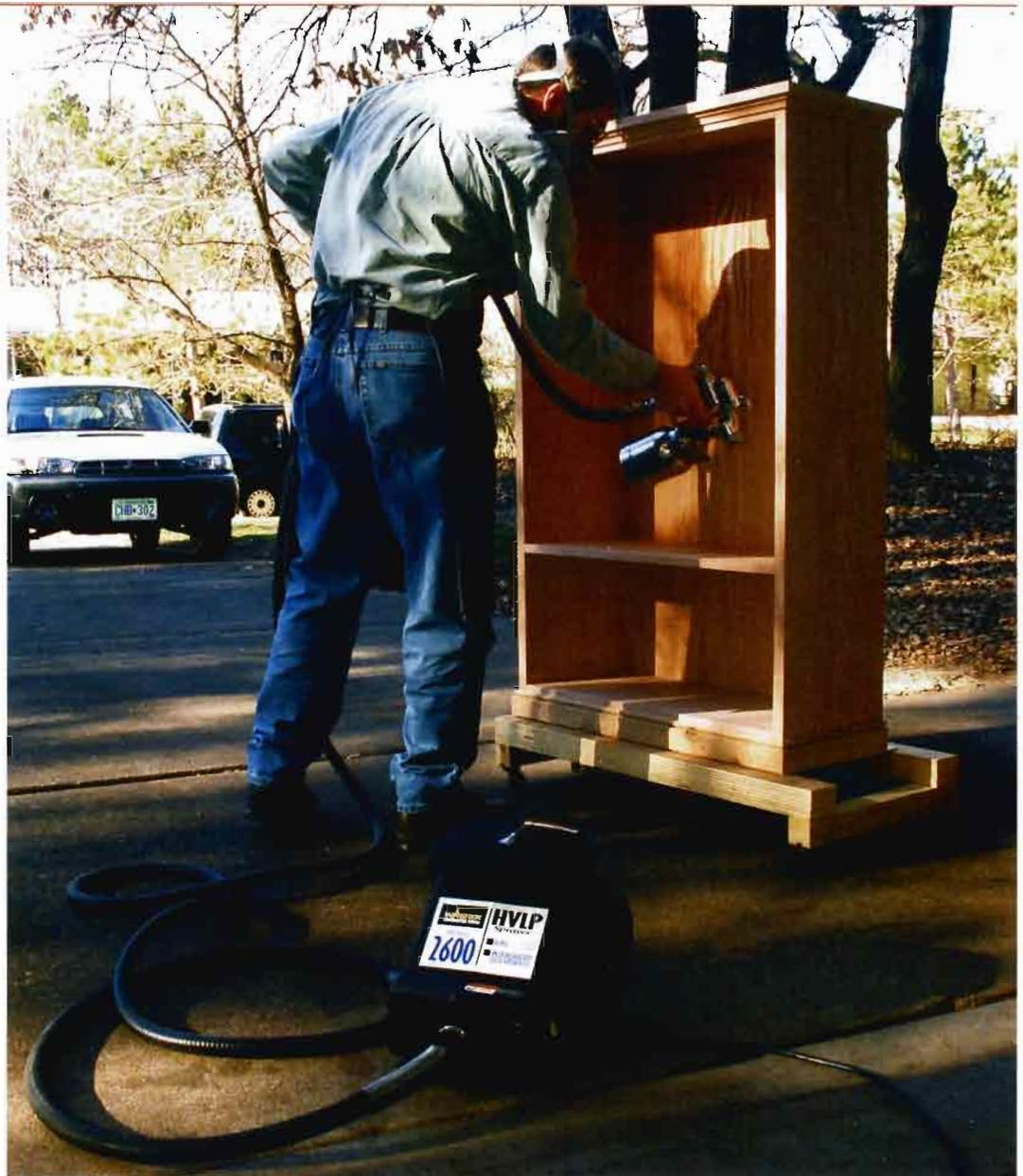
UNLIKE CONVENTIONAL HIGH-PRESSURE SPRAY GUNS that hook up to large-volume compressors and are sold separately, HVLP sprayers are sold as complete units consisting of a gun, a turbine, and an air hose.
