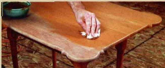
**APPLY THE STAIN.** To help achieve the result you want, the wood-coloring process starts with a coat of oil-based stain; golden oak was used for the porringer table.
