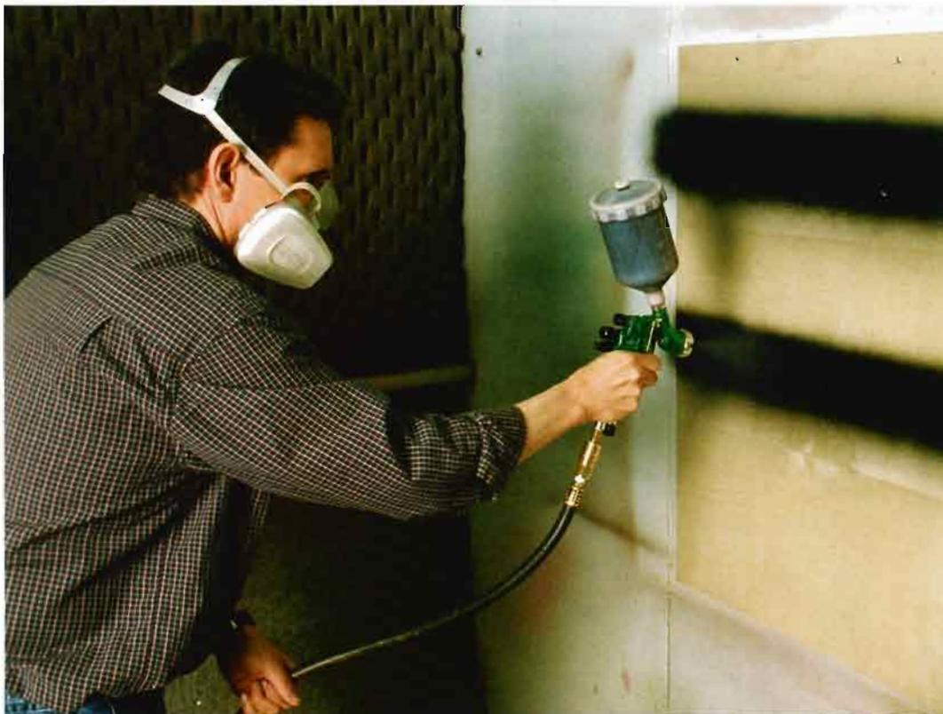
**ADJUST YOUR LACQUER FOR EVERY OCCASION.** When spraying a vertical surface, it is important that the finish dries before it has a chance to sag and run.
