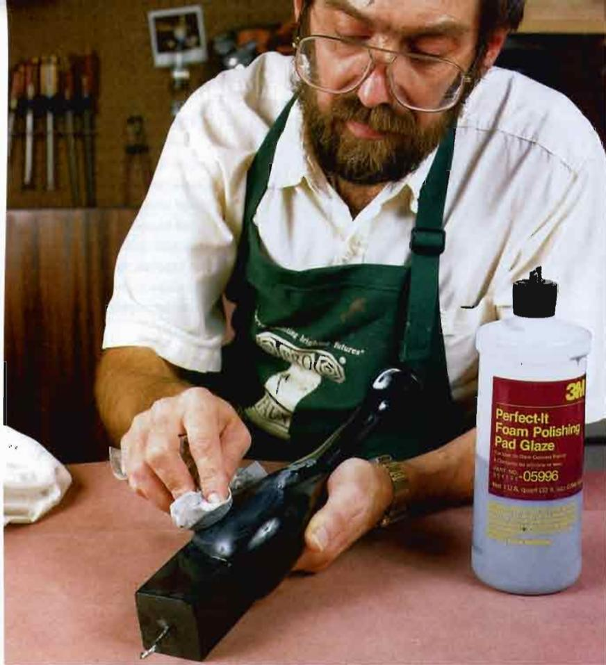
**FOR A HIGH-GLOSS FINISH,** rub out the clear coats with liquid automotive polishing compound. As a finishing touch, Minick buffs out the clear-lacquer top coat (one of five) on a coffee-table leg.
