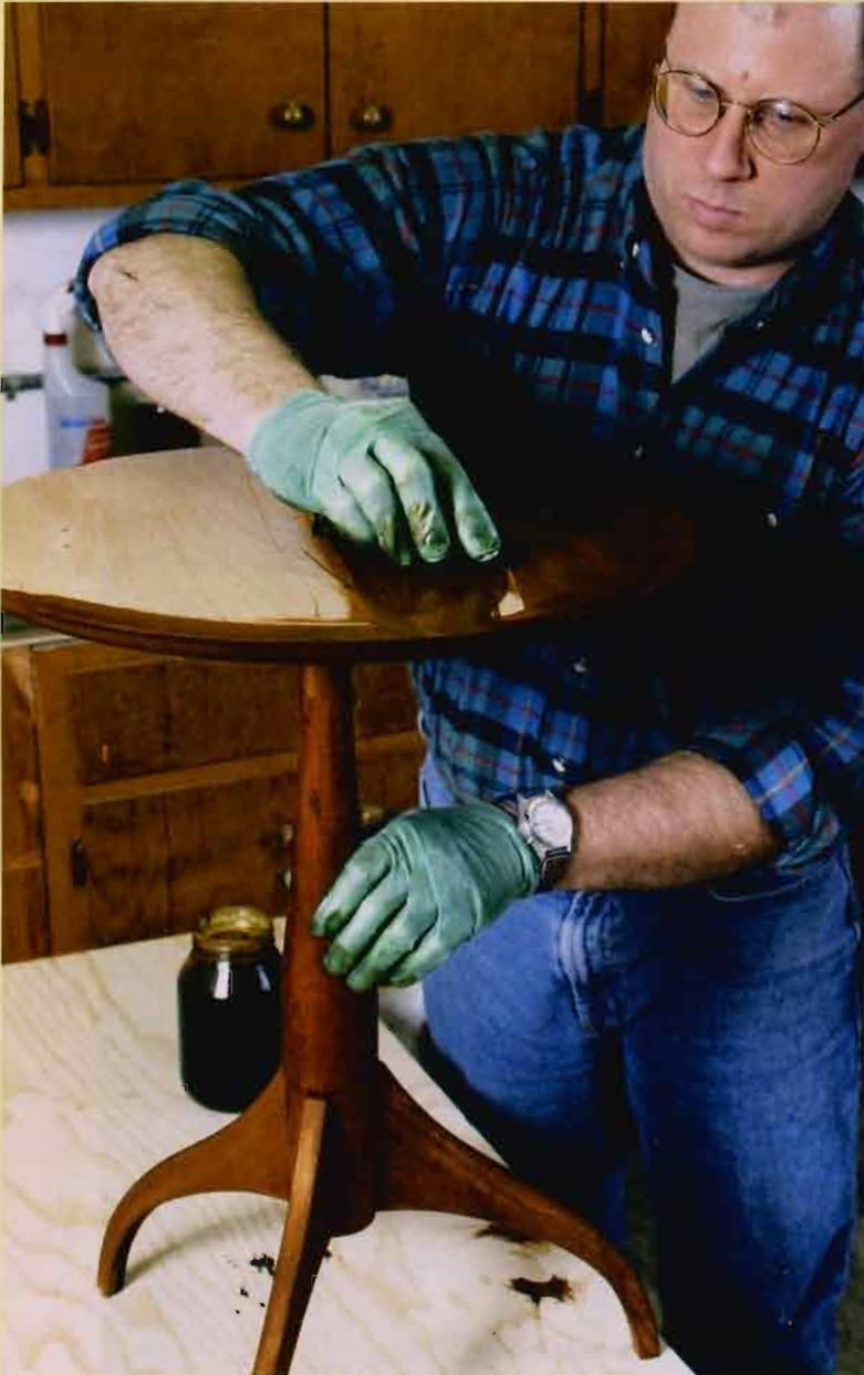
**WATERBORNE DYES ARE RUBBED ON WITH A RAG.** Flood the workpiece when applying stains and dyes. Work quickly, and wipe off any excess to avoid lap marks.
