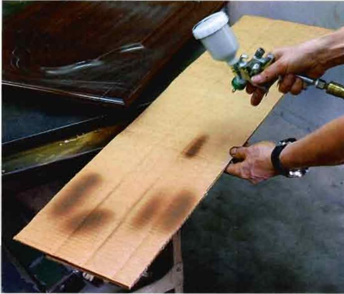
**SHADING AND TONING.** Before spraying a shading finish tinted with color, use a scrap of cardboard to set the size of your spray pattern.
