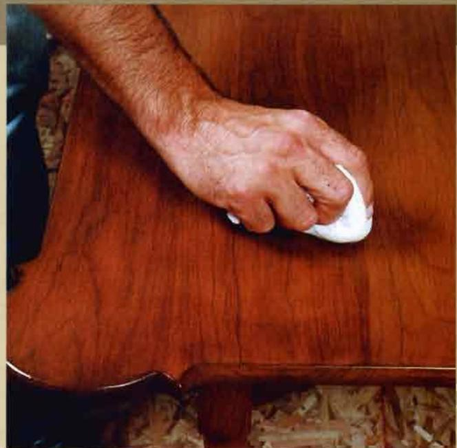
**WIPE ON A TOP COAT.** The top coat brings out all of the color and depth in the layers of glaze.
