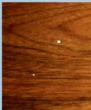
1. **Water contamination in spray equipment:** Install water separator in air line.
