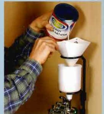
**FILTER THE FINISH.** Strain the finish through a cone filter to catch impurities that could clog the spray gun.
