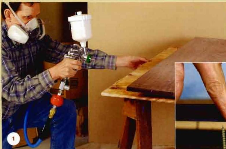
**SPRAY THE EDGES.** With the gun parallel to the panel's surface, make one pass on all four edges.
