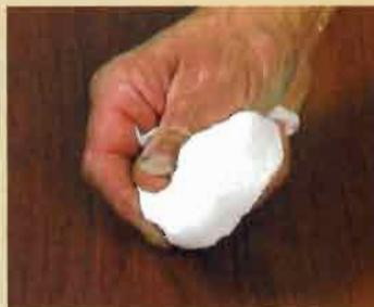
**A CLOTH PAD** helps control the application of the glaze coats. The pad is made from a couple of rectangular-shaped pieces of an old cotton T-shirt. Wrap one piece around a folded piece to create a soft pad that will fit comfortably in your hand.
