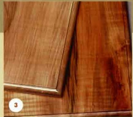
oil is available in a pure, unrefined form and in a heat-treated or polymerized form. The heat-treating process makes the oil a bit more durable and speeds up the drying time. It also minimizes a tendency of tung oil to “frost” (dry to a whitish, matte appearance). Tung oil is paler in color and has better moisture resistance than linseed oil.
