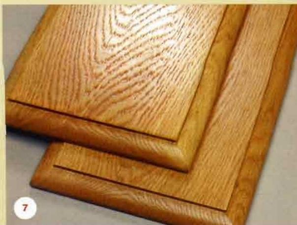
elastic and softer than medium- and short-oil varnishes that contain a lower percentage of oil. Medium-oil varnishes comprise most interior varnishes on the market. Short-oil varnishes (also known as heat-set varnishes and baking enamels) require extremely high temperatures to dry, so they're used only in industrial applications.
