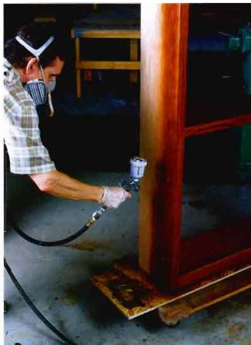
**APPLYING STAINS.** With a touch-up gun you can apply stains fast and evenly. Here, Jewitt uses the gravity-feed touch-up gun with a plastic cup to spray a water-based dye stain on an oak bookcase.
