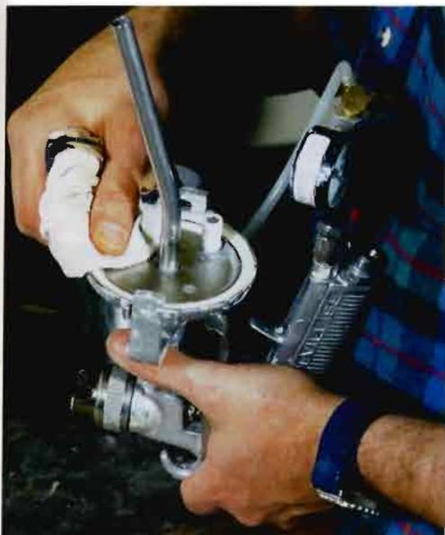
**CLEAN THE GASKET.** The gasket needs to be free of debris; otherwise, the gun will not seal properly and will leak when tipped.
