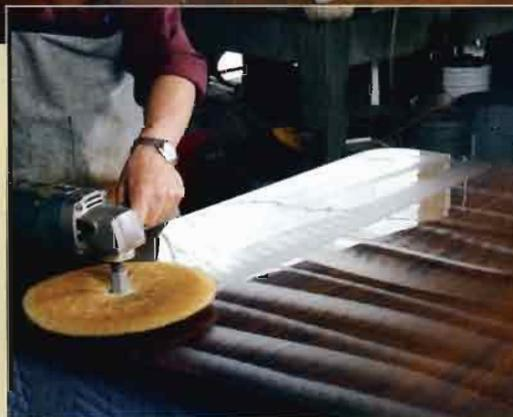
**USE COMPOUNDS IN A SEQUENCE OF GRITS.** After wet-sanding the surface, the author buffed this table first with Meguiar's #1 medium-cut cleaner, then with #2 fine-cut cleaner. After that, he finished with #9 swirl remover to fill in the tiny hairline scratches left by the #2 cleaner.
