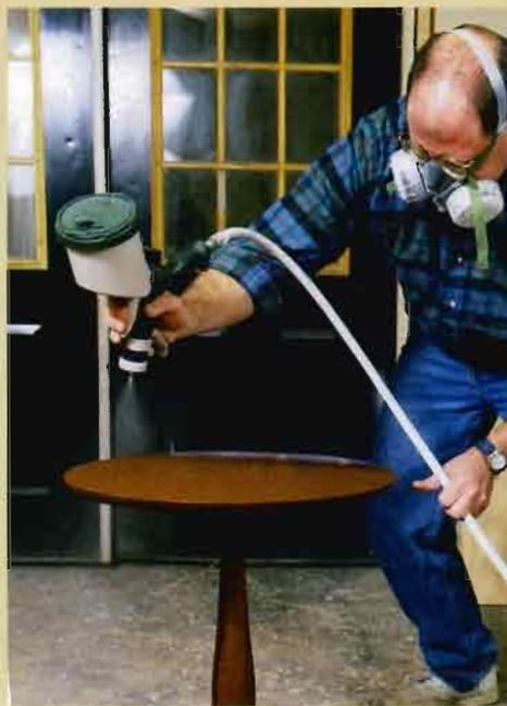
**DON'T STOP BEFORE THE EDGE.** Keep spraying until the pattern falls off the edge of the workpiece. On the next pass, overlap the previous section.
