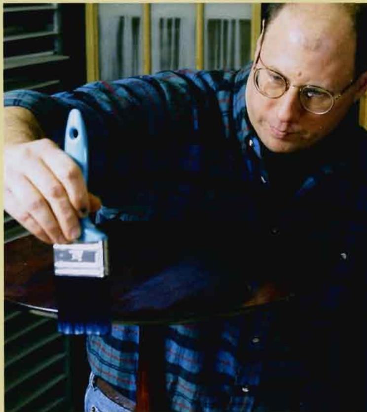
**ONCE YOU'VE STARTED,** work from a wet surface to a dry section. Brush quickly and with the grain; let the bristles skate off the workpiece surface to lessen brush marks.
