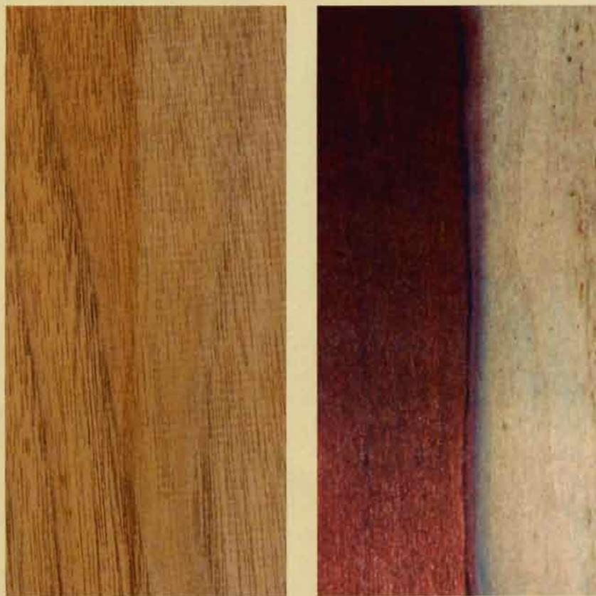
**CHLORINE BLEACHES REMOVE DYE STAINS.** The natural color of walnut (left) is virtually unchanged by an application of chlorine bleach. But most of the dye stain on the birch veneer (right) has been removed with the same solution.
