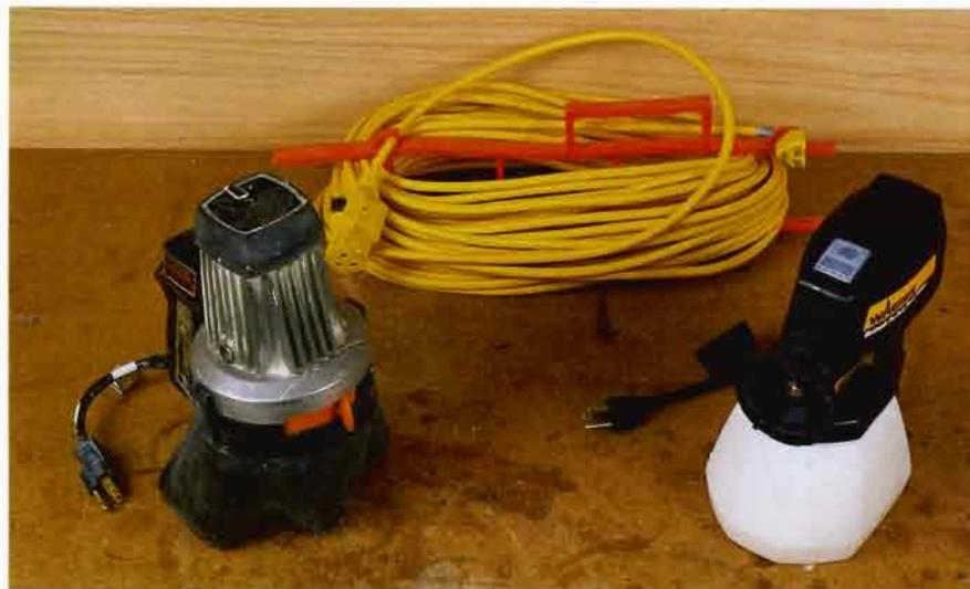
**AIRLESS SPRAY SYSTEMS WORK WELL** with latex paint and most varnishes, but they don't apply other finishes well. If not the right viscosity, the finish will be poorly atomized and leave a coarse, blotchy surface.
