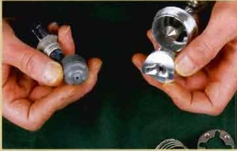
**GUNS CAN BE INTERNAL MIX (LEFT) OR EXTERNAL MIX (RIGHT). The spring, retaining ring, and baffle have been removed in the external-mix gun.**
