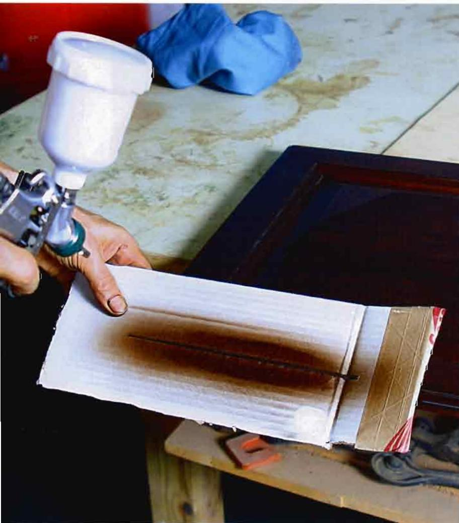
problem, and one of the most common is rubbing through the finish and the stain when the job is nearly completed. If you have a gravity-feed gun with an airbrush attachment, you can literally “draw” some color or patch the finish on a particular problem area. If you don’t have this attachment for your regular spray gun, the small spray pattern of a touch-up gun allows you to feather in finish or color so that it blends in invisibly.
