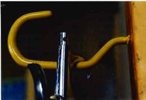
**SMALL DETAILS MAKE FINISHING EASIER.** A turntable (above) allows you to rotate a workpiece as you spray, which makes the job go faster and the results look neater. This technique is especially effective for spraying pieces that have many sides or odd shapes. A large, vinyl-coated hook to hang the spray gun (left) offers a safer, no-sparks alternative to metal-to-metal contact, and bright colors make it easy to locate.
