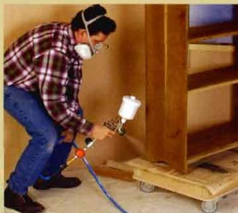
**AVOID RUNS ON VERTICAL SURFACES.** Apply overlapping strokes from bottom to top, but do not apply a cross-hatch spray across the grain, as too much finish likely will sag or run on a vertical surface.
