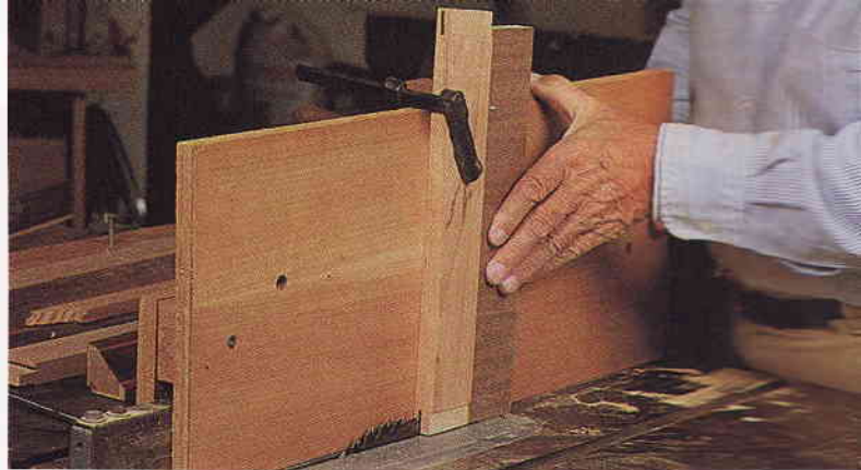
Apron tenons are cut with a plywood jig that is guided by the saw fence. The jig holds the apron so that its end runs flat against the saw table.
