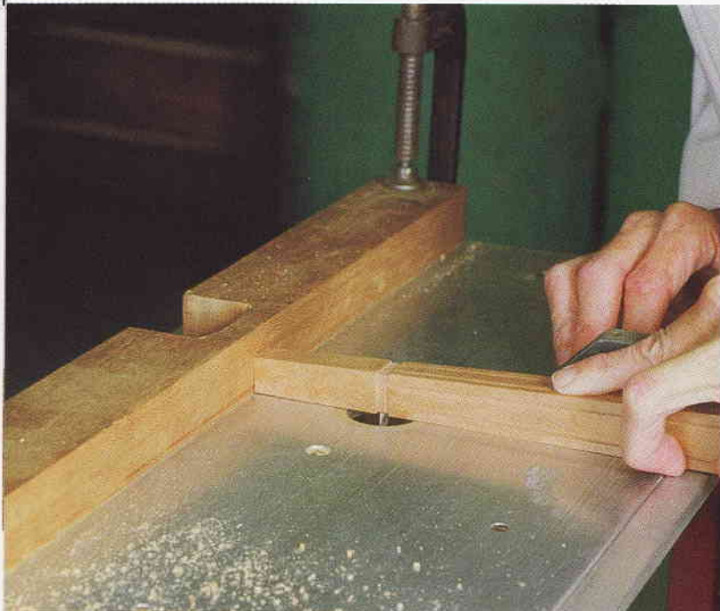
The author routes the banding groove in a leg by running the miter gauge bar along the router table's front edge. The router-table fence, which locates the cut, is clamped parallel to the table's front edge.
