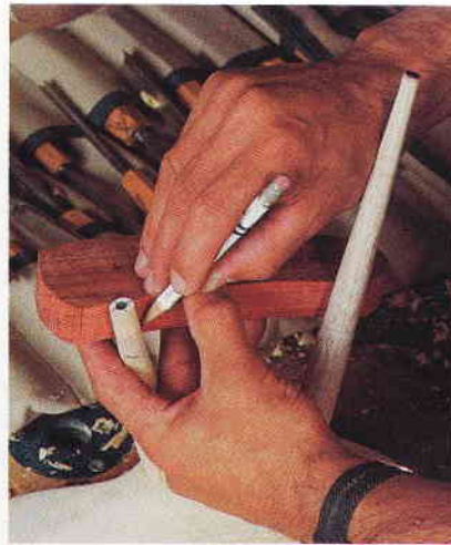
Left: Before drilling the armrest for the back posts and arm posts, the author holds it in position and marks the edge where each post will meet it. Then he sights the direction to point the drill, where each post appears plumb, and marks direction lines on the top of the armrest ( right ).
