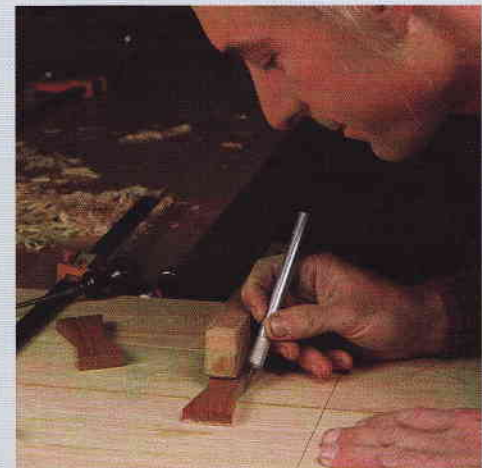
1) Scribe the outline of the key with a knife or an awl.
