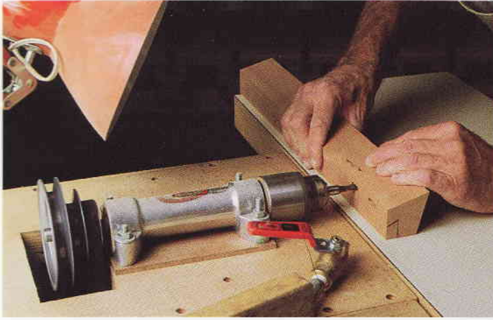
Day's shopmade horizontal mortiser chops mortises in the ends of the aprons and the sides of the legs. He prefers to work free-hand, gauging each mortise's depth by a line drawn on the table.
