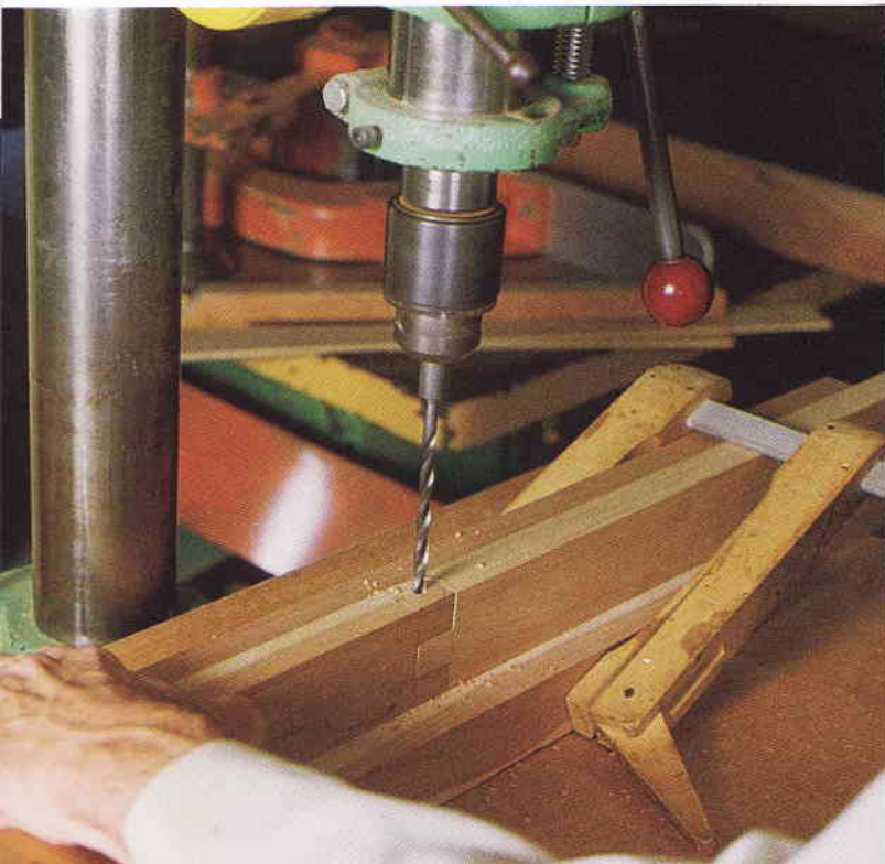
The hinge-pin hole is drilled through the two-part rear apron after an end-to-end finger joint is cut on the two parts, but before the vertical corners are rounded over to form the hinge barrel.
