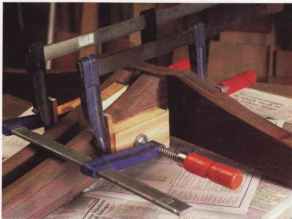
Clamping long and odd-shaped pieces—Blocks are clamped to the sides of the short feet with a properly sized spacer between each pair of feet. The blocks provide surfaces parallel to the long foot to apply clamping pressure during glue-up.
