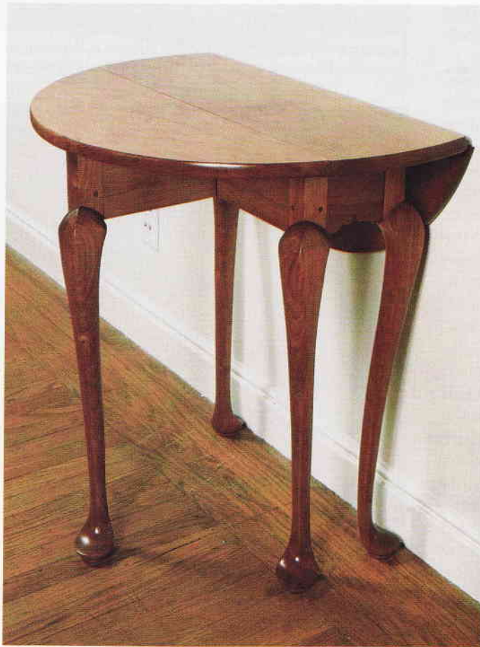
Modesty and majesty —This small Queen Anne breakfast table contains a broad range of joinery. Pinned tenons, knuckle joints and half-blind dovetails connect the aprons and legs, and rule joints run between the leaves and fixed top.
