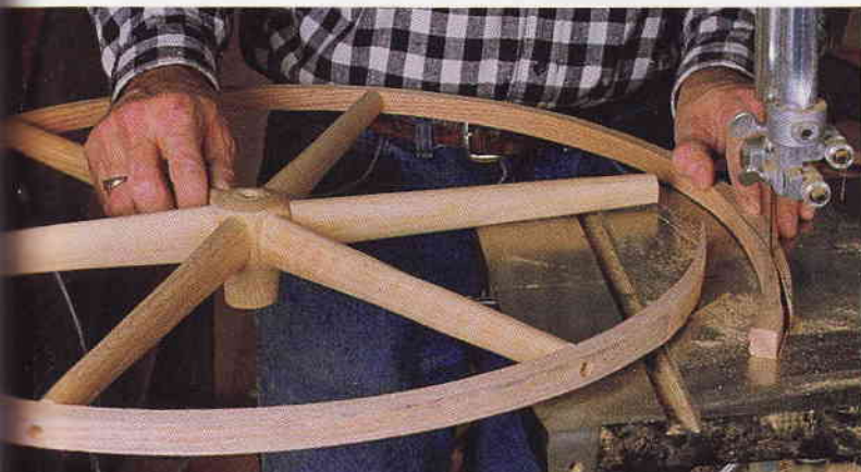
Dunbam bandsaws close to the scarf joint line: above the line on one end and below the line on the other. Then, he will smooth the scarf joint's mating surfaces with a rasp.
