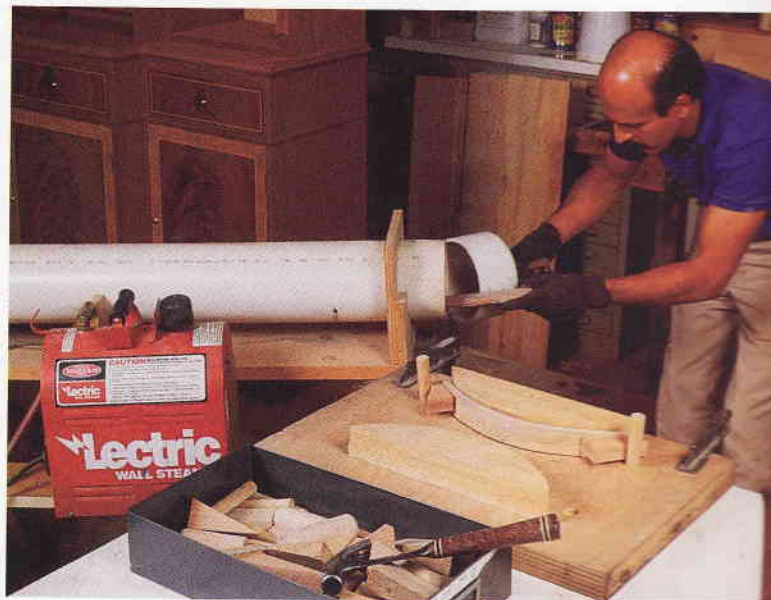
Above: Rodriguez scoops out the saddle with an inshave. Since the tool's long, angled handles prevent him from cutting steeply into the seat, he'll finish around the back edges with a wide gouge. Right: The author carves the front of the seat to a line that is marked on the middle of the edge and that curves around the sharp corner where the top rolls over. Below: Rodriguez steam bends the combs for about 45 minutes in a closed plastic pipe connected to a wallpaper steamer. Then the combs can be wedged against forms on his plywood bending fixture.
