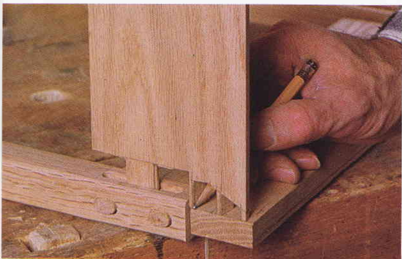
After fitting the rail tenons to the leg mortises, Dunham draws around the dovetail pins on the side rail to mark out the tails on the tray portion of the front rail. The depths of the pins must be adjusted along a 30° angle to fit tightly to the bevel that he'll plane on the inside edge of the front rail after marking and cutting the tails. The side rail is beveled before the pins are cut.
