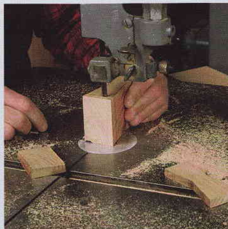
Cherry butterflies —Vogt bandsaws a stack of keys from a block of cherry.
