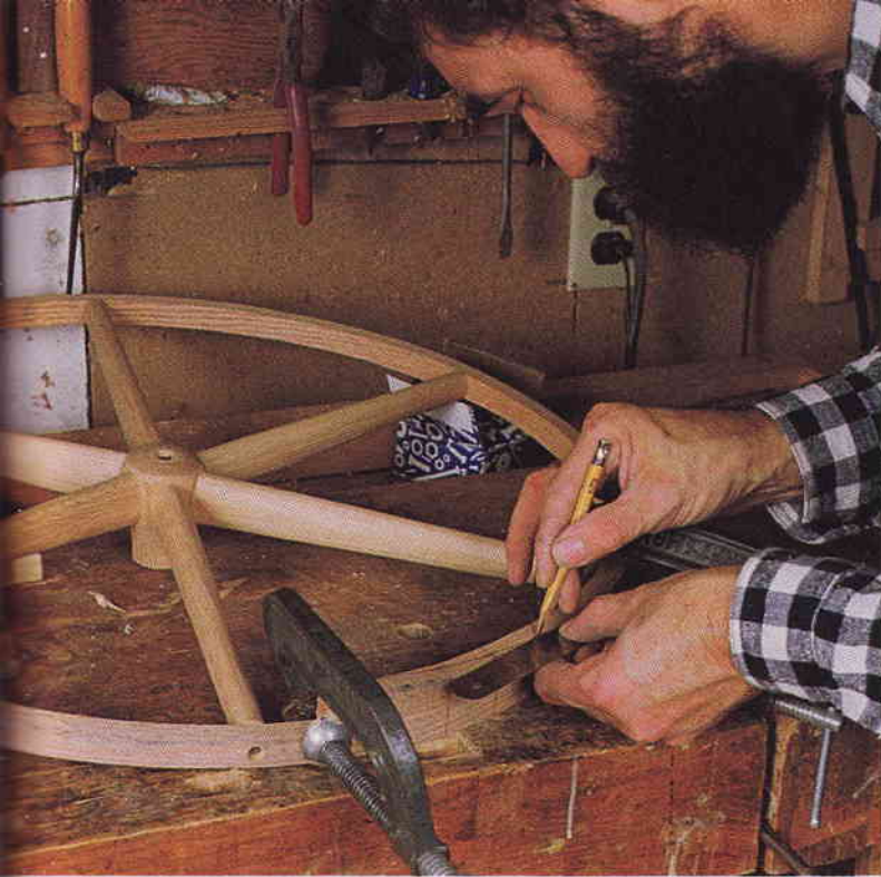
Before the rim is screwed to the last spoke, the rim's ends are clamped as shown above and lines are transferred down both sides as references for laying out the scarf joint.
