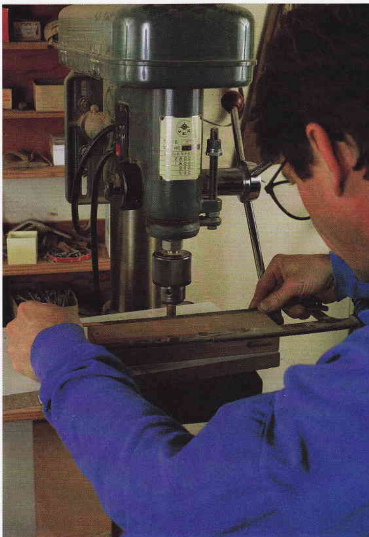
A hacksaw blade makes quick work of an overlong bushing. With his drill press set at its lowest speed, the author makes two 1/2-in. bushings from one 1-in. bushing. It's easy to tell when you're through the bushing because sawdust from the dowel starts coming off the blade.
