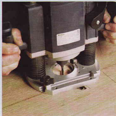
3) Plunge-rout the mortise with a \frac{1}{4} -in. straight bit.
