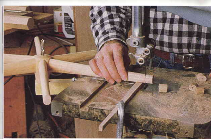
The spokes are trimmed to length after they're glued into the hub. The drill bit, which acts as the pivot point, must be aligned with the bandsaw blade and centered exactly 11 \frac{3}{8} in. from the blade for the wheel to be 24 in. in diameter when the rim is wrapped around the spokes.
