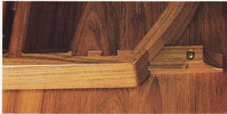
The table glide extends through the end apron, which is dovetailed to the side apron. Also shown are the dovetail joints that connect the frame's base block and the cross rail to the side apron.
