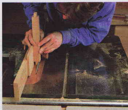
From the scrap bin, a serviceable, dependable tenoning jig. It may not look like much, but the author's tenoning jig has seen more than a few projects go out of the shop over the years. An accurate 90° back stop is all it takes; careful guiding of the workpiece does the rest.
