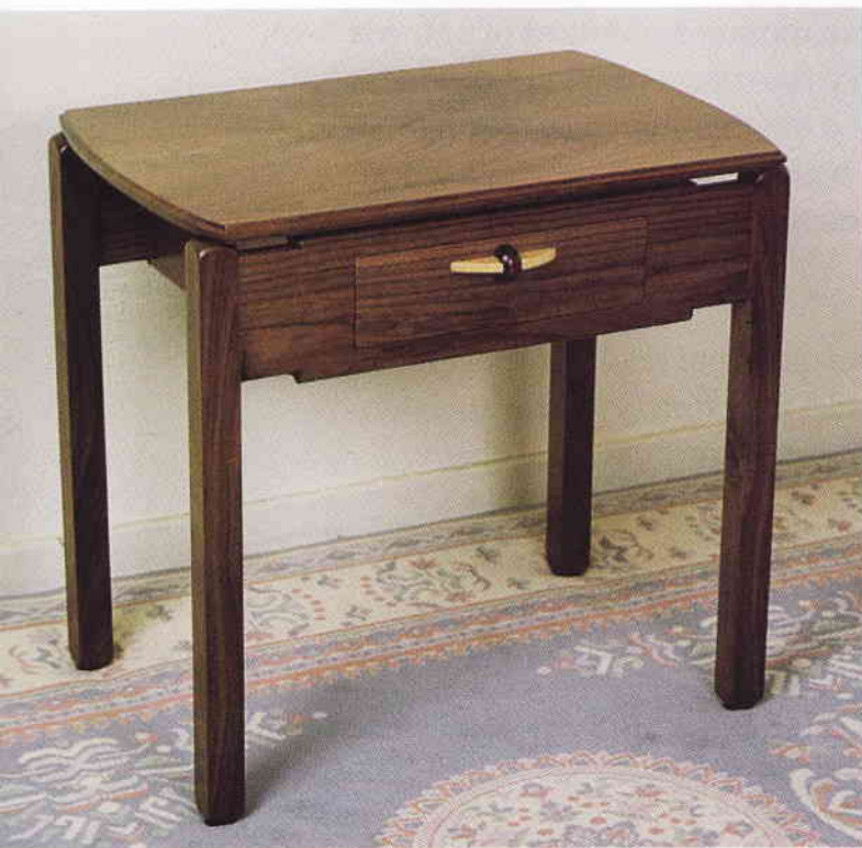
The author's occasional table was designed to fit the character of the wood: a single plank of 1 5/8" walnut that he resawned for the book-matched top, matched pairs of legs and most of the other parts. The top has room for magazines, a lamp or other accessories. The table has a single drawer with all-wood guides and a custom-made wooden pull.
