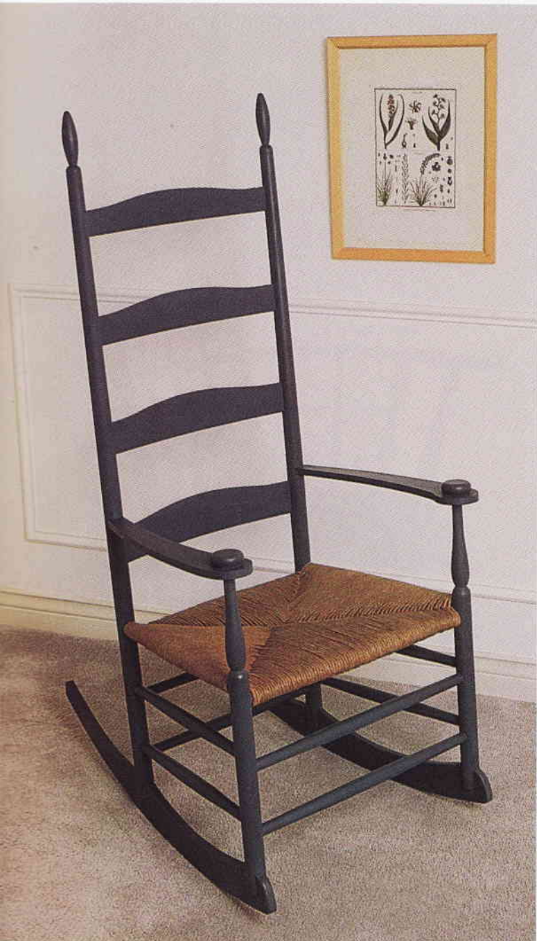
This chair, based on a photograph of a Shaker rocker, was made with commercially available dowel stock for the rungs, legs and back uprights. The author steam-bent the back slats and uprights.
