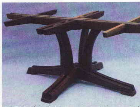
Doubling the frame members reduces the mass in the feet, legs and tabletop supports. It also simplifies the joinery and adds visual interest.
