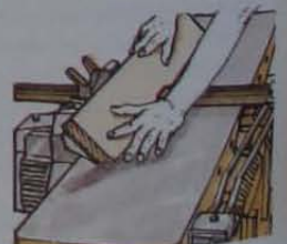
Planing a bevel Support the work with your left hand
