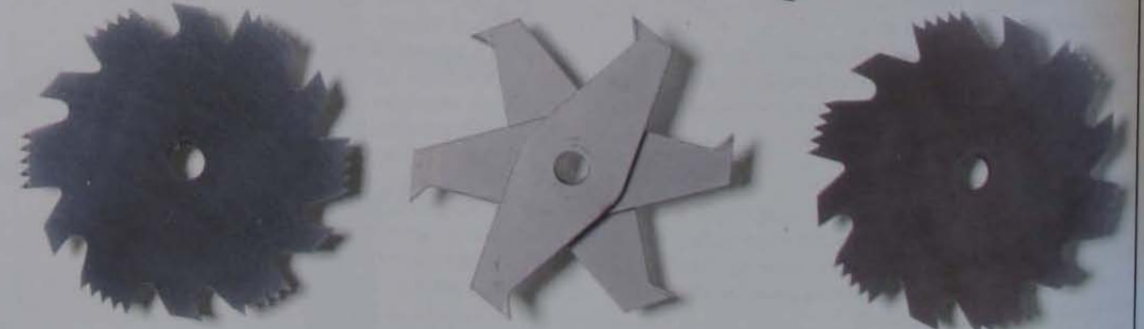
Chipper blades are sandwiched between dado saw blades
