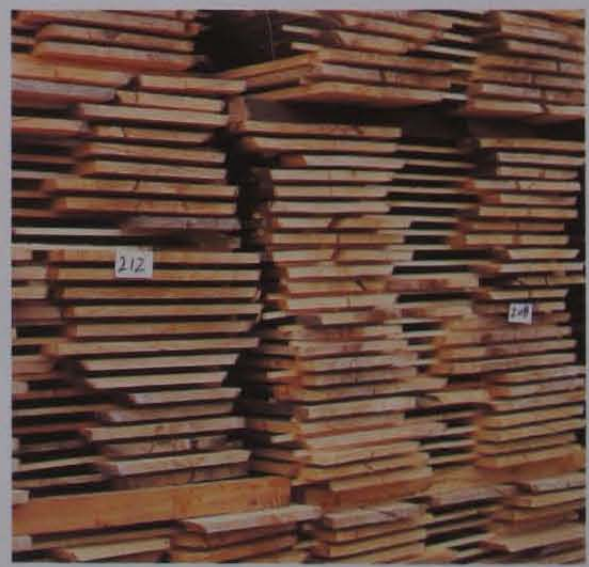
Sawn boards are dried by natural airflow through the stack.
