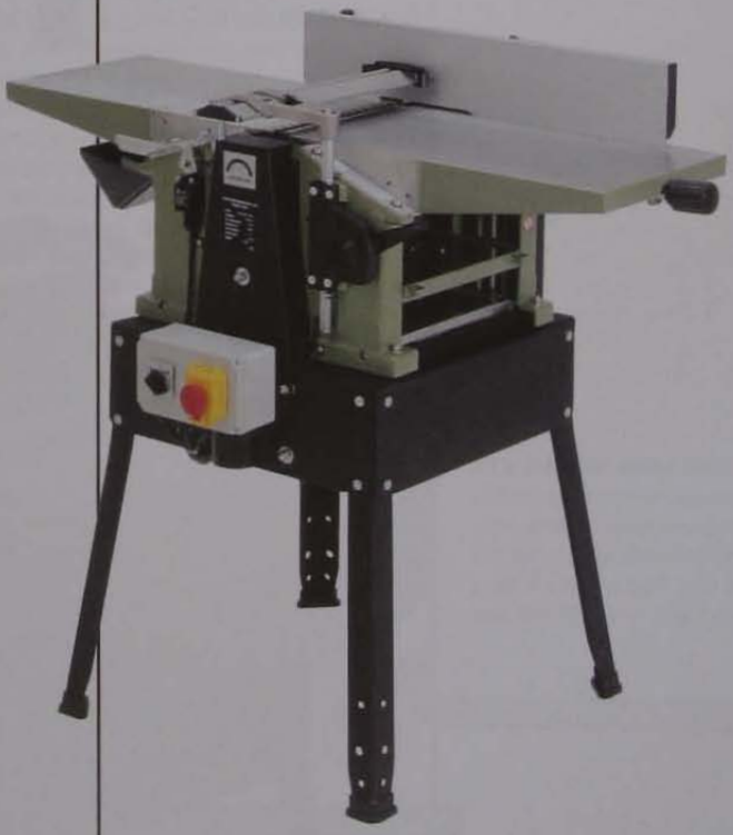
Planers should have accessible on/off switches
