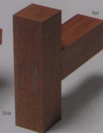
Twin mortise-and-tenon joint heavy construction
