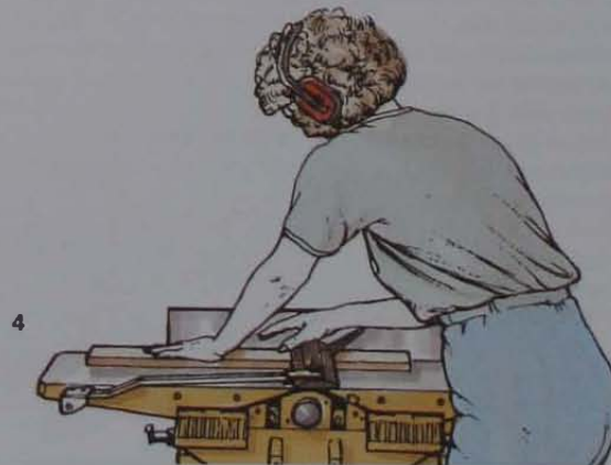
Tilt the fence to plane a bevel
