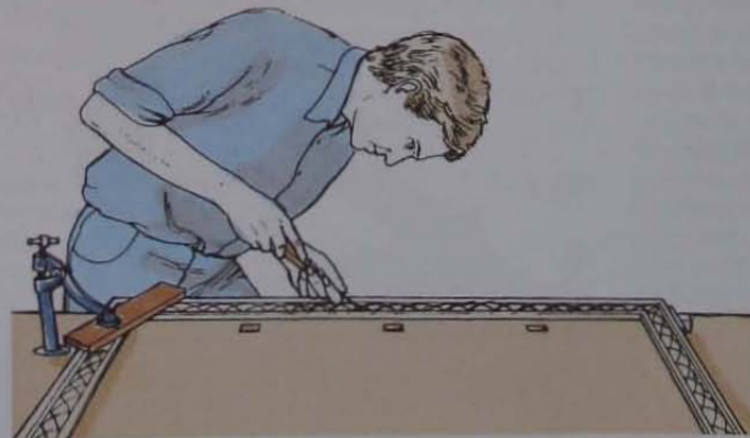
A traditional woodworking bench provides ideal support for flat workpieces
