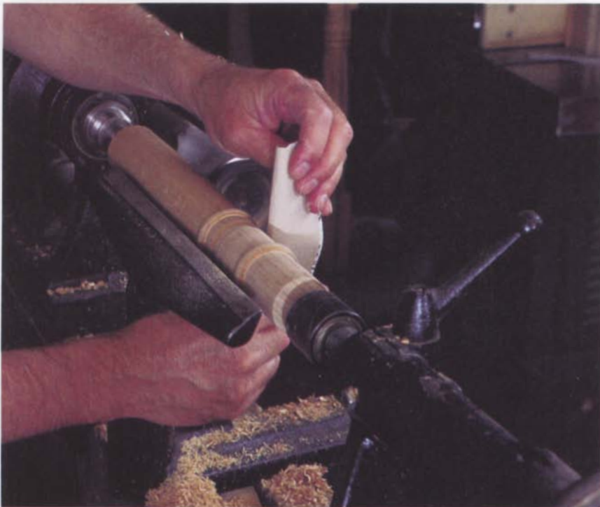
Beginners should slide the rest back out of the way during sanding (top), but experienced turners can sand opposite the rest so they don't have to remove it (bottom).
