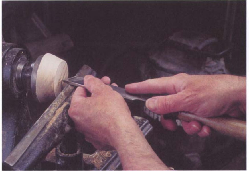
Lightly touching the point of a skew to the center of the glue block before drilling will ensure that the drill starts perfectly on-center.
