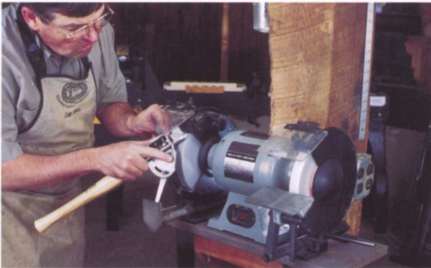
The basic Wolverine jig from Oneway gives you a base unit to mount under each wheel, a tilting table that is good for scrapers, plane irons, and standard woodworking chisels, and an arm (pocket jig) for sharpening roughing gouges and for use with the Vari-Grind jig.
