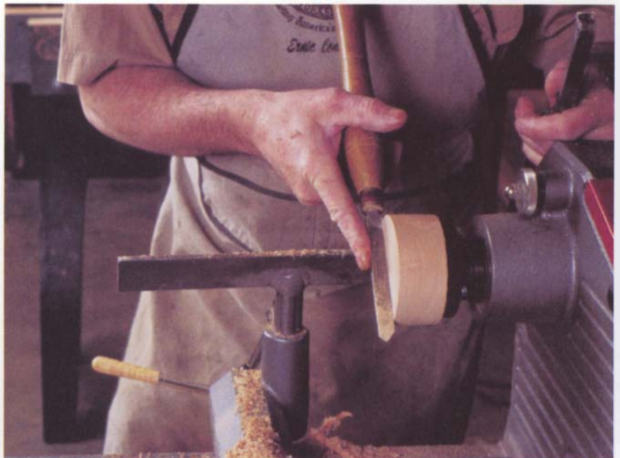
When the face is dead flat with a straight edge, it is square to the headstock spindle.
