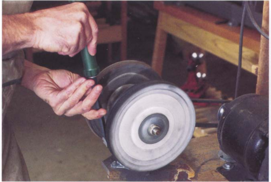
Proper buffing technique when honing a spindle gouge requires you to buff off the edge and to hold the tool tangentially to the wheel.
