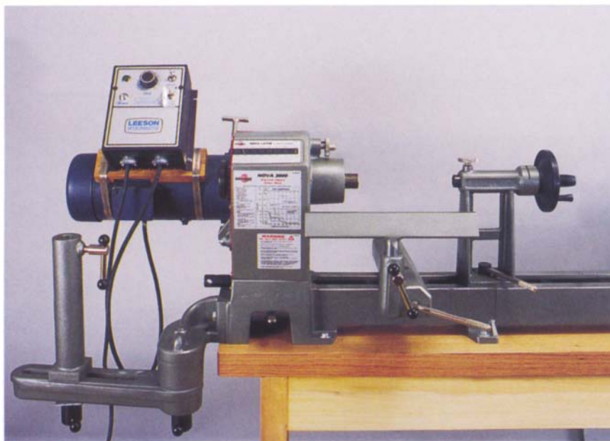
A DC motor is a nice way to add variable speed to an existing lathe. Many manufacturers now offer DC (or variable-cycle-rate AC) as the method of variable speed.
