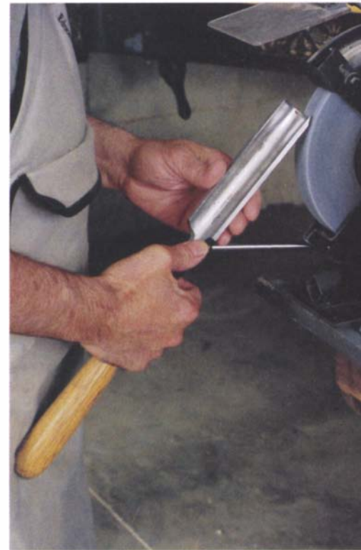
If you are already comfortable with freehand grinding, you don't need a jig or a rest. Simply plant your feet well in front of the grinder, and rest the tool handle on your thigh.
