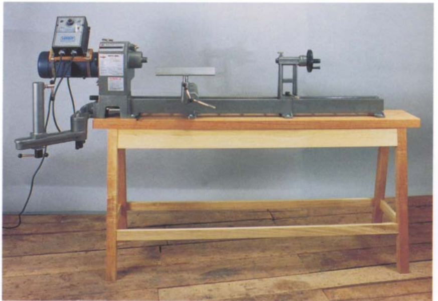
The Nova 3000 is a well-designed, mid-range lathe. It offers all the features of the Delta 46-700 with greater swing, DC power options, and a modular bed design that allows the bed to extend. Nova also builds an ornamental attachment for this lathe.
