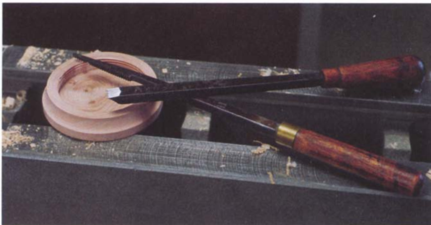
Shown here is a set of antique thread chasers, but you may purchase new chasers from Craft Supplies.
