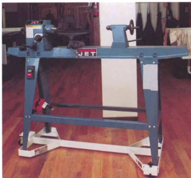
Based on the Delta 46-700, this Jet lathe is a good small lathe that offers good swing and between-center distances with a swing head for occasional larger faceplate work.
