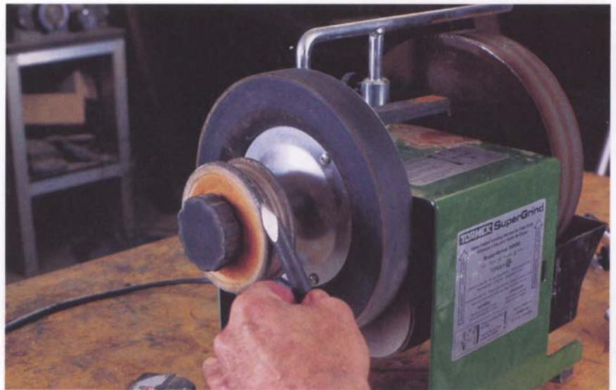
For the inside of gouges, the optional profile honing stop on a Tormek machine mounts outboard on the normal strop supplied with the machine.
