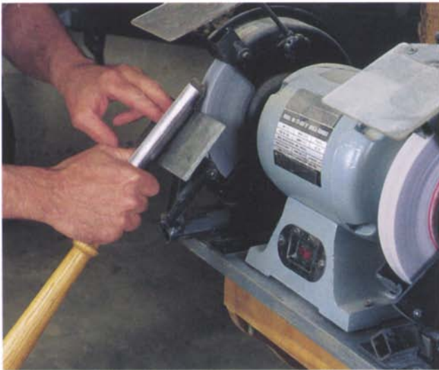
A roughing-out gouge may be sharpened on a platform rest (left) or in a pocket jig (right). The platform rest is better because tool-handle length precludes a long bevel on most home-shop-sized grinders.
