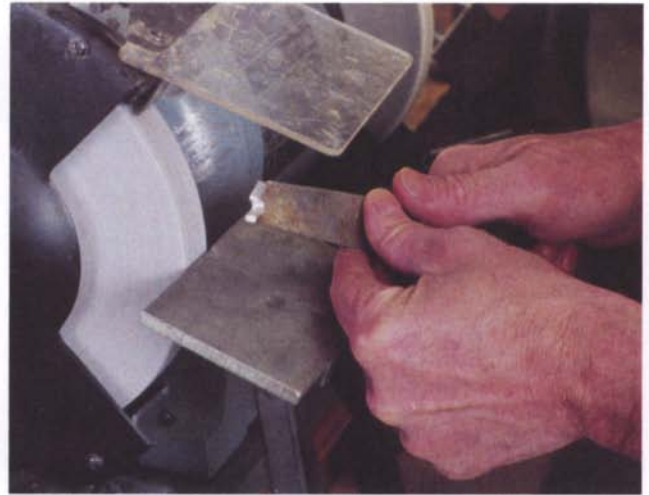
When the scraper is ground, it should look like this. Note the undercut is also about 5° to the sides in the area of the bead.
