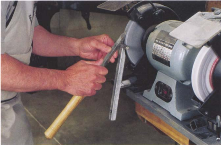
A cutoff tool is easy to grind by eye. Simply touch both bevels to the grinder to achieve a 42° or less point, inclusive. Keep the point centered on the blank, especially on diamond tools.
