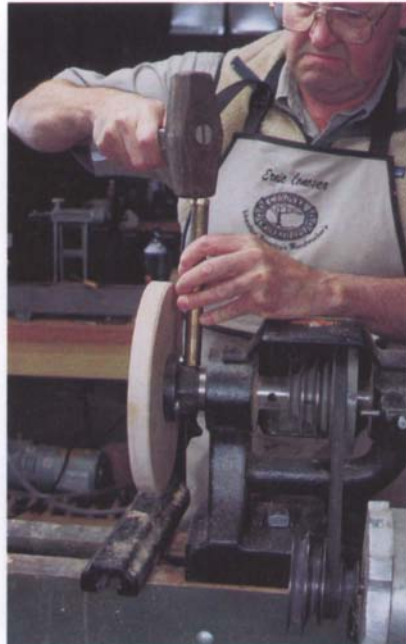
Delivering a solid blow to the edge of a faceplate with a hammer and brass drift often frees a frozen faceplate.
