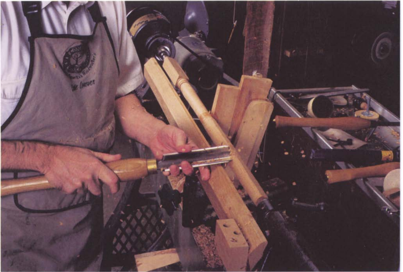
A full-length wood rest works just fine for turning long stair balusters.
