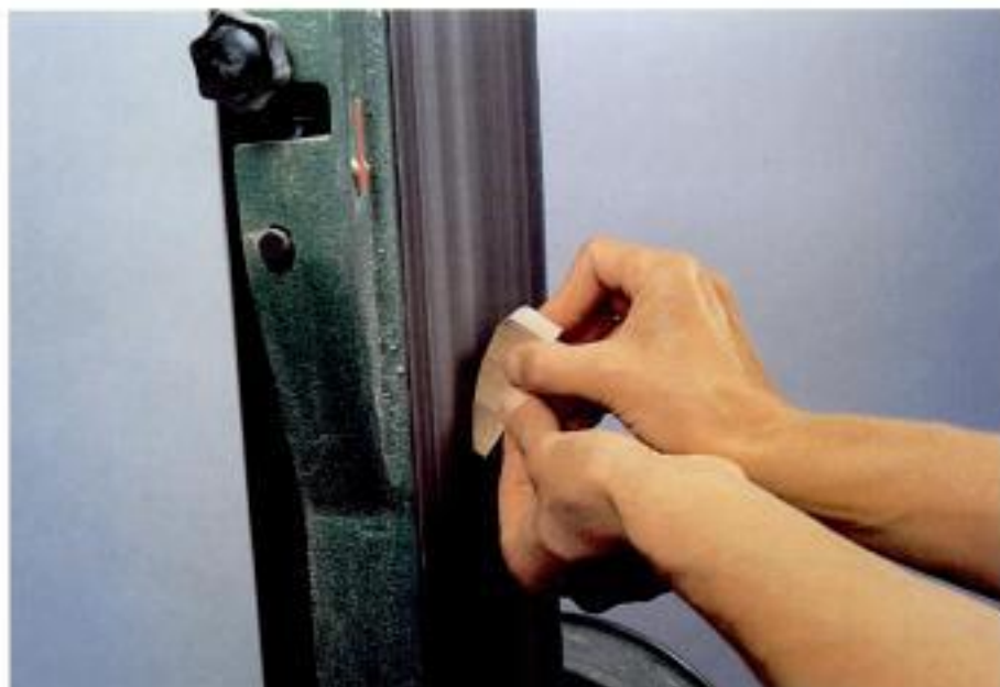
Photo 4-10 You can add depth to the drawer pulls by rounding them with a curved taper.
