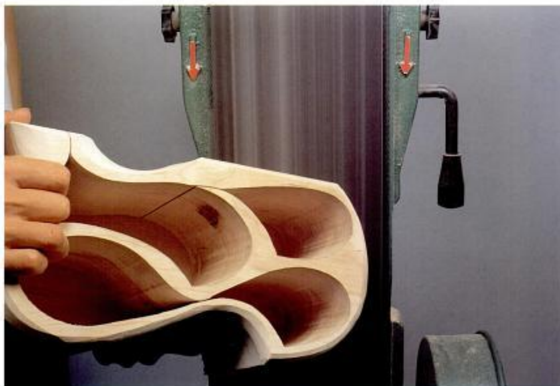
Photo 4-5 Shape the edges by working the box at an angle and upwards against the belt. By working the piece side to side and front to back, you can quickly rough your box into a more rounded shape.
