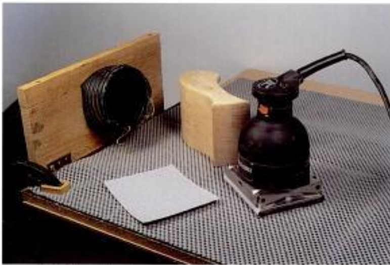
Photo 4-17 To collect dust as you palm sand, you can make a stock-style hose-holder with scrap wood, corner braces and screws. Or you can simply clamp the hose to the edge of your workbench.
