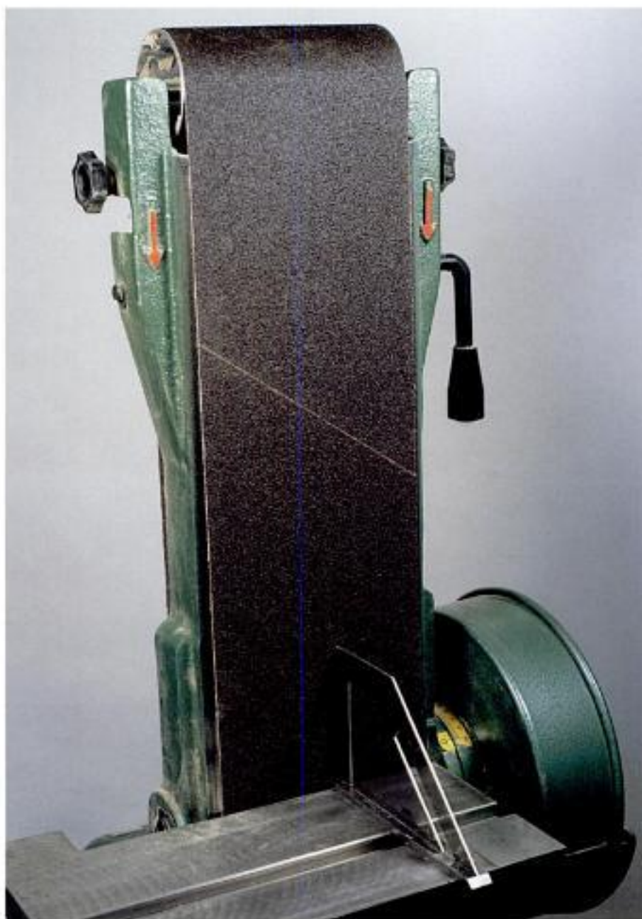
Photo 1-2 You will use your belt sander in its vertical position, with the table at 90° and as close to the belt as possible.
