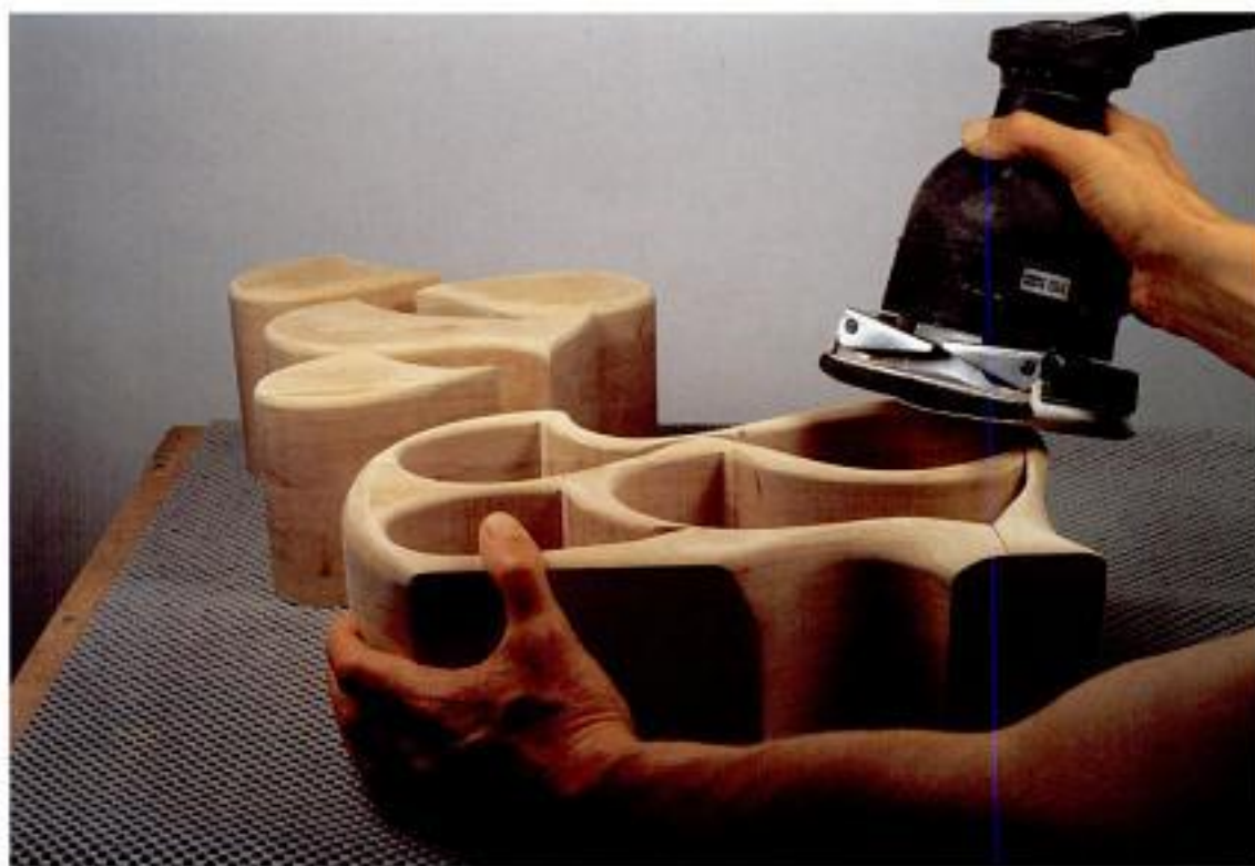
Photo 1-5 Tried and true, the Porter-Cable 330 can't be beat for this type of palm sanding.
