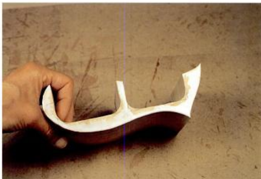
Photo 3-16 As with clamping the back on, use discretion when spreading glue to the inside edges of the drawer parts in order to avoid chipping it off later. However, it's always good to see a little glue coming out of the outer sides to know the bond is good.
