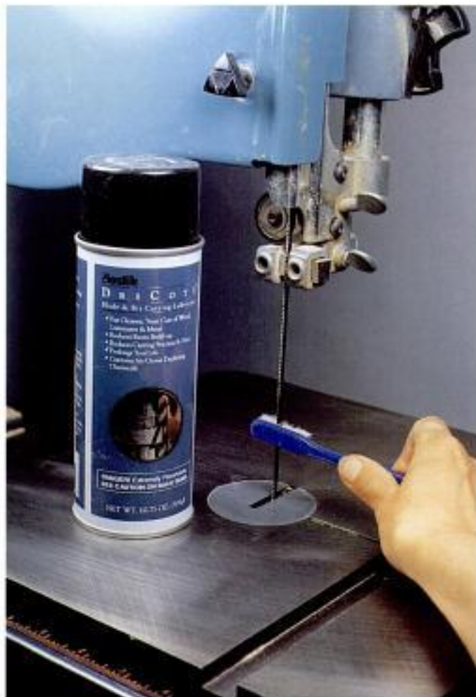
Photo 3-4 A clean, lubricated blade offers less resistance when making thick cuts. This reduces the chance of the blade bowing while you cut.
