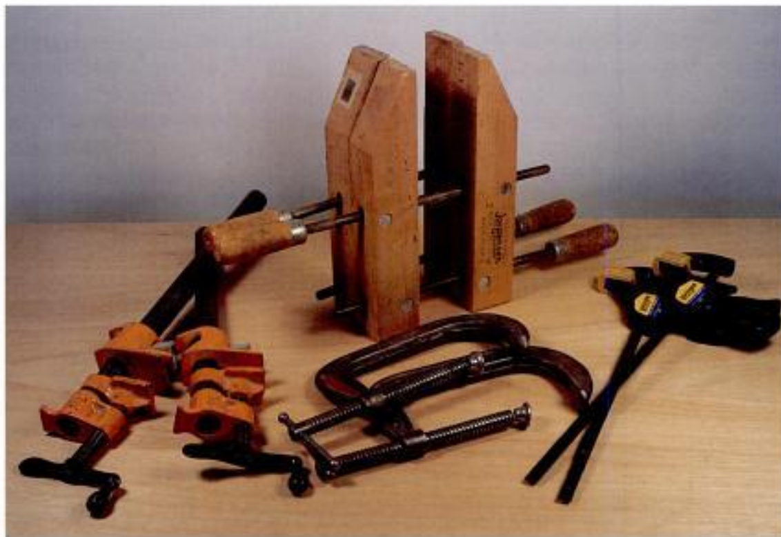
Photo 1-4 Hand screws are your foundation clamps for these projects, but having a variety of clamps available is ideal.
