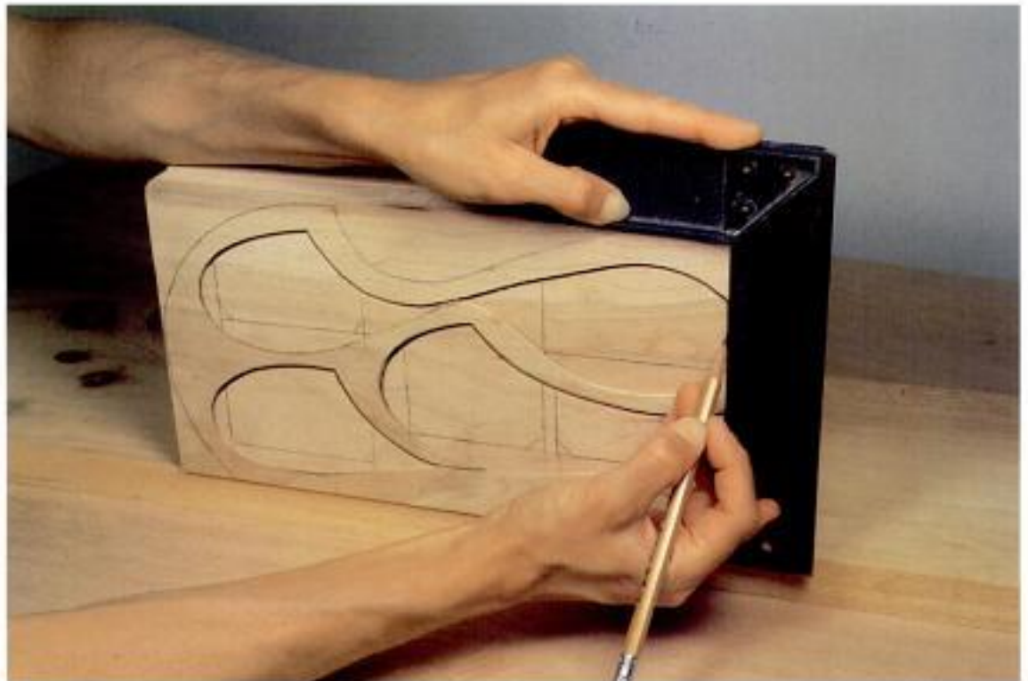
Photo 3-10 The easiest way to mark straight sides and bottoms for the drawer hollows is to square them in relation to the outer block.
