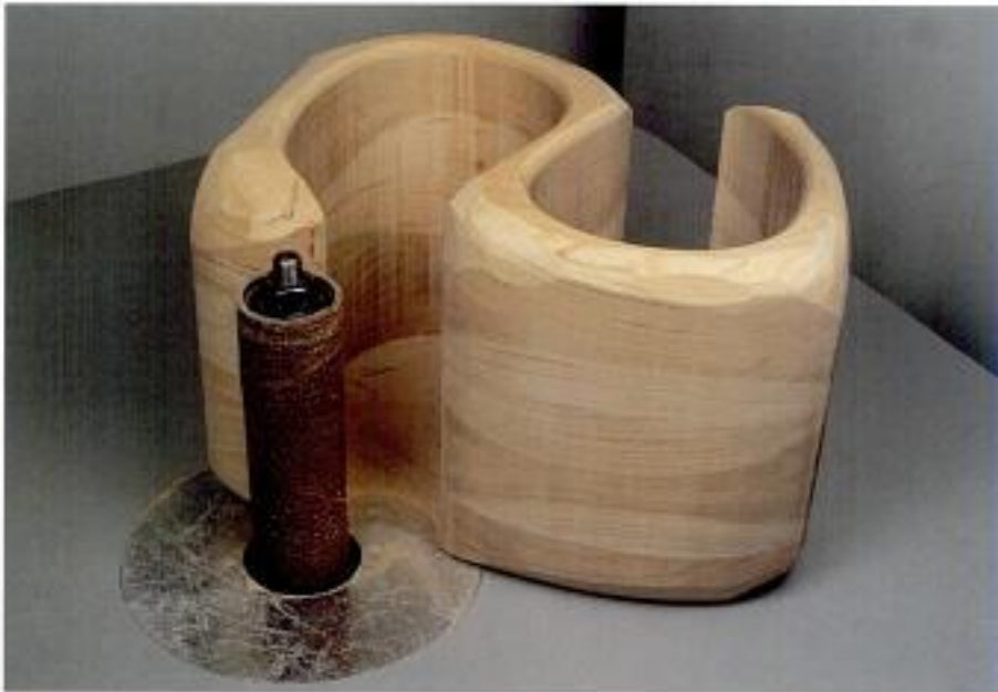
Photo 4-16 Sand the rough back at the open drawer ends smooth using either your oscillator, drill press or portable drill.
