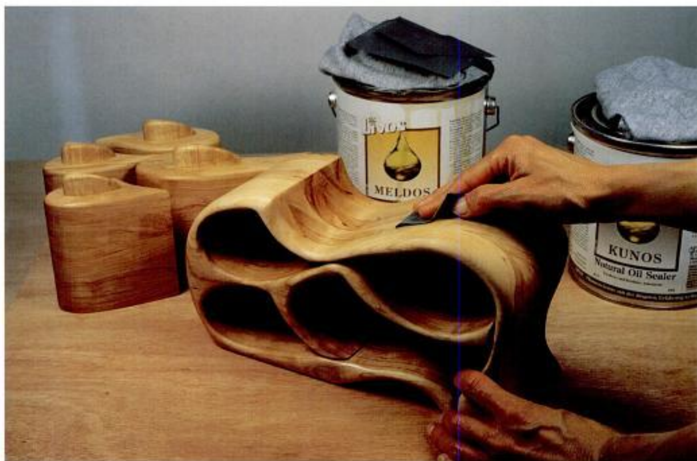
Photo 5-2 A firm, wet sanding sets your box up for a fuzz-free finish. It's very important to wipe off the box after a few minutes, even if it looks dry. The same applies to succeeding coats.
