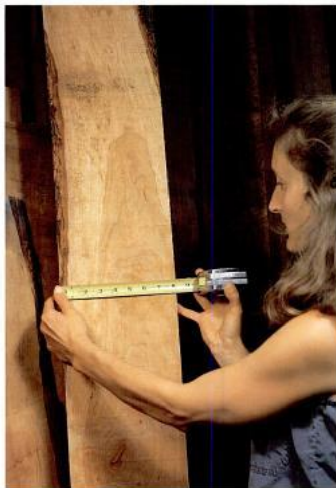
Photo 2-2 Keep your project dimensions in mind in order to minimize waste when selecting stock. Also remember that a board with sapwood can become a stunning band saw box.
