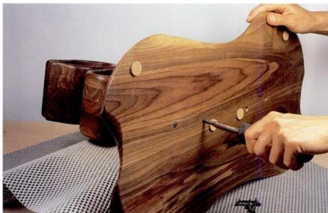
Padded support protects and steadies the boxes while you mount the base. Remember to remove all drawers before you proceed.
