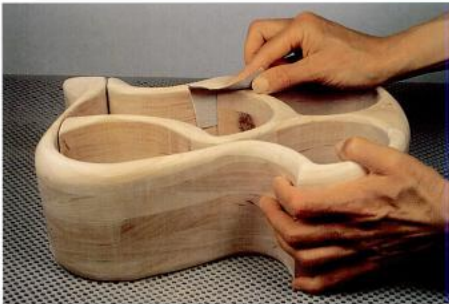
Photo 4-20 Beginning with coarse paper, soften the chiseled kerfs.
