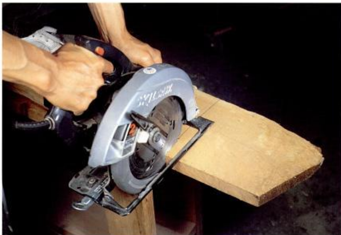
Photo 2-3 Rough-cut off any extra length prior to surfacing. This makes long stock easier to handle while planing and jointing.
