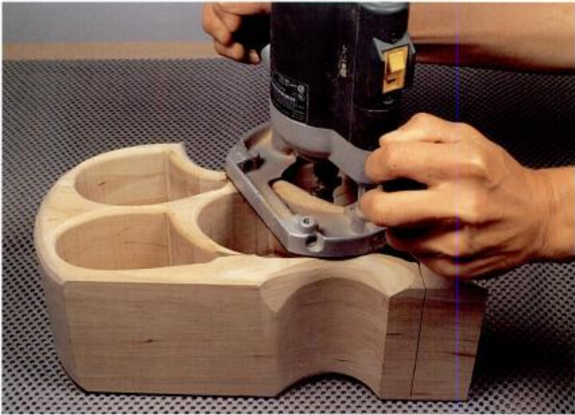
Photo 4-12 Round over the drawer opening with a \frac{1}{8} " roundover bit.
