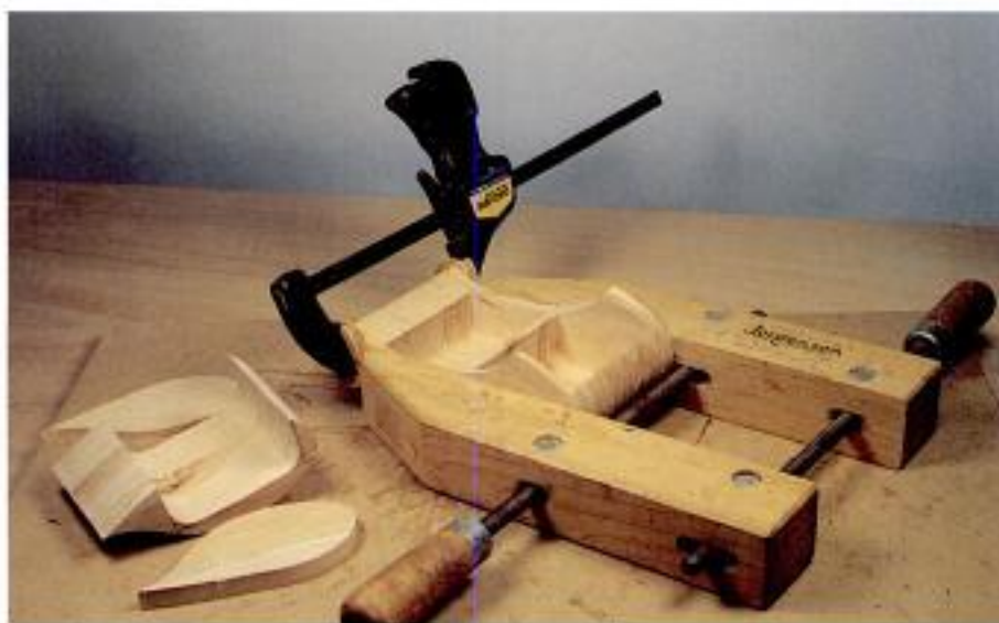
Photo 3-17 A hand screw and a flat surface simplify the task of clamping drawers. In most cases, you'll have to work with the pieces to keep them even while you clamp.
