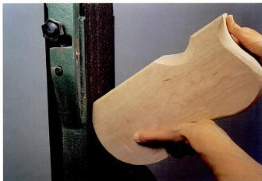
Photo 4-11 Hold the box or drawers tightly as you sand out the cross-grained lines. Use an upward motion against the face of the 120-grit belt. Repeat this process using the 180-grit belt to lessen your palm sanding later.
