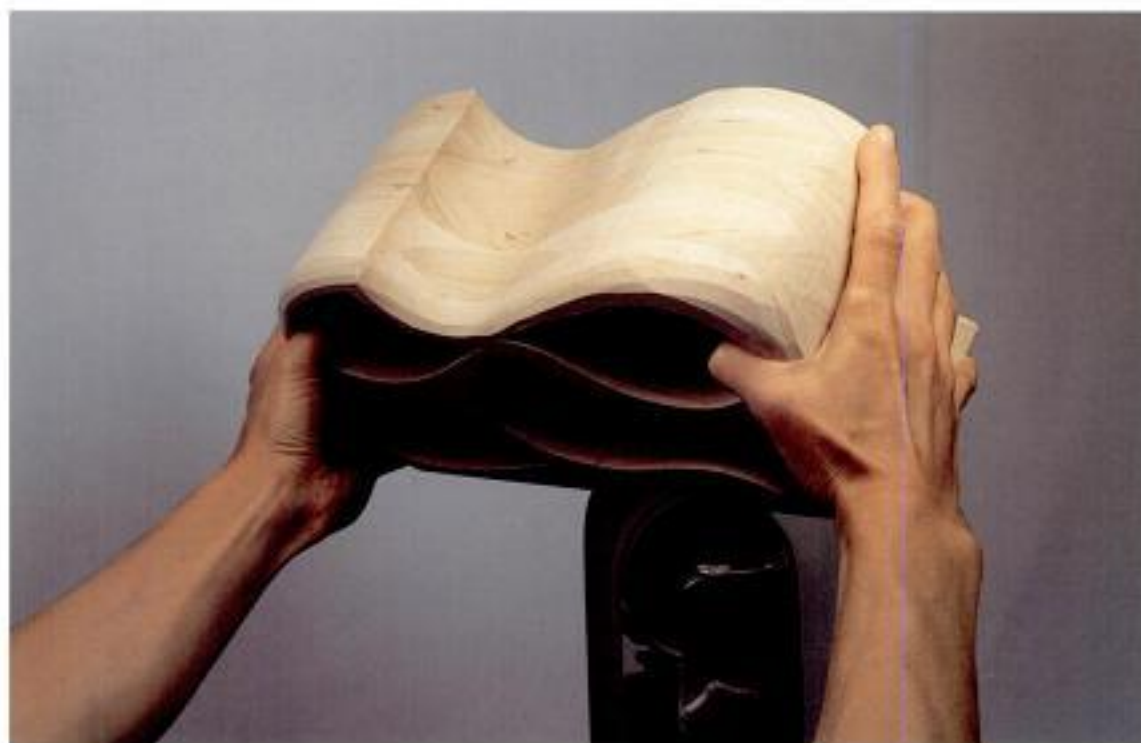
Photo 4-6 Try rolling and twisting the concaves over the cylinder to exaggerate the curves.
