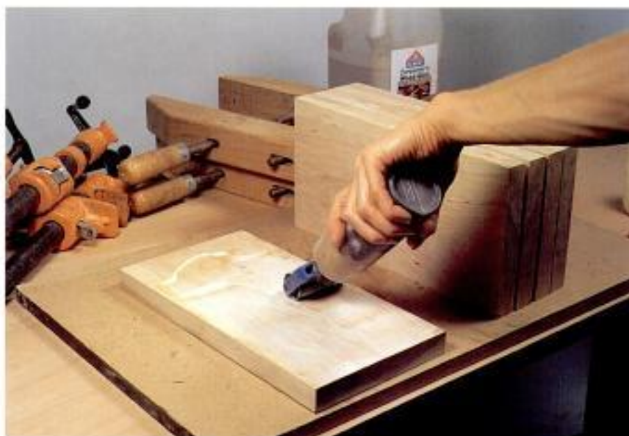
Photo 2-11 A roller helps you spread glue thoroughly and evenly over the pieces to be laminated.
