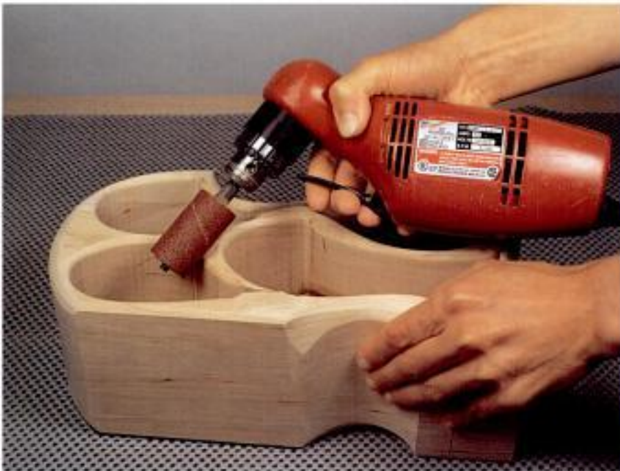
Photo 4-13 As an option, or if you don't have a router, you can roughly round over the openings with a coarse sanding drum in your portable drill. 80-grit on the palm sander will quickly smooth it out.
