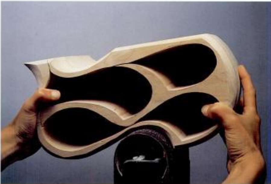
Photo 4-3 Create smooth, concave surfaces by working the box against the pull of the belt, front to back over the top cylinder.
