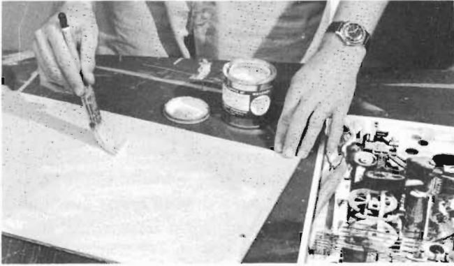
3 Gluing. We quickly brush glue on one side of the board, covering the entire surface.
