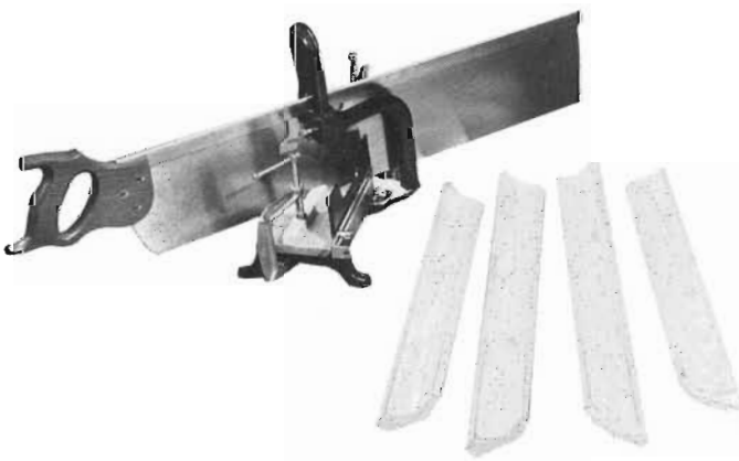
8 Cutting completed. The four sides of our frame are cut and we are now ready to tackle the tricky job of joining.
