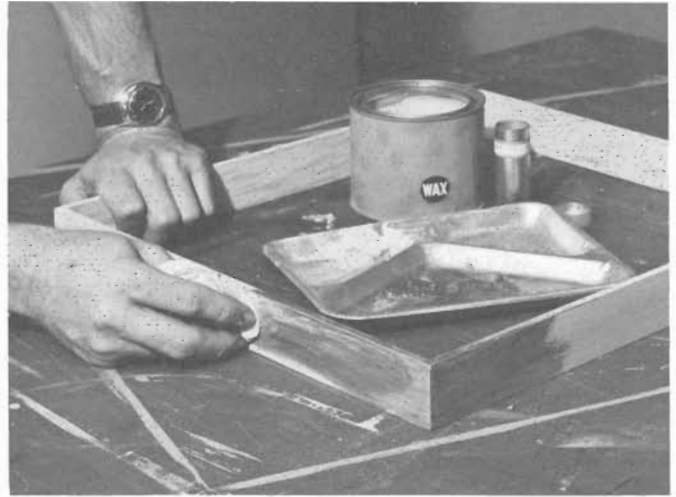
3 Applying gilt. Simply rubbing the wax gilt mixture over the thoroughly dry frame completes this gilt.
