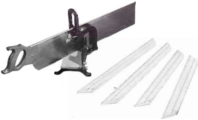
7 Cutting completed. The four sides are now ready for joining.
