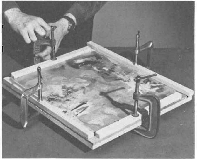
10 Clamping. While the second coat of glue is still wet we position the strip, and clamp the two surfaces firmly with the C clamps. Be sure to use scrap pieces of parting strip to protect the painting and to spread the clamp pressure evenly along the edge of the panel.
