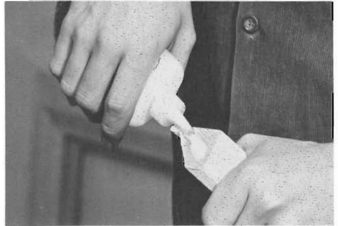
8 Gluing. Next we apply a liberal coating of glue to the miters of one long and one short side.
