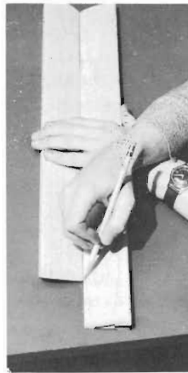
4 Measuring. After repeating the first step, the first long side serves as a pattern to mark the second.
