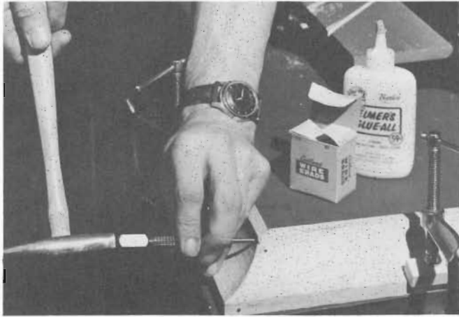
10 Setting. Using the nail set we sink the brad heads below the surface of the wood. This completes one half.
