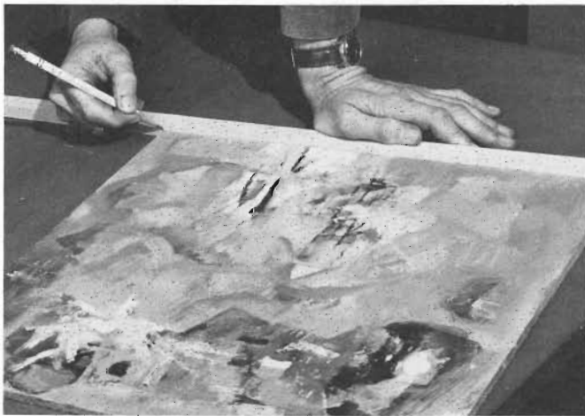
1 Measuring. Using the panel as a pattern we measure the first long side of the parting strip.
