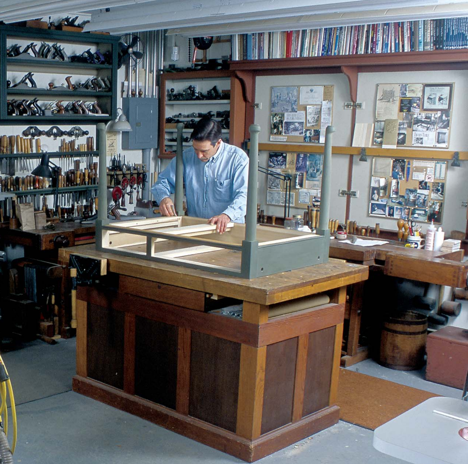
Craig Bentzley's shop is a model of compact efficiency. Thoughtfully designed storage and carefully positioned machines create an environment for smooth production of woodworking projects.
