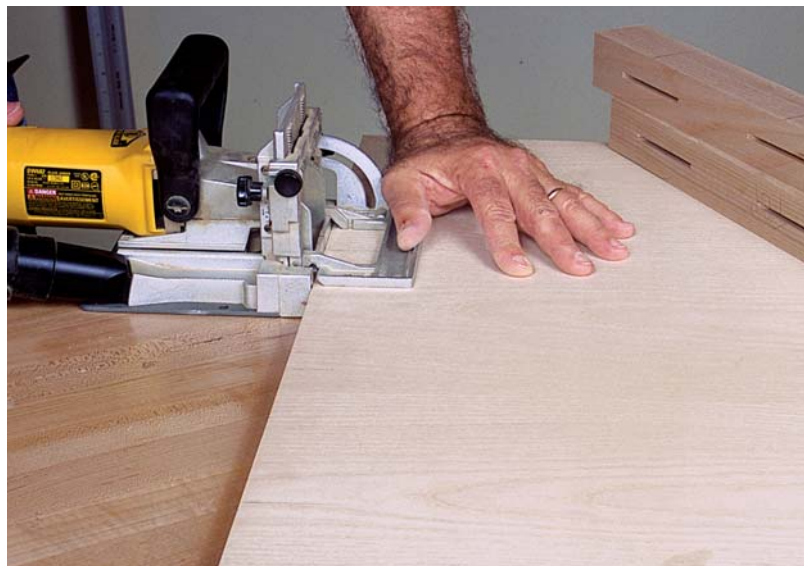
PHOTO I: Center the biscuit slots across the edges of all the panels.
