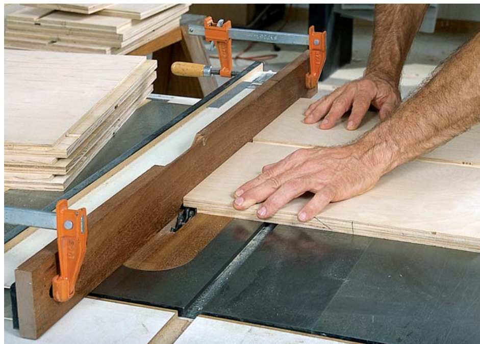
PHOTO F: Sawing rabbets on the table saw requires the use of an auxiliary fence to prevent cutting into your saw's rip fence.
