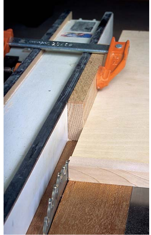
PHOTO H: To saw edging flush to the ends of panels, align a shim block flush with the outside face of the sawblade teeth.
