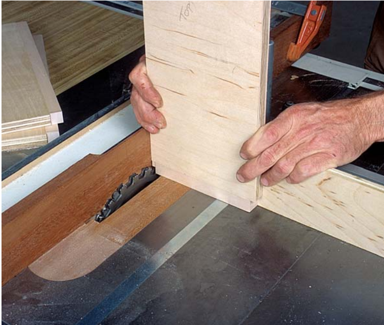
PHOTO I: To cut the notch where the end of a panel slips into a joint, the author uses a good dado head and an auxiliary rip fence. A miter gauge guides the workpiece, with a piece of scrap backing up the cut to minimize exit tearout.
