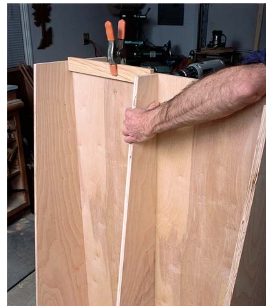
PHOTO G: When attaching the dividers, use spacers to temporarily hold them in position for screwing.
