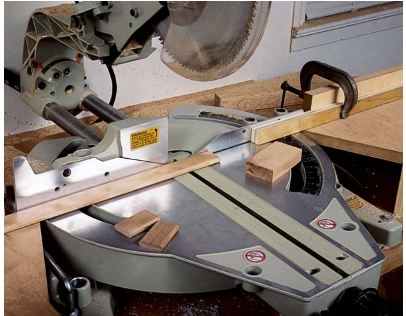
PHOTO B: To safely crosscut multiple short pieces like these loose tenons, set the cutup using a spacer placed against the stop block. Remove the spacer before making each cut.
