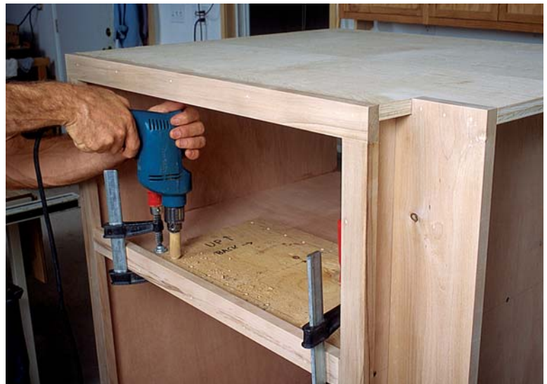
PHOTO G: A plywood template is used to establish the shelf-pin spacing. A dowel on the drill bit serves as a depth stop.
