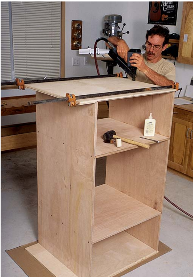
PHOTO A: Pipe clamps are used to pull the case top against its rabbet shoulder while gluing and nailing the sides to the top and bottom. The clamps are removed immediately after nailing.
