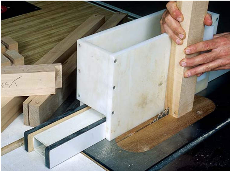
PHOTO B: The cheek cut for the rabbets was made using a shopmade tenoning jig on the table saw. The blade and fence have been set up using scrap, which was then test-fitted in the dado.
