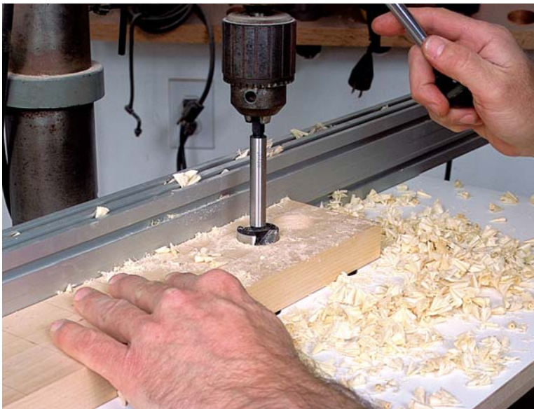
PHOTO E: Use a Forstner or multispur bit to drill flat-bottom holes in the rack bases, stopping short of the bottom by \frac{1}{8} in.
