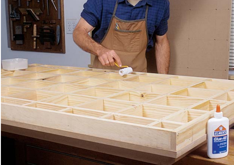
PHOTO F: Use a small paint roller to apply white glue to the ribs for attaching the panel.
