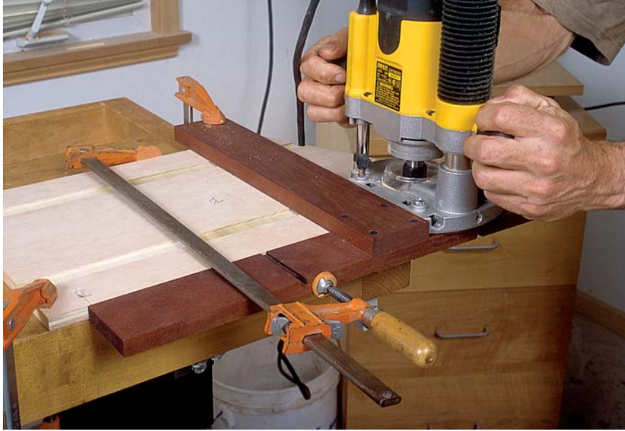
PHOTO N: To cut the lag-screw slots in the base, guide your router using a T-shaped jig clamped to the workpiece.
