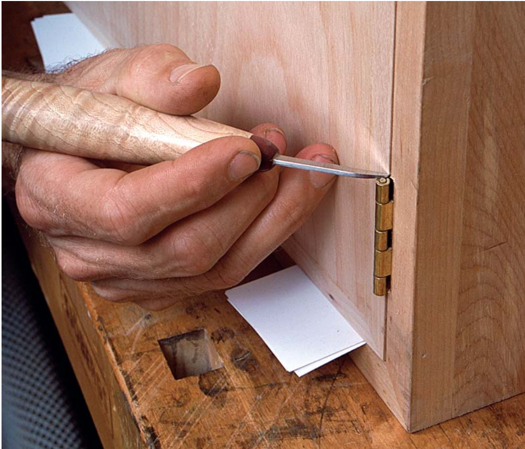
PHOTO A: After trimming the inset door enough to slip it in its opening, press its edge against the hinge that's installed in the case mortise. Lay a sharp knife blade against the hinge leaf, and press the blade into the door edge to transfer the hinge-mortise location to the door.
