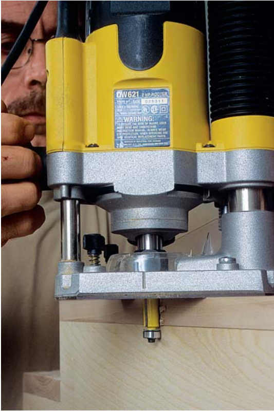
PHOTO E: Rout the face-frame overlap using a flush-trim bit.
