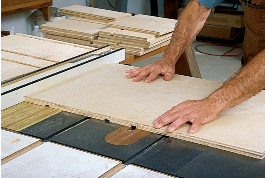
PHOTO E: When sawing dados with a dado head on the table saw, keep the workpiece solidly against the rip fence and maintain constant downward pressure near the joint.
