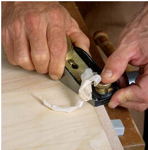
PHOTO B: Using a block plane set for a very fine cut, finish trimming the edging flush to the panels.
