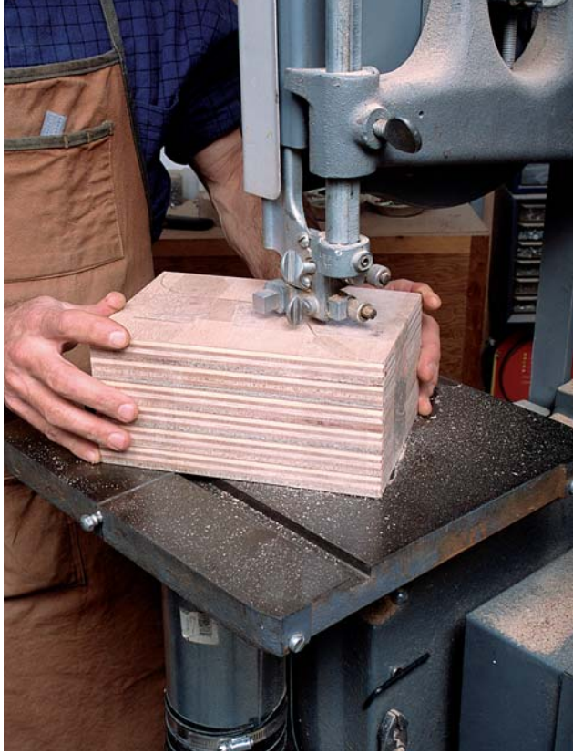
PHOTO A: When making the gussets, it's efficient to tape a stack of blanks together and gang-saw them on the bandsaw.
