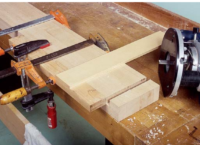
PHOTO A: Rout the dadoes in the base rails using a shopmade square to guide your router. For efficiency, gang the two rails together for the cut. (The extra edge joints you see here are a result of using butcher-block counter-top for the rail stock.)
