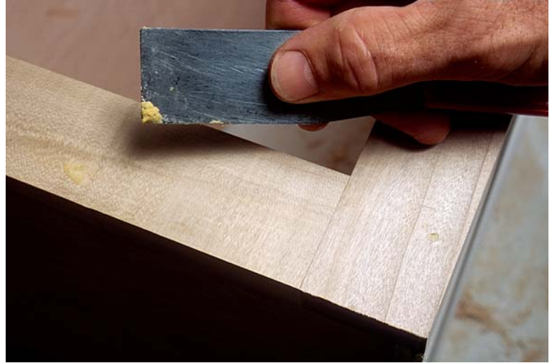
PHOTO F: When putting nail holes, load just a dab of putty on the corner of the knife to minimize the spreading of the putty into adjacent wood pores.
