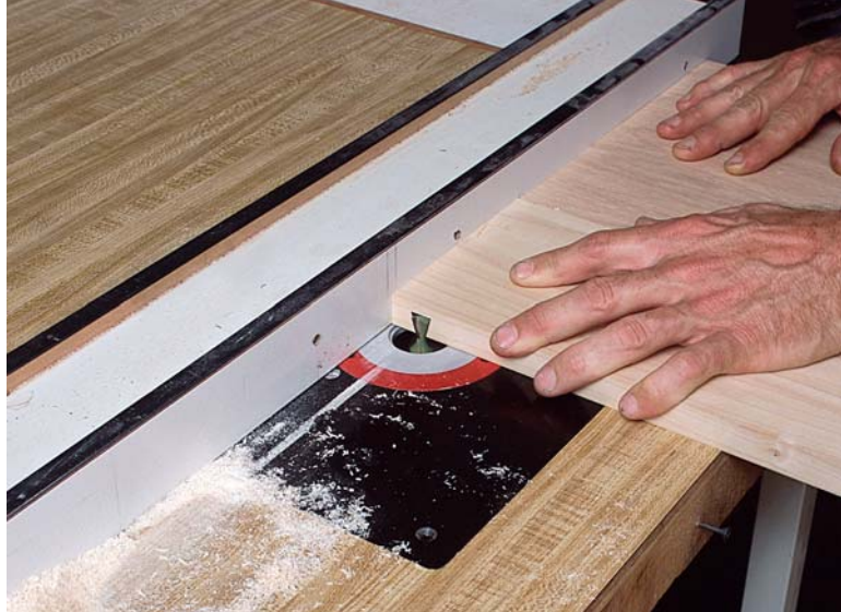
PHOTO G: After routing a groove with a straight bit to remove most of the waste, finish up the dovetail slot by routing it with a ½-in. dovetail bit. Hold the workpiece firmly against the fence while backing it up with a square piece of stock to support it and minimize exit tearout.
