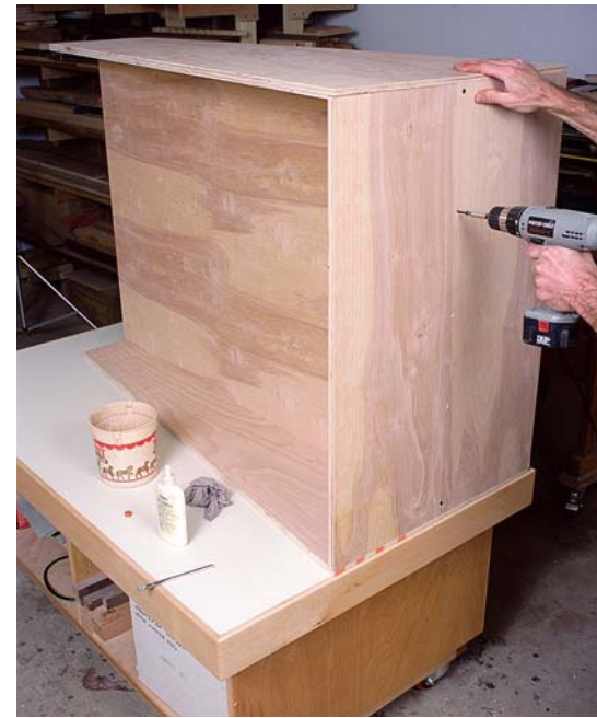
PHOTO F: After temporarily attaching the sides to the center panel with one screw each, glue the bottom panel to the center panel.
