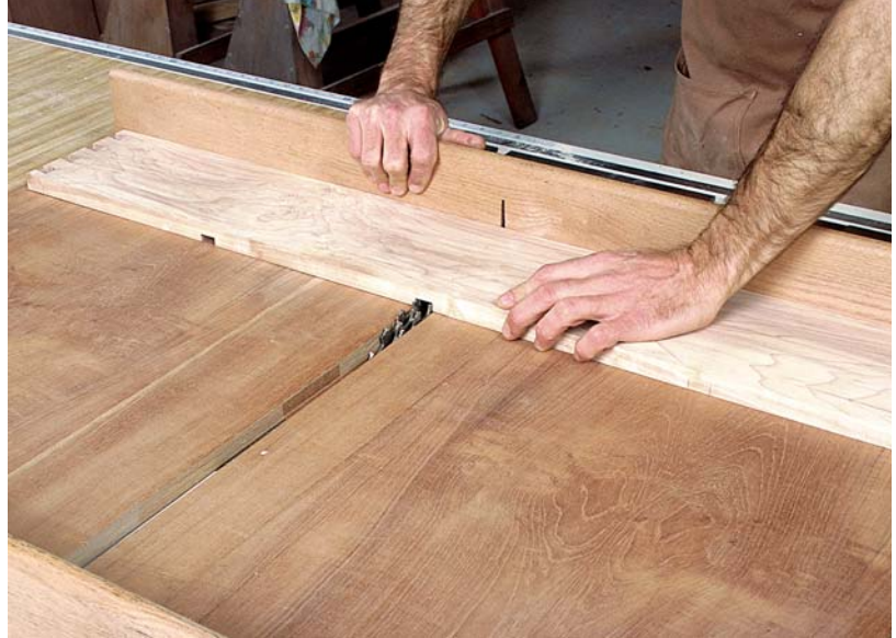
PHOTO A: You can cut the dados for the shelves and divider using a dado head on the table saw. Guide the workpieces using a crosscut sled or a miter gauge with a long auxiliary fence.
