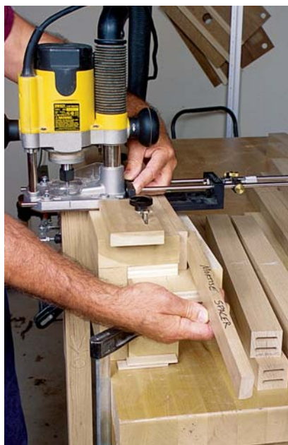
PHOTO B: To rout the second rail mortise, reposition the 5/8-in.-thick spacer behind the edge-guide fence, which shifts the router forward.
