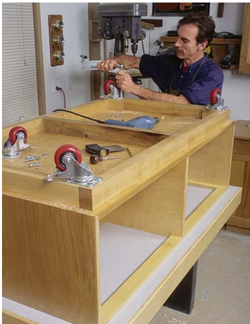
PHOTO M: Attach the casters to the base using lag screws and washers.
