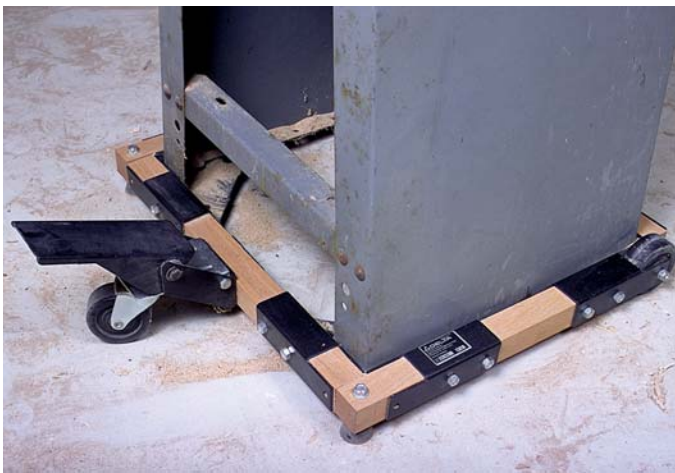
PHOTO F: A wide variety of mobile bases are available for woodworking machines. Delta® makes a kit that consists of corner brackets and a lift wheel to which you add suitable shopmade rails.
