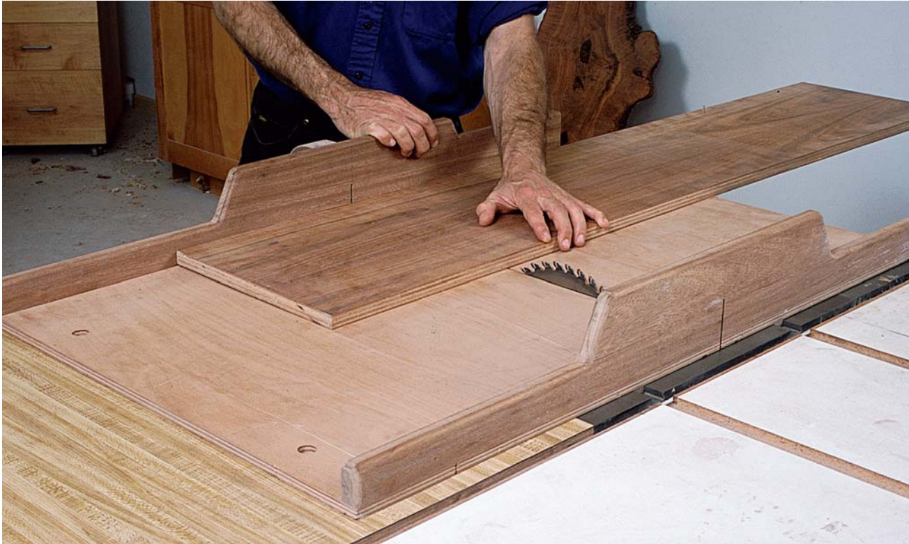
PHOTO C: A crosscut sled runs in the saw's miter-gauge slots and provides a long fence and base for carrying large workpieces safely and accurately through the blade.
