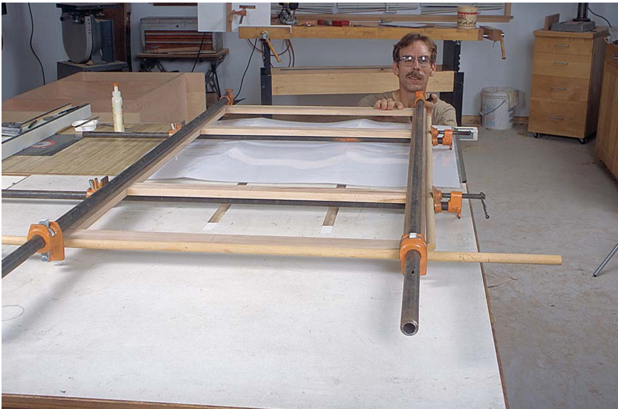
PHOTO D: To prevent buckling under clamp pressure, use \frac{3}{4} -in.-dia. dowels to center the pressure against the edges of the \frac{3}{4} -in.-thick stock. Sight down each clamp to make sure it's centered across the width of the workpiece.
