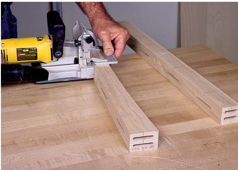
PHOTO H: When cutting the biscuit slots in the rails and legs, always reference your biscuit-joiner fence against the inner faces of the pieces.
