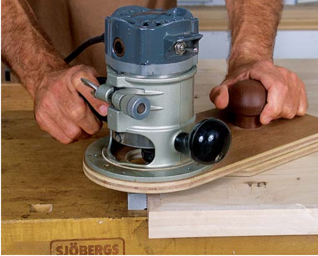
PHOTO A: Using a router with a flush-trim subbase, cut the edging almost flush to the surfaces of the outer panels.
