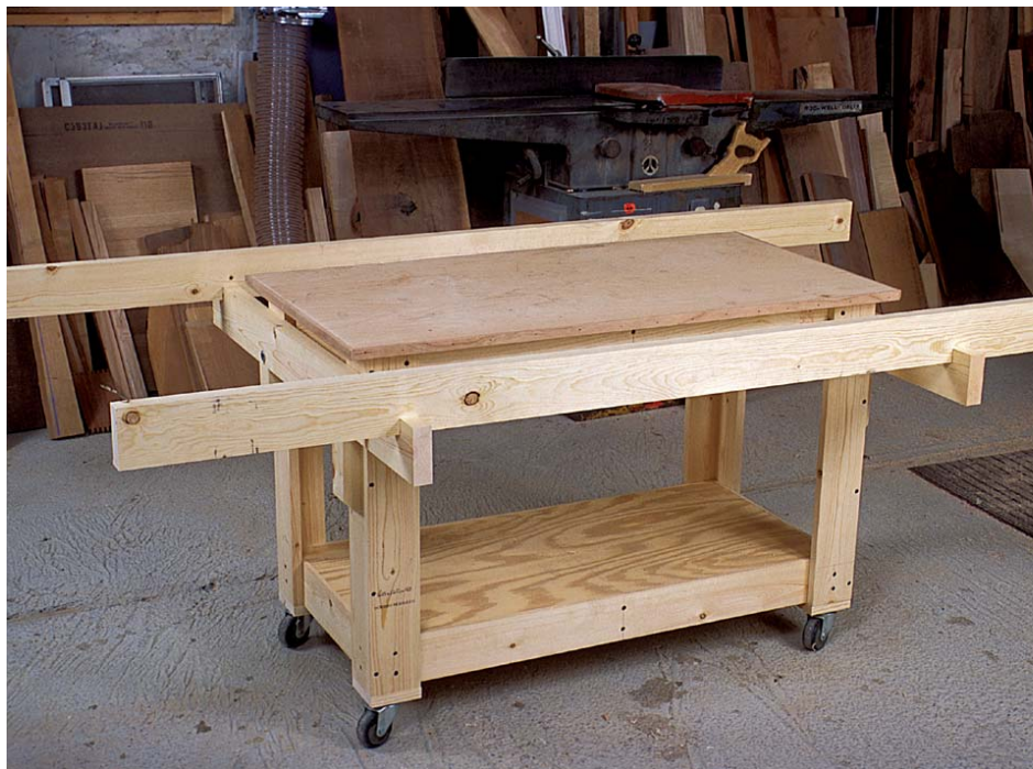
PHOTO D: Ken Burton's mobile parts cart is outfitted with removable outriggers for performing double duty as an auxiliary support when feeding sheets of plywood onto the table saw.
