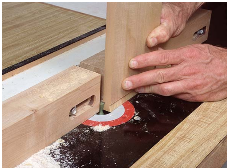
PHOTO H: Rout the mating tails by burying the bit the proper distance in the fence and feeding the drawer sides on end. Rout both faces, test the fit, and readjust the fence as necessary.
