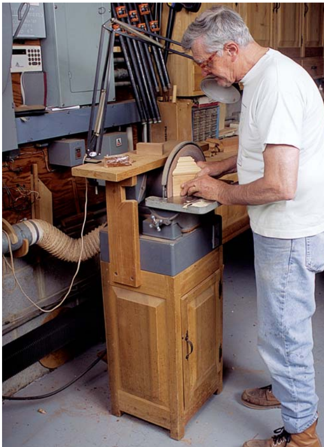
PHOTO H: A workstation should include everything needed for a particular process. Andy Rae's sharpening station consists of a grinder, a stone pond, and a cabinet to house various sharpening jigs. Note that the grinder is placed at a comfortable height and is shrouded to prevent it from scattering metal particles.
