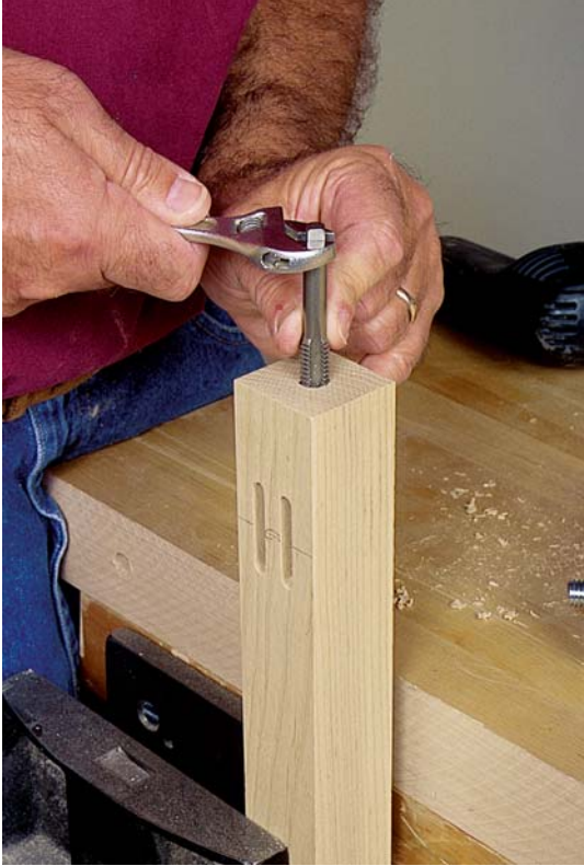
PHOTO D: Thread the hole for each caster bolt using a tap
