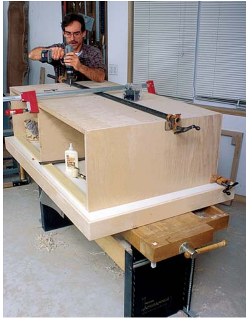
PHOTO L: With the sides dry-clamped to the spine and with the unit upside down, glue and screw the bottom to the spine and divider using #6 by 2-in. drywall screws.
