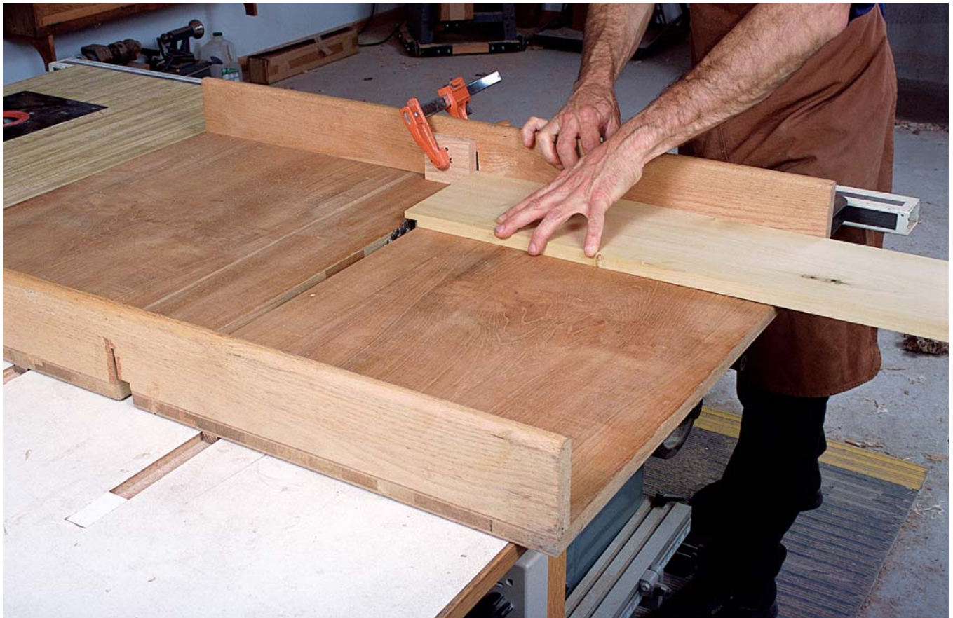
PHOTO C: One way to easily cut rabbets in the ends of long boards is to use a cross-cut sled to feed the workpiece across a dado head on the table saw.
