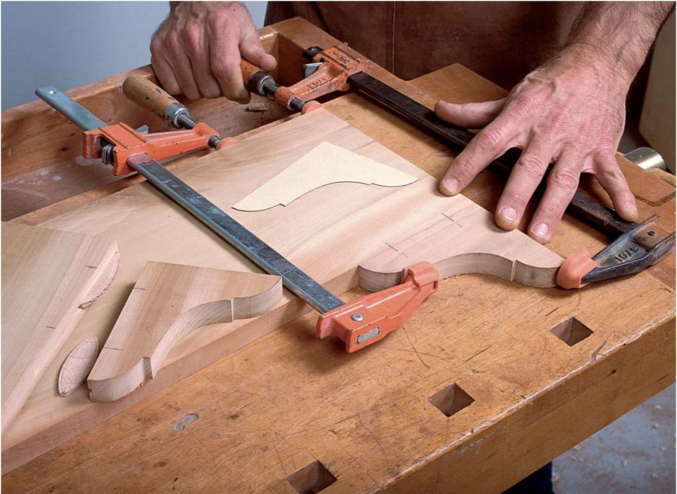
PHOTO D: After cutting the biscuit joints, clamp the corbels in place using clamps with soft jaw pads.
