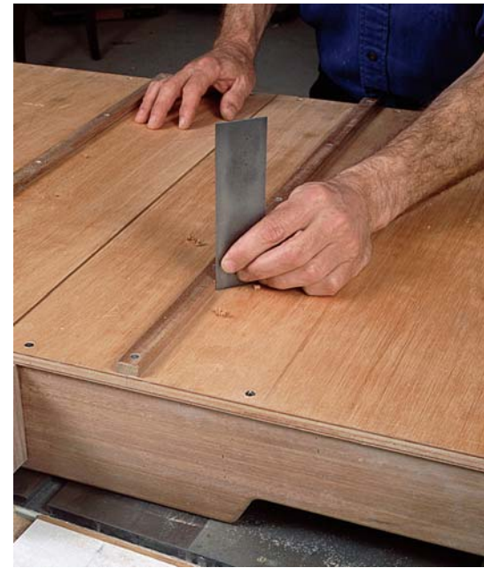
PHOTO D: A scraper blade works great for trimming the sled runners for an easy, sliding fit in the saw's miter-gauge slots. Shave a bit at a time from any area that shows glossy rub spots from travel in the slots.
