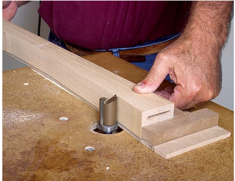
PHOTO E: After bandsawing close to the rail’s curved cut line, use a template and pattern bit to rout to the final profile.
