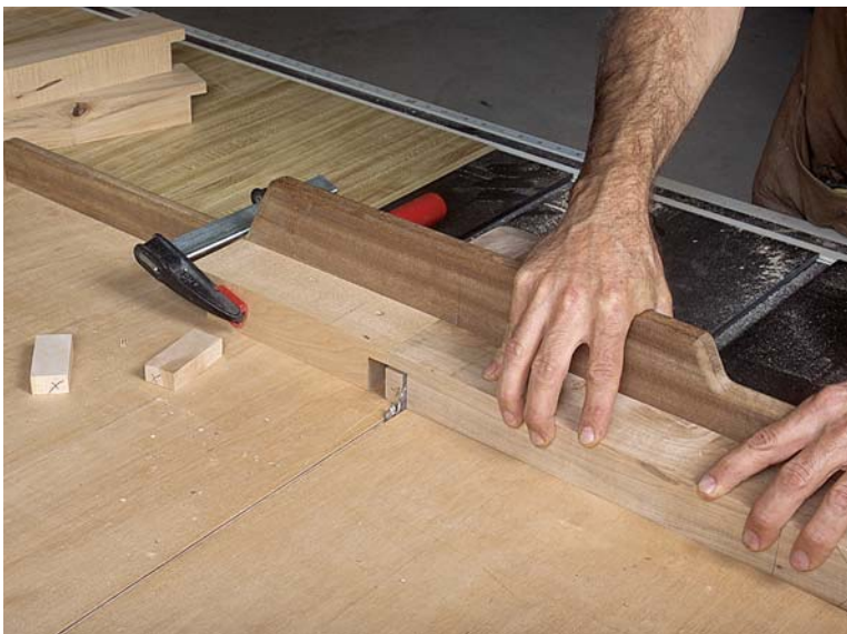
PHOTO C: The shoulder cut for the rabbet was made using the table-saw crosscut sled. The test piece cut for the previous step makes the perfect stop block, allowing space for the offcut to fall away.
