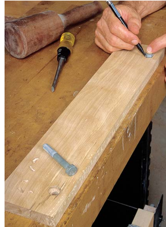
PHOTO O: To cut the bolt-head recesses in the extension-table backs, insert a bolt into each hole and then trace around the head with a sharp pencil. Clean out the waste with a chisel, making the recess just slightly deeper than the head.
