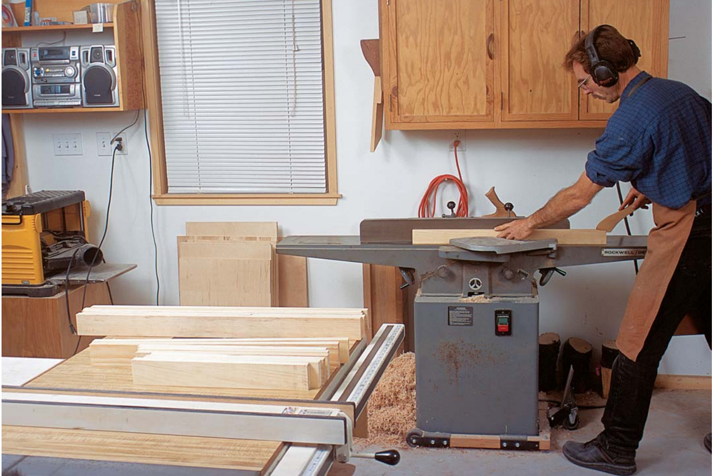
PHOTO E: Locating a jointer near a table saw makes for efficient milling and allows use of the table-saw wing as staging for workpieces being jointed.
