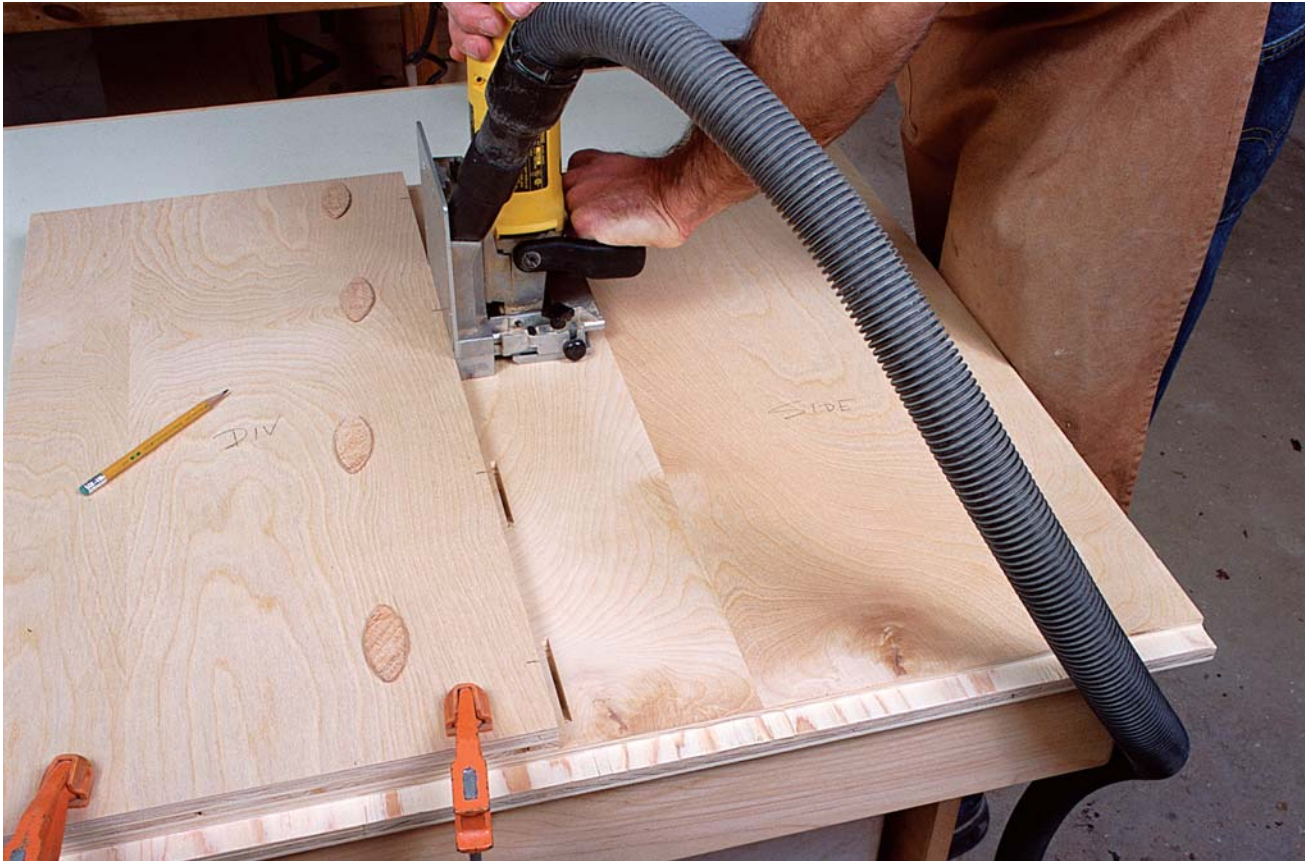
PHOTO F: After marking out the divider location, clamp it adjacent to its layout line. Cut the slots in the case side registering the biscuit-joiner base against the divider. Afterward, cut the slots in the end of the divider.
