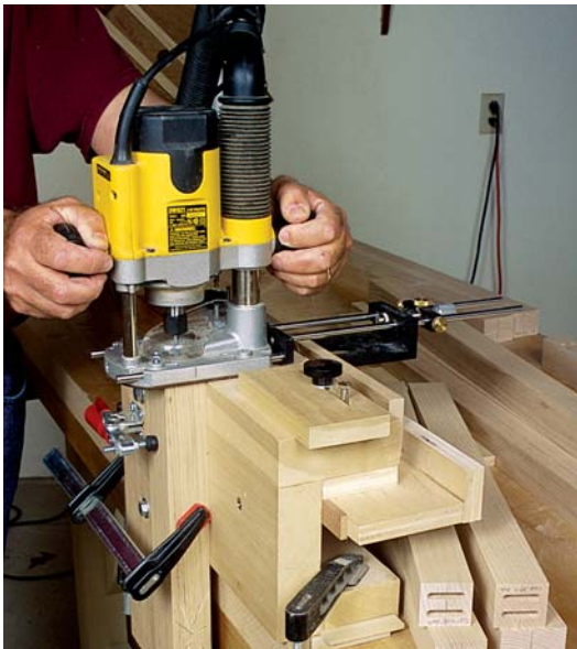
PHOTO A: To rout the first mortises in the end of a rail, mount the rail to the mortising jig, clamping it to the vertical work holder. Make the cut with a 5/8-in.-thick spacer placed between the edge-guide fence and the rear of the jig.
