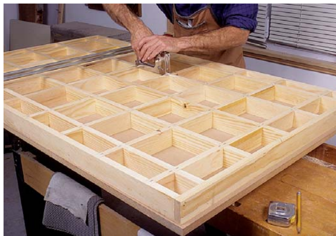
PHOTO E: A staple straddling each short rib and full-length rib holds the pieces together. A bar clamp applies pressure across the assembly to ensure snug contact of the pieces.
