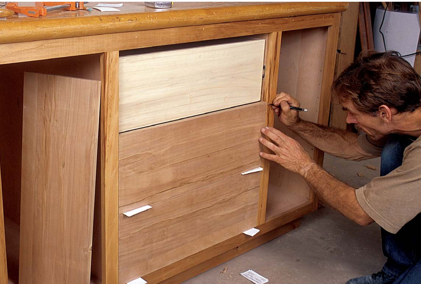
PHOTO J: To fit the drawer fronts, shim them for proper spacing and then mark the ends near the corners for a consistent gap, making sure they're parallel with the adjacent stiles. Connect the marks with a fine pencil line run against a straightedge, and plane to the line.
