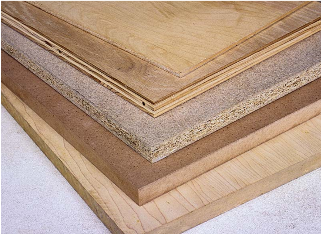
PHOTO K: Hardwood plywood is available with a variety of face veneers, including birch, lauan, and oak. MDF is a dense, stable, flat form of particleboard suitable for applications that require smooth, dead-flat surfaces.
