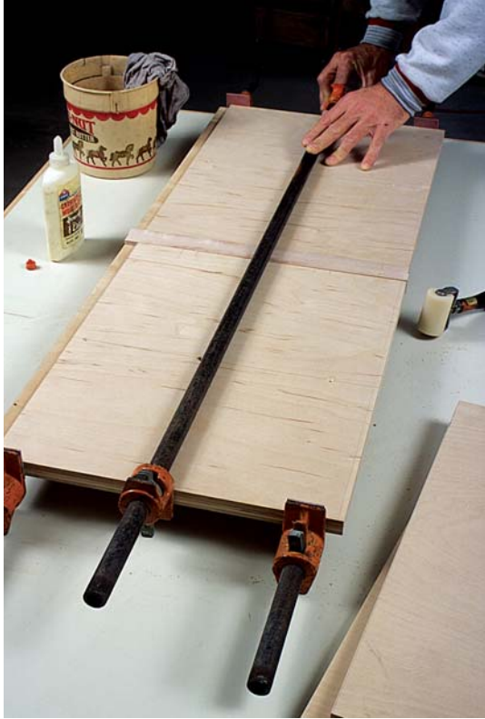
PHOTO G: When gluing edging on similarly sized panels, sandwich the edging between the two panels. Alternate clamps over and under to prevent the workpieces from buckling under pressure.
