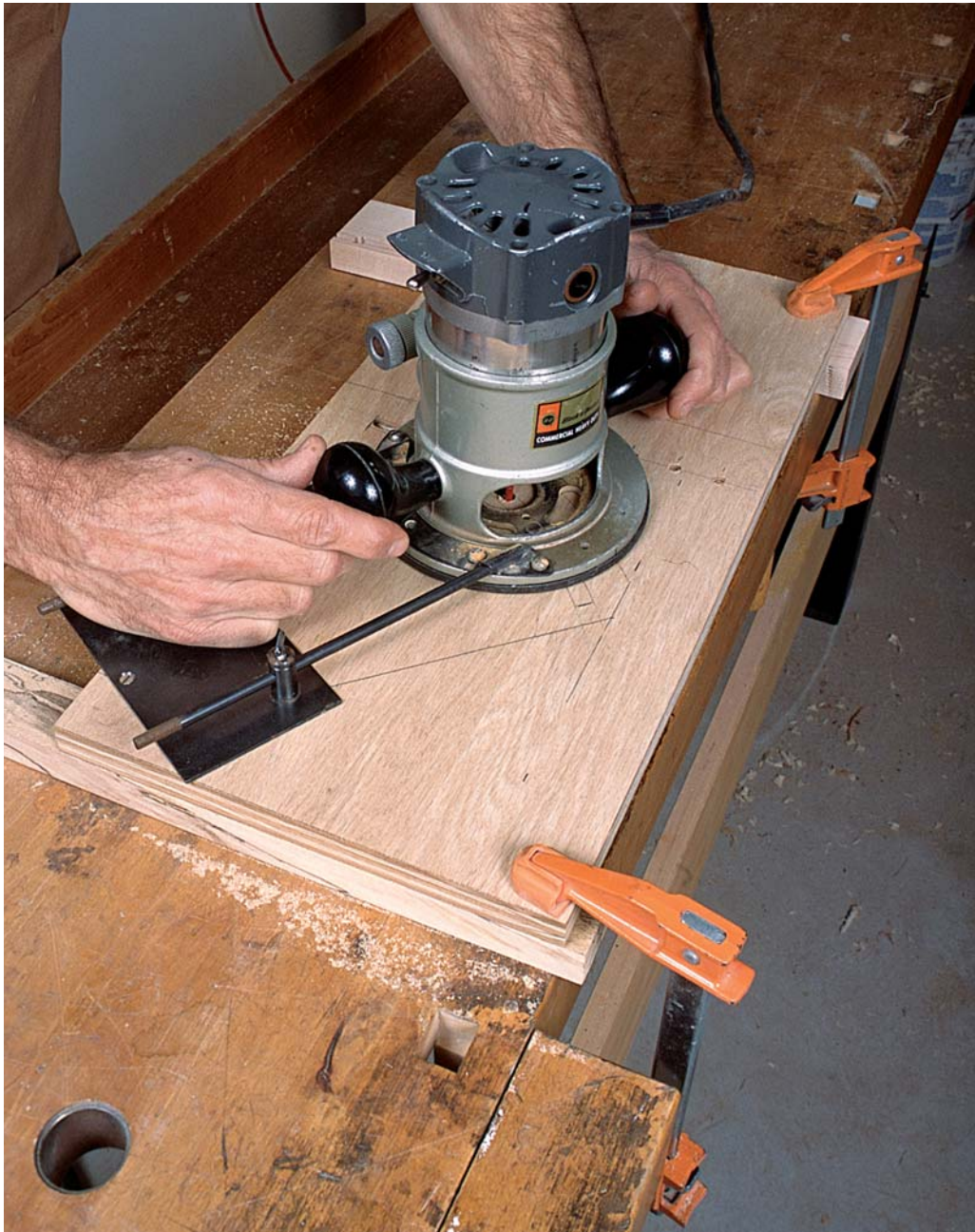
PHOTO D: After laying out the brackets, use a trammel to cut the curved slot before sawing the brackets to final shape.
