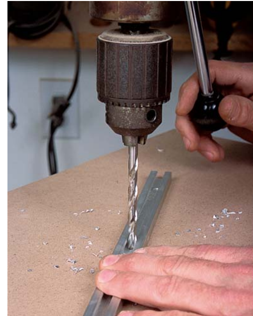
PHOTO F: After drilling the screw-clearance holes in the T-track, use a ½-in.-dia. twist drill bit to countersink them for #6 flathead screws.
