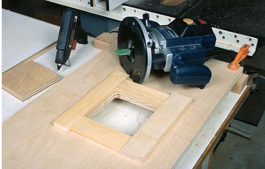
PHOTO C: After sawing the opening for the insert slightly undersize, place the insert over the hole and surround it tightly with blocks affixed to the table using hot-melt glue. Then use a pattern-cutting bit guided by the blocks to finish the cut.
