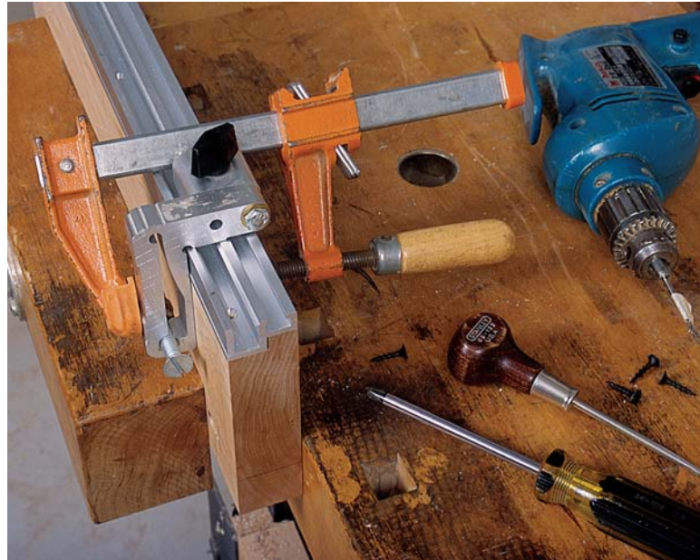
PHOTO Q: For accurate alignment when installing the half-track, attach a flip stop to the track and then clamp it against the face of the fence before drilling the track attachment screws.
