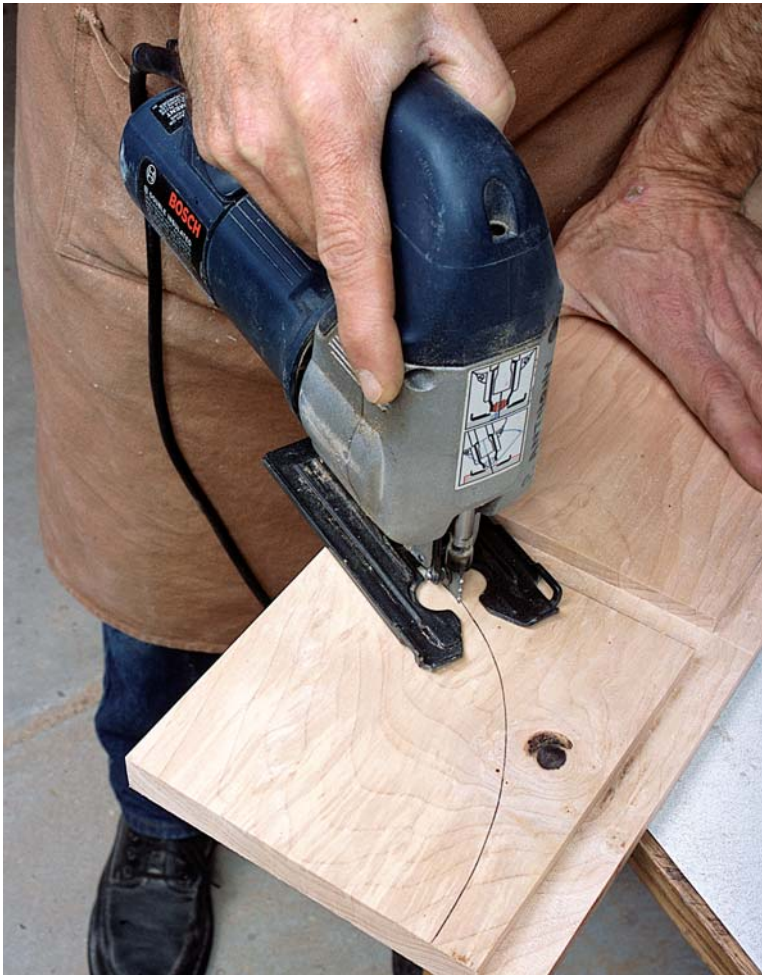
PHOTO D: Cut the curves on the bottom edges of the sides after sawing the dados for the bottom shelf and the rabbet for the back.
