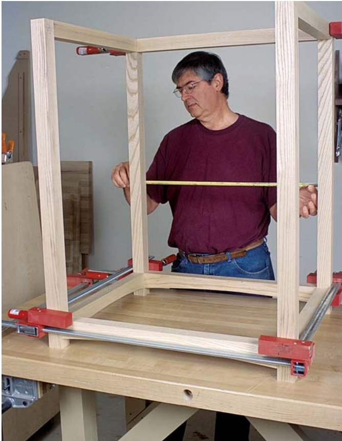
PHOTO G: After dry-clamping the legs and rails, Hylton measures the openings to determine the measurements for the back, bottom, and side panels.
