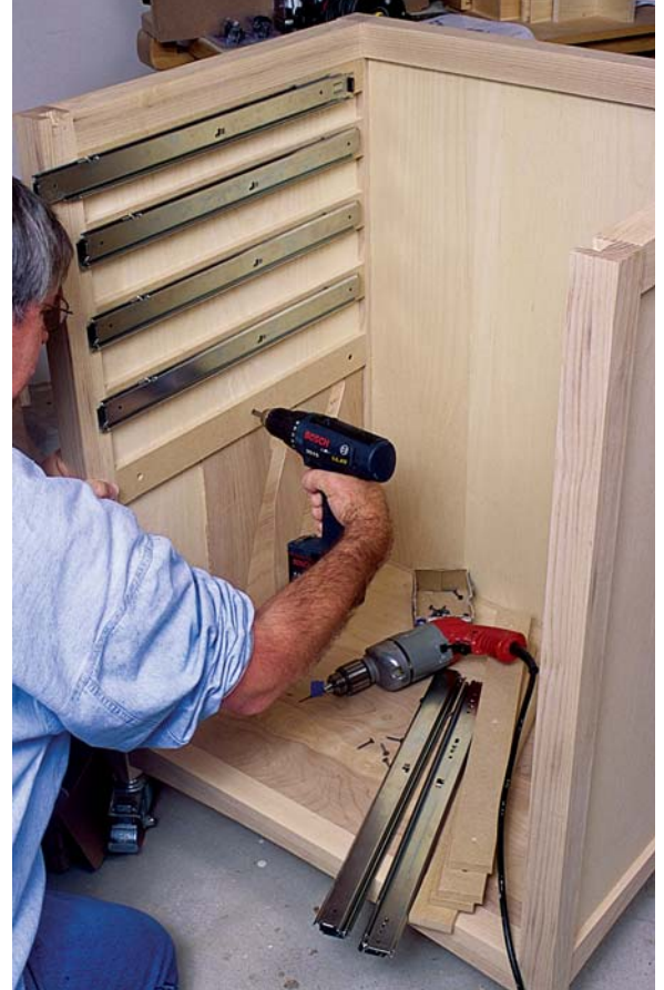
PHOTO J: To keep the drawer-slide shims perpendicular to the case front, Hylton rests each shim on a square plywood panel pressed against the case side. Starting with the uppermost slides, he works downward, sawing the panel shorter to install each subsequent pair of shims.
