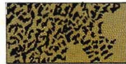
Silicone carbide is a synthetic. It is shiny, black and has sharp cutting slivers.
