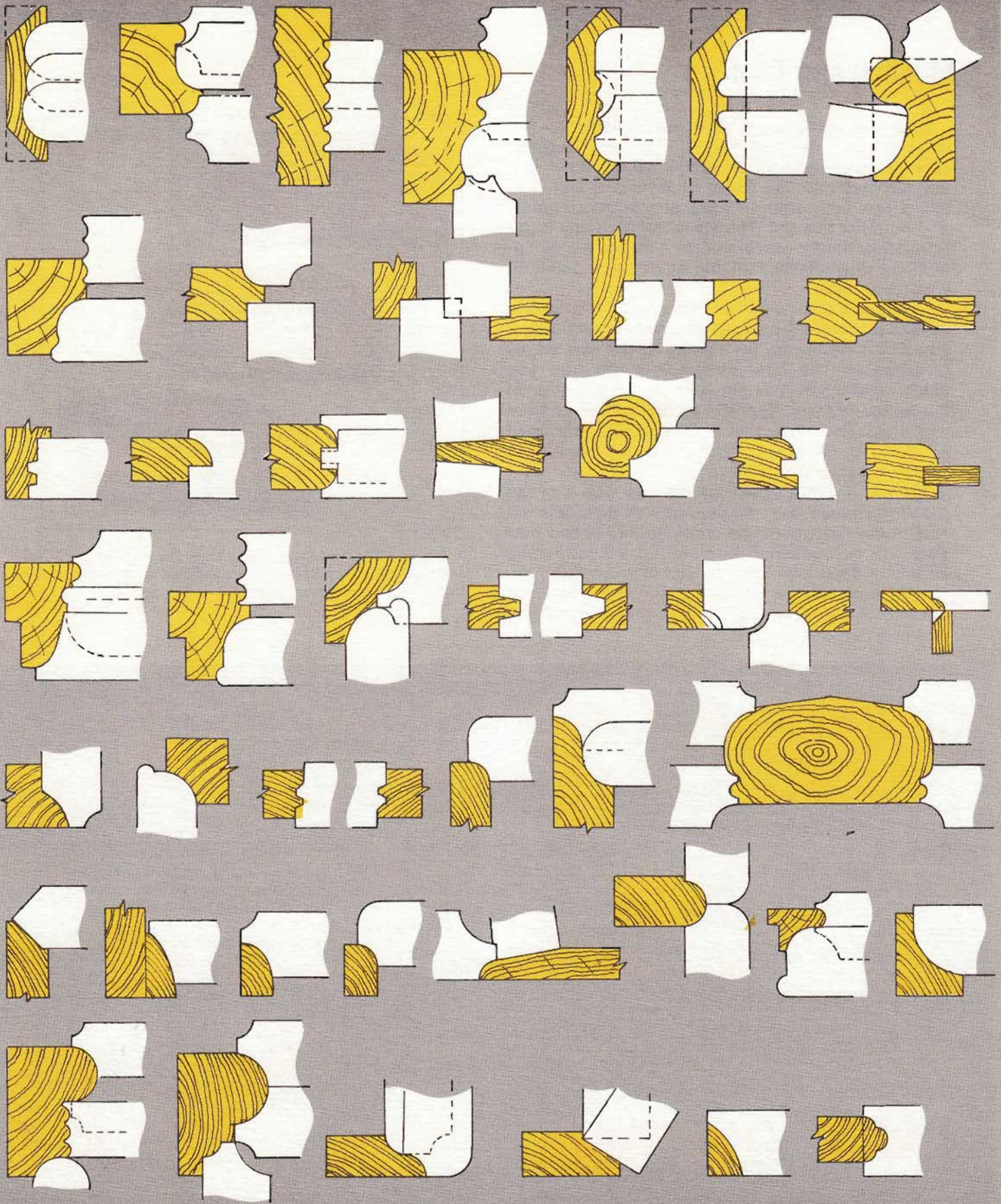
The molding blades shown above can be used in combination to create all the designs shown here, as well as a great many other configurations.
