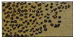
Garnet is a reddish brown mineral and provides a medium hardness but with excellent cutting edges.
