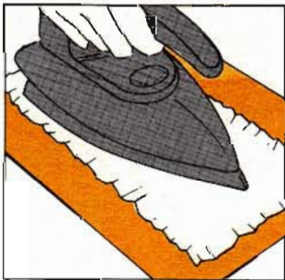
Another way of flattening blisters is to iron them with a moderately warm iron. Put aluminum foil between the iron and the veneer.
