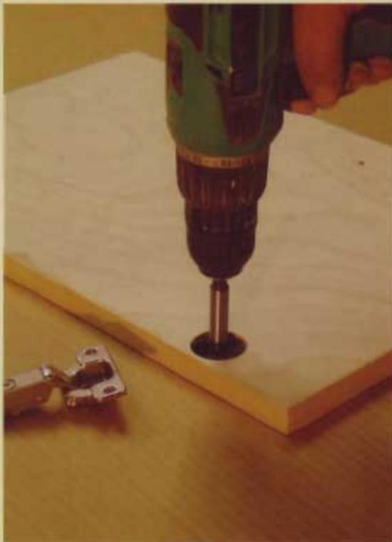
**1** The hinges come in two parts: the hinge cup and the mounting plate. Start by drilling a hole in the door to hold the hinge cup. You'll need a 35mm or 1<sup>3</sup>/<sub>8</sub>" Forstner bit. To locate the center of the hole for the hinge cup, make a pencil mark <sup>7</sup>/<sub>8</sub>" (22mm) from the edge of the door.
