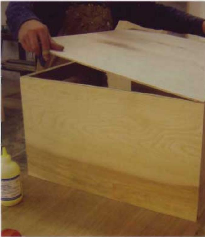
**5** These cabinets can have the backs screwed directly on to the cabinet cases.
