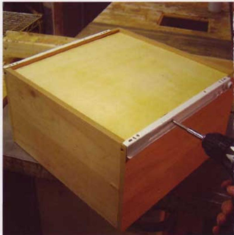
**14** With the drawers placed upside down on a workbench, it's easy to install the drawer-side runners with self-tapping  $\frac{1}{2}$ " (13mm) screws. Then you can set the drawers into the cabinet whenever you're ready.
