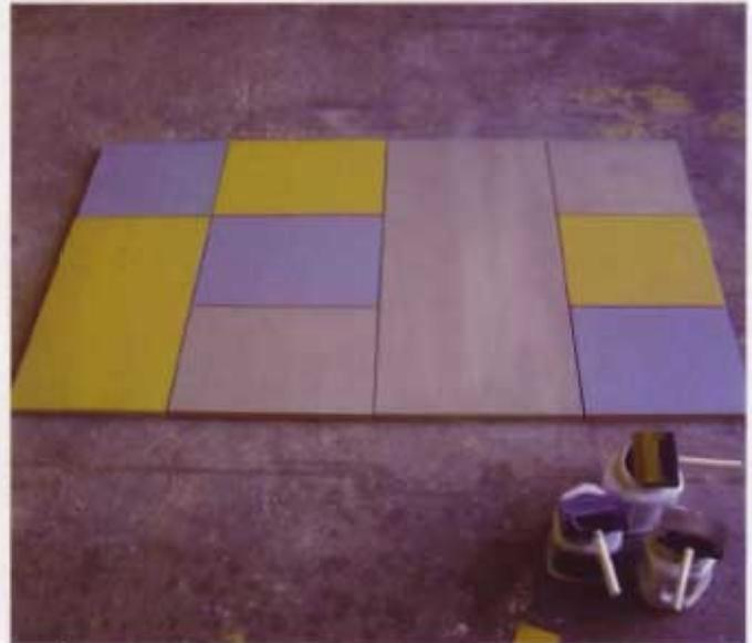
8 Making the doors and drawer fronts for this project couldn't be simpler. No edge-banding is required, and all you need to do is cut out MDF rectangles. To help develop the color scheme for this project, I laid out the doors and drawer fronts in their actual configuration. For me this was much easier and more direct than trying to work on paper.
