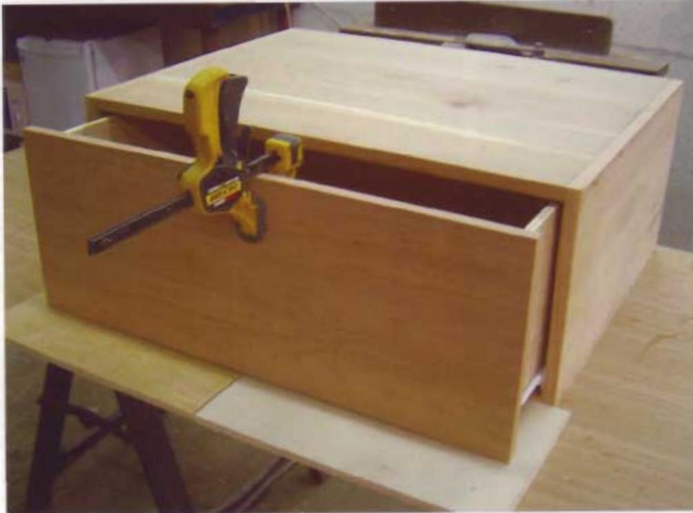
**13** For the single drawer box, place a  $\frac{1}{2}$ " (13mm) shim beneath the drawer front to set it at the proper height.
