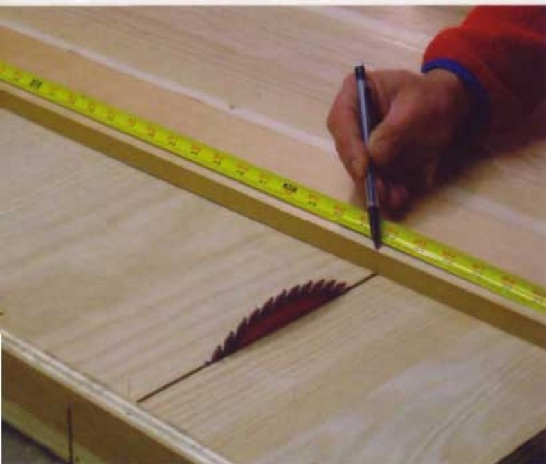
**1** Cut the end panels first. They are the largest components and the smaller pieces can later be fabricated from their offcuts. Then cut all the other  $\frac{3}{4}$ " (19mm) cherry parts.
