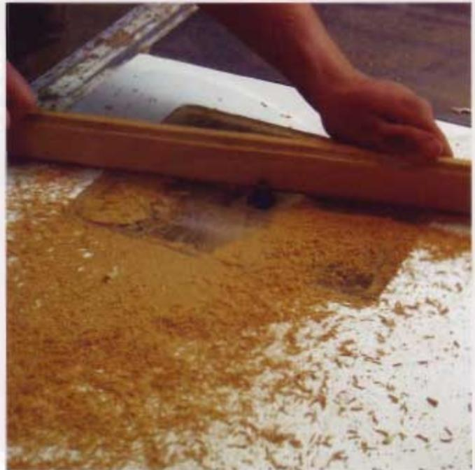
**8** Since this was a pretty elegant project, I decided to tile the top with 12" x 12" (305mm x 305mm) limestone. That meant installing a 1 3/4"-wide (44mm) trim strip for the front edge, because the tiles are 1/4" (6mm) thick. If you're doing a standard wooden top, make the trim strip 1 1/2" (44mm) wide. I routed the top and bottom edges of the strip on the router table.
