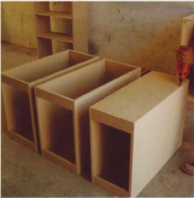
5 Since this project allows for some "quick and dirty" construction techniques, you can simply screw and glue the backs directly onto the cabinet boxes.
