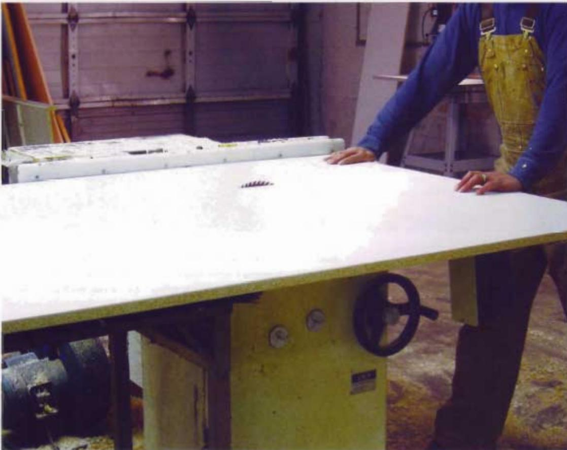
**1** Build the smaller, wall-hung cabinet first. I cut the parts to size using my table saw and a blade specifically meant for cutting melamine. While most any combination blade will provide acceptable results, melamine-specific blades tend to produce the smallest amount of tear-out.
