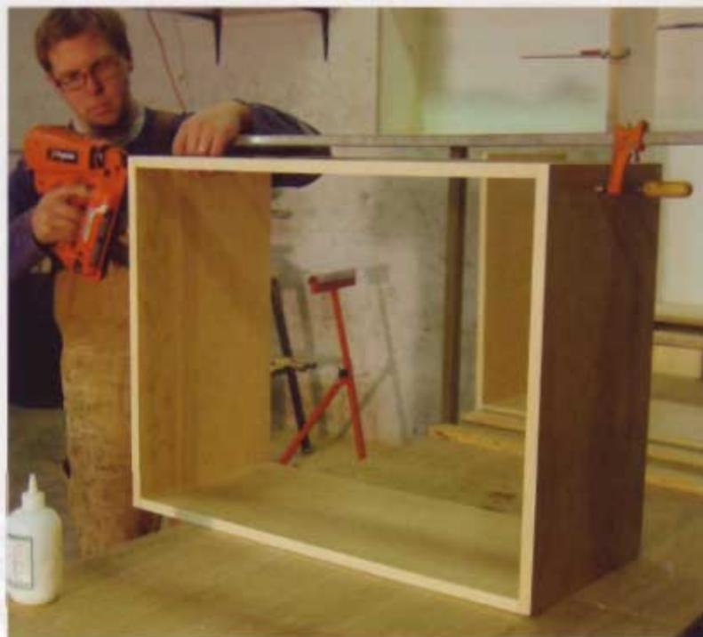
**4** The layout of some of these cabinets allows a few shortcuts in their construction. You'll notice that the sides of cabinets B,C,E and F are not exposed. This means you can save some time by just nailing or screwing the cases together.
