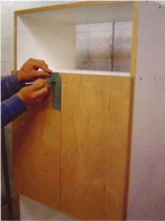
**9** An inexpensive template (available at most home centers) makes for quick and consistent layout of the door pulls. You can see that the grain of the doors matches nicely—this is because they came from the same piece of plywood.
