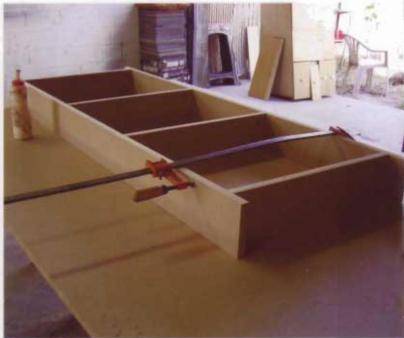
**2** The cabinet boxes sit on a single base. It measures 4½" (114mm) high and spans almost the entire footprint of the niche. I set the sides in about 1" (25mm), just in case the front and back of the base needs to be trimmed for a precise fit. Position the center supports evenly across the interior of the base.
