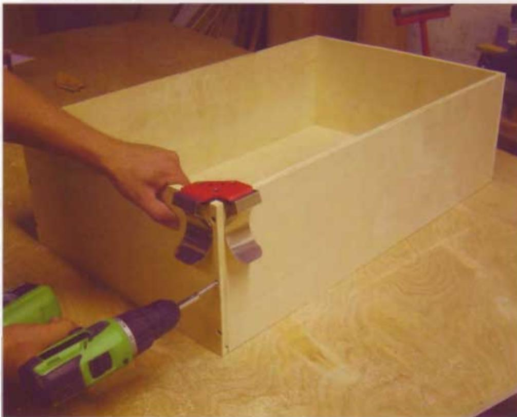
**12** I kept it simple and glued and nailed the drawers together. Then I varnished them. For details on the drawer installation, see *Installing Drawers with Accuride-style slides* on page 50.
