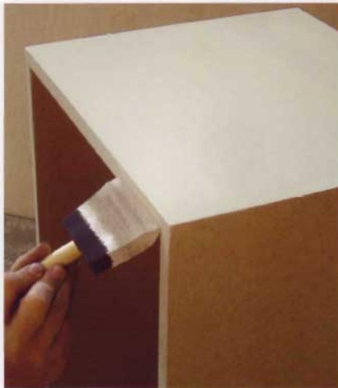
**8** Paint the dresser units before installing the drawers to avoid getting paint on the drawers and sliders. The only parts that need paint are the tops and the front edges, as the drawers will hide the insides and the end panels will conceal the outsides.
