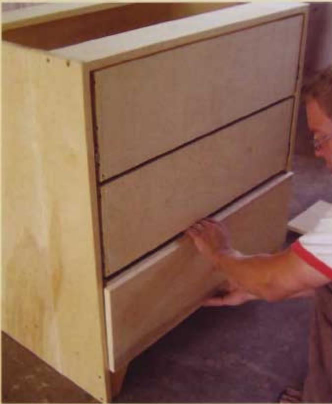
**3** Place a screw into the first hole on each side of the drawer, then pull the drawer out. Apply downward pressure on the drawer to make sure it is sitting flat and level, then screw in the back of the slides as well. When the bottom drawer is in, remove the spacers and place them on top of the drawer—this paves the way for the next drawer to be installed. The top drawer is installed in the same way.
