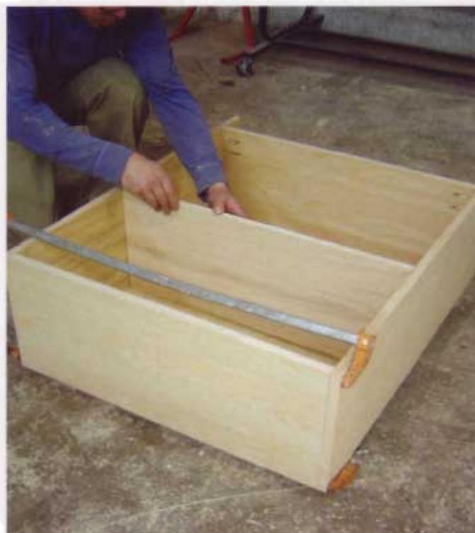
8 The center shelf is installed with pocket screws. Measure up 21 1/4" (540mm) from the bottom edge of the side panels and align the top side of the shelf accordingly.
