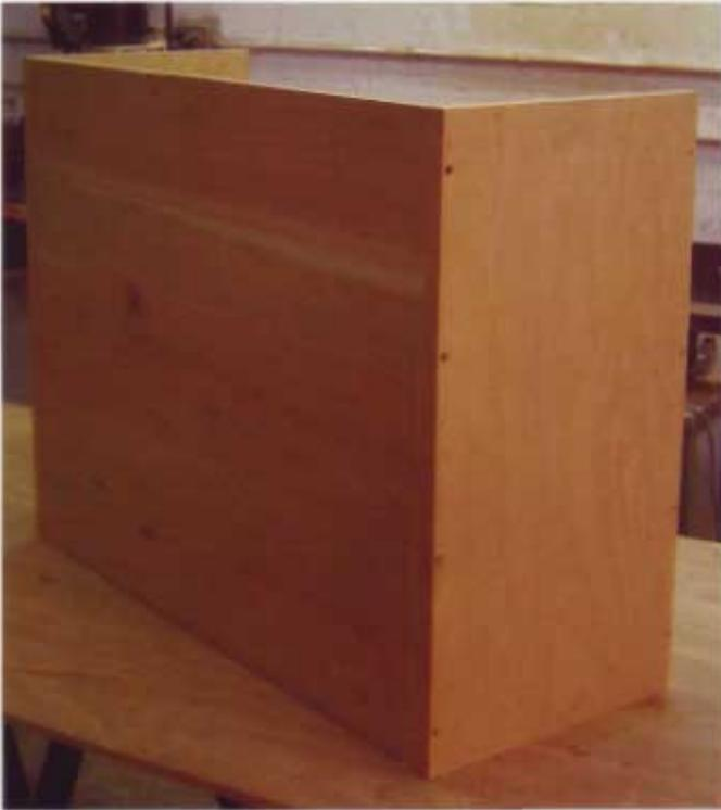
**7** Build the single drawer box and install the cabinet side runners in it. I positioned the front corner of the runners  $\frac{1}{2}$ " (13mm) above the cabinet bottom.
