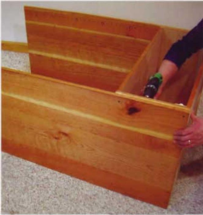
**22** The shoe cubbies above the single drawer unit are made with two short end panels attached to the sides of the drawer box. I ran screws front the inside and the outside the box for maximum holding power.
