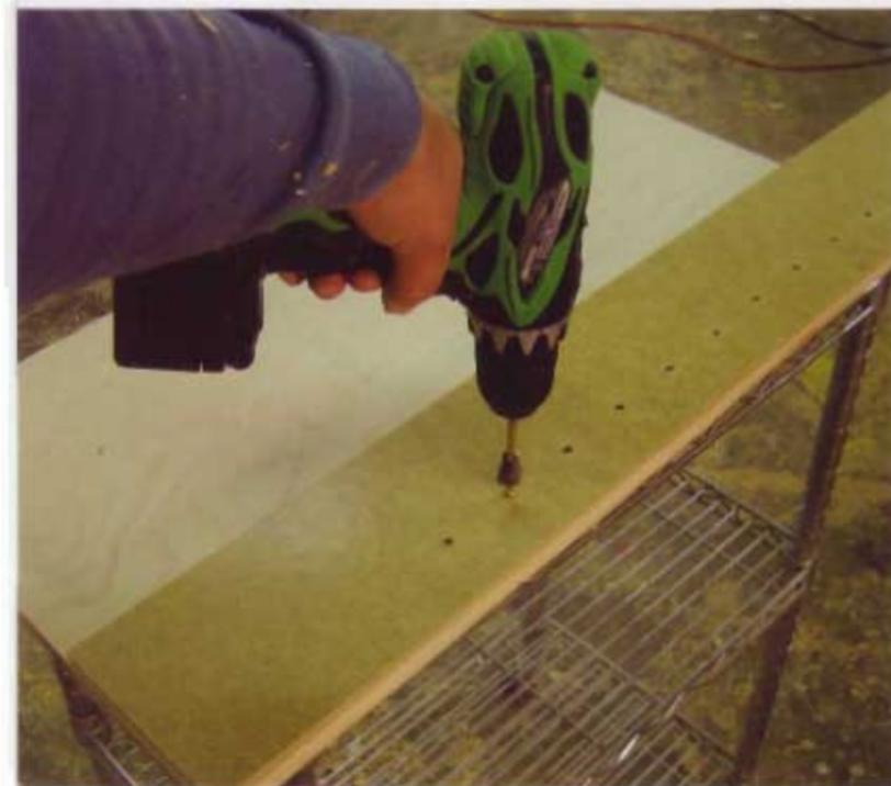
**3** The cabinet parts require some work prior to assembly. You can do the edge-banding now or later, but I find it easier to drill the shelf-peg holes early on in the process.
