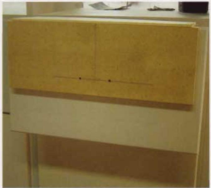
**17** Because the holes for the chosen drawer pulls required unique spacing, I made my own alignment guide and I used it for all six drawers.
