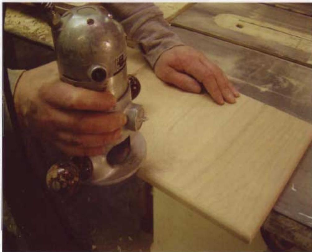
**15** I detailed the front edges of the MDF drawer fronts using a  $\frac{3}{8}$ " (10mm) roundover bit. This detail looks nice and eliminates the chipping that often occurs on edges left at 90°. Drawer fronts can be a high-wear area.
