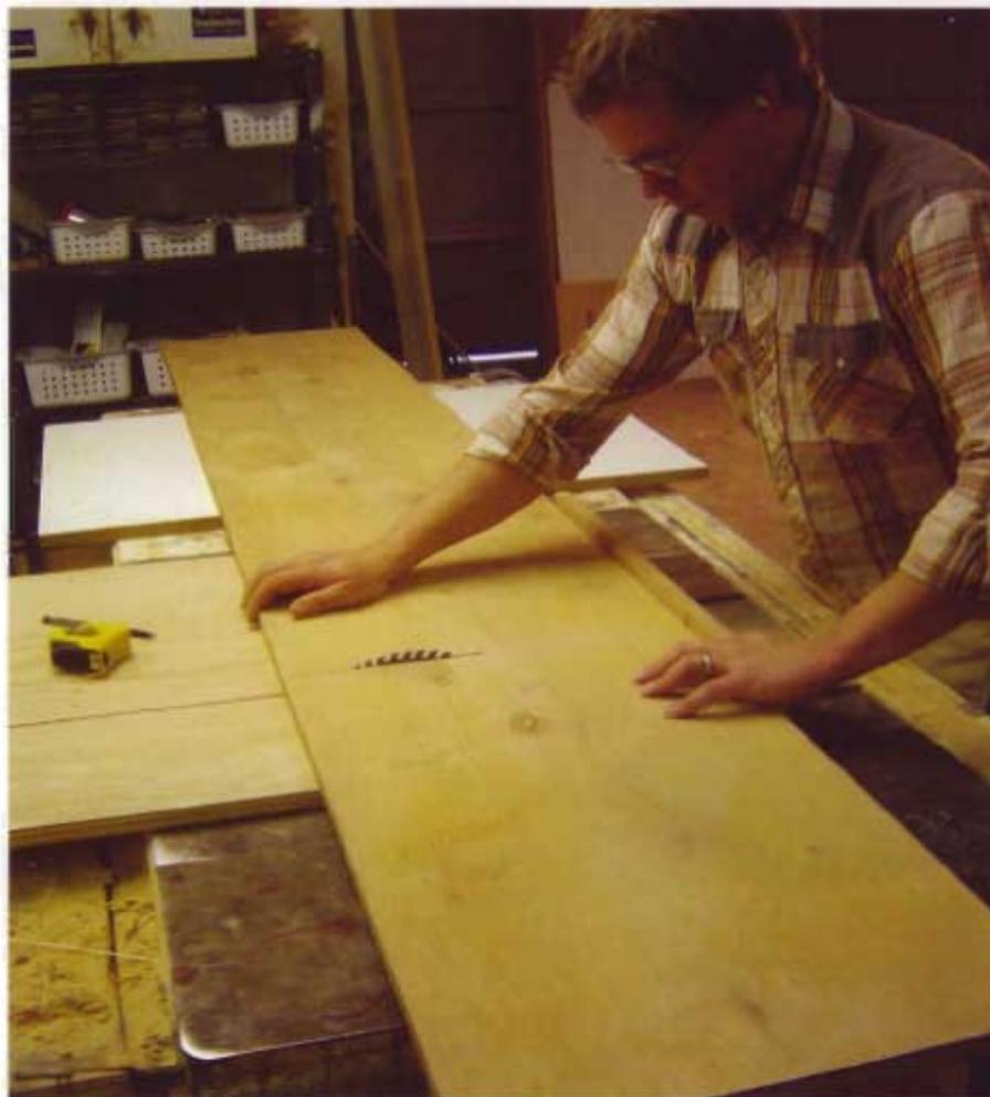
**1** Begin by cutting out the parts for the dresser units. I used MDF because it takes paint well and requires no edge-banding, a detail which saves a considerable amount of time. You'll notice that some of the material I used is veneered with alder. I used it only because I got a good deal on it and was able to position those components in such a way that they wouldn't be visible after installation. It's also a good idea to cut out the three end panels at this time, since you're set up for it.
