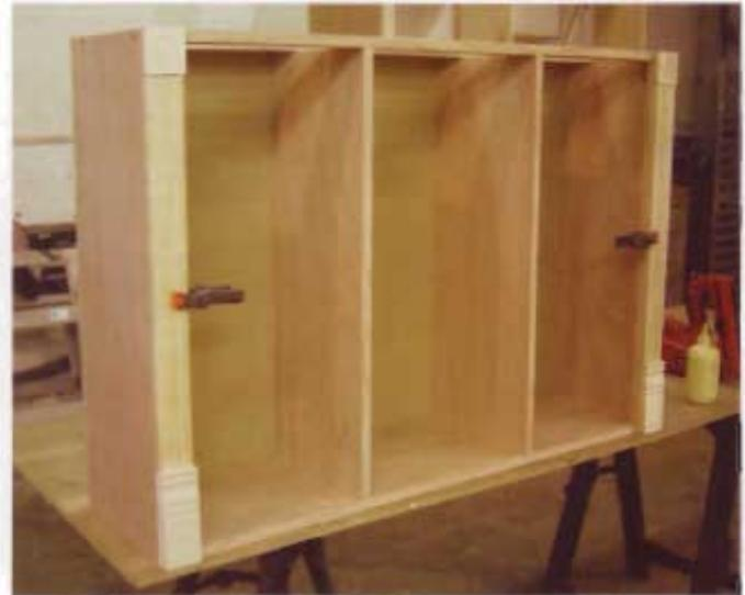
**2** Rip and crosscut the parts for the base cabinet, then assemble it with screws. The screw heads won't show, since end panels will cover the sides of the cabinet. We dressed up the cabinets with some trim from a local home center. The trim consists of a length of fluted molding, a rosette and a plinth. The parts are glued and nailed to the cabinet, and the nail holes are later filled with a stainable putty. Screw the two vertical partitions from the top, bottom and back.
