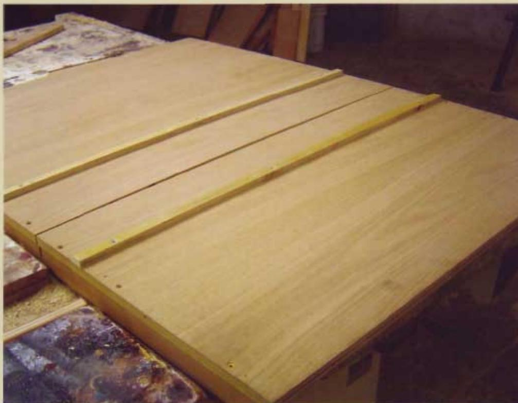
You'll want to start by milling two strips of hardwood that fit into the grooves on the table-saw top—they should move easily from front to back, but they should have very little side to side movement. The
