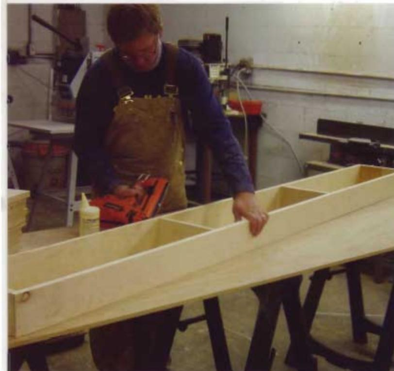
**1** Begin by assembling the cabinet bases with glue and nails. Don't worry about the nail heads being exposed because a piece of trim will cover it later on. You'll also notice that the stretchers are inset to the fronts and backs, which is important because it allows you to use stretchers of the same length for both the sides and the interiors of the bases.
