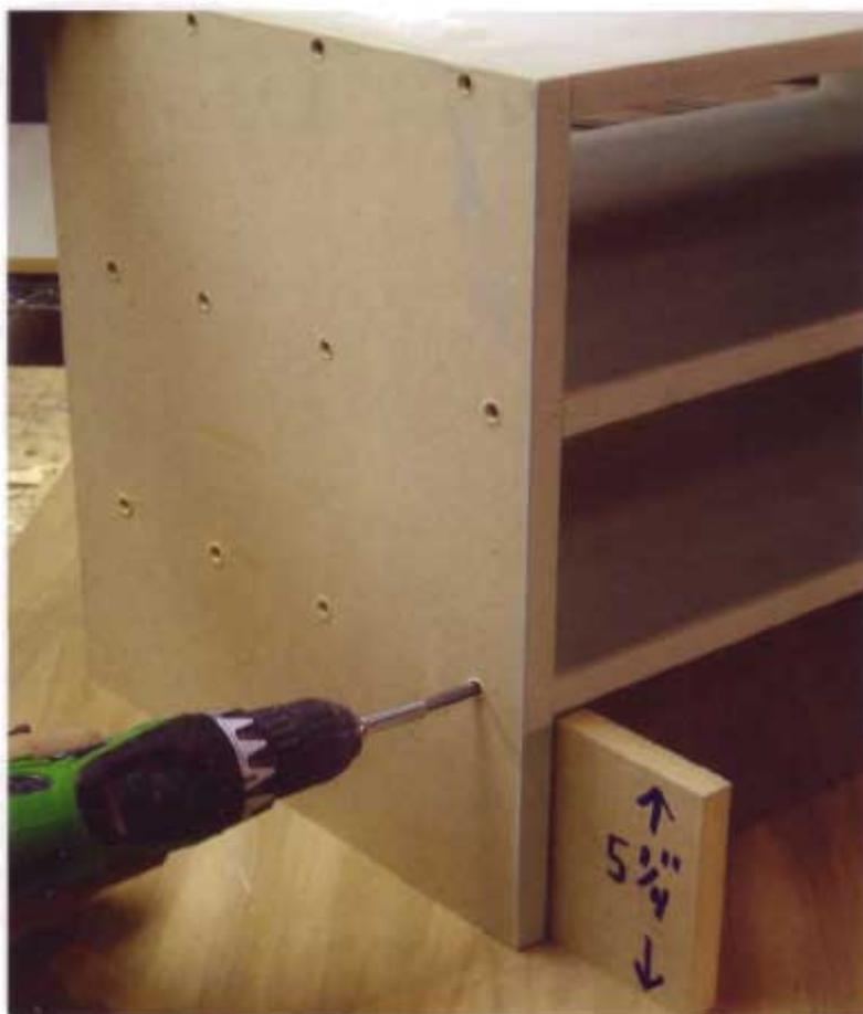
**9** Painting the parts of the shoe cubbies prior to assembly is a must—the tight corners and small spaces are really tough to finish otherwise. When the paint was dry, I used a  $5\frac{1}{4}$ " (133mm) spacer to align the shelves consistently. After the assembly is complete, sand the joints and touch them up as needed.
