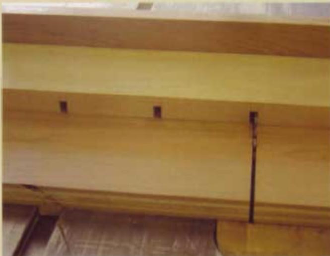
4 Using a miter gauge or a table-saw sled, I cut a series of dados across the piece of wood. The dados should be spaced equidistant from one another and should be as wide as the finished dividers will be [about 1/4" (6mm) wide].
