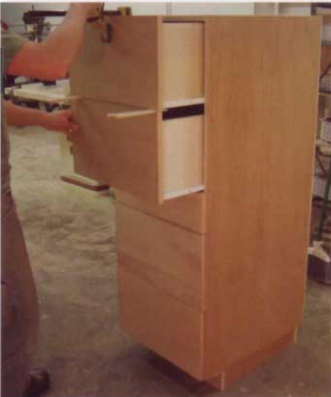
**12** The cabinet top won't allow enough room to get a clamp in place for the top drawer front, so you'll have to pull it out along with the drawer below it. Work carefully and you shouldn't have a problem keeping the parts aligned.
