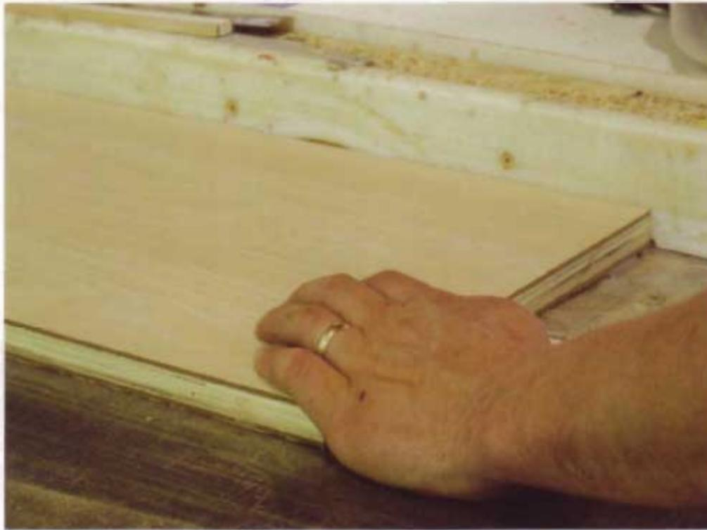
2 The sides, top and bottom are all grooved to hold the 1/4" (6mm) oak plywood back. I used a router table and a straight-cutting bit.
