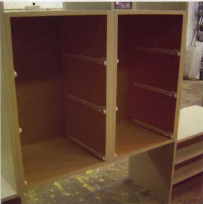
**13** I used three-quarter extension drawer slides for this project. Install the cabinet-side slides in the cabinets first.
