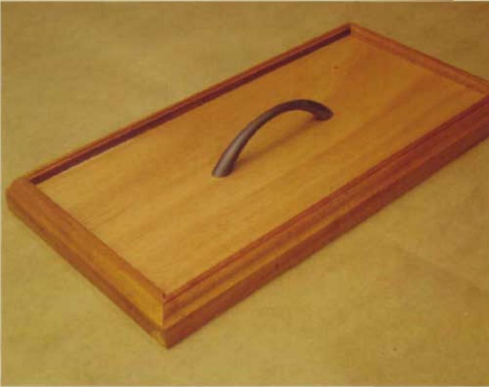
4 Miter joints allow the profile to wrap seamlessly around the panels.
