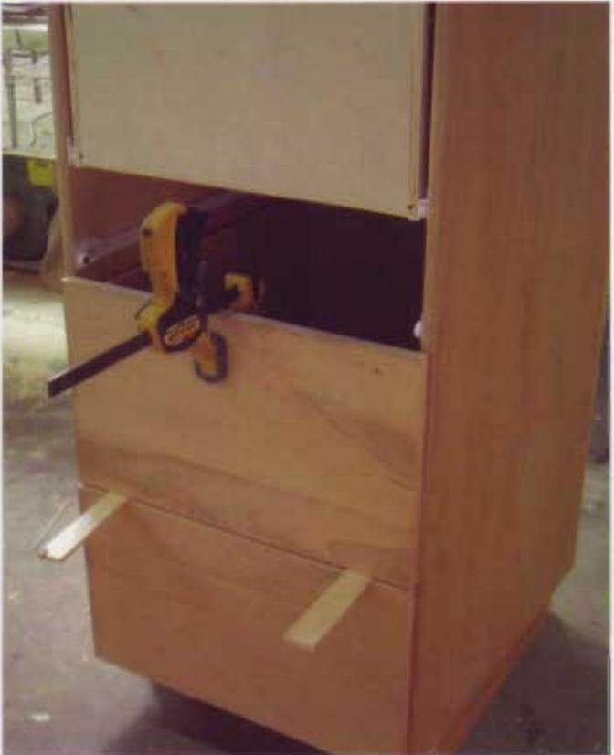
**11** The remaining drawer fronts can be positioned using shims to create an  $\frac{1}{8}$ " (3mm) gap between the drawers. Note that all of the drawer fronts can be repositioned during the final installation if necessary.
