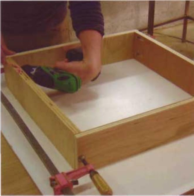
4 I built the base for the tall drawer cabinet from scrap plywood. Only the front piece had to be cherry. The grain orientation didn't matter on the other three sides, either.
