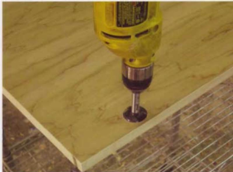
**10** The doors are made from  $\frac{3}{4}$ " (19mm) plywood that has been edge-banded on all four sides. The holes for the European-style hinges are located 4" (102mm) from the top/bottom edge of the doors, and  $\frac{15}{16}$ " (24mm) from the side.
