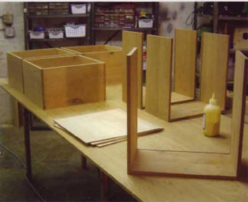
**12** These fairly simple drawers are built with  $\frac{1}{2}$ " (13mm) material that's glued and nailed at the corners. The bottoms fit into a groove I ripped near the bottom edge of the drawer stock.
