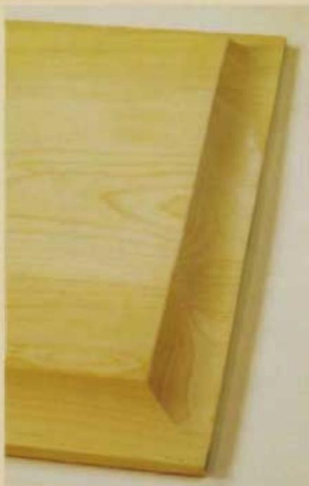
**9** If you'd like to make a true raised-panel door, the same process applies. Instead of the plywood center panel, though, you'll need to glue up a solid wood panel about  $\frac{5}{8}$ " (16mm) thick. Once it has been squared up and sanded, you can run it across your router table equipped with a panel raising bit.
