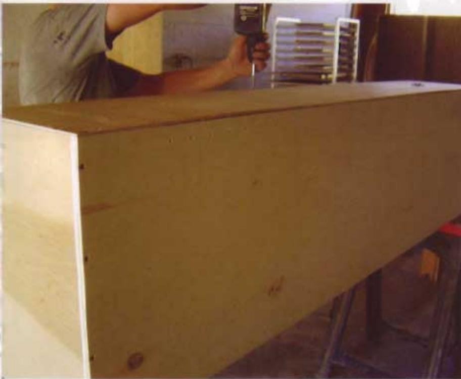
4 The  $\frac{1}{4}$ " (6mm) plywood back is attached with screws and glue.
