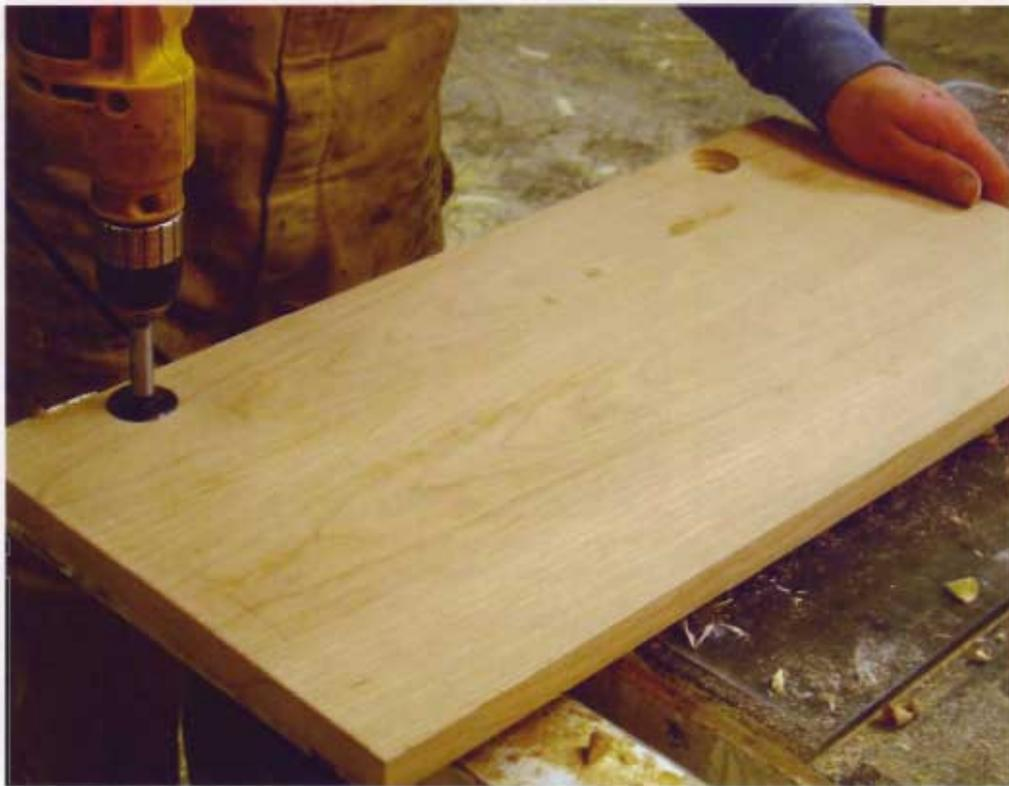
**7** I made the doors from some scrap cherry plywood. (You can use the species of wood you desire.) Use a  $1\frac{3}{8}$ " (35mm) Forstner bit to drill the hinge holes 4" (102mm) from the top and bottom edges of the doors, and  $1\frac{3}{16}$ " (21mm) in from the edges.
