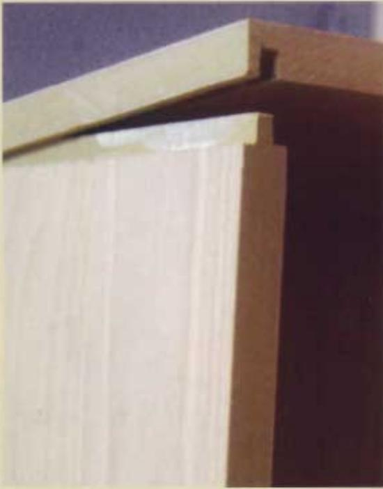
When done properly, the tongue fits into the dado without force. I lock it into place using wood glue.
