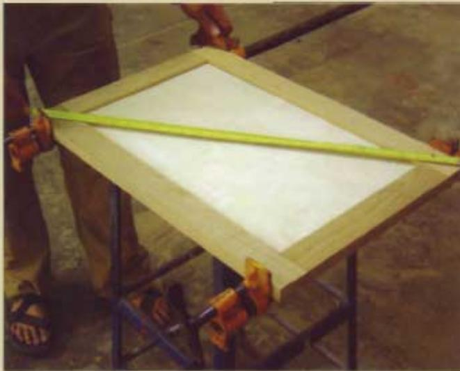
6 You'll need to measure the diagonals to make sure the door is square. The diagonals need to be exact. If they're out of square, I place a clamp across the diagonal that is too large and give it a gentle squeeze. It should slide right into place.
