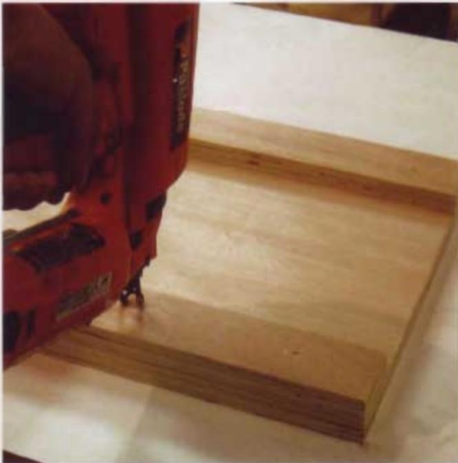
**7** This countertop begins with a 48" x 12" (1219mm x 305mm) blank. I built up the edges with 3/4"-thick (19mm) strips of plywood to give it a more substantial look.
