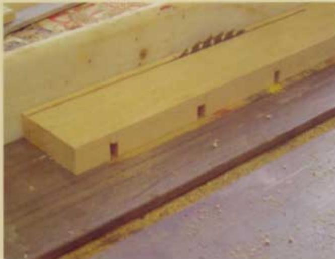
5 The depth of the dados should equal half the height of the block of wood. Once the notches are done, you can put a regular blade back on the table saw and rip the block of wood into 1/4" (6mm) strips.
