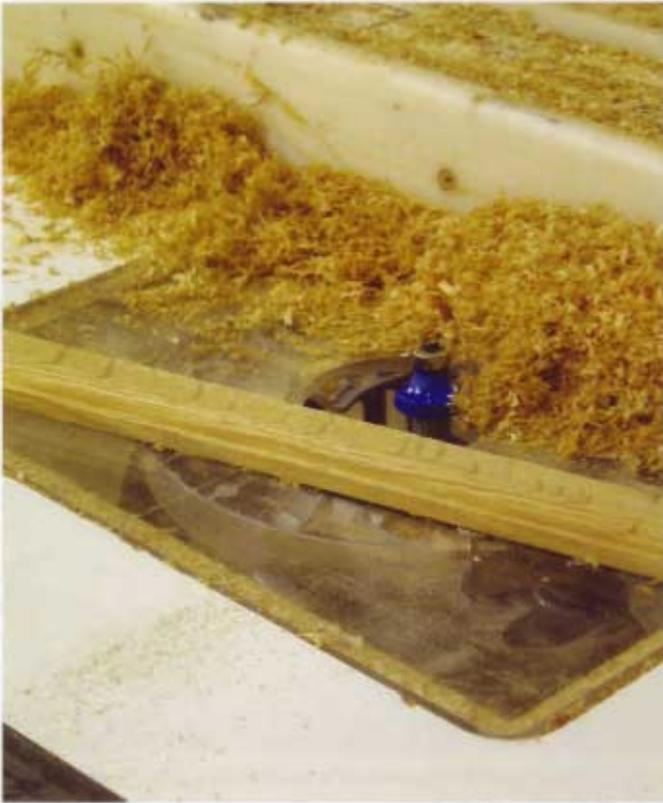
**9** I made a matched pair of edged-panel drawer fronts for this piece. I created the molding profile with a  $\frac{1}{4}$ " (6mm) roundover bit. The bottom edge of the cutter was raised to  $1\frac{1}{16}$ " (27mm) below the top of the router table. For more details on this construction method, see *Beyond the Basic Box*.
