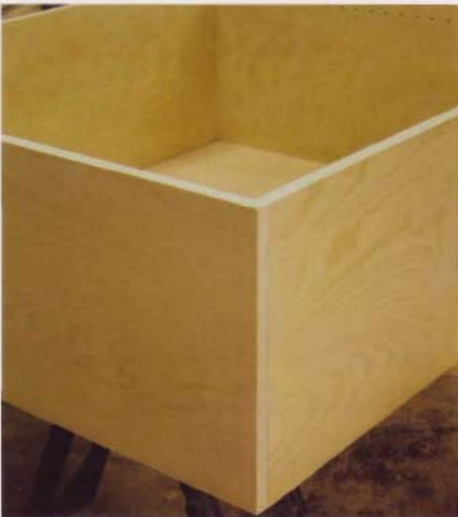
**7** Instead of nailing or screwing on the back, you can cut a dado into the cabinet parts for the back to nestle into. This takes a little more time but creates a very professional look. Note that the bottom edges of the side panels are visible on cabinet H, so be sure to edge-band them as well.
