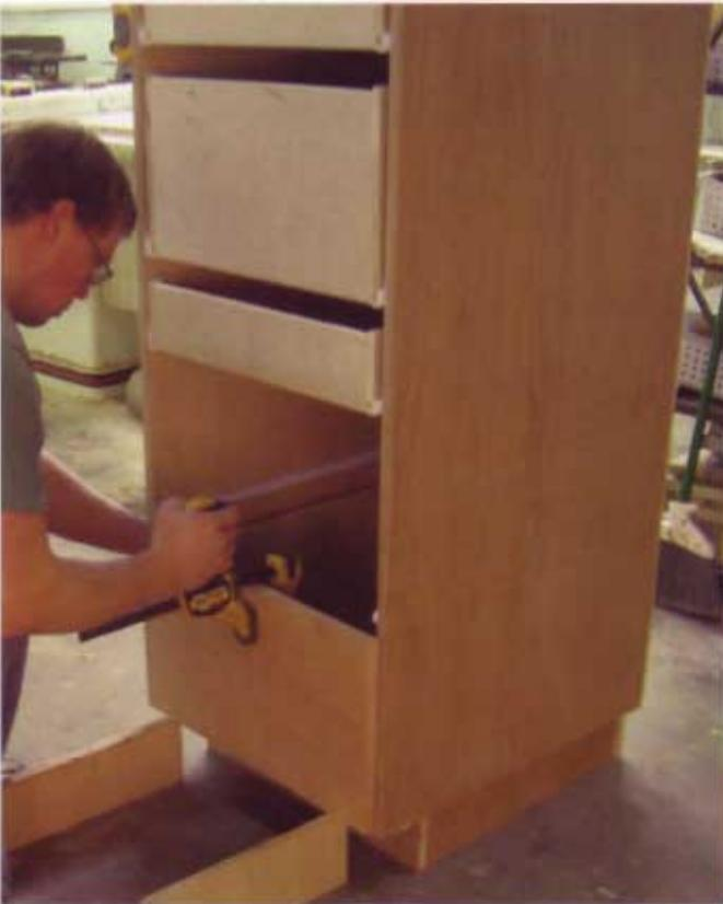
**10** These drawer fronts are simple to make, but a bit tricky to attach. Starting with the tall drawer cabinet, you'll need a pair of  $4\frac{1}{2}$ " wide (114mm) shims, which will hold the bottom drawer front at the correct height. By removing the second drawer, I had enough space to get a quick clamp in place to hold the drawer front onto the drawer. I secured it from the inside with two 1" (25mm) screws.
