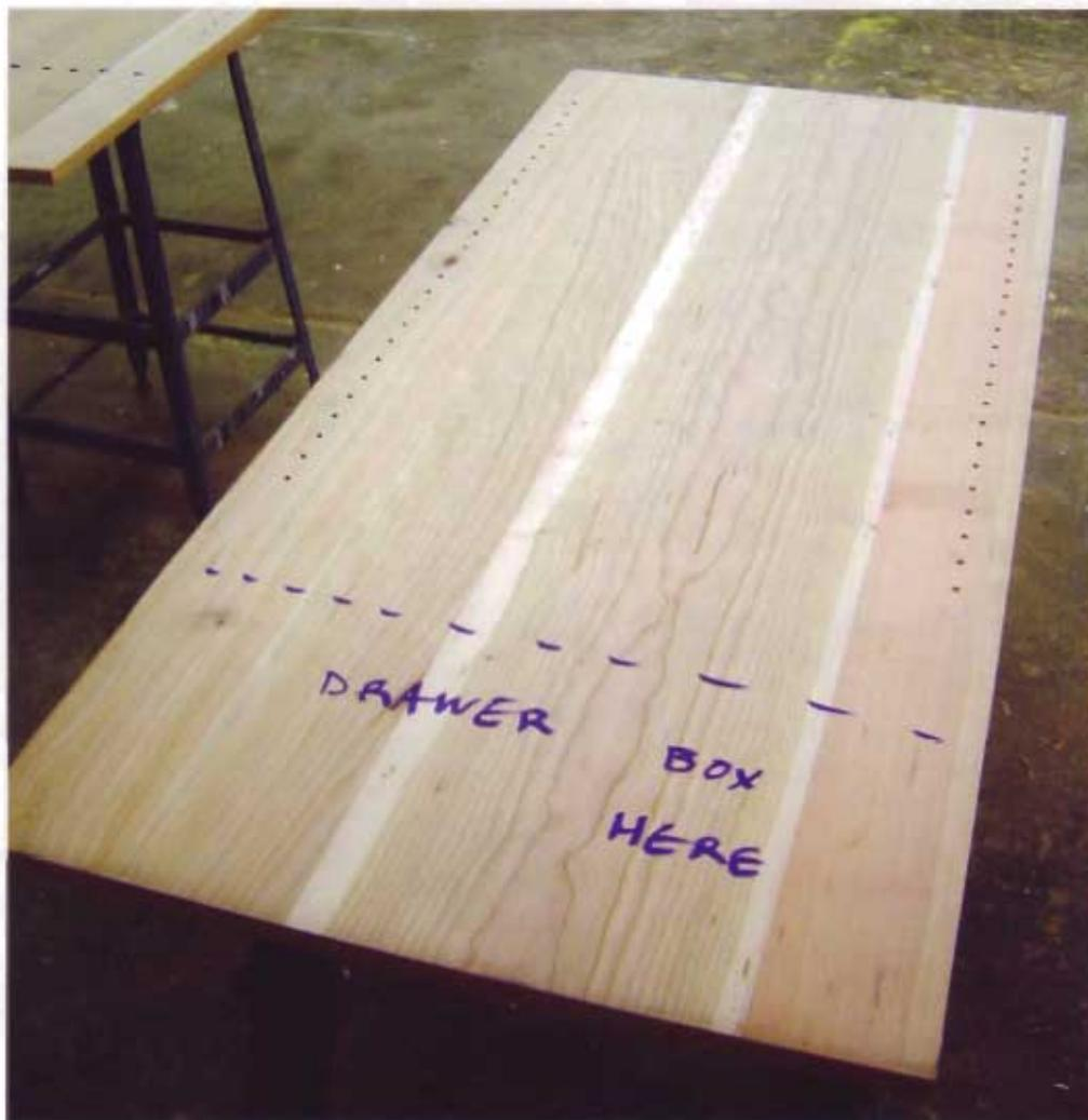
**3** When drilling the holes for the shelf pegs, lay out the end panels in matched pairs. (I suggest labeling the back edges of the panels with a marker.) This is easy to do, and failing to do so can wreak havoc later on.
