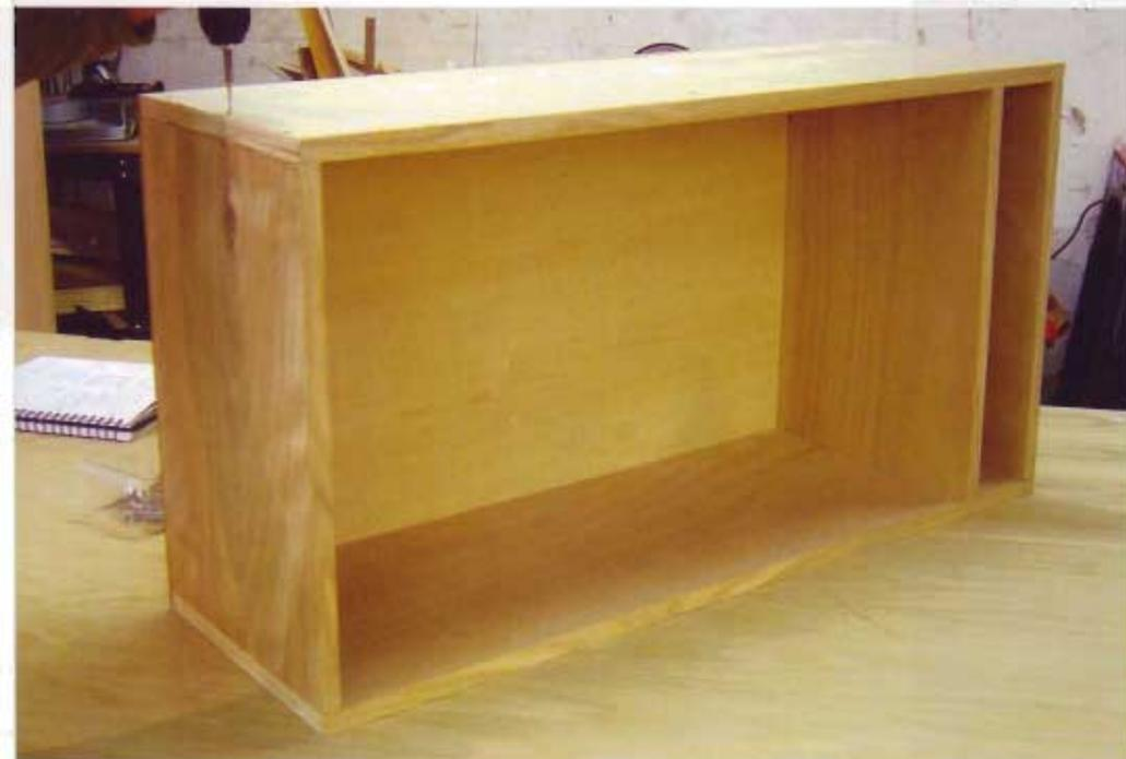
**12** The upper cabinets come together with butt joints held together with glue and screws. The backs are glued and nailed on.
