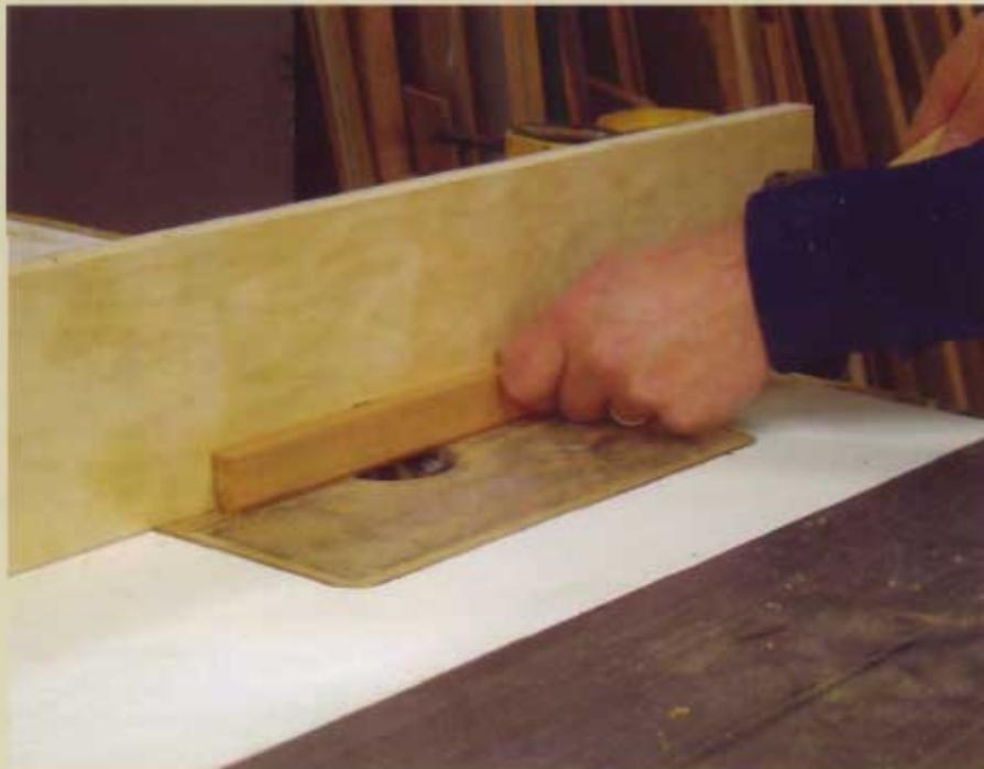
1 For most applications, I use moldings that measure around 1" x 1/2" (25mm x 13mm), but you may want to experiment with different sizes and see what looks best. I use a sacrificial fence clamped to my router table's fence so that the bit is only partially exposed. This allows me to expose only as much of the bit as I need. I suggest cutting most profiles in several passes. It's safer and usually provides a neater, crisper profile.
