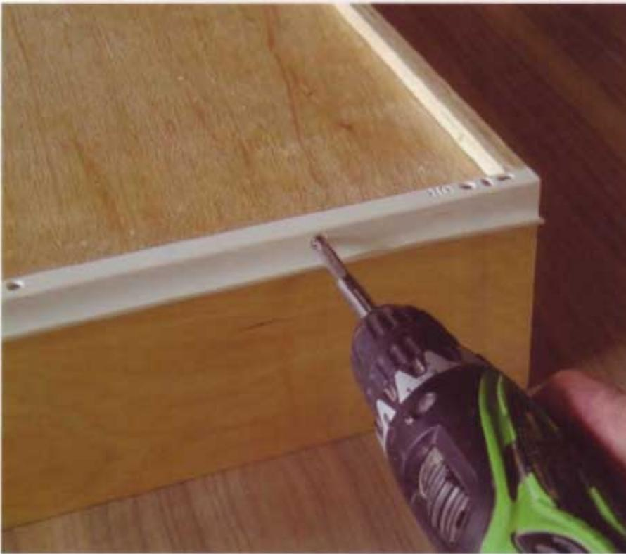
**9** As long as you've positioned the cabinet side runners correctly, the drawers should be a cinch to install. With the drawer placed upside down on a workbench, the drawer rails can be placed on the bottom of the drawer and screwed on. The front edge of the rail should be flush with the front edge of the drawer.
