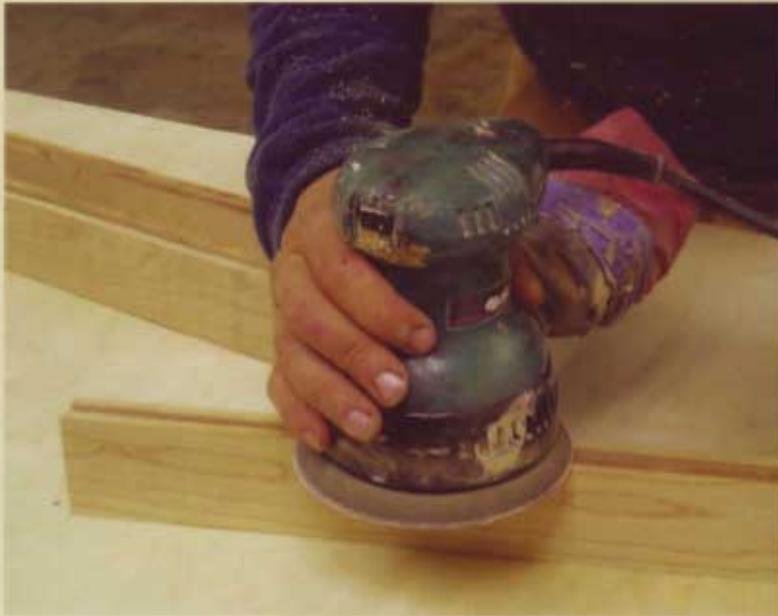
4 Prior to assembly, I recommend making sure the inside faces of the stiles and rails have been sanded smooth. Once the door is assembled it is very difficult to sand these areas.
