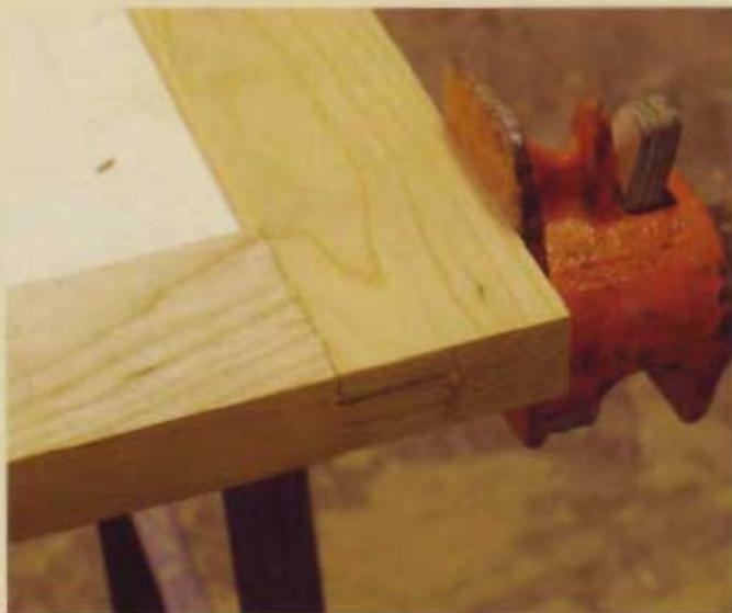
**7** Once the glue has cured, you can sand the face of the door frame and its edges. I don't sand the panel once it has been enclosed in the frame, as it is harder to sand evenly. Depending on the overall style and look you're going for, you can rout the outside edges of the door on a router table or with a hand-held router.
