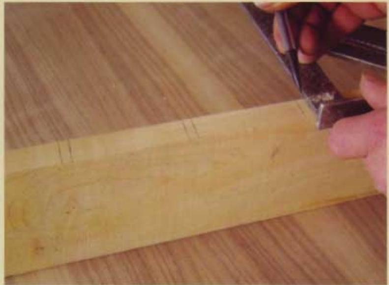
**3** To make the dividers, I start with a 1"-thick (25mm) piece of hardwood lumber. For an 18"-wide (457mm) drawer, I would ideally start with a piece that measures 24" × 6" (610mm × 152mm).
