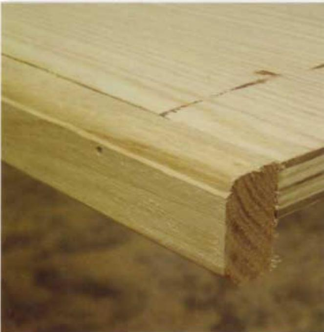
**11** Attach a hardwood strip to the front edge of the upper shelf. It will keep the shelf from sagging over time. I used the same router bit to profile the hardwood strip as I did for the drawer fronts. Doing so provides for nice continuity between components.
