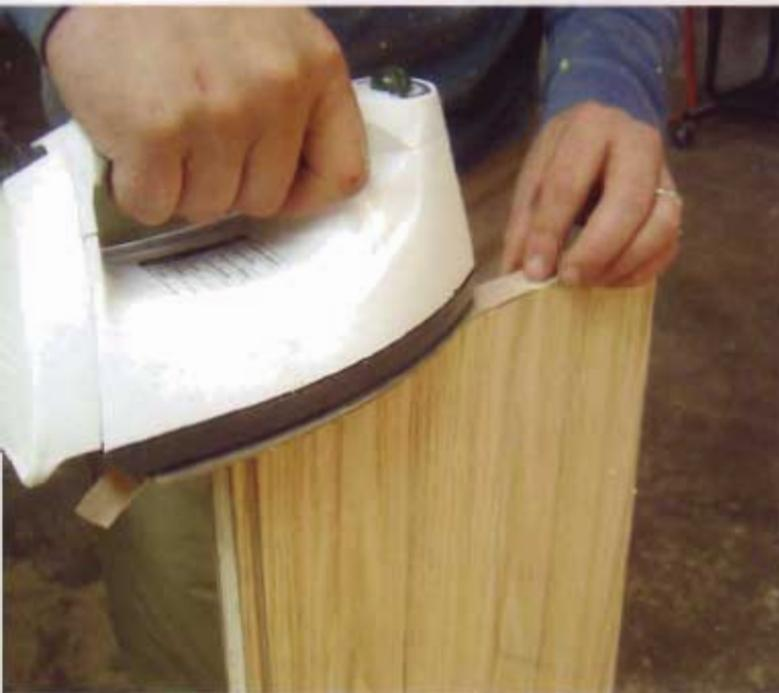
3 Once the groove has been cut, edge-band the parts. This sequence is important because the edge-banding covers up the groove that shows through on the ends of the plywood.
