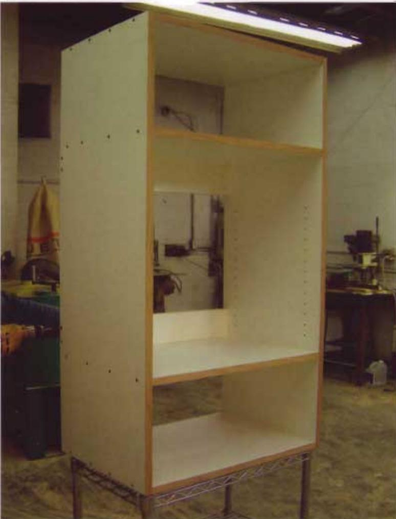
**6** The back wall stretchers provide a place to screw the cabinet into the studs in the wall. I placed them inside the portion of cabinet that will be hidden by the doors. Doing so makes for a less cluttered look when the cabinet is installed.
