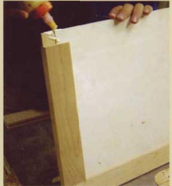
5 After test-fitting the parts, you can glue up the door. Make sure to wipe any glue squeeze-out from the corners immediately, as glue that has had a chance to set up in the nooks and crannies will be very hard to remove.
