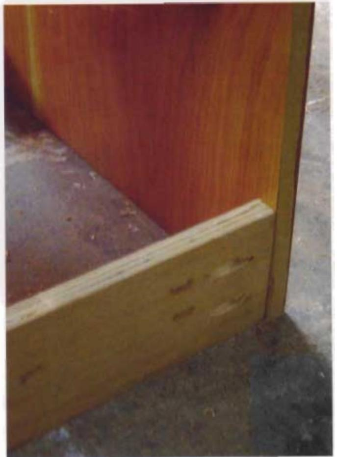
**15** Two of the stretchers are positioned at the bottom of the unit, one at the front and one at the back, where they form a base for the bottom shelf. Place the pocket holes for the screws on the back side of the stretchers where they'll be out of sight.
