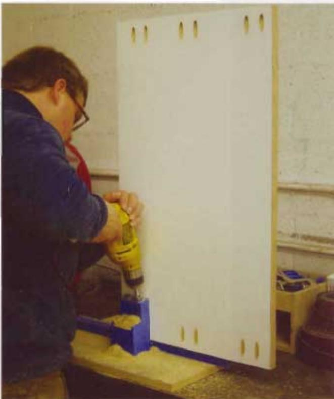
**11** I used pocket screws to hold the bottom in place. I chose pocket screws because I wanted the exposed screw heads on the bottom right side of the piece to be concealed. Fastcap self-stick screw head covers would've helped, but pocket screws are equally quick and look even better.
