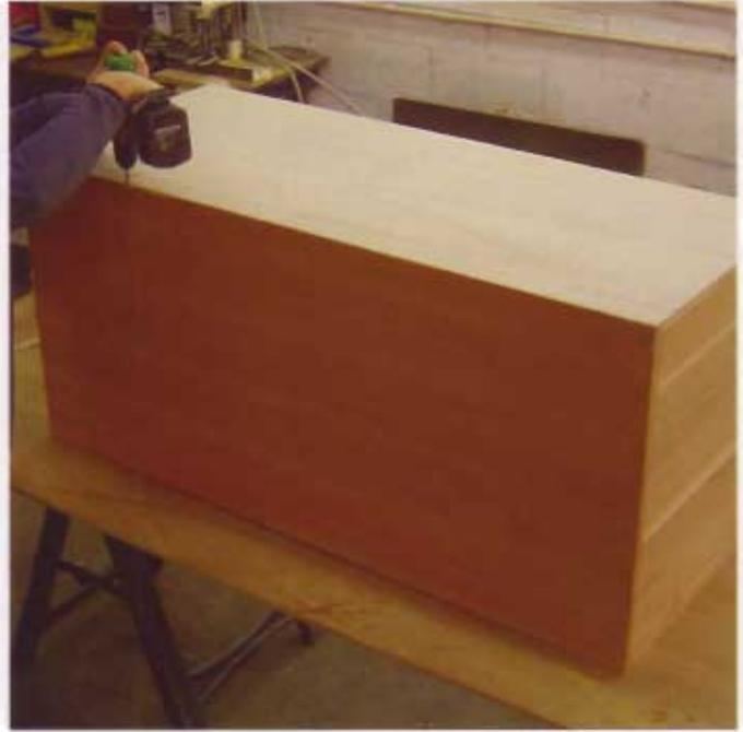
5 The tall drawer cabinet is straightforward: It is a four-sided box with the back screwed on.
