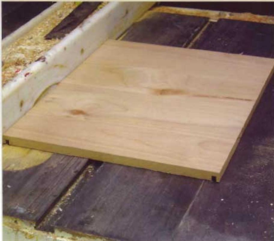
2 I cut a dado into each side panel near the ends, where the front and back panels will attach.
