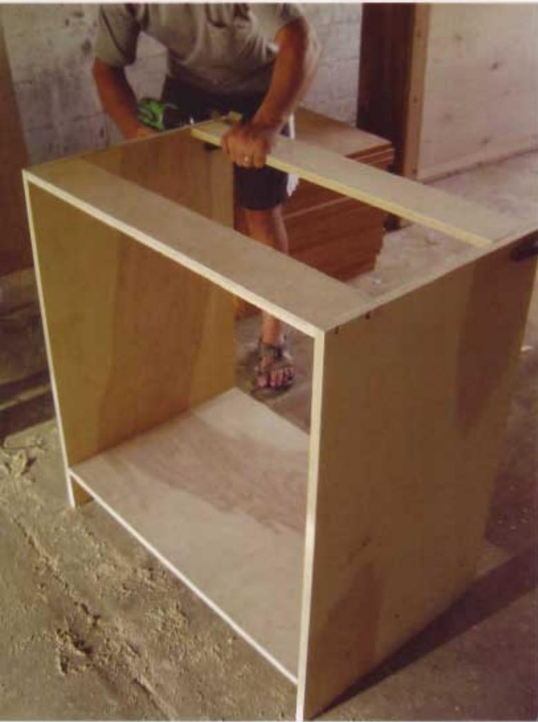
**6** The two top slats are attached in the same manner as the bottom, except they are positioned flush with the top of the cabinet sides.
