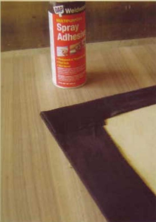
**2** This false bottom is then dropped into the drawer—note that you must size it  $\frac{1}{8}$ " (3mm) smaller than the drawer's interior.
