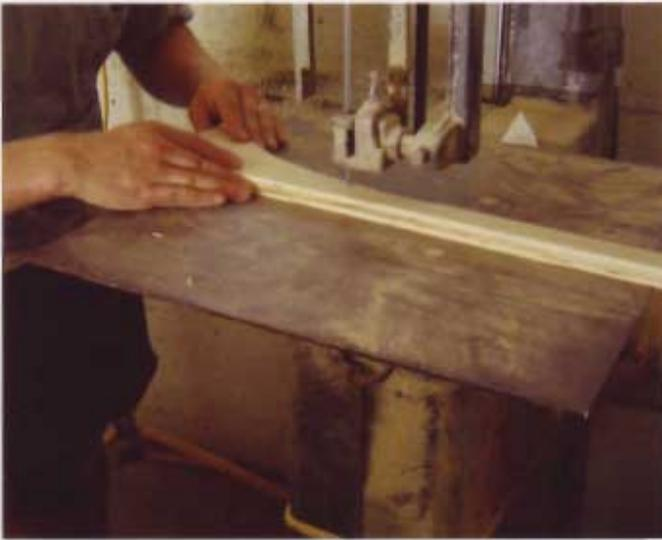
**8** For the toe kick, cut out a rectangle that will fit precisely into the recess at the bottom of the cabinet. I decided to add a decorative cut to create some visual appeal.
