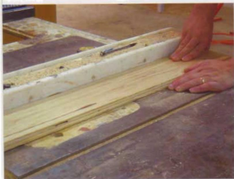
**14** The tower is composed of two end panels connected with stretchers. The stretchers are ripped from  $\frac{3}{4}$ " (19mm) cherry plywood and edge-banded on their long edges.
