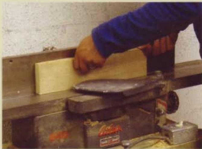
**1** Once you have an accurate measurement for the finished door, you can start to make a list of the parts you'll need. A frame and panel door is usually comprised of five parts: a center panel, generally  $\frac{1}{4}$ " (6mm) thick, and a solid wood frame, which consists of two vertical stiles and two horizontal rails. I usually mill an extra frame part or two because it doesn't take much extra time, and it will be well worth it if you make a mistake later on and need a replacement.
