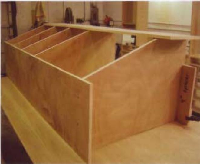
**1** Begin with the corner units. You'll notice that they are not symmetrical. This is because the units on the long wall are 12" (305mm) deep, but the units on the short walls where the clothes rods go are 16" (406mm) deep to accommodate hanging garments. This doesn't pose any problems in construction but it is an important aspect of the design. The shelves are fixed into place with screws. Note: It is a lot easier to edge-band the shelves before assembling the corner units.
