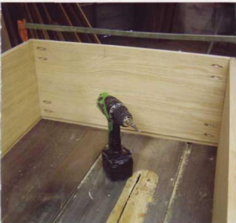
5 The top gets sandwiched between the sides. Locate the pocket holes on the bottom side where they are out of sight.
