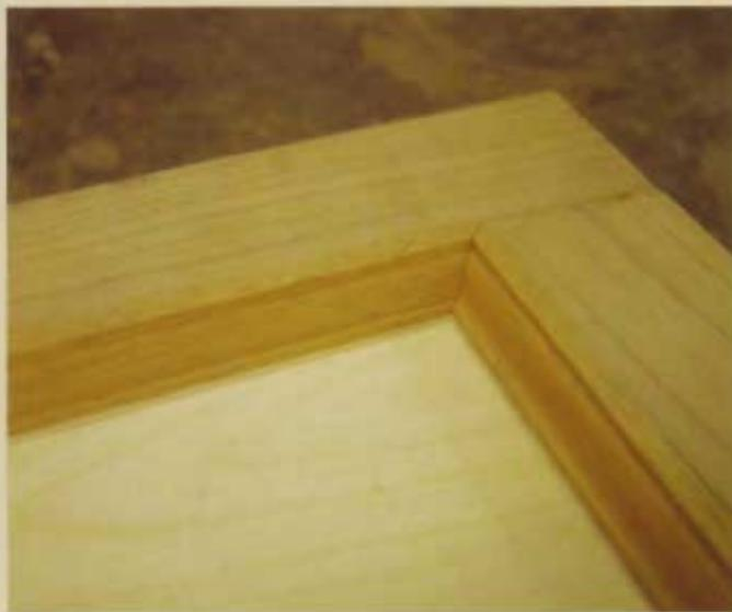
**8** To add another interesting detail, you can make a small molding on your router table and apply it to the edge of the panel where it meets the stiles and rails.
