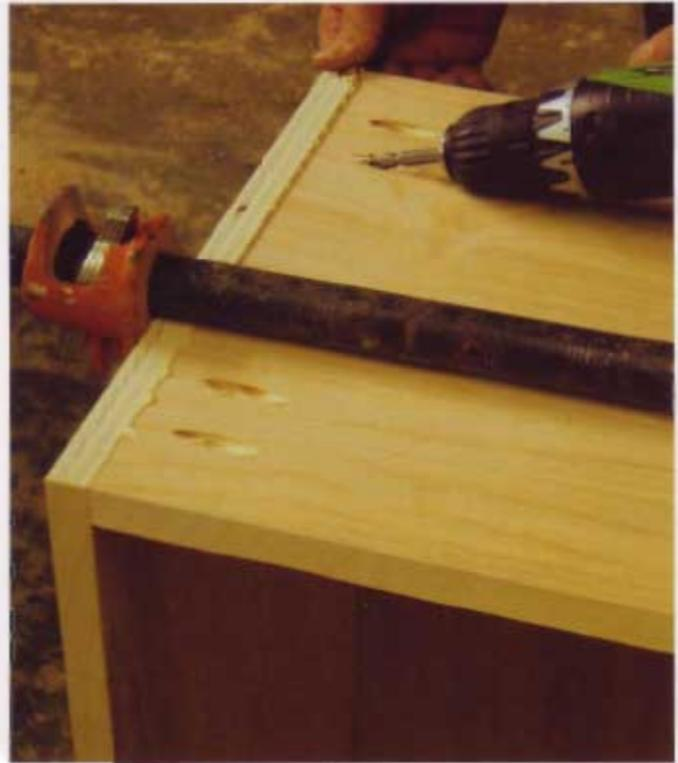
**6** Cabinets A, D, G and H all have at least one side exposed, so I chose a more refined method of construction for them. On the exposed areas, I used pocket screws instead of through screws. I suggest immediately wiping away glue squeeze-out with a damp paper towel.
