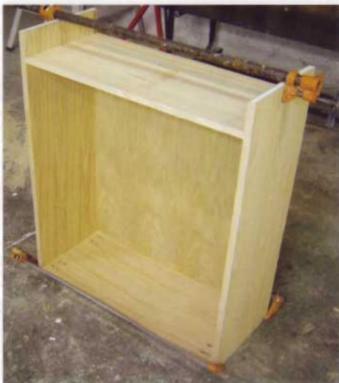
7 The bottom is sandwiched between the sides, just like the top. To position it correctly, measure down 3" (76mm) from the bottom edge of the sides and make a couple of small marks in pencil.
