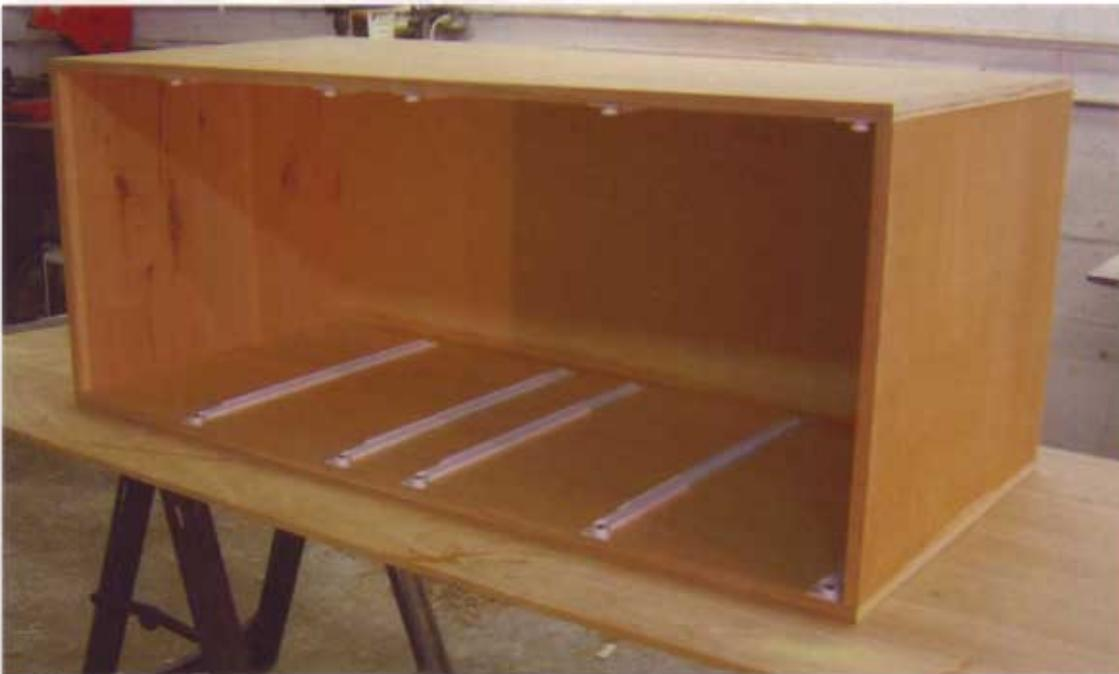
6 The drawer slides separate into two halves: the cabinet side runner and the drawer rail. In addition, the parts are assigned to either the right or left side of the drawer. The cabinet side runners screw directly onto the inside face of the cabinet sides. To locate the positions of the cabinet side runners, refer to the drawing on page 31.
