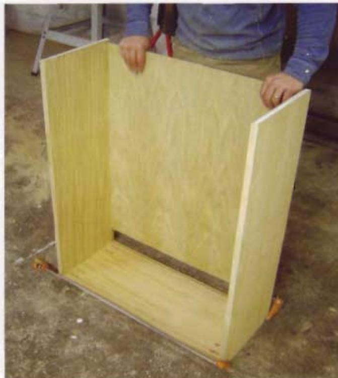
6 The back should slide in easily without excess force. Test-fit prior to applying the glue.
