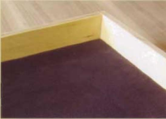
**1** A jewelry drawer starts out like any regular drawer, built in the usual manner. The velvet bottom is made by wrapping a  $\frac{1}{4}$ "-thick (6mm) piece of plywood with velvet. I use a spray adhesive on the underside of the false bottom to secure the velvet.
