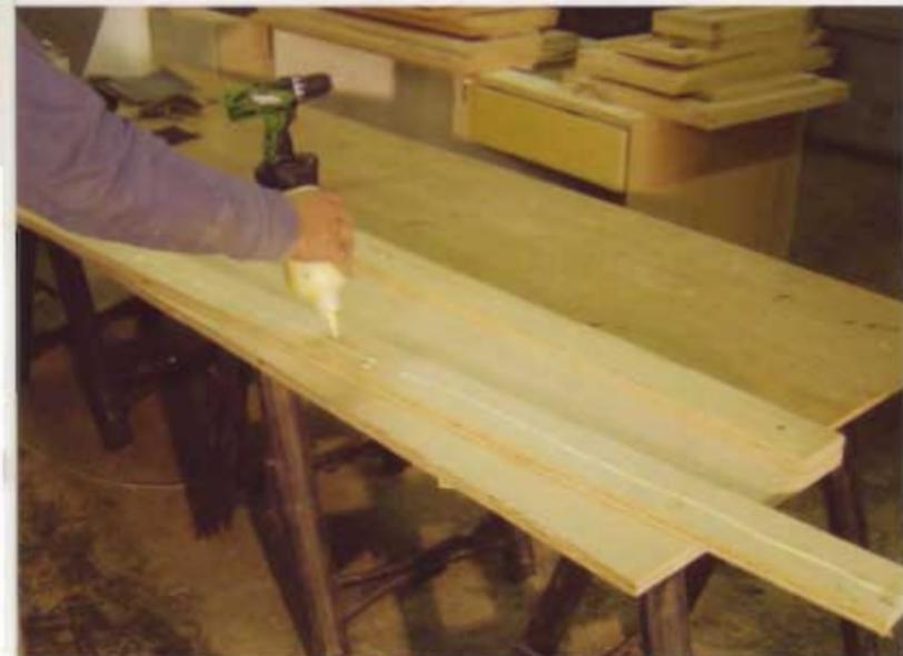
**9** The countertops consist of  $\frac{3}{4}$ " (19mm) plywood that is doubled-up at its edges. Glue and screw down the 4"-wide (102mm) strips for maximum stiffness and durability. The exposed edges can be edge-banded with 2"-wide (51mm) banding when the glue has dried.
