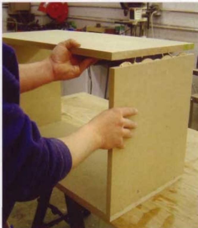
**5** After a test-fit to make sure the slots are properly aligned, I glued up the assemblies and applied even clamping pressure. The test-fit may seem like a waste of time, but it's not. If you discover a discrepancy in the fit, you'll save a lot of time, stress and mess if you catch it before there's glue all over the place.
