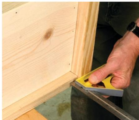
The edge of the lid is in from the edge of the bench. Set the combination square to the right distance, hold it against the back edge of the side, and push the back edge of the top in place.
