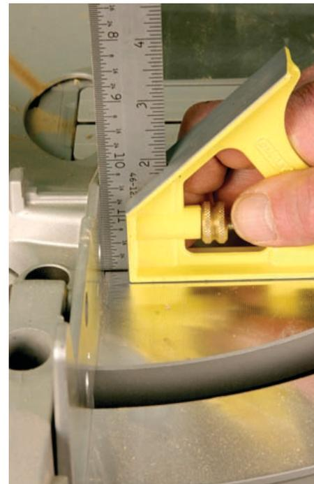
A less-common problem is that the fence isn't square to the table. Check this along several points on the fence. A twisted fence will wreak havoc with your accuracy.
