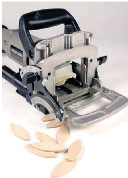
Biscuit joiners cut a football-shaped recess in two parts to be joined. The biscuits fit into that recess and (with a little glue) hold the joint together.
