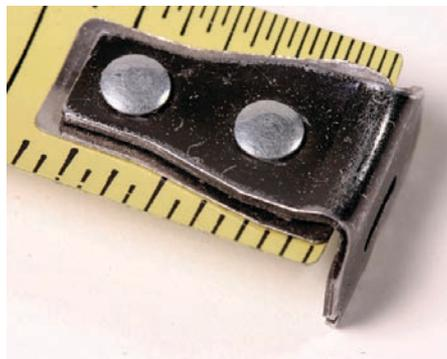
The hook should move in and out. The distance it moves should be equal to the thickness of the hook itself. Tweak the hook with pliers until the tape consistently measures inside and outside measurements.
