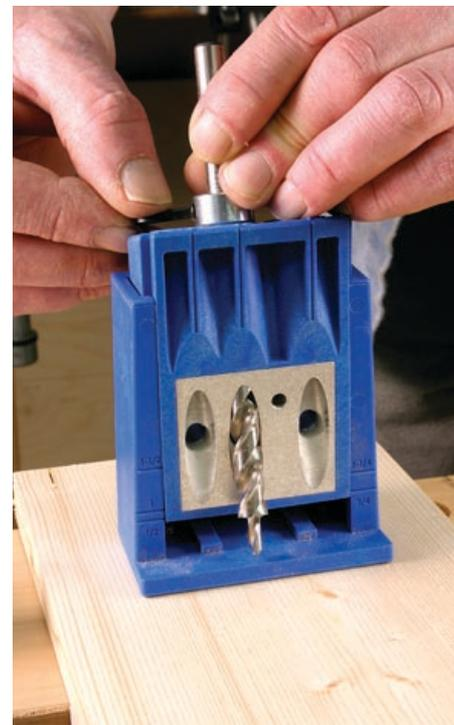
Setting the depth of the stop collar is simple. With one hand, you can push the collar down on the jig and hold the tip of the bit about  $\frac{1}{8}$ " above the jig. Use your other hand to tighten the set screw on the collar.
