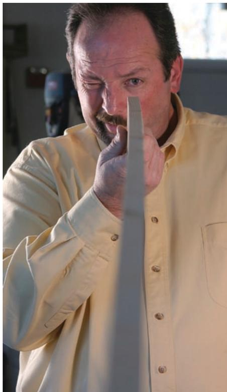
Looking down the edge of any board will help to uncover any defects in the lumber such as twisting, warping or crowning.
