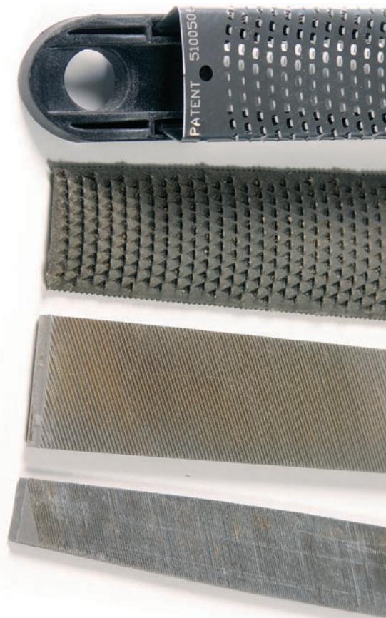
of their coarseness. Bastard cut is the coarser one; smooth cut is the finer one. Because we're going to do most of the work with a jigsaw before turning to a rasp, I recommend you try to get a smooth cut rasp. Look for one that has one flat face and one face that curves out. Sometimes this is labeled as a half-round profile. This will allow you to shape inside curves.
