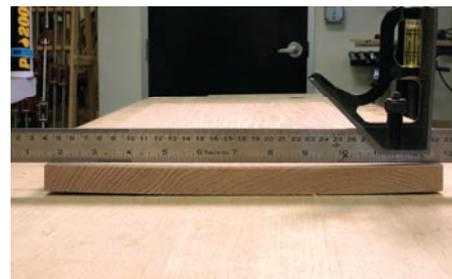
The use of the straightedge portion of the combination square will help to identify any cupping in the board. Return these boards to the stack and select another!
