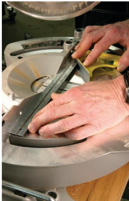
The fences on these saws can be bent during assembly. When you get your saw out of the box, check the fence with your square to ensure it's straight. If it's not, take the saw back and exchange it. A bent fence is almost impossible to fix and will cause a lifetime of headaches.
