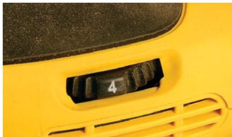
Generally, the variable-speed feature is unnecessary on a random-orbit sander. The only time I've slowed down the tool is when I was dealing with some really thin veneer. That's it.
