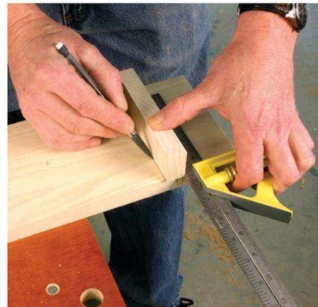
Measuring isn't always the best way to work accurately. Holding a block of scrap against the blade of the square guarantees that the line drawn will represent the thickness of the piece that will fit in the notch. It's much more important that the slot and the shelf be identical in size than it is to know the exact thickness of the shelf. Every time you measure and mark something you introduce the opportunity to make a mistake. I consider measuring to be a last resort, and avoid it when I can.
