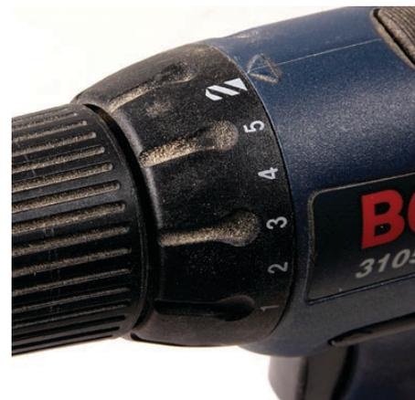
Setting the clutch as shown will disengage the clutch, allowing you to drill at full power and speed. This is in the drill's instruction booklet that you threw away.
