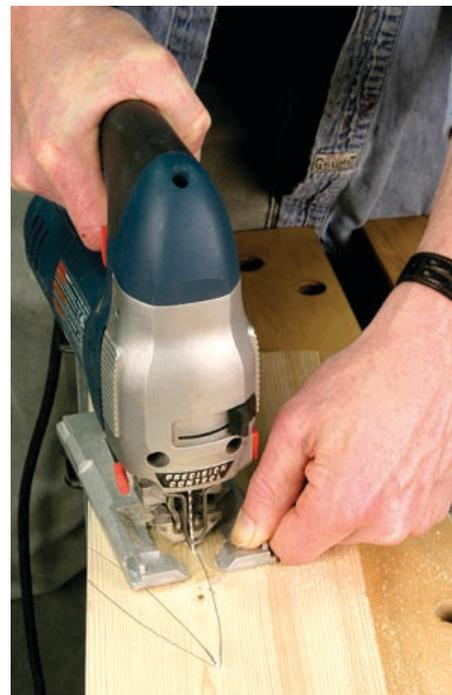
The jigsaw is a two-handed tool. A thumb on the baseplate will help steady the tool and will allow you great finesse as you round curves and track a line. We've removed the plastic guard on this saw (sorry, we shouldn't do that). With the guard in place, it's quite a feat to cut yourself.
