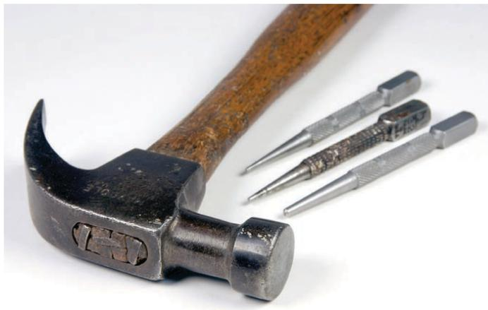
A good wooden-handled hammer and a few nail sets can serve you for a lifetime. Avoid the fiberglass and metal hammers. They are not as forgiving on your joints (as in your shoulder and elbow).
