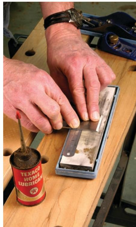
By propping up the back of the blade as you work the back, you'll greatly speed the polishing action of this critical surface. The ruler ensures that every time you do this it will be consistent.
