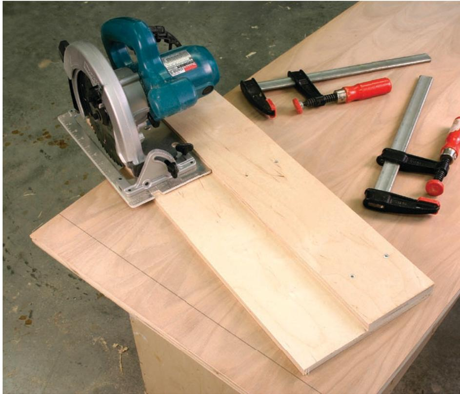
time you run the saw against that scrap, while the saw is resting on the plywood, the cut will be correct to your layout. One thing to remember is that you need to set the depth of cut to the material you are cutting and the thickness of the plywood. This will shorten the thickness of cut of the saw but you get accurate results each and every time. If you need the additional depth, resort to the hand-held cut methods described earlier in “Making the Cuts Freehand.”
