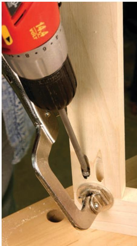
grain of the piece that the screws go in. As you practice, try varying the amount of glue that you use until you get just a small amount squeezing out when you drive the screws. Using more glue than necessary will only create a mess to clean up, and can lead to some big problems when finishing. If you're driving the screws with a cordless drill, use the lowest speed available and the long driver bit that comes with the kit.
