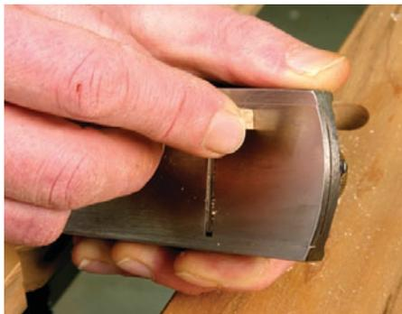
A small block of wood can check the setting of your plane's iron. If the block of wood has the same amount of drag all across the mouth, then your blade is centered in the mouth and is projecting squarely – get to work!
