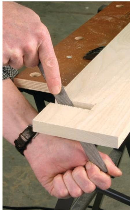
Using both hands helps to keep the rasp in a vertical position. Remove material evenly with long strokes of the rasp until you are down to the layout lines. Working to the lines will help you to keep the edges of the notches straight.
