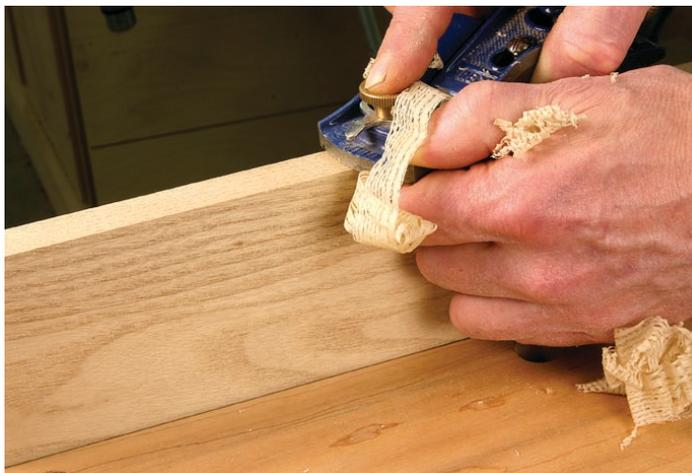
Note the grain on the face of the board. See how it is heading up toward the edge being planed? Think of those grain lines as fur. If the tool is pushing them down as it works, the chances are your cut will be sweet.
