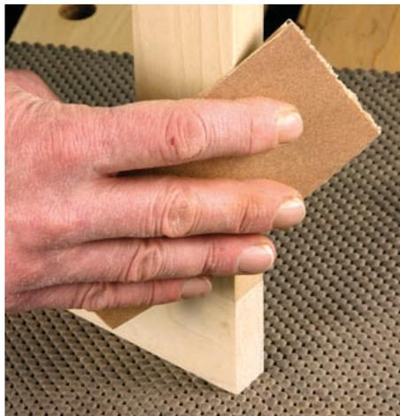
Always “break” the edges of your work before finishing. This makes your project nicer to the touch and makes your edges less susceptible to damage.
