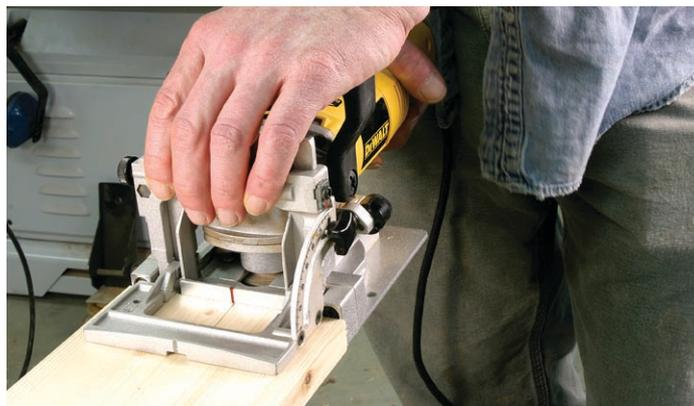
An alternate way to plunge: Squeeze the fence and tool handle together to make the cut.
