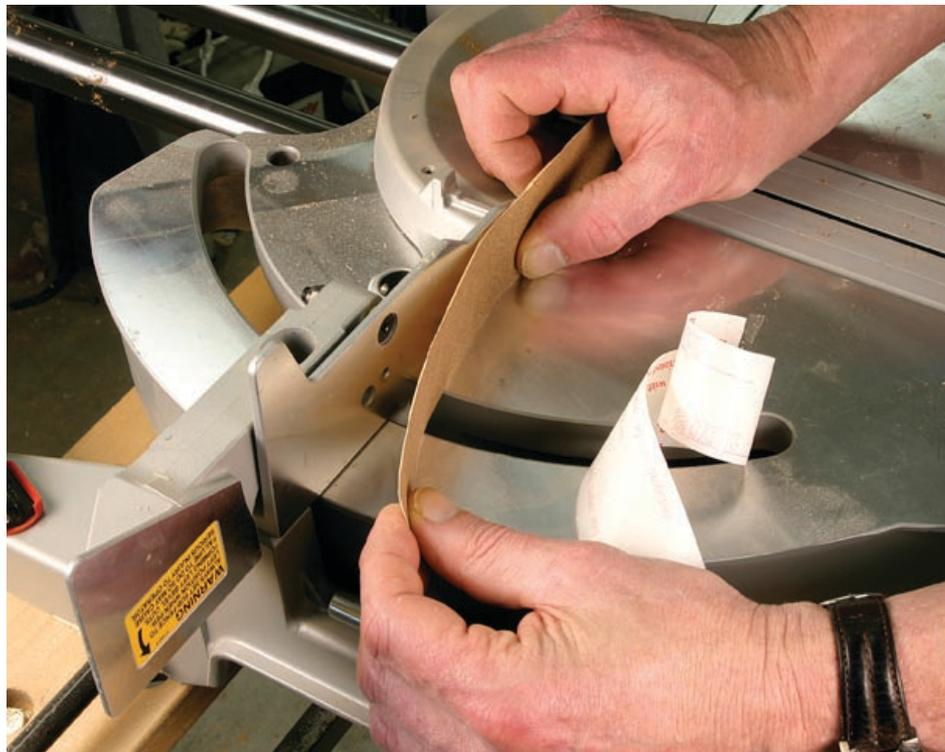
Personally, I don't understand why they make the table and fence so smooth and slippery. Their job is to support and grip the work. Even after using these tools for 13 years, I still struggle with keeping the work immobilized as I cut it. If it shifts even a tiny bit during the cut, your cut won't be square. Adding a bit of self-stick sandpaper to the fence works wonders.
