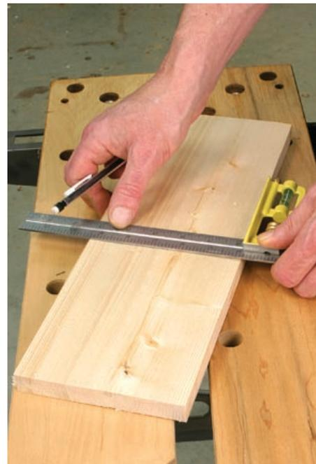
Now flip the square over and show the ruler to the line. If your square is true and your line consistent, then the line and the ruler should be perfectly parallel. If the line and the ruler don’t match up, try the operation again before you reject the square – it’s easy to trip yourself up when checking your square.
