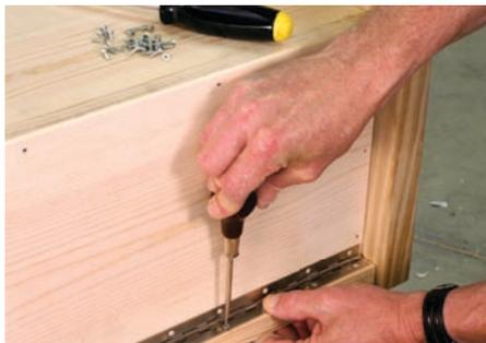
When installing a piano hinge, first install just a few of the screws. Then test the hinge.
