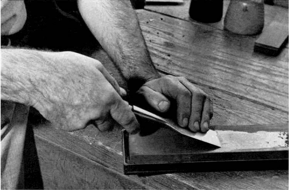
Plate 19. Sharpening a chisel.
