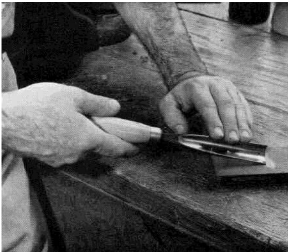
Plate 23. How to hold a gouge when sharpening.
