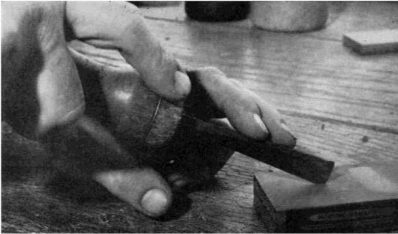
Plate 21. Proper angle at which V tool should be held to remove tip.
