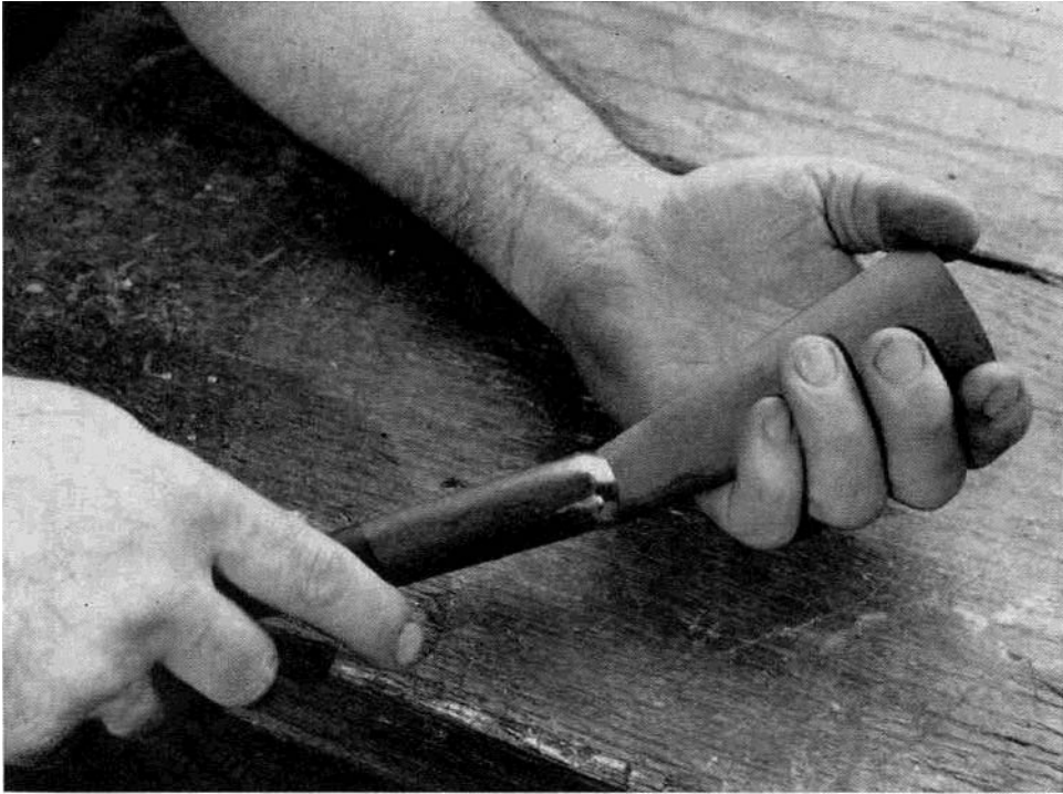
Plate 24. Removing burr from gouge with slip-stone.
