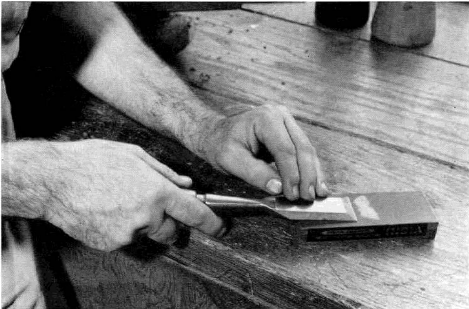
Plate 20. Removing the burr from sharpened chisel.
