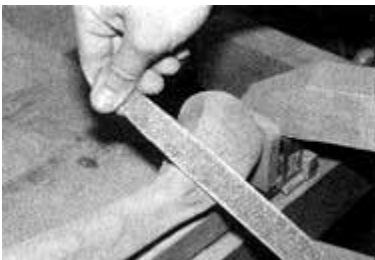
Fig. 11. Feather a flat on the top surface of the Foot.
