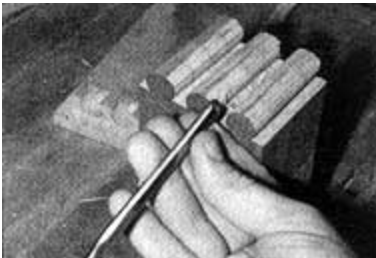
Fig. 18. Shave all the pins in the stack just to the line.
