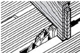
Fig. 4 Cutting the opening for Drop Leaf supports – 1/2 of the depth at a time.
