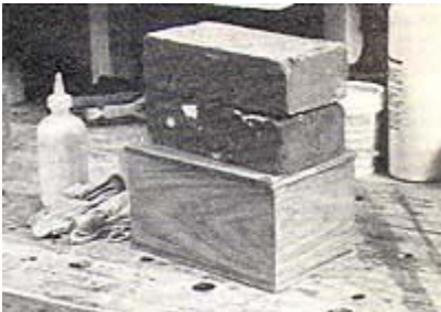
Fig. 4. Apply the top and bottom and place weights on top.
