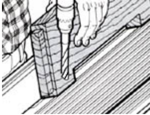
Fig. 5 Drilling screw pockets in sides. Drilled at 10° with a 1/2" brad point bit, to within 3/8" of the bottom. Use a 1/4" brad-point bit to make pilot hole for the #12 roundhead screws.
