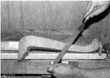
Fig. 10. Chamfer the stock between control lines.
