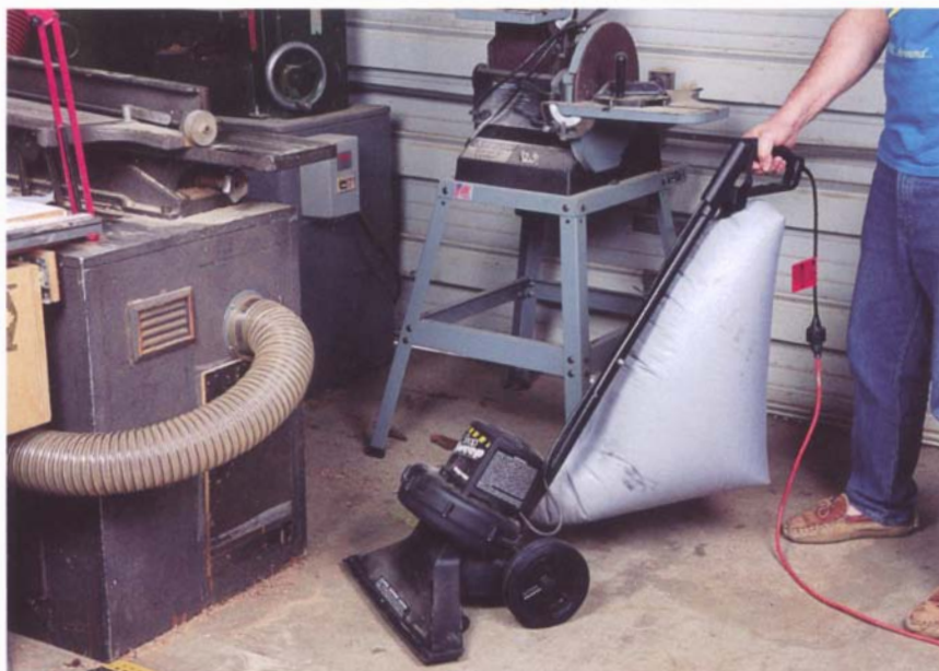
A specialized tool designed for cleaning up large shop floors, the Shop-Vac Shop Sweep uses a wide-mouth floor pickup and powerful blower to whisk chips and debris up and into a zippered fabric bag that's easy to empty.
