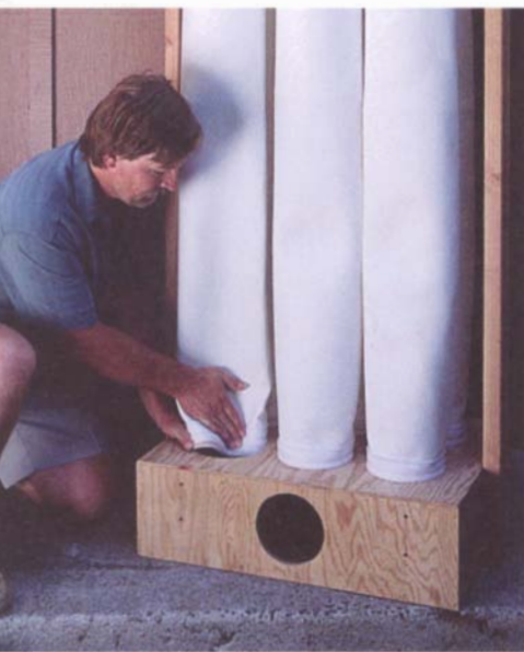
The small-diameter filter tubes that attach to a shaker box provide lots of surface area for clean air to escape through the filter fabric. The open end of each tube has a springy metal band inside, which locks into a hole to seal the bag to the plywood shaker box.
