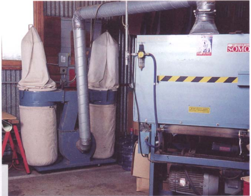
A central dust-collection system hooked up to all the machines in the woodshop conveys chips and sawdust to collection bags or canisters for convenient disposal.
