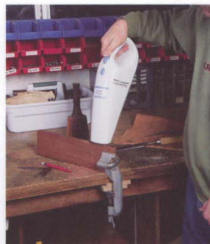
Cordless portables, such as the 7.2-volt Black & Decker Dustbuster, are great for benchtop cleanup chores or for removing waste from joints cut by hand, such as these mortises.
