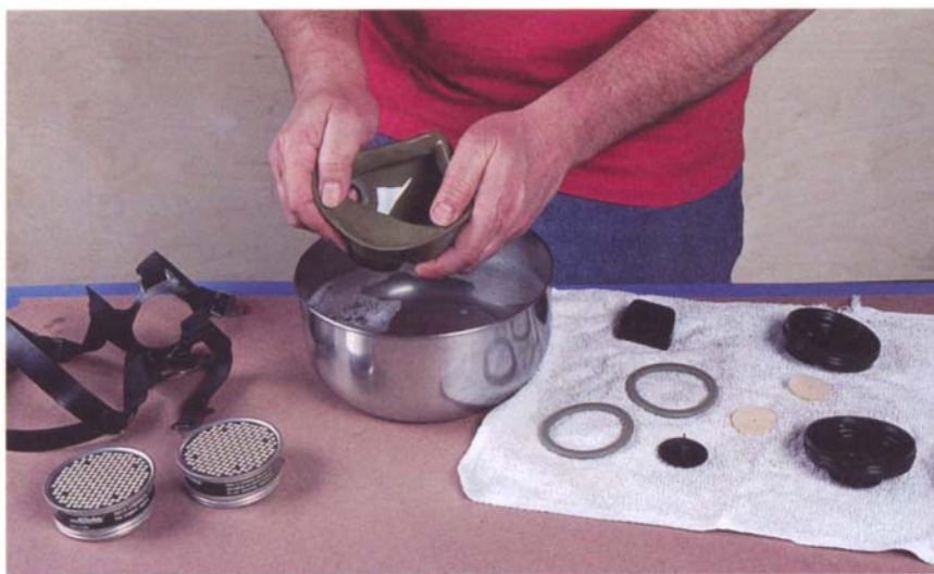
Washing a rubber or neoprene facepiece with a mild detergent between uses helps keep it sanitary, as well as ensuring that the valves work correctly and that the facepiece continues to seal effectively.
