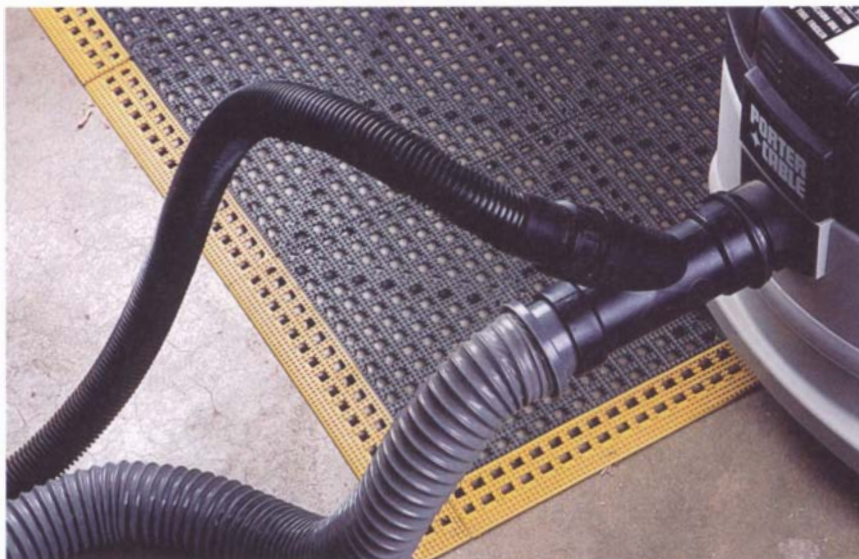
Fitting a wye connector, made from plastic pipe fittings, to the intake on a shop vacuum allows the connection of two hoses, so that both tools served remain ready to run with dust collection.
