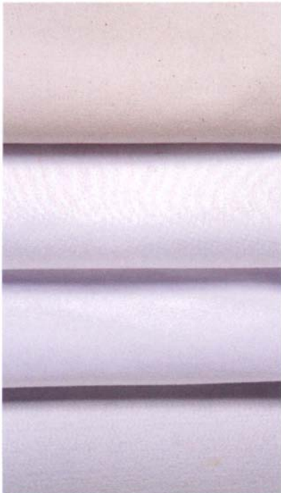
Not all filter fabrics are equally effective at straining respirable dust from the air. Here are four popular fabrics for dust filtration, arranged from worst to best filtration (from top to bottom): cotton sateen, woven Dacron®, knitted polyester, and felted polyester.
