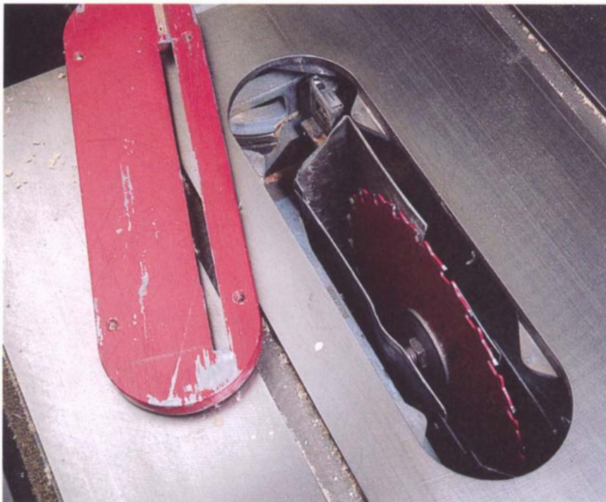
A shop-built sheet-metal hood fastened to a table saw's trunnion assembly provides effective dust capture on a contractor's-style saw that doesn't have an enclosed base. The hood tilts with the blade as you tilt it for bevel cuts.
