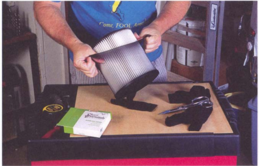
Pulling a nylon stocking over a pleated-paper filter prevents coarse chips and shavings from getting stuck in the deep pleats and clogging the filter, making it easier to clean.
