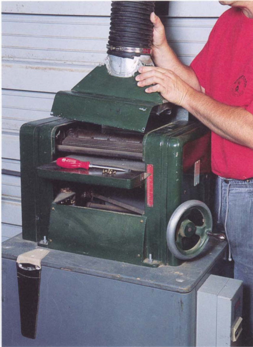
A sheet-metal hood surrounding a thickness planer's cutterhead is a must for clean planing operations. Unless they're whisked away by dust collection, chips are pressed into freshly planed wood surfaces by the machine's outfeed roller.
