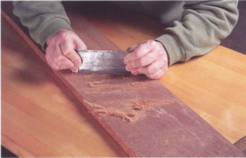
A well-tuned cabinet scraper is a clean and quiet alternative to using a dust-churning power sander to smooth the surface of a wood panel, plank, or part.
