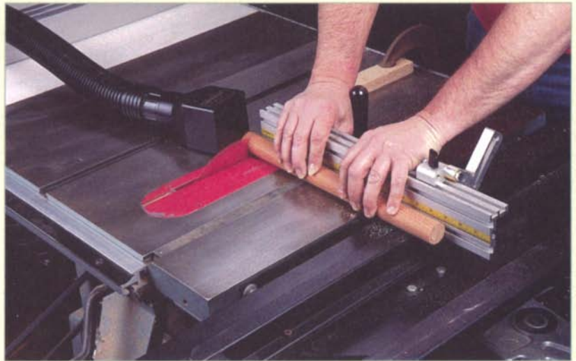
You can use a shop vacuum to suck up small workpieces, such as the short round slices shown here, before they are snagged by the blade and chewed up or thrown. Here, the vacuum hose connects to a Veritas® Magnetic Dust Chute, which adheres to the saw's cast-iron top.
