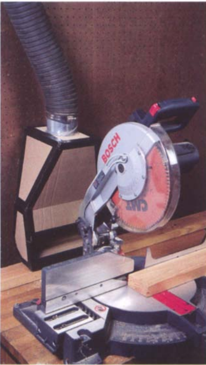
A venturi-box hood, mounted behind a compound miter saw, speeds airflow and thus improves the capture of sawdust hurled by the sawblade. Made from corrugated cardboard and tape, the hood has a mouth wide enough to catch chips even when the saw is set for a miter cut.
