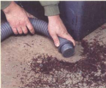
Stretching a piece of wire mesh over the end of a vacuum hose prevents it from accidentally sucking up small tools and hardware.
