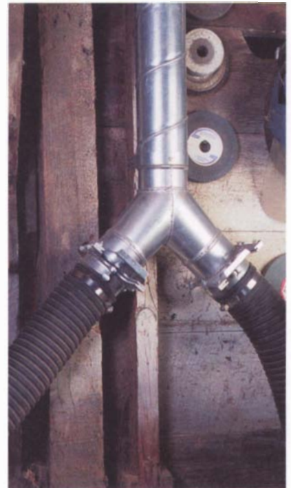
Wye branches are handy fittings for connecting a single branch duct to two machines. Blast gates fitted on both legs of the wye allow you to open the gate to one machine at a time.
