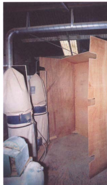
Building a movable enclosure can cut down on the noise created by a dust collector located inside the shop. The plywood box shown here has notches cut in the sides, to allow it to fit tightly against the wall, and is fitted with wheels for quick access to the collector.
