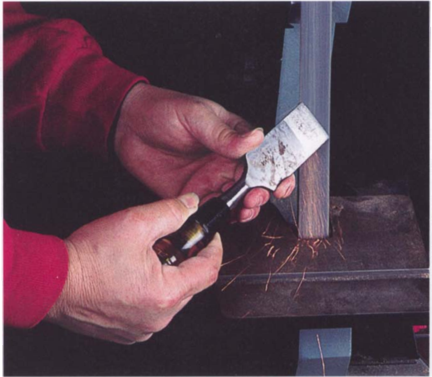
Grinding an edge on a tool, such as this bench chisel, generates a shower of sparks, which can quickly ignite any fine wood powder that has collected around the base of the grinder and cause a shop fire.
