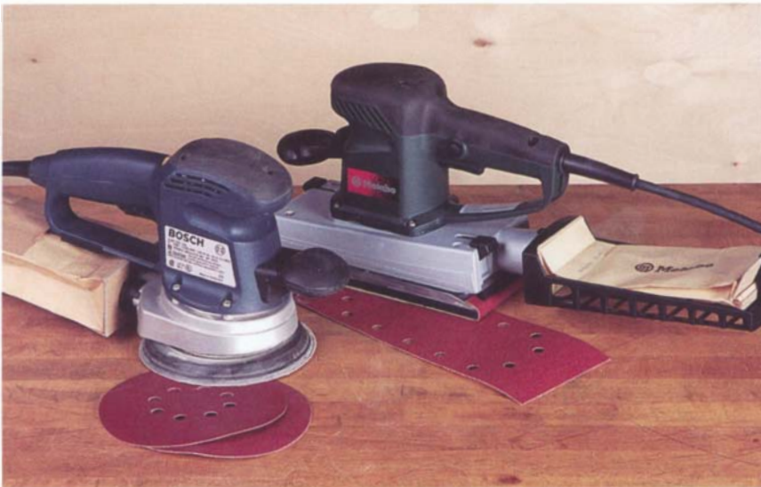
The disposable paper bags on these portable power sanders do a better job of filtering out fine dust than most cloth bags. They also make it easier to dispose of the fine dust they collect.
