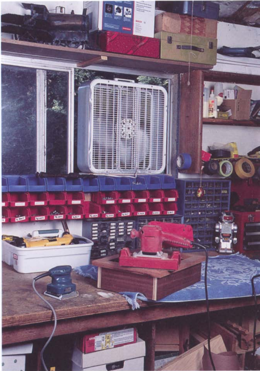
A simple box fan perched on an open windowsill or in a doorway can provide enough ventilation to remove the lion's share of fine sanding dust generated in a small woodshop.
