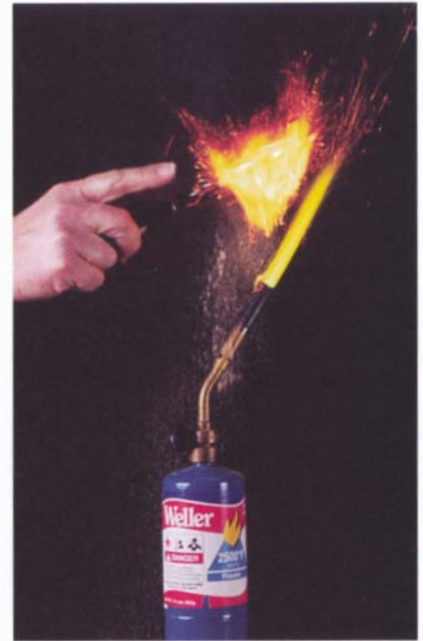
A small pinch of fine wood dust sifted over a blowtorch flame combusts with surprising volatility, demonstrating how readily fine dust in a collection system can burst into flames. (Please don't try this at home!)
