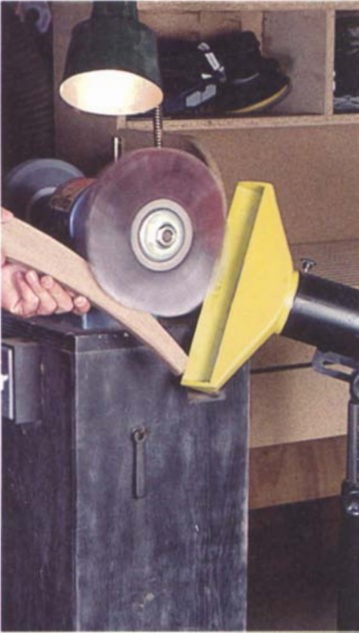
A dust nozzle mounted on a freestanding base is efficient and versatile for collecting fine dust from arbor-mounted wheels and drums.
