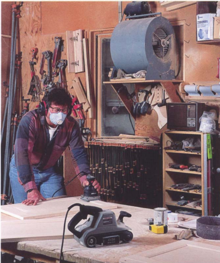
Cabinetmaker Cliff Friedlander uses a large squirrel-cage fan to exhaust fine sanding dust from his shop in temperate Santa Cruz, California. An open window across the shop allows fresh air to enter.
