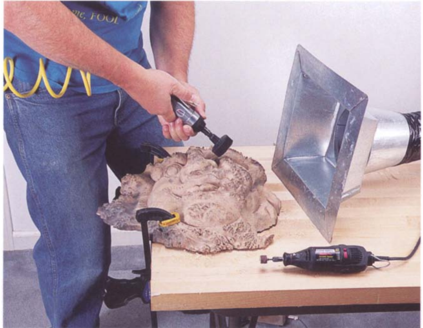
Dust and chips created by freehand sanding or grinding operations can be captured if you work close to a flanged hood. The hood here was made from a sheet-metal roof jack joined to 4-in. flexible hose.
