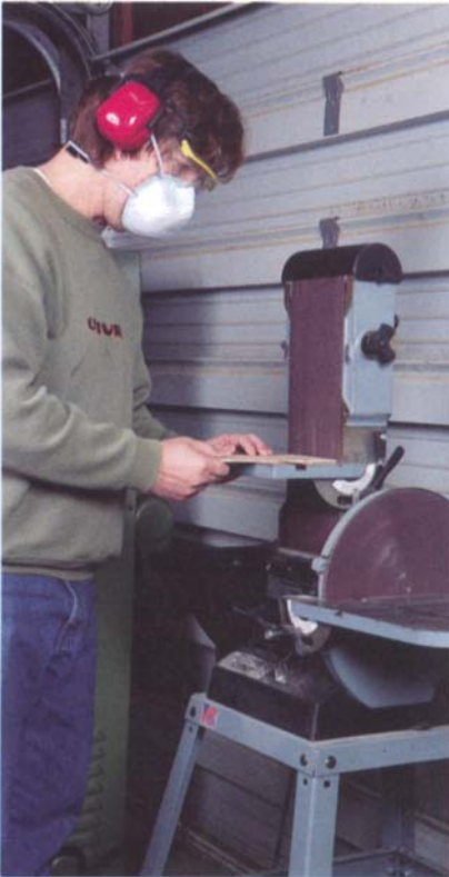
A disposable face mask provides inexpensive respiratory protection from the long-term effects of fine dust, created in great quantities during jobs such as machine sanding.
