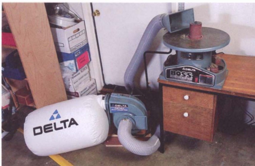
The Delta 50-820 compact portable collector is easy to wheel around the shop to wherever it's needed. It takes only moments to connect the collector to a small machine, like this oscillating spindle sander.
