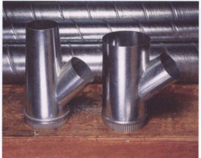
For efficient system performance, ducts should merge at a 45-degree angle whenever possible. A lateral tee (right) connects a branch to two ducts of the same diameter; a tee-on-taper (left) is used when the connecting ducts change diameter.
