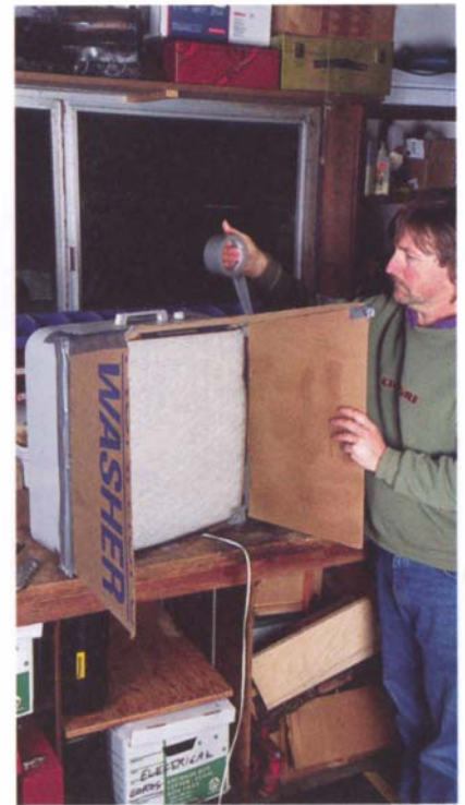
To make shop ventilation more efficient when using a box fan, tape a three-sided cardboard baffle to the fan's frame. A furnace filter taped to the front of the fan traps dust and keeps the fan blades clean.
