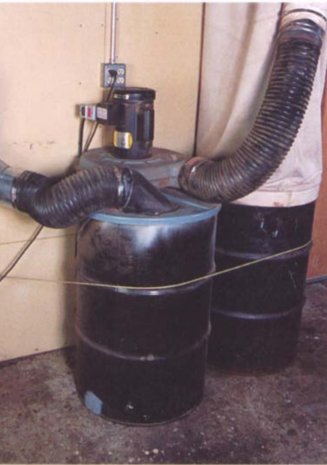
Barrel-top collectors, such as this Delta 50-665, provide the safety and performance of two-stage collectors in a compact unit that can serve as a central collector for a small-shop system.
