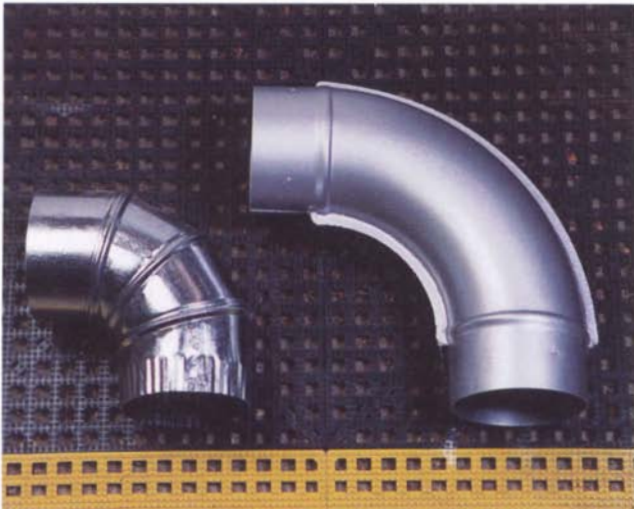
The large-radius elbow (right) allows air and dust to negotiate turns in the ductwork with less friction than a standard tight-radius HVAC pipe elbow (left), making for a more efficient collection system.
