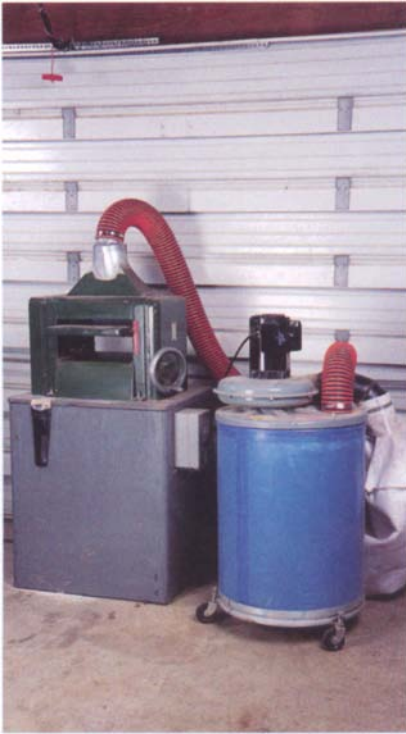
Portable collectors, such as the canister-top Delta 50-179 shown here, are a step up from shop vacuums, both in terms of power and chip-gathering capacity.
