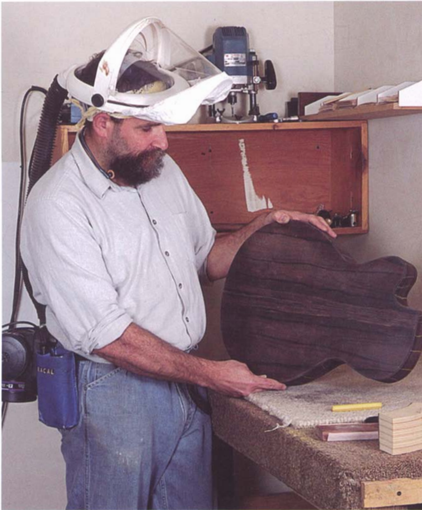
To get maximum protection from the dust of exotic woods, guitar maker Jeff Traugott uses a PAPR. Most PAPRs have a belt-worn filter and battery pack that blows air into a visored helmet or headpiece via a flexible hose.
