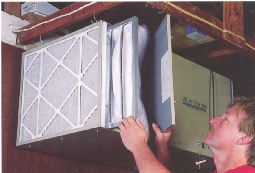
To make cleaning and replacement easier, most air-filtration devices house their prefilters in a slide-in compartment on the front of the unit. The JDS Air-Tech 2000™ model 8-12 shown here also has a side door that allows easy access to the unit's bag-type main filter.
