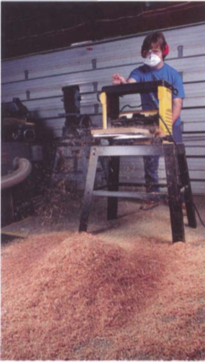
Without dust collection, the large shavings generated by even a small thickness planer grow into mountains of debris that get underfoot and can create a fire hazard.
