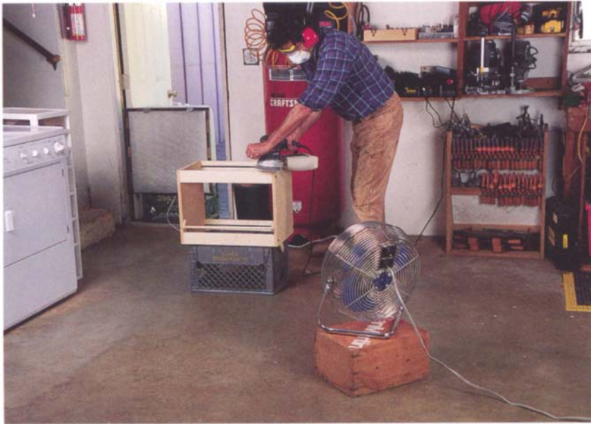
A household box fan with a furnace filter taped over its intake, set in an open doorway, provides an effective means of removing fine sanding dust from the shop. To improve ventilation performance, use a circulation-type fan to blow dusty air away from you and toward the box fan.
