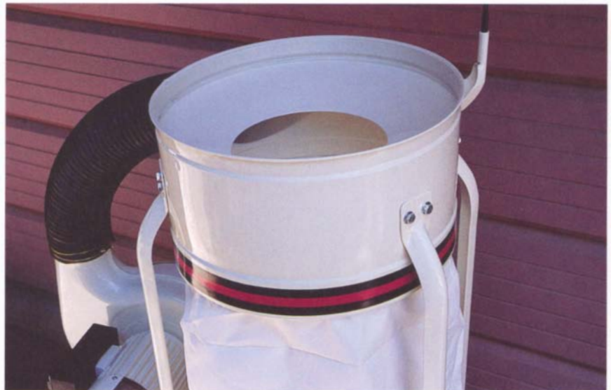
The dust-deflector ring inside the bag holder found on many single-stage collectors encourages large debris and coarse dust to swirl and settle to the bottom of the lower bag.
