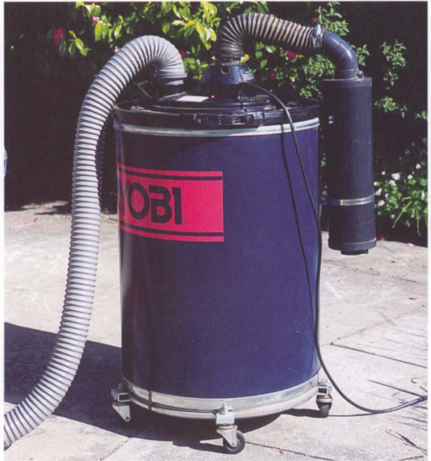
Quieting the nerve-grating racket produced by some canister-style shop vacuums can be done by adding a muffler. Here the compact plastic muffler is mounted to a Ryobi shop vacuum.
