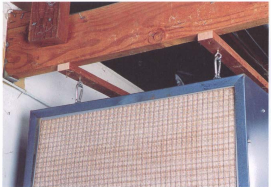
Spring-loaded safety hooks and eyebolts provide a secure means of attaching an air-filtration device to the ceiling of your shop yet allow it to be taken down for convenient cleaning or servicing.
