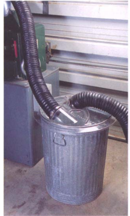
A dust preseparator canister lid fits atop a standard galvanized trash can and adds capacity to a small collection system as well as preseparation ahead of the blower.
