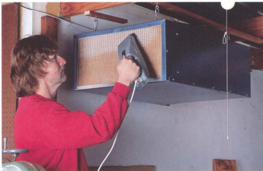
To prolong an AFD prefilter's life, vacuum it clean when it has become coated with dust. The vacuum's brush tool allows thorough cleaning without damaging the filter.
