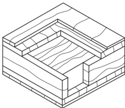
Banded Lumber Core: Bands must be made from clear stock; other specifications are as agreed upon by buyer and seller. Bands can be applied to one or two ends (B1E, B2E); one or two sides (B1S, B2S); two ends, one side (B2E1S); two sides, one end (B2S1E); or two sides, two ends (B4)
