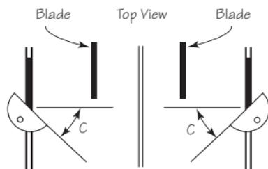
Angle of Miter Gauge (C)
