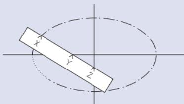
3. Position the straightedge so that Point Z falls along the vertical line and Point Y falls along the horizontal line. Hold the straightedge in position, then mark Point X, which represents a point on the circumference of the ellipse.
