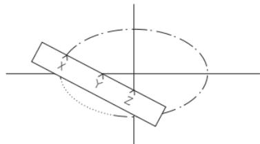
4. Continue moving the straightedge, always keeping Point Z on the vertical line and Point Y on the horizontal line. Mark a new Point X after each movement of the straightedge. Mark as many points as needed to create a smooth curve along the entire circumference of the ellipse.
