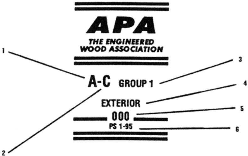
The grade mark for plywood, identified by the face and back veneer grades, includes (1) the grade of the face veneer, (2) the grade of the back veneer, (3) the species group number, (4) the exposure durability classification, (5) the lumber mill that produced the panel (shown as a number) and (6) the applicable product standard.
