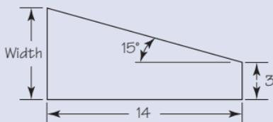
The desk side creates a right triangle with one known side (B) and one known angle (A). To determine the overall width of a side, calculate the length of side C, then add that length to 3".
