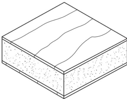
MDF Core: A medium-density fiberboard core with hardwood veneer on each face
