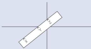
1. Draw a horizontal line at least 48" long on the glued-up stock for the tabletop. At the midpoint of the horizontal line, draw a vertical line at least 30" long. Make sure the lines are perpendicular to each other.
