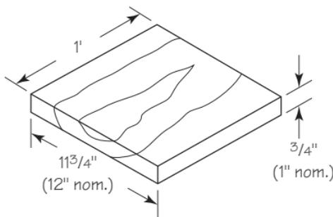
Several formulas are used to calculate board feet, but the one most often used is as follows:
