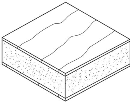
Particleboard Core: A particleboard core with hardwood veneer on each face
