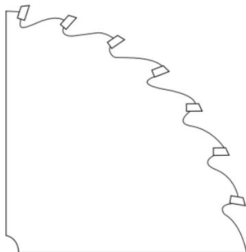
For cutting with (parallel to) the grain. Requires fewer and larger teeth than crosscut blades. Cut is relatively rough. Blade shown is carbide-tipped.
