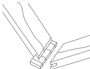
Miter With Spline Key
