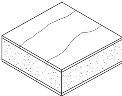
Hardboard Core: A hardboard core with hardwood veneer on each face
