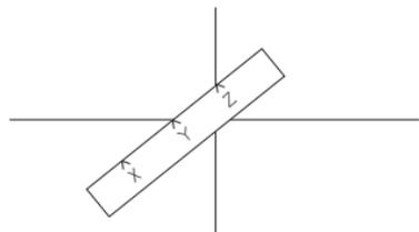
3. Position the straightedge so that Point Z falls along the vertical line and Point Y falls along the horizontal line. Hold the straightedge in position, then mark Point X, which represents a point on the circumference of the ellipse.
