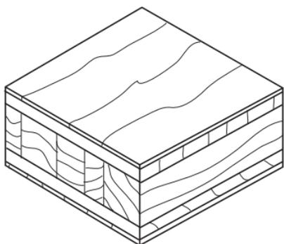
Lumber Core: Made from three, five or seven plies of edge-glued solid lumber; may be either hardwood or softwood; species mixing not allowed. Grades available are Clear, Sound and Regular. A Regular grade clear-edge version is available with edge strips at least 1½" wide to facilitate edge molding and shaping
