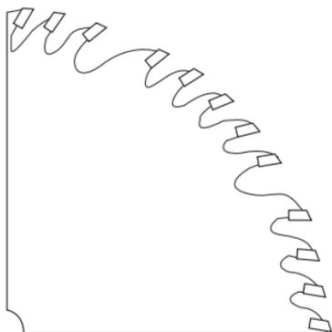
For both crosscutting and ripping. The number and size of the teeth are a compromise between the crosscut and rip blade designs. Eliminates having to constantly change from rip blade to crosscut blade. A good general-purpose blade for all cuts, but it doesn't rip as well as a rip blade or crosscut as well as a crosscut blade. Blade shown is carbide-tipped.
