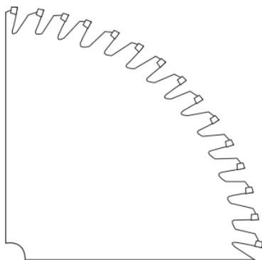
For cutting across the grain or at a diagonal. Has more teeth than rip or combination blades, resulting in a smoother cut with a minimum of splintering. Blade shown is carbide-tipped.
