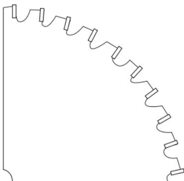
Plywood blade shown, but specialty blades also include laminate-cutting blades, thin kerf blades and others. Blade shown is carbide-tipped.
