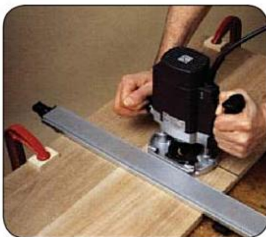
A combination bar clamp and edge guide helps a router cut a dado that is perpendicular to the panel edges.
