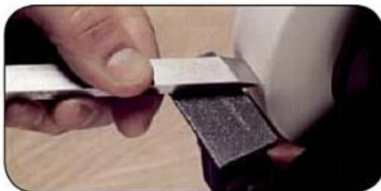
The grinder is a multipurpose tool for the wood turner. Here, the nicked cutting edge of a skew chisel is squared before grinding the bevel.
