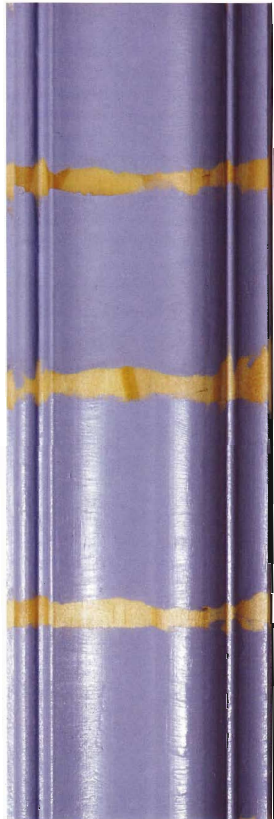
Four types of paint finishes in descending order—flat, eggshell, semigloss, and gloss. They range from matte to shiny.
