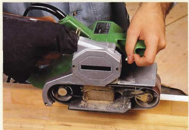
A belt sander has two drums that spin and guide a continuous belt of sandpaper over the work.
