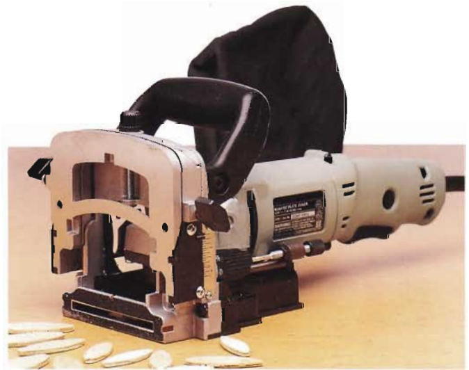
A biscuit joiner cuts slots into the edges of boards so that you can join them securely with wood wafers and glue.
