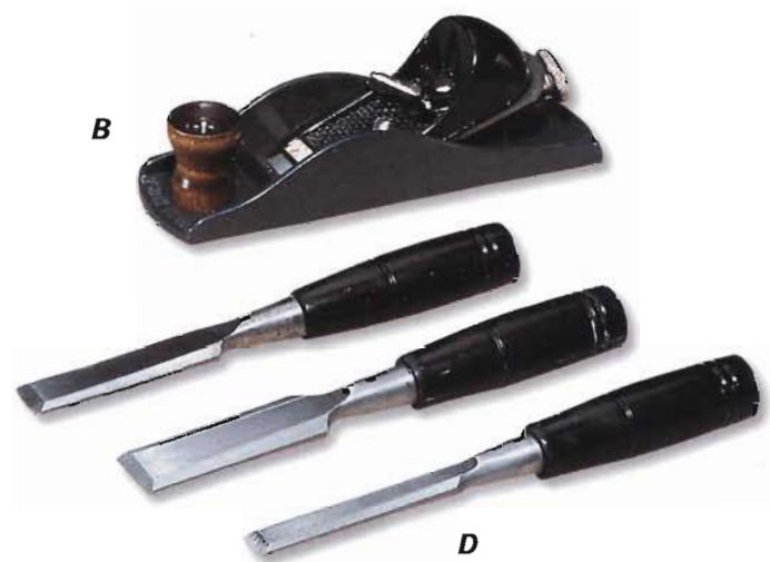
A —bench plane; B —block plane; C —cabinet scraper; D —chisels; E —utility knife
