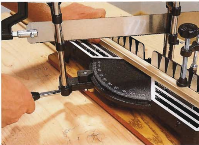
2 Like power models, hand miter boxes can swing and lock to cut angles left or right of the 0-deg. central setting.
