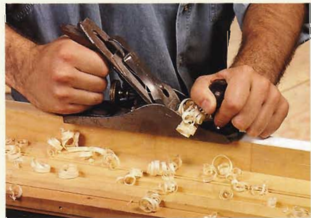
A hand plane with an adjustable blade and a long bed can true up and clean the edge of a board.
