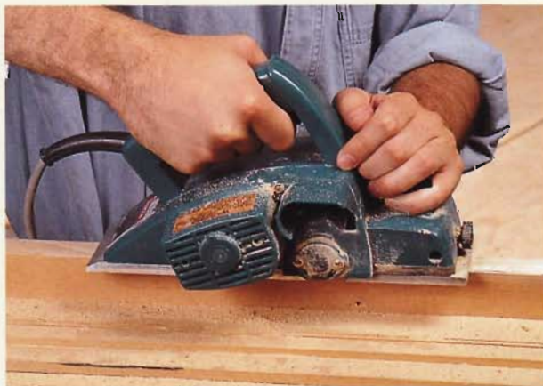
A power planer has a small rotating blade that you can adjust to remove a little or a lot of wood.
