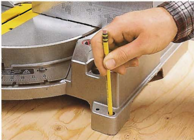
4 Set your saw on the center of the platform, and mark the bolt-down locations with a pencil.
