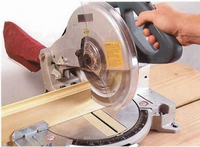
1 Start by making a square cut (or miter if you plan to cut a cope) on the far end of the board you need to piece.
