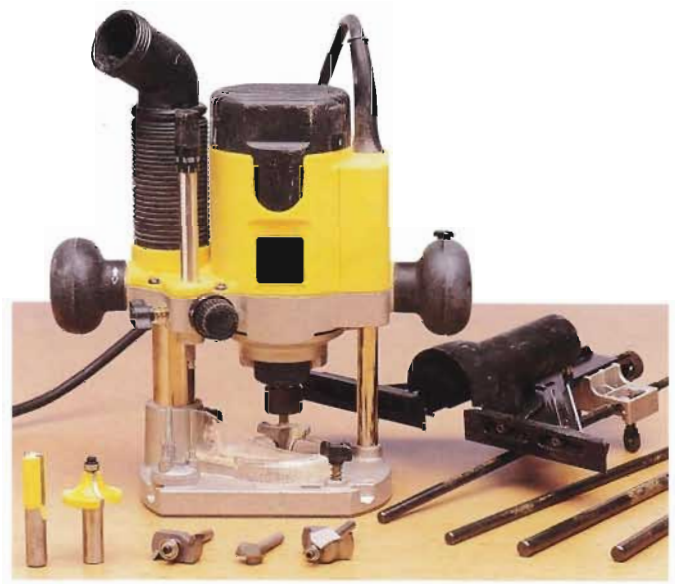
A basic router setup includes a rip fence with extension guides, straight-cutting bits, and molding profile bits.
