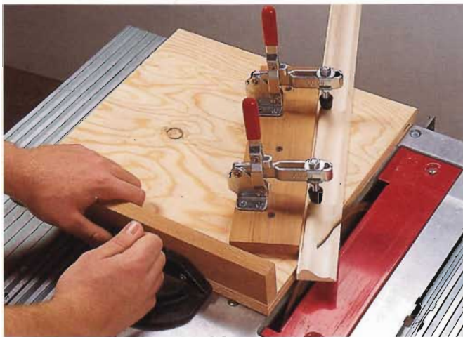
5 Screw hold-down clamps to the angled member of the jig to hold trim pieces firmly in place as you cut them.
