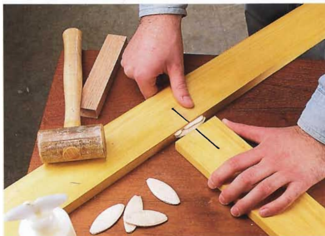
5 Set compressed wood wafers into one side of the joint, tap the other board into place, and clamp overnight.
