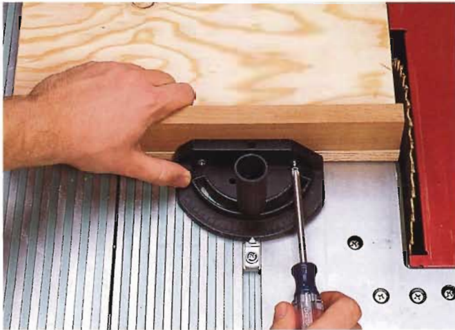
2 Screw the jig to the table saw's miter gauge, aligned flush with the blade. (The blade guard is removed for clarity.)
