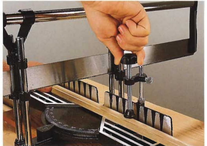
1 Many hand-powered models have a built-in clamp you can use to secure the stock against the saw fence.
