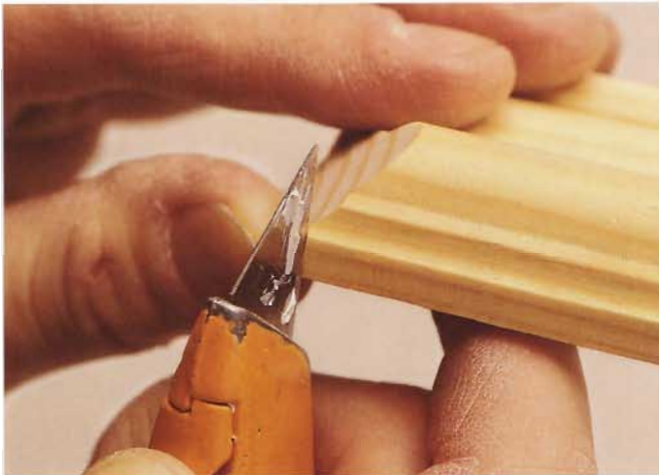
2 Use a utility knife to trim off the feathered edge of the miter cut, which is easily broken during assembly.
