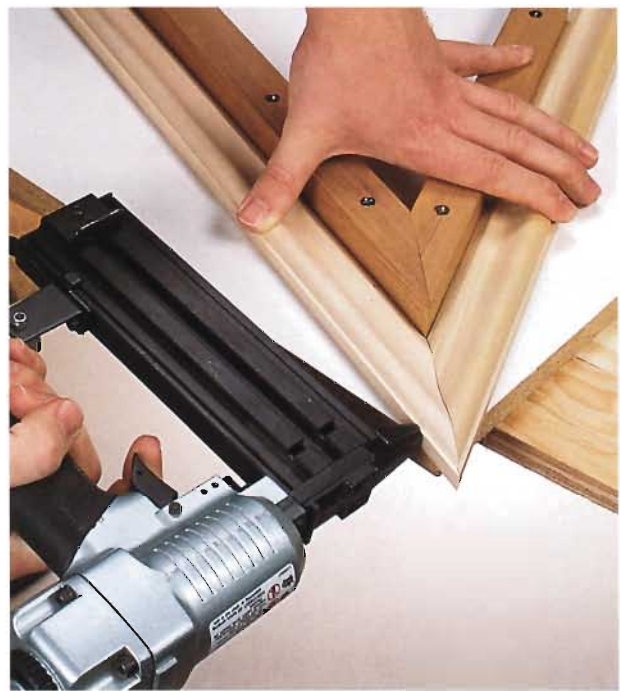
A jig like this , secured to a work surface, allows you to hold the frame pieces for a tight fit and secure nailing.
