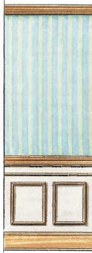
36" Wall-Frame Treatment with Vertical Frames
