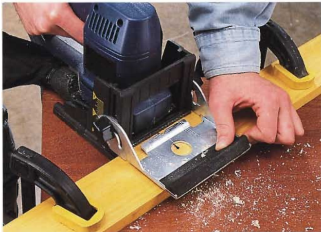
2 Set the depth of cut of the plate joiner; then line up the notch on the shoe with your mark and pull the trigger.
