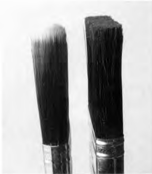
A chisel-cut brush (left) has bristles that taper to a slightly rounded point in the middle. A square- or flat-edge brush (right) has bristles that are all the same length.
