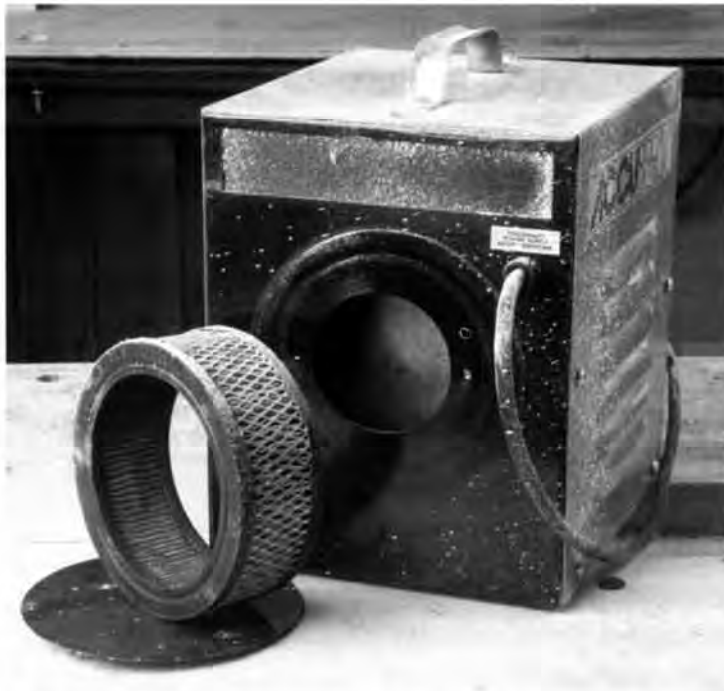
Turbines keep your air system clean and are easy to maintain. Just clean or change the filter from time to time.
