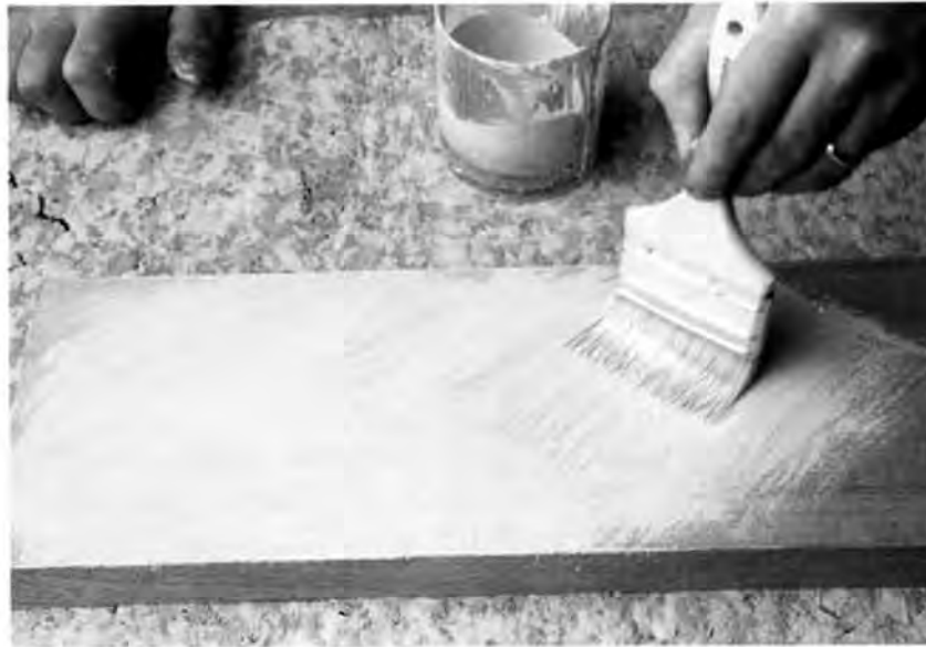
An inexpensive, disposable brush is a good tool for working paste filler around and into the surface of the wood.
