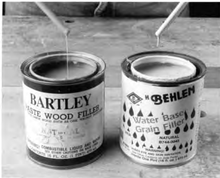
The oil-based paste filler on the left and the water-based product on the right look alike in texture and work the same. Other than the color, only real differences are how fast they dry and how compatible they are with other finishes.
