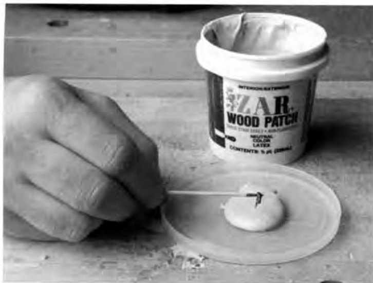
A little tint goes a long way. The small drop shown here is enough to turn this wood putty a deep, red, earthy color.
