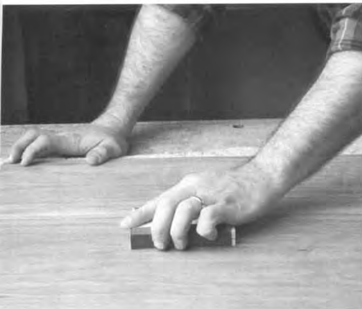
Begin the rubbing-out process by using wet/dry sandpaper to remove surface imperfections.
