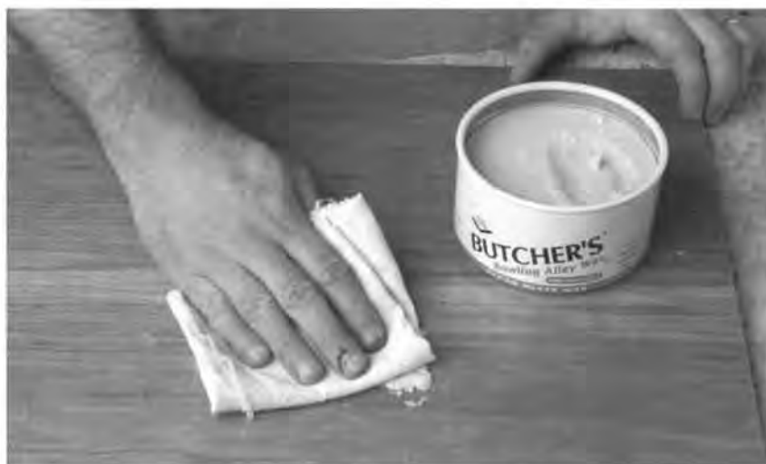
A final coat of wax, though not usually necessary, will give the finish a warmer, softer glow.
