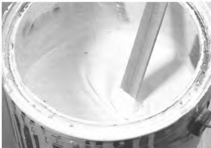
If a can of reactive finish, such as this pigmented primer, is left unsealed, the top will skin over fairly quickly.
