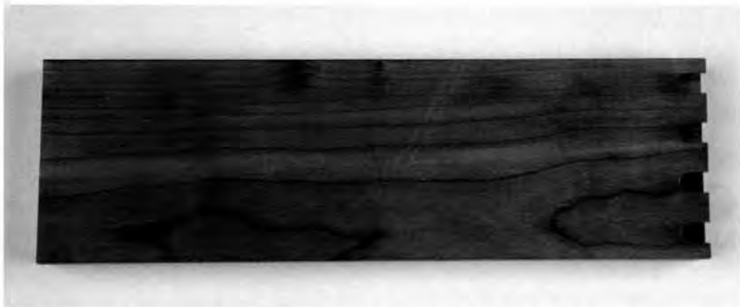
The scratch on this piece of cherry is plainly visible under the oil finish on the top but is much harder to see when coated with the water-based finish on the bottom.
