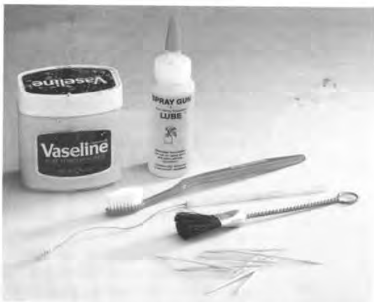
A basic gun maintenance kit should contain at least one stiff brush, some toothpicks, and an appropriate lubricant.
