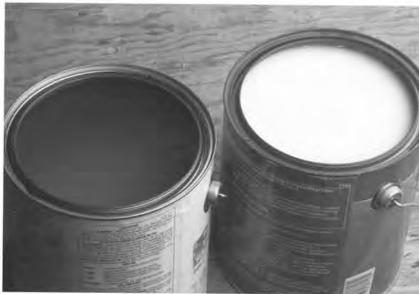
Compared with the clear, solvent-based product shown on the left, cans of water-based finish appear white or milky.
