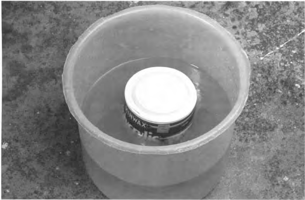
Submerging a can of finish in a bucket filled with hot water will warm the finish and help it flow better and dry quicker.
