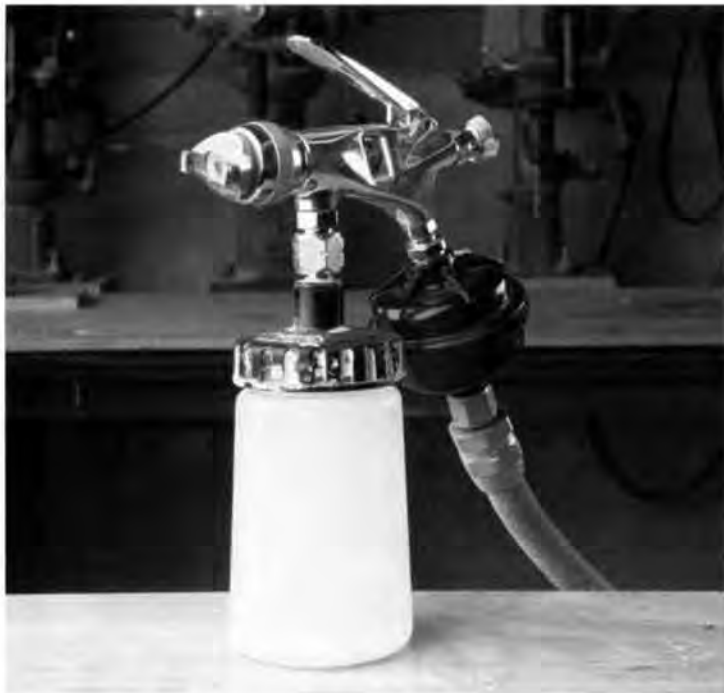
Disposable in-line filters are less expensive alternatives to fixed filters and come in handy when spraying at a job site.
