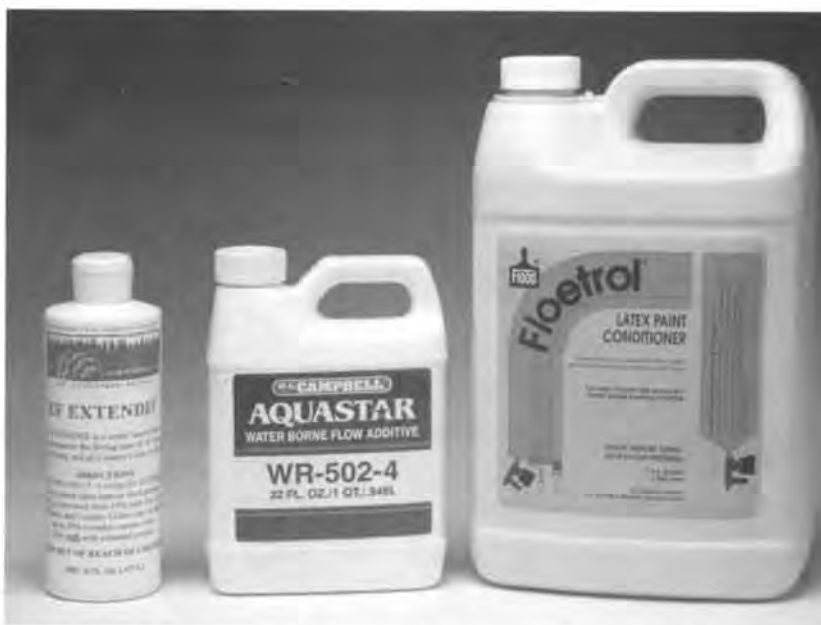
Additives for water-based products include extender (left), which is used to lengthen the “open” time of brushable finishes; flow additive (center); and paint conditioner (right), which helps latex paint flow and level better.
