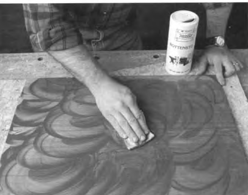
A final rubbing with rottenstone brings the surface to a high shine.
