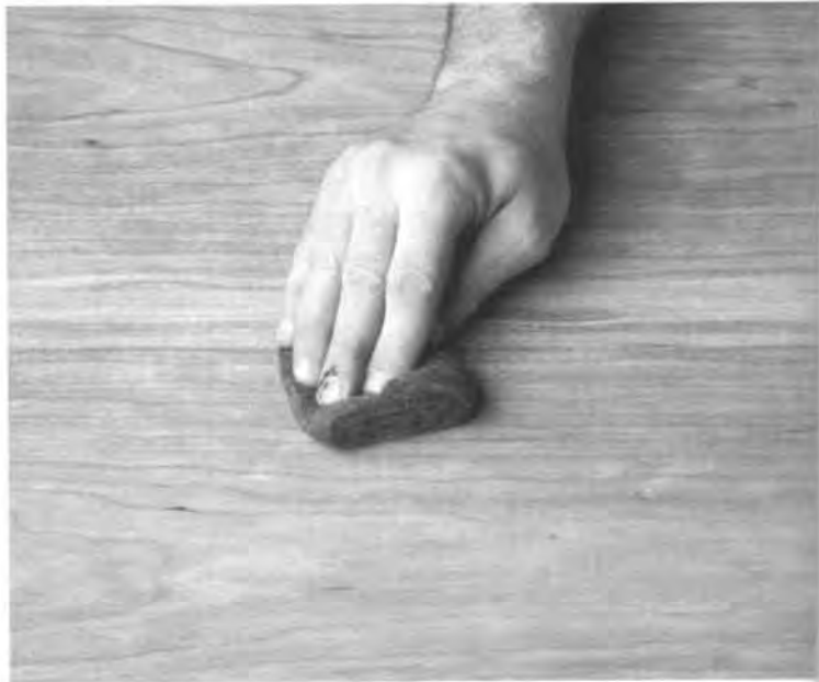
Use very fine 0000 steel wool to dull the entire surface, giving it a flat, or matte, finish.
