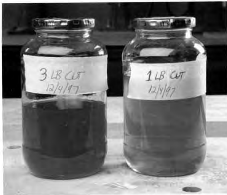
The cut refers to the ratio of shellac to alcohol. Compare the color of the 3-pound cut on the left with the 1-pound cut on the right.
