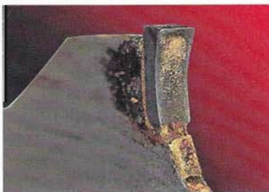
Before. Resin builds up on the shoulders and gullets of a blade, as well as the cutting edge.
