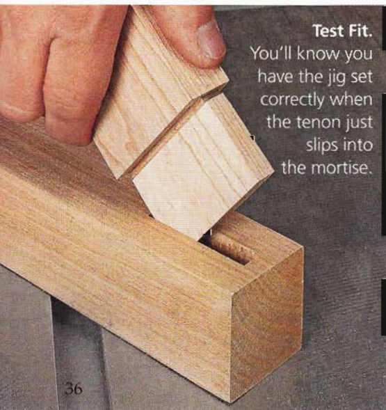
Cheek Cuts. After making the first cheek cut (above), flip the workpiece for the second cut and then test the fit (left).
