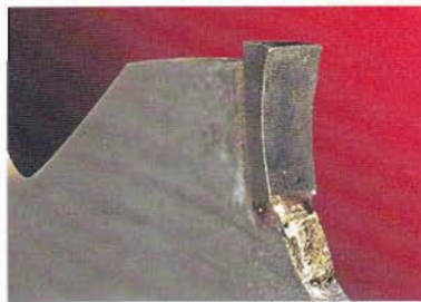
After. A good cleaner will remove resin without much scrubbing with a brush or pad.
