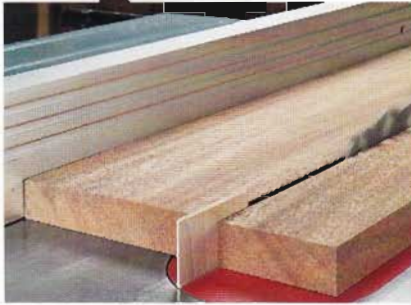
Splitter. When a blade guard can't be used, a shop-made splitter works best.
