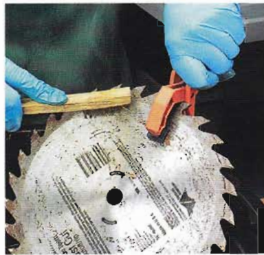
Elbow Grease. A brass brush is handy for cleaning the shoulders and gullets of accumulated resin.
