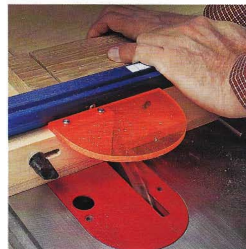
Blade Guard. The guard helps to keep your fingers away from the spinning blade as it exits the sled.
