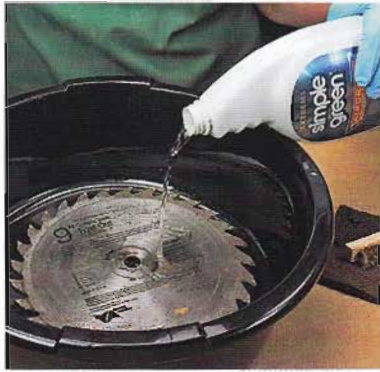
Apply Cleaner. Use a clean oil pan or other flat plastic pan to soak the blade in the cleaner.
