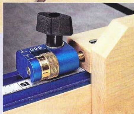
Box Joints. Turn the crosscut sled into a precise box joint jig with this commercial micro-adjuster.
