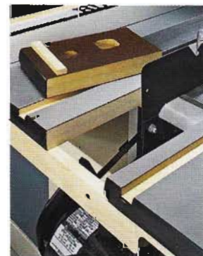
Splitter Insert. Removal of the "pop out" insert makes way for installation of the splitter and the blade guard.
