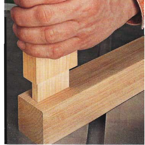
A Snug Fit. After sneaking up on the final fit, it just takes firm hand pressure to seat a perfectly sized tenon.
