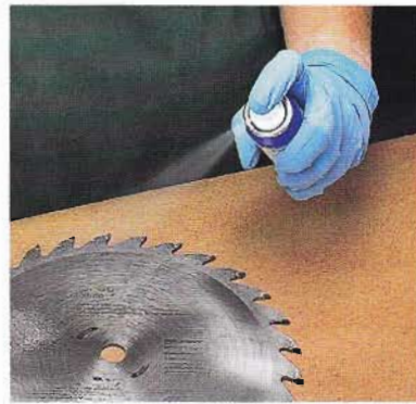
Protect. Be sure to apply rust inhibitor to surfaces cleaned with water-based cleaners.
