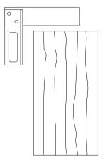
Place the two boards to be joined with the face sides together.
