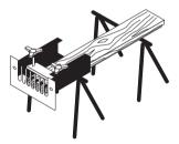
It can be screwed to a bench. Ensure packing piece is used under timber and jig. Ensure also that the other end of the timber is supported.
