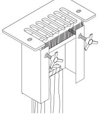
Both boards should rest against the underside of the guide plate. Ensure both pieces of wood are firmly pressed against the left hand edge of the jig: one piece against the offset stop, the other against the side of the jig
