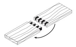
For floor boards the glued joint must be placed over a joist or a
