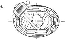
Rout the outside edge of the frame in an anticlockwise direction at repeated depths of 2-3mm until breakthrough is achieved.
