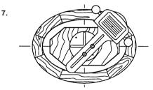
Rout the inside edge of the frame in a clockwise direction at repeated depths of 2-3mm until breakthrough is achieved.
