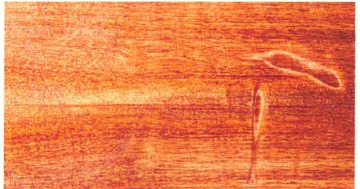
Sanding is the answer to many wood preparation problems, but it can also cause trouble. Sanding across the grain leaves ugly scratches that are emphasized by stain. Power sanders can leave gouges and divots.
