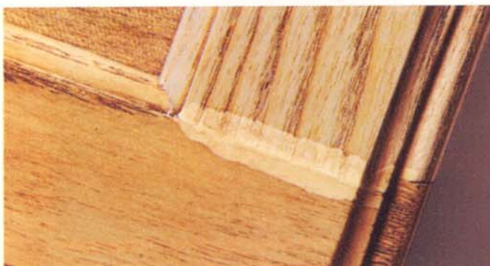
Excess glue leaves telltale marks under stains and finishes.
