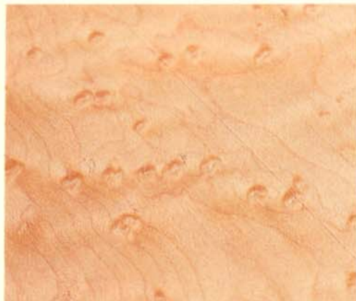
TEAR-OUT IS DRAMATICALLY REDUCED when a birdseye board is wetted just before planing. Look at the birdseye pattern—this is the same board as the one above!
