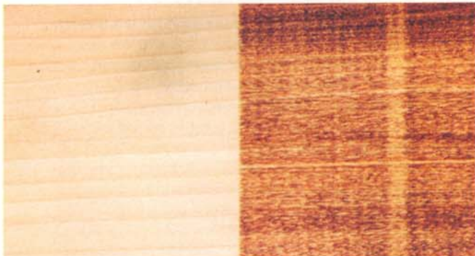
Machine marks that are practically invisible on an unfinished board stand out when you stain.
