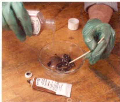
STEP 2. Make your own glaze by mixing burnt umber artists oil and liquid glazing medium into a paste. Don't go overboard—a little glaze goes a long way.
