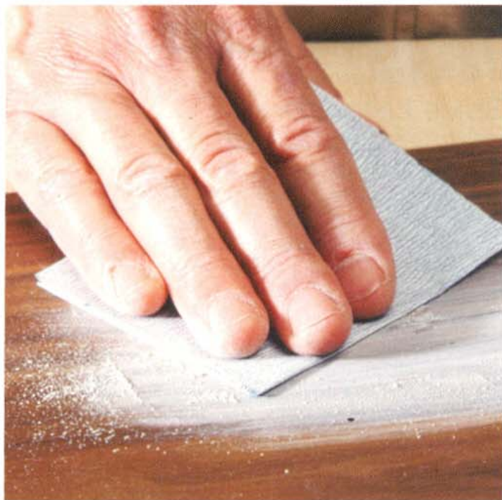
Sanding sealer is much easier to sand than polyurethane, and its sanded surface allows topcoats to firmly adhere.
