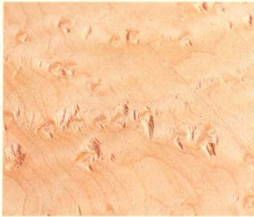
TEAR-OUT IS TYPICAL when you run a birdseye board through a planer. The grain changes direction around each birdseye, so it doesn't matter which way you run the board. It's gonna tear out in chunks.
