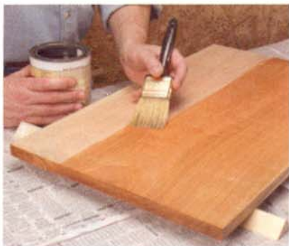
STEP 1. Seal the surface with two thin coats of dewaxed shellac. This keeps glaze from lodging in cherry's tiny pores and turning them unnaturally dark.
