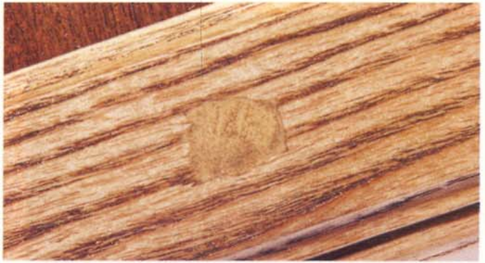
Wood putty rarely takes stain like wood, so special care is required to disguise it.
