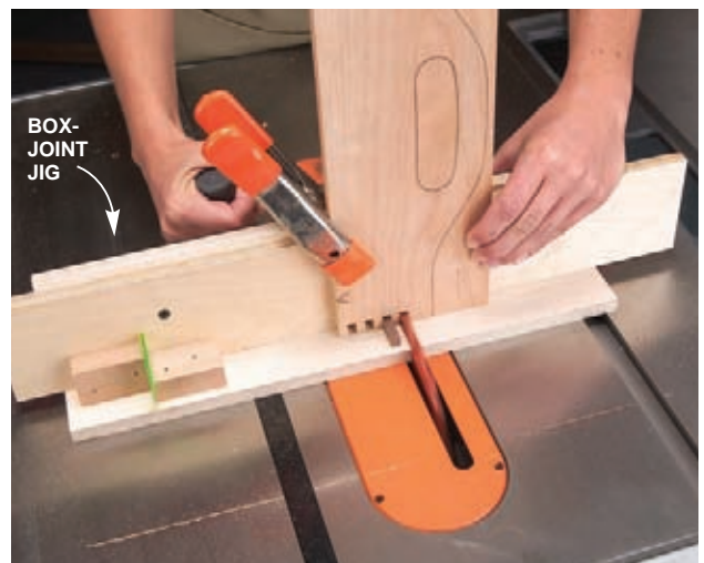
Great-looking box-joints are easy to make. I used a shop-made jig and my tablesaw, but these sturdy joints can also be cut on a router table or with a dovetailing jig.
