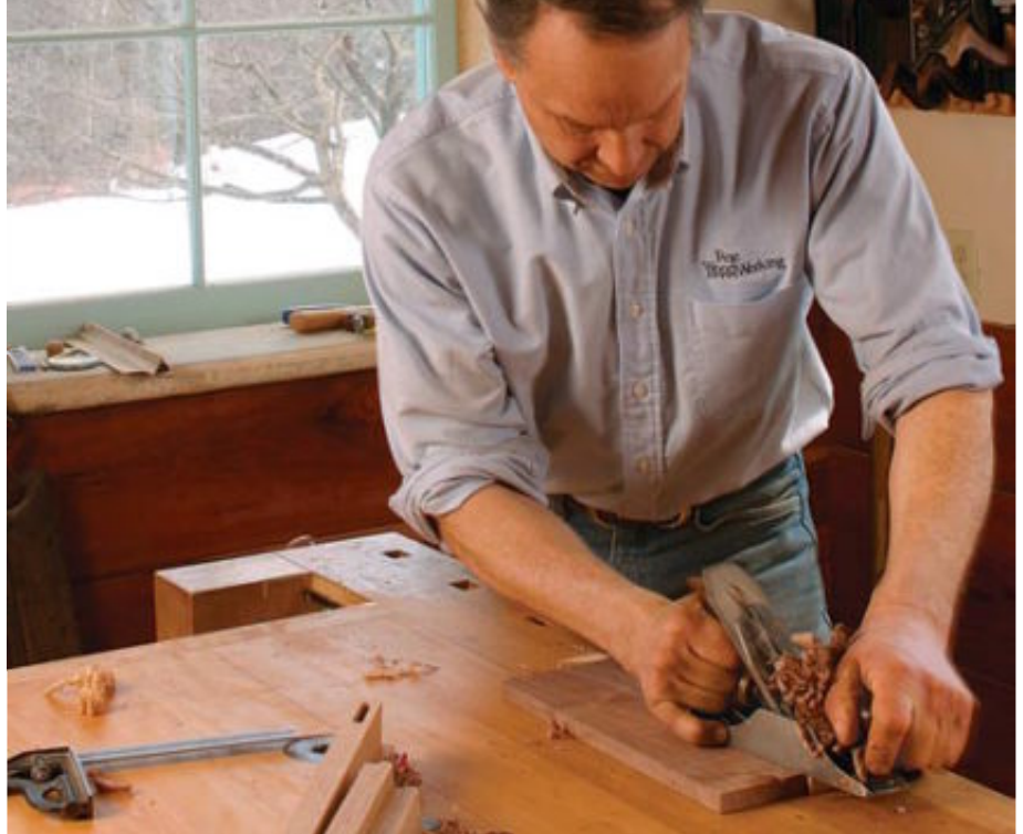
Working a surface. The No. 4's size makes it ideal for flattening or smoothing a small panel.
