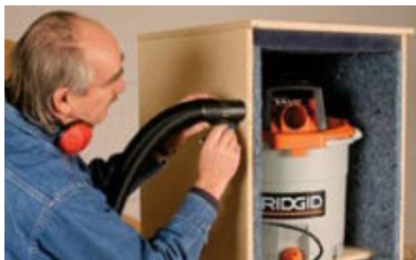
Mark the hose inlet. Use the vacuum in the box to mark where the hose will enter the box (above). For a cleaner cut through the padding, clamp a piece of plywood or Masonite to the inside (left).
