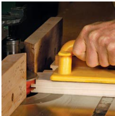
Cutting the joint. To make end-milling easy and safe, the workpiece is held against a fence that slides in the slot in the table (left). Once you've set the cutter height for one half of the joint, you can change cutters for the mating half without tweaking the fence or height settings (right).
