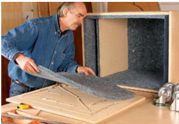
Apply the acoustic padding. The inside of the box is lined with acoustic padding stuck to the particleboard using construction adhesive.
