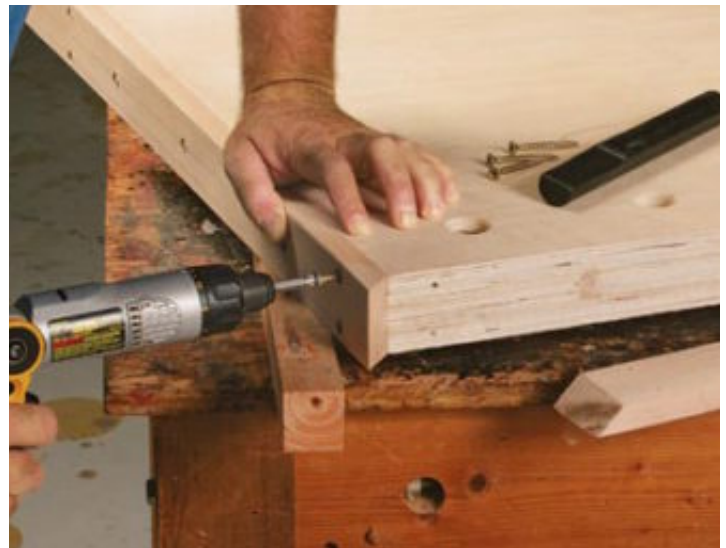
Triple-thick plywood top. Three layers of 3/4-in. Baltic birch make a hefty workbench top. Maple strips attached with coarse-threaded screws give the top a splinter-free, solid-wood edge. Holes for round benchdogs are drilled, then chamfered at the top.
