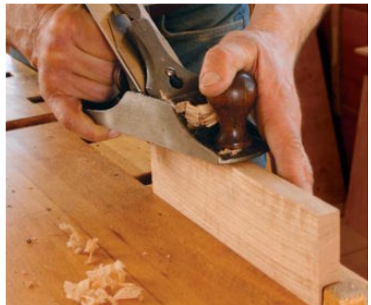
Make fine adjustments. The No. 4's throat can be closed to take very fine shavings, perfect for precisely fitting parts such as a drawer face.
