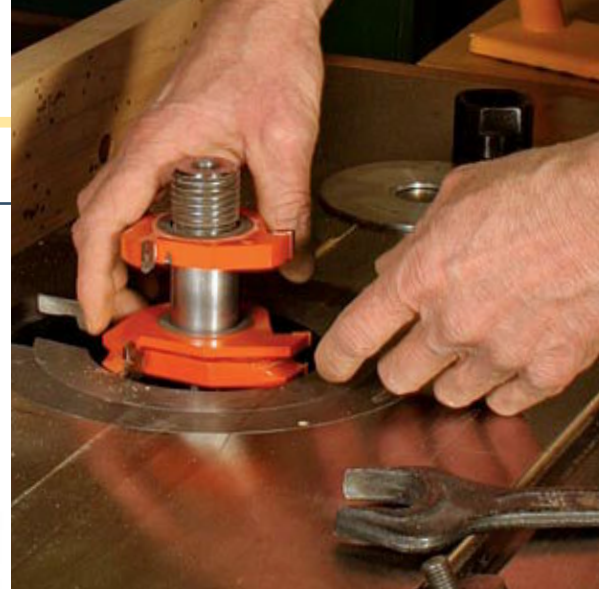
One cutter set, many frames. Stackable cutters let you resize, reposition, or delete the panel groove for solid panels, glass panes, or no panel at all.
