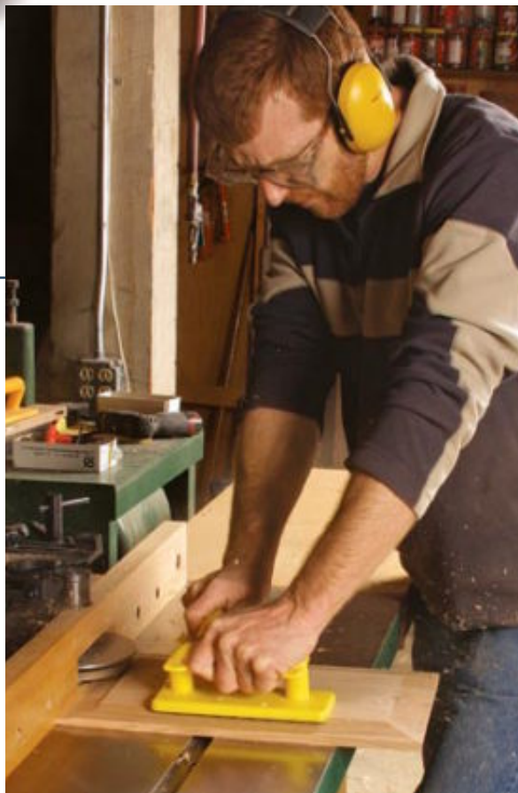
Cutter on top. To give a raised panel a consistent edge thickness, the cutter is flipped to ride above the work, with a bearing collar below. To support the work for the length of the cuts, a single fence replaces the split fence.
