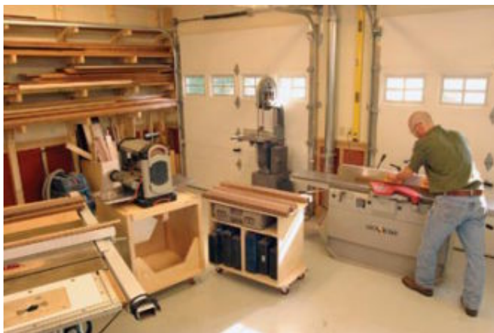
Materials and milling. With the lumber rack built next to the garage door (left), Teague can move materials easily into the shop. The jointer and tablesaw are nearby (below) for milling, and a planer cart and lumber cart roll between them to complete an efficient array.
