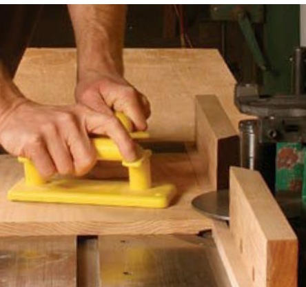
Cutter on bottom. To shape a drawer front, the cutter and bearing collar are stacked so that the work rides above the cutter.
