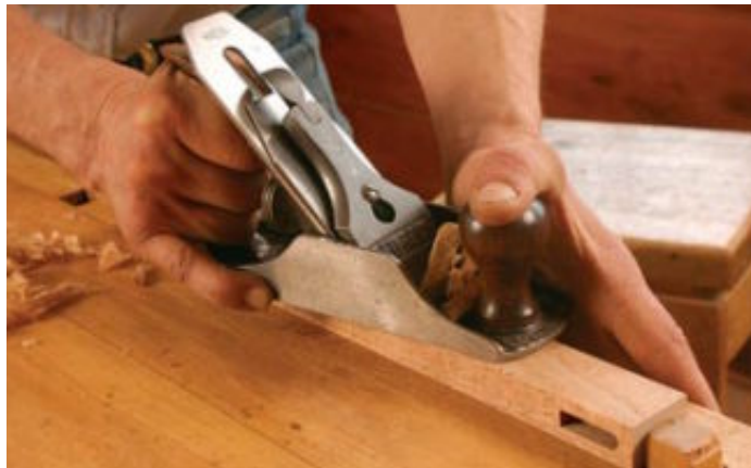
Cleaning up small parts. A few passes clean up machine marks and put a finish-ready surface on a stile.
