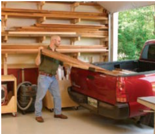
Materials and milling. With the lumber rack built next to the garage door (left), Teague can move materials easily into the shop. The jointer and tablesaw are nearby (below) for milling, and a planer cart and lumber cart roll between them to complete an efficient array.
