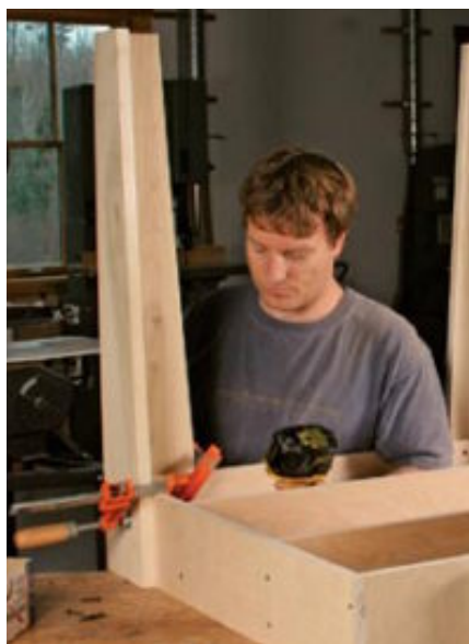
Attach the legs. Glue and clamp the legs in place before screwing them to the base from the inside.
