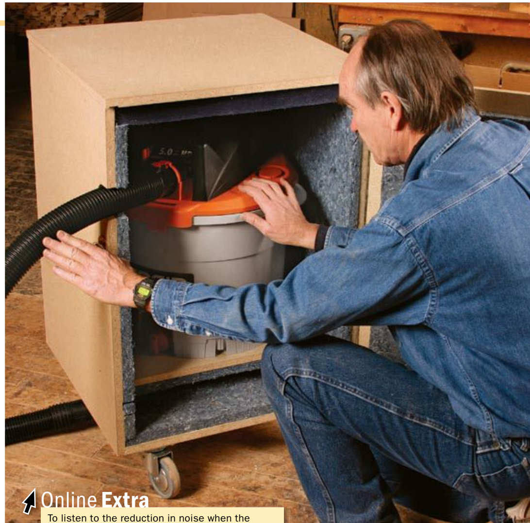
Mark the hose inlet. Use the vacuum in the box to mark where the hose will enter the box (above). For a cleaner cut through the padding, clamp a piece of plywood or Masonite to the inside (left).
