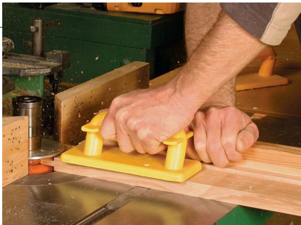
Cutting the joint. To make end-milling easy and safe, the workpiece is held against a fence that slides in the slot in the table (left). Once you've set the cutter height for one half of the joint, you can change cutters for the mating half without tweaking the fence or height settings (right).
