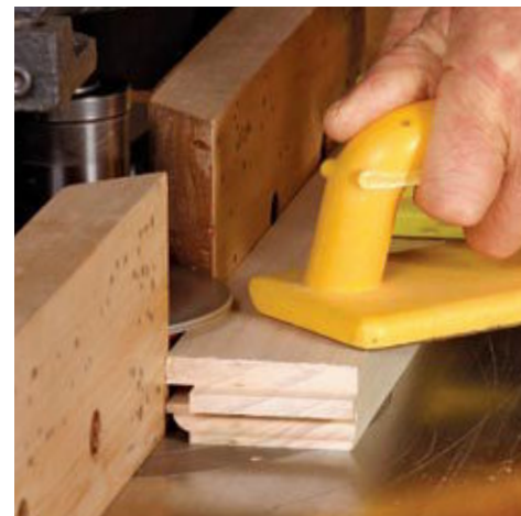
Cutting the joint. To make end-milling easy and safe, the workpiece is held against a fence that slides in the slot in the table (left). Once you've set the cutter height for one half of the joint, you can change cutters for the mating half without tweaking the fence or height settings (right).
