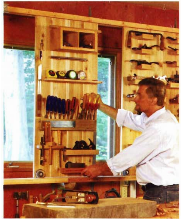
Rolling racks are versatile. To make the most of the shop's wall space, Burkin used inline-skate wheels to create four rolling tool racks. They allow him to use the space in front of the windows without permanently blocking them.
