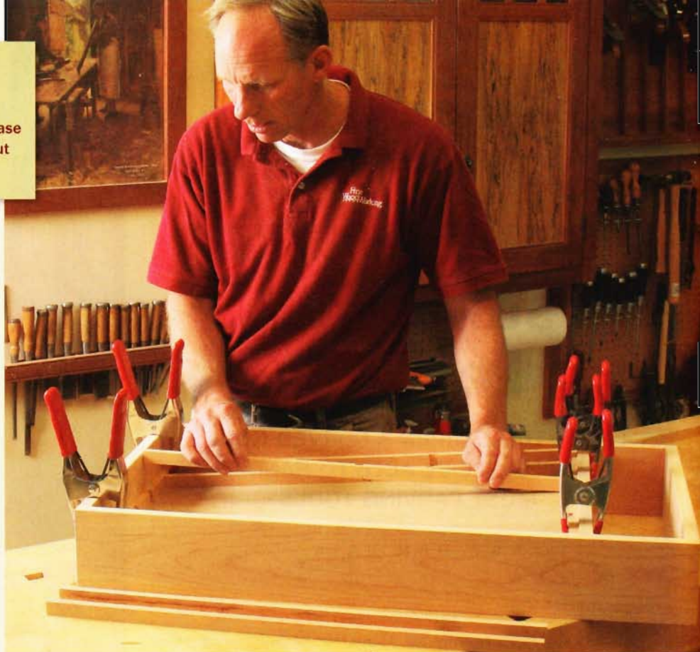
Glue in the interior frame. Install the top and bottom frame pieces first, then attach the vertical pieces. You can glue them to the back panel without clamps, but the joinery must be tight. Drill the bootlace holes in the short horizontal pieces before gluing them in.
