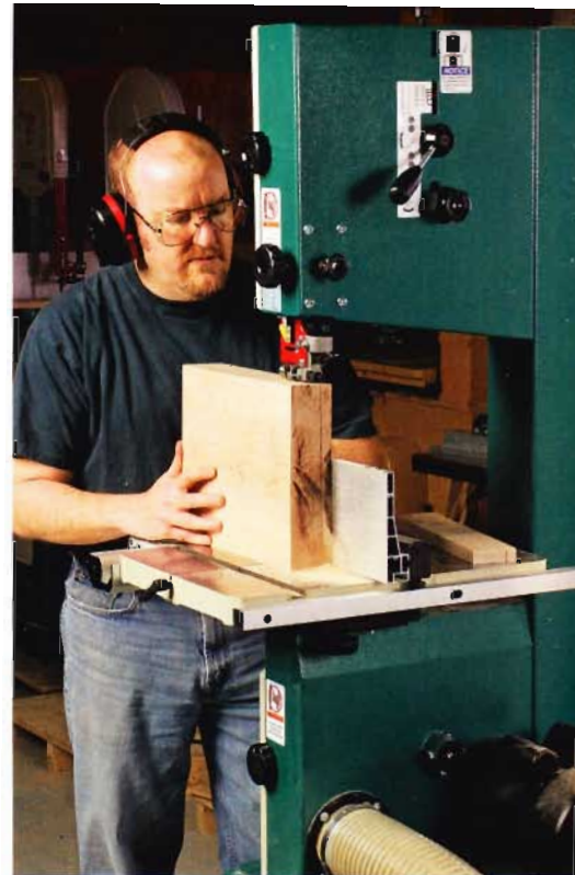
Resaw beast. The Grizzly 14-in. bandsaw comes with a tall fence and plenty of muscle to resaw wide stock.
