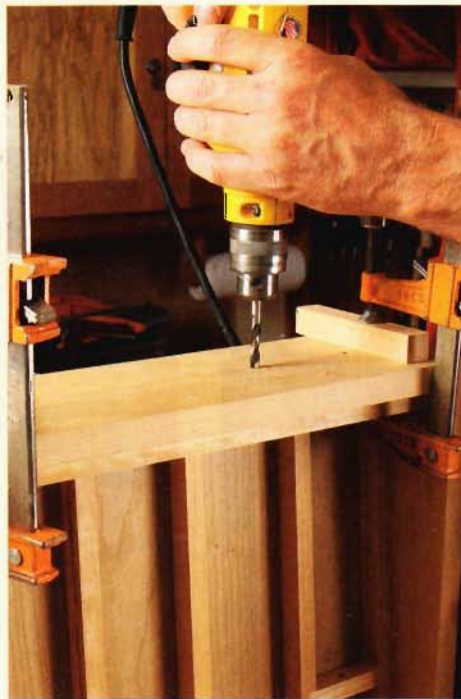
Holes for the hooks. Once the case is glued up, drill holes through the top piece for the bootlace hooks. Clamp a backer board underneath to prevent tearout.
