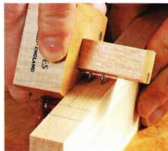
Mark the mortise. A mortise gauge marks both walls of the mortise at the same time.
