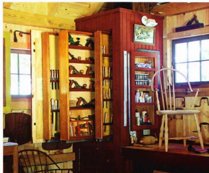
Turn drawers on end. Vertical panels, mounted on full-extension slides, pack Waters's large collection of hand tools into a small space, and the setup makes it easy to reach them.
