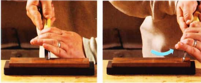
Center to side. Place the stone on the bench so its long axis crosses your body. Tilt the handle upward until the blade is seated on its bevel.
