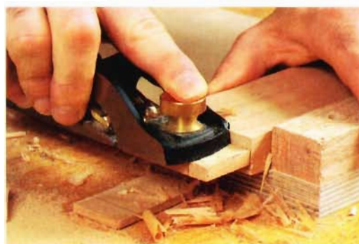
A tenon to match. The tenon is marked with the same setup as the mortise, ensuring that the tenon is the same thickness as the mortise.
