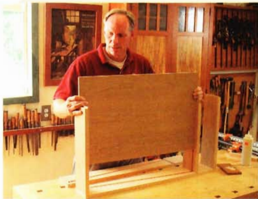
Build the box first. The plywood back panel is glued into its grooves, making the cabinet rigid.
