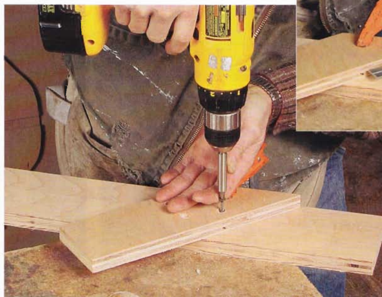
Wiggle room. Use bolts and slightly oversize holes when you need room for adjustment, such as on this crosscut-sled fence.
