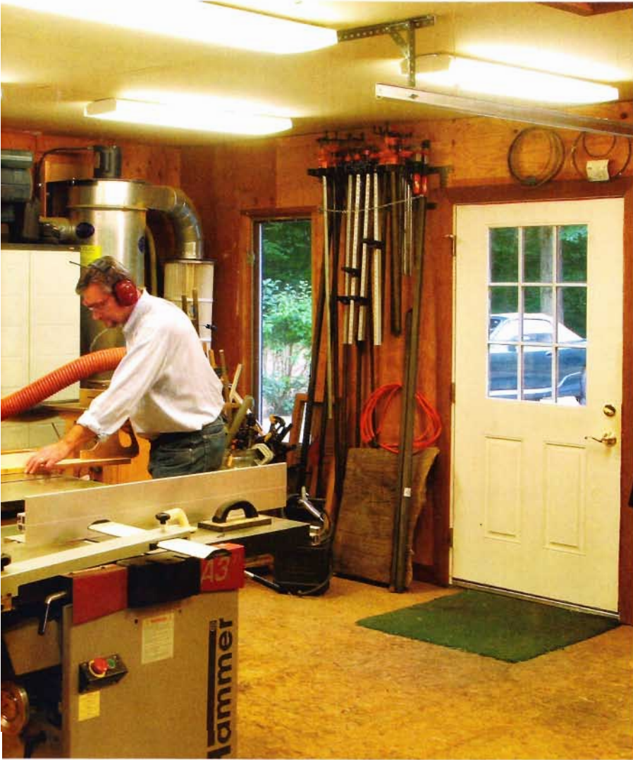
Rolling racks are versatile. To make the most of the shop's wall space, Burkin used inline-skate wheels to create four rolling tool racks. They allow him to use the space in front of the windows without permanently blocking them.
