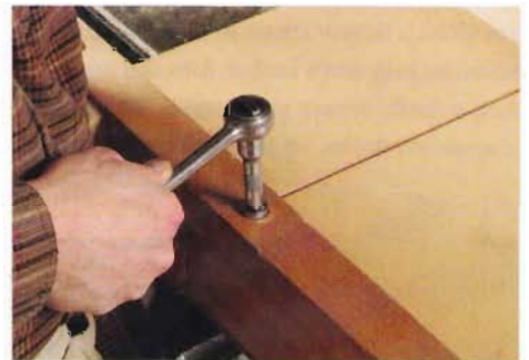
Wiggle room. Use bolts and slightly oversize holes when you need room for adjustment, such as on this crosscut-sled fence.
