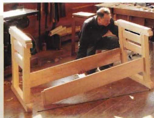
Big stretchers. Threaded rod gives a secure connection between the stretchers and trestles.
