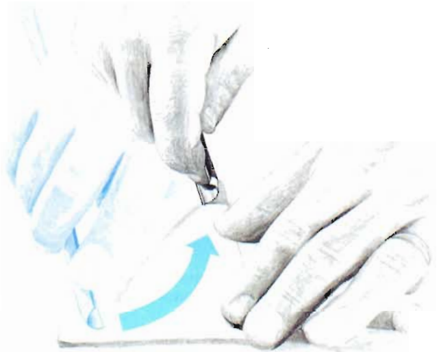
Put a curl in it. Faia simply folds the strop over to work the inside of the gouge.
