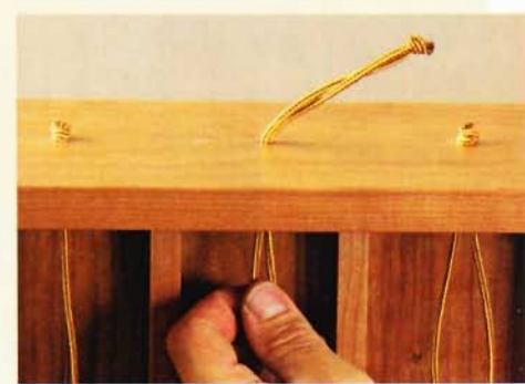
Custom hooks. Make a loop using a square knot (top) and thread it through its hole (above). Experiment to get the right-length loop for each plane.
