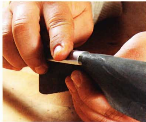
Put a curl in it. Faia simply folds the strop over to work the inside of the gouge.
