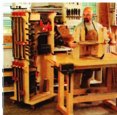
Clamp cart rolls, too. Paolini saves time by always having clamps close at hand, rather than walking back and forth to a wall-hung rack.
