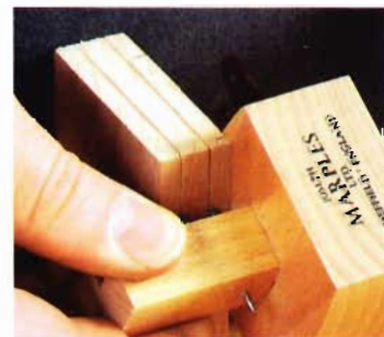
A tenon to match. The tenon is marked with the same setup as the mortise, ensuring that the tenon is the same thickness as the mortise.
