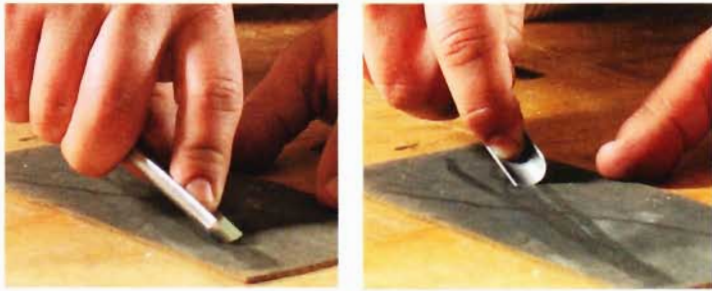
Pull and roll. Faia starts with the edge on one corner and pulls the tool toward him, rotating it onto the opposite corner as he goes.
