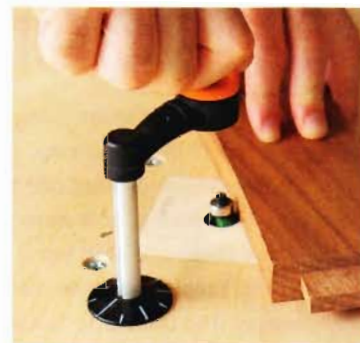
Crank and lift. The Triton comes with its own lift system for above-the-table height adjustment and bit changes.
