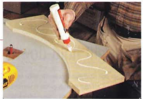
Glue for keeps. For jigs that will see repeated use, glue the components together.
