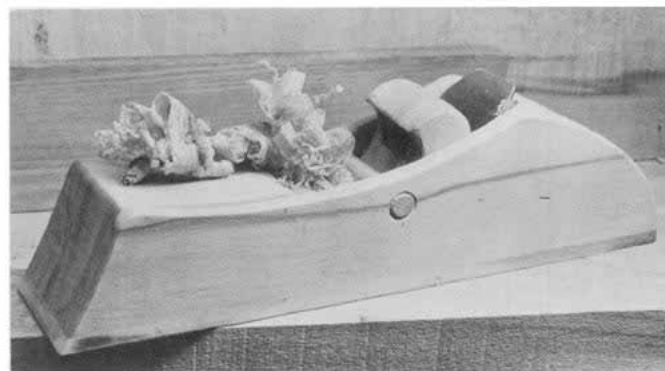
The finished plane, test shavings and all. Make the upper body shape whatever is most comfortable for you.
