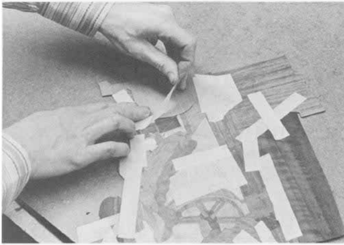
Veneer for house beam is taped in position to back of picture being cut by double-bevel method. Other tape is holding previously cut pieces that have been white glued.
