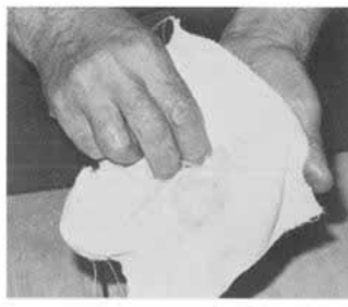
Making up a pad and working in the white pumice sprinkled on the surface, which will fill pores.
