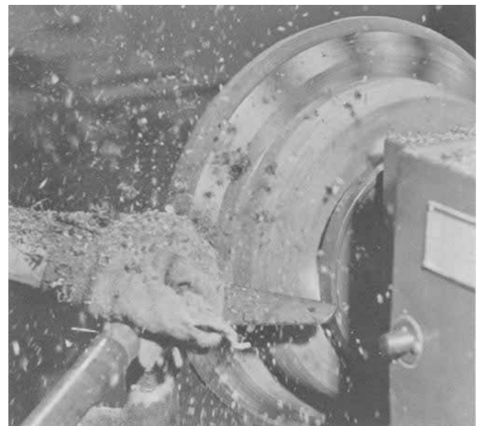
Outside of bowl is turned and finished first with lathe set at low, 600 rpms. Top walnut board gives the bowl stability during this stage. The handrest is on a moveable tripod.
