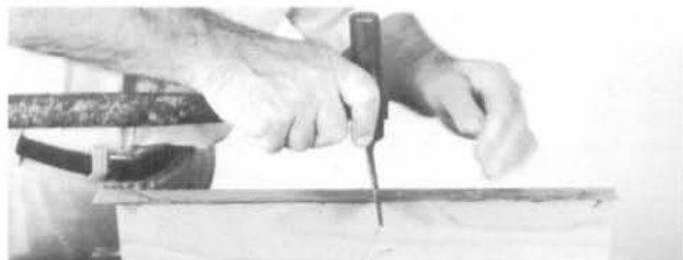
Use the veneer hammer to squeeze out the glue all along the edge.
