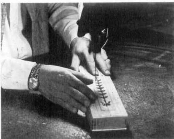
Jason French saws a sandwich of 16 veneers for fan inlay parts. The dotted line is pounce, a powdered asphaltum applied through perforations in the master pattern.
