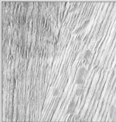
Bookmatching shows the difference between compression and tension surfaces. Compression side, right, has more sheen and is smoother than tension side.
