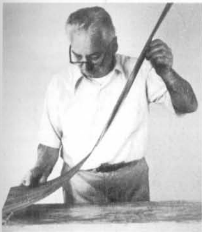
Lay veneer face down in glue. The glue that smears on it will help hammer slide easily.
