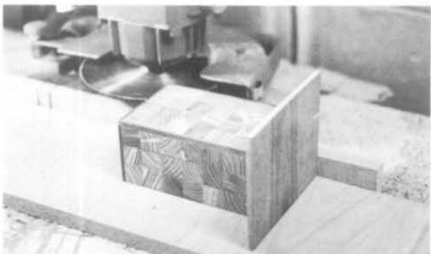
Radial arm saw with fine-tooth blade cuts lid off box. Back-up board keeps veneer from splintering.
