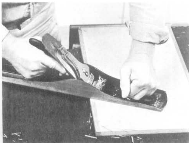
Rest the toe of the jointer plane firmly on the substrate to prevent tapering the lipping.
