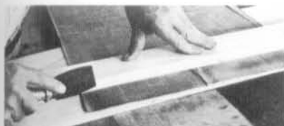
Saw veneers to length with straightedge, backup board.
