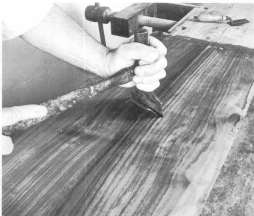
With both sheets stuck and the seam trimmed, reheat with the iron and push hard with the hammer to squeeze the excess glue out through the line of the joint.
