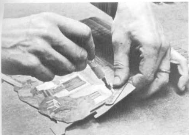
Sewing needle is used to make hole along line of cut. Jeweler's saw blade will then be fed through and mounted on the jig saw for cutting out.
