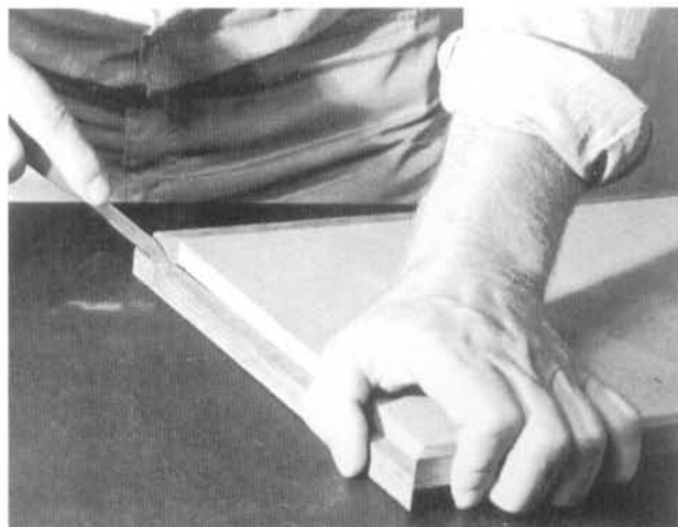
With the mitered lipping glued to the panel sides, use a marking knife to scribe the miters on the end lipping.
