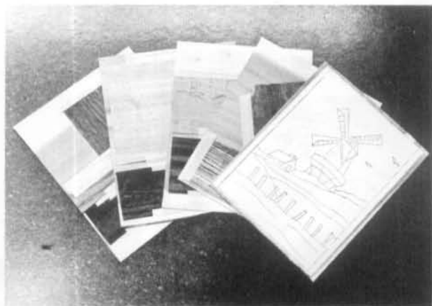
Photograph shows "pad" of veneers ready for assembly and cutting with pad method. Cross-sectional drawing shows how beveled saw kerf eliminates gap between pieces in double-bevel-cut method.
