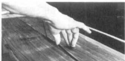
Saw through both veneers at once, carefully lift top sheet and peel away scrap beneath.
