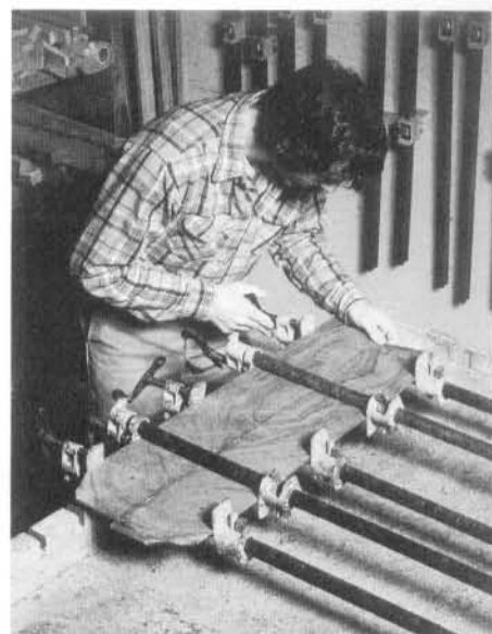
Thick veneers are stiff enough to be glued up just like boards. Flush up the show surfaces, and alternate clamps top and bottom so the leaves won't buckle.
