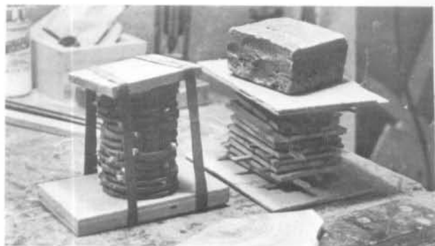
Branches sliced and stacked for drying. Weight, right, and strips of inner tube, left, keep oysters from warping.
