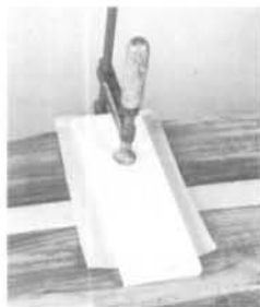
Block and clamp hold curly spot down while glue cools; strip of heavy paper along seam keeps it closed until glue dries. Then a sharp scraper cleans off paper and glue.
