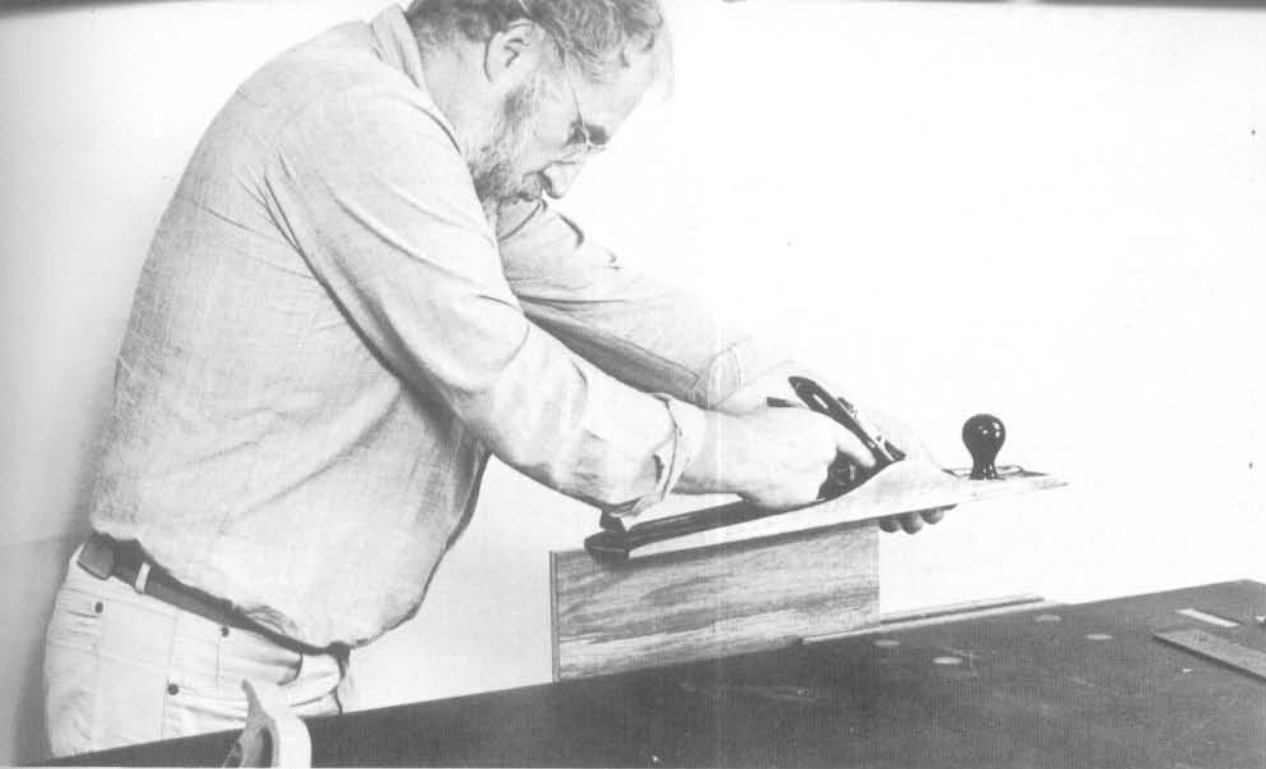
Finish the edges of the veneered panel with a jointer plane, after first trimming with a veneer trimmer, router or knife.
