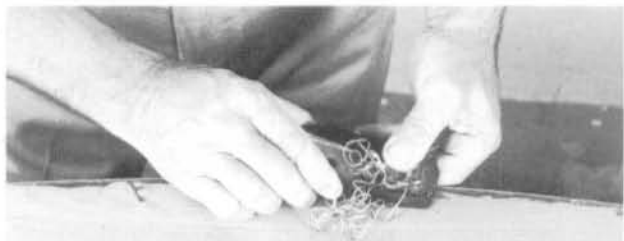
To trim a curved edge, let the glue dry hard, and plane.
