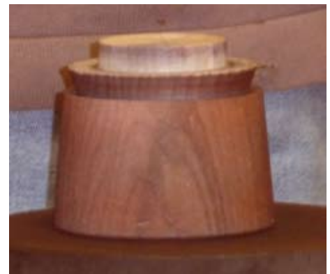
Figure 27. The finish sprayed box bottom portion is shown with the jam fit chuck still fitted to the opening.
