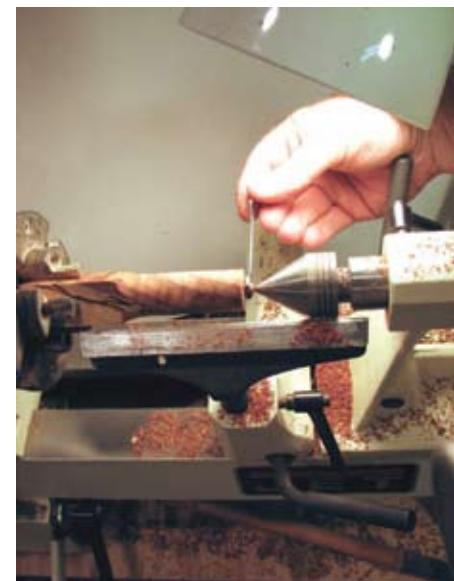
Figure 4. Sizing the tenon.
