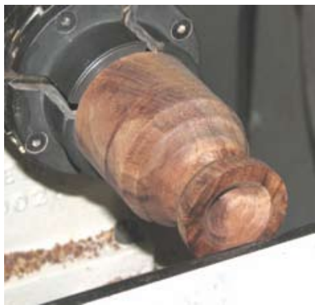
Figure 9. Central depression is turned to 15/16 inch deep.
