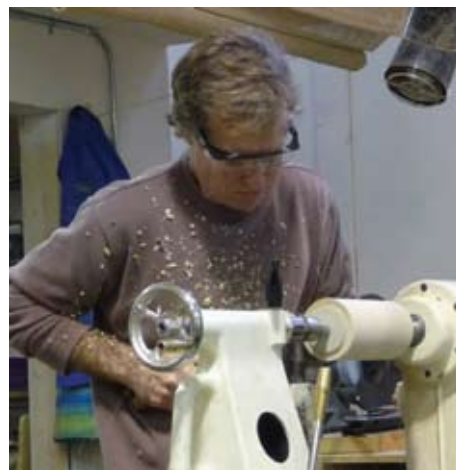
Figure 1. Matthew is turning tenons on each end of the center mounted chunk of wood that will eventually become a box.
