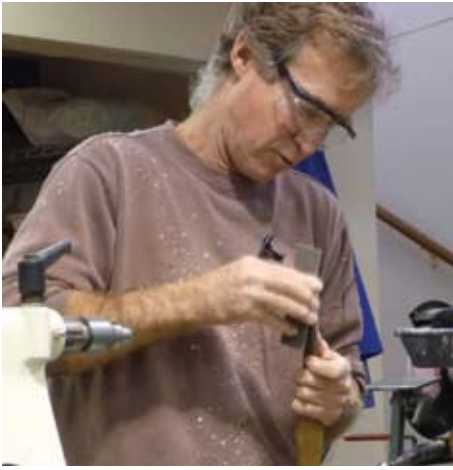
Figure 3. Here Matthew is honing the turning tool before proceeding. He did very little grinding of his tools during the demonstration, but honed them often with a diamond hone. He says that in his shop he uses a water stone. He prefers the Water stone to the diamond hones.
