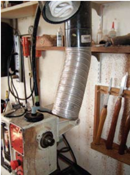
Andy's dust extraction system at the lathe.
