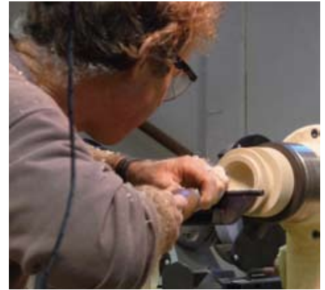
Figure 11. In this photo, Matthew is hollowing the inside of the lid using the Eliminator. He found this tool gave a better finish than either the Berger tool or the Oneway Ring Tool that he has been using for years.
