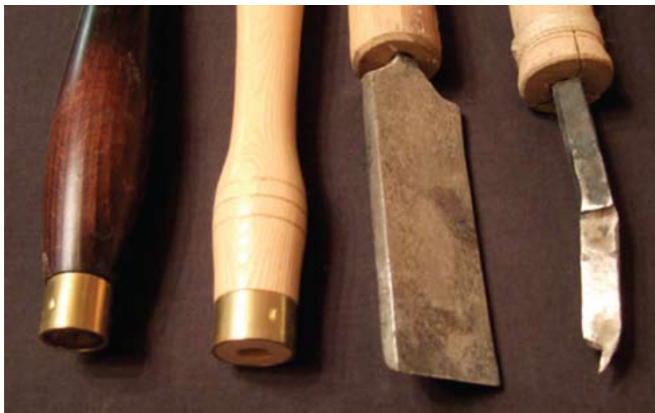
Figure 1. This photo shows 4 tools; the left two are commercial handles; note the tubings used and dimples to keep the ferrules in place. The wide scraper in an oak handle uses no ferrule, and the little hook tool, forged and ground from a stone chisel, shows a split handle "saved" by a string ferrule superglued (desperate maneuver, but still working after many years).
