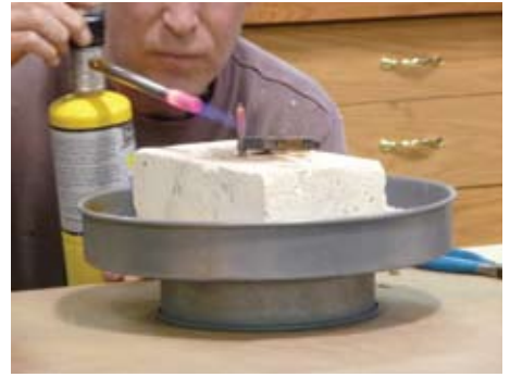
Figure 19. In this photo, Matthew is melting a bit of silver solder onto the tip end of a piece of brass.
