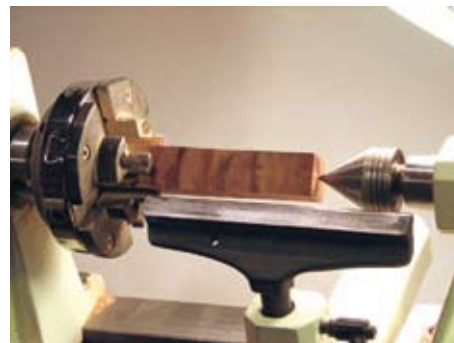
Figure 3. Starting to turn the handle of the scoop.
