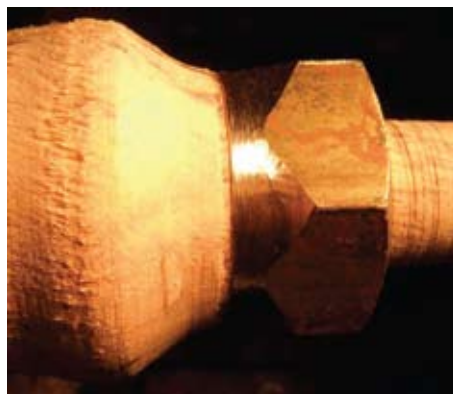
Figure 7. Brass nut turned half way.
