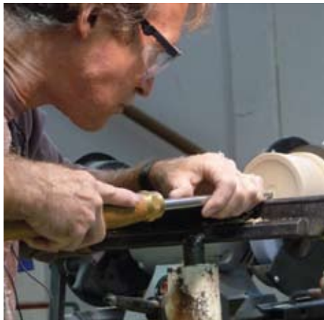
Figure 7. Matthew trued up the bottom and then hollowed it using the Berger tool. The hollow is only slight to make sure that the box sits on the outside edge of the box bottom.
