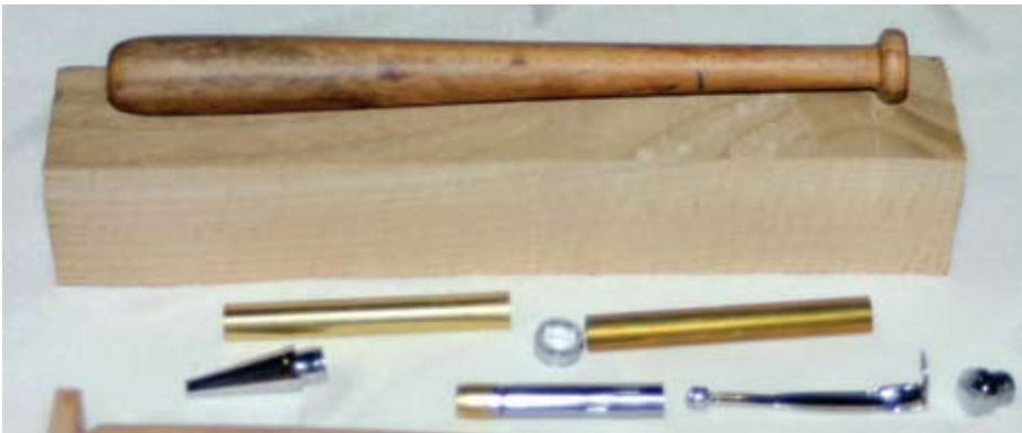
Figure 2. This photo shows the blank, the pen kit parts and a prototype baseball bat I once made for a model for the closed end bat pens.
