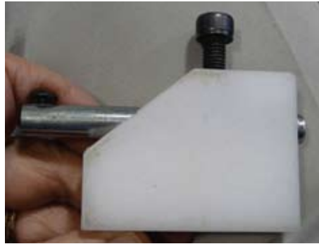
Figure 8. This photo shows the jig that Soren Berger sells to use in sharpening his tool.
