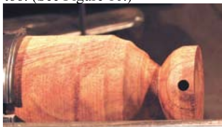
Figure 10. Hole drilled for handle tenon.
