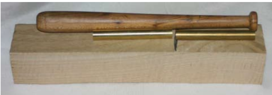
Figure 3. This photo shows the bat model on top of the blank with the tubes positioned the way I decided to use them.
