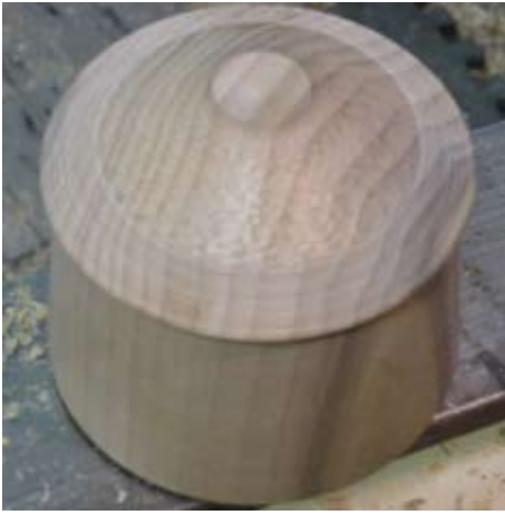
Figure 14. The finished turned box with some texturing done on the lid is ready to stain or color. The texture on the lid consists of some small beads in a section near the rim. The remainder of the top was textured with a rotary tool, simply touching the lid as the lathe rotated.
