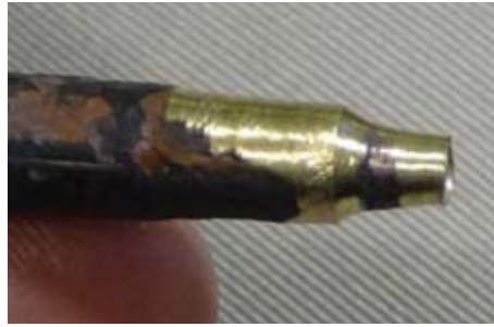
Figure 16. This photo shows one of his tips designed to burn dimples on the surface of the box.
