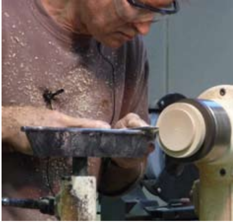
Figure 6. Matthew is now turning the tenon to fit the recess in the box. The box will be mounted on this tenon while he turns the bottom and will remain on while he does the texturing, coloring, and finishing.
