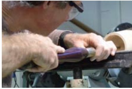
Figure 4. Matthew then hollowed the box using the Berger tool and had his introduction to Jack McDaniel's Eliminator tool, which he is using here. He has been using the Berger tool for a long time, but seemed to be impressed the Eliminator tool. He used a scraper to make a square area for the lid tenon to fit into.
