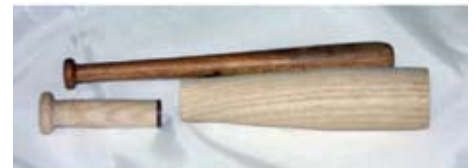
Figure 6. This photo shows the two roughed out blanks and the bat model.
