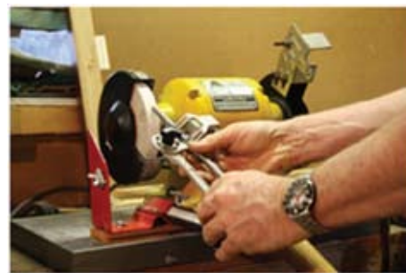
The Nova Sharpening Centre being used to sharpen a gouge.
