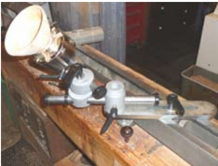
The Vermec Carving Mount fitted to my Nova DVR Lathe. The mounted bowl is being held with the Vermec chuck.
