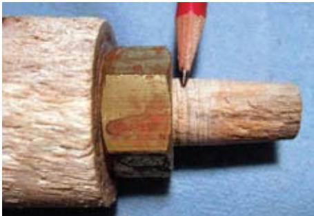
Figure 4. The nut has been screwed all of the way against the shoulder.
