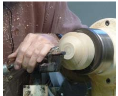
Figure 13. With the lid fitted into its jam fit chuck, Matthew final shapes the top of the lid. The pencil mark near the center is the size to which the lid top will be turned.
