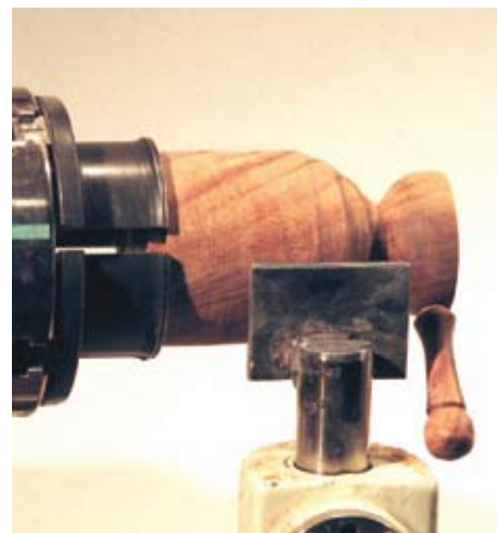
Figure 12. Small Tool rest to use for final turning of the bowl.
