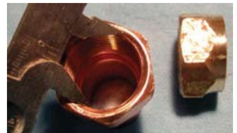
Figure 8. Determining the proper tenon diameter.
