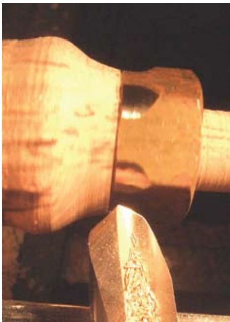
Figure 5. The nut has been partially turned round.
