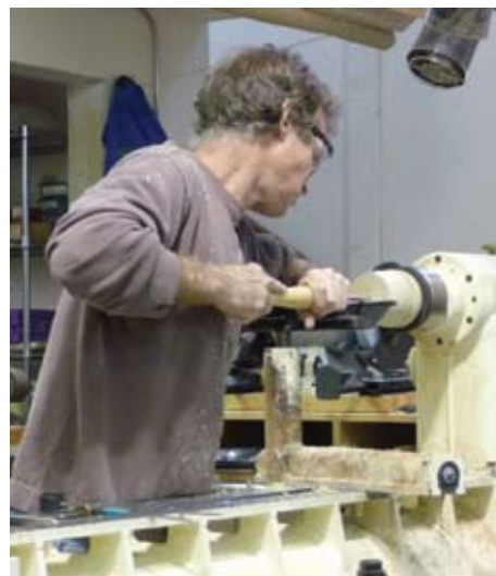
Figure 2. With the lid portion parted off using a hacksaw with the lathe running, Matthew mounted the bottom portion in the chuck and is truing up what will be the top of the bottom portion of the box.
