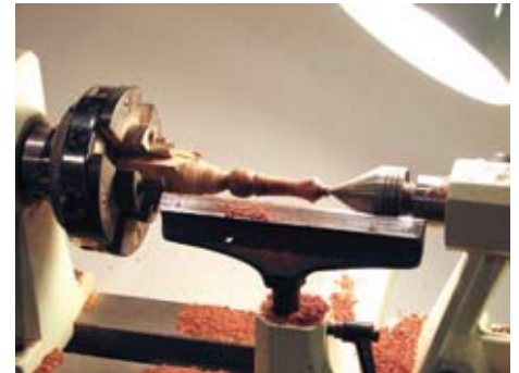
Figure 5. Finishing the handle shape.
