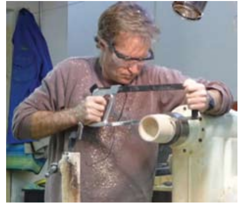
Figure 5. Here Matthew is parting off the box using a hacksaw with the lathe running. He is leaving an inch or so of material mounted in the chuck, which he will then turn into a jam chuck to finish the bottom of the box and to protect the inside while he sprays the wood with colors and finishing lacquer.
