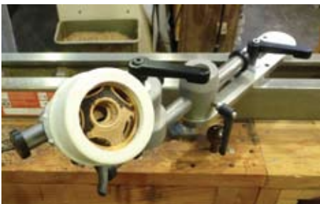
I mounted my Chinese Ball Chuck with a ball that I've been doing some burning on with my soldering iron.
