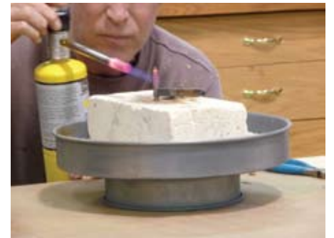
Figure 20. In this photo, Matthew is silver soldering the burning tip onto the rod that will fit into the soldering iron.
