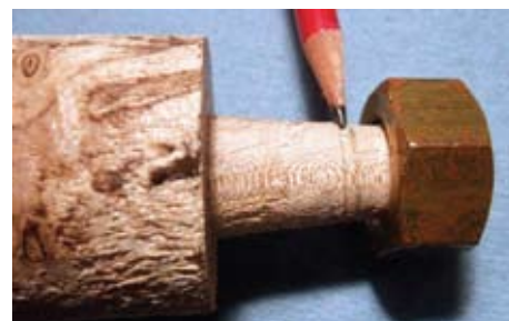
Figure 3. When the nut has been screwed on finger tight it leaves marks as shown by the pencil point.
