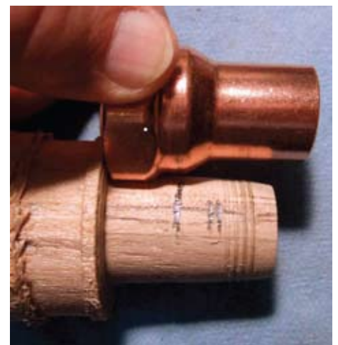
Figure 9. This photo shows the tapered tenon.
