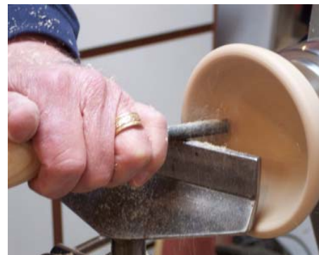
The 3/8" tool being used to hollow the inside of the bowl. There was a bit of tendency for this small tool to chatter.
