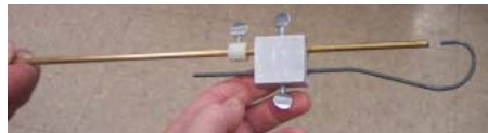
This is a wall thickness gauge that J. Paul Fennell uses when turning his hollow forms.
