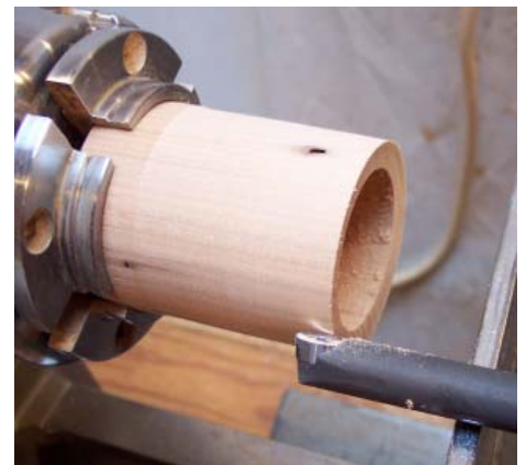
Cutting on the outside of the box.
