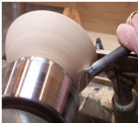
Turning the outside of the bowl with the 1/2" bar held in my Kelton tool handle.
