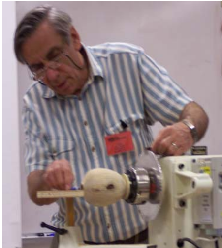
J. Paul Fennell laying out the pattern on a small hollow form.
