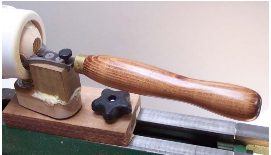
The swinging jig with a tool handle screwed to the swinging arm. The distance from the pivot point to the face of the tool handle is 1.25".
