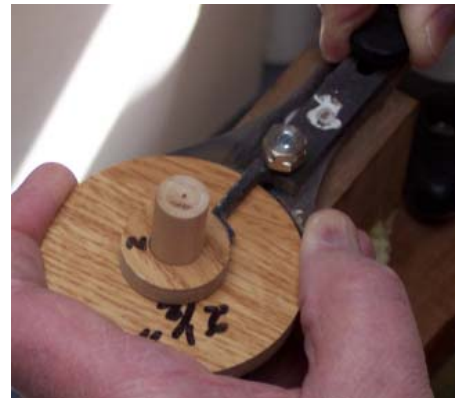
Setting the cutter and locking it down. The gauge has a 1/2" dowel in the center with disks to fit over it.
