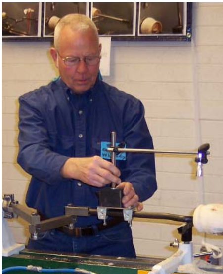
Magnetic base laser pointer mounted on the Elbo Hollowing Tool.
