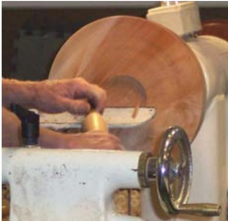
**Photo 6.** Although the center of the smallest bowl to be cored can be removed with the coring tools, Hal indicated that his experience was that it was easiest to simply turn away the center of the smallest bowl, unless the wood was a very expensive exotic wood that you would want to create a very small bowl to use all of the wood possible.
