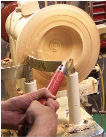
Photo 16. Starting the next core out. Using this system it is fairly easy to maintain the wall thickness of the cores that are being removed.
