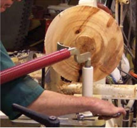
Photo 13. Hal started with a new blank that had been trued and had a foot turned for the chuck. In this photo, he is setting up the Oneway system. He is positioning it to remove the smallest core first. With the Oneway system, the cutter swings in an arc so that it is fairly easy to determine how deep the tool will cut and there is less danger of ruining the largest bowl.
