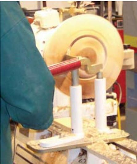
Photo 14. Here the coring tool is starting to cut the smallest core.
