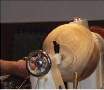
**Photo 3.** Here Hal has finalized the outside shape and is finishing the tenon (foot) that will be held in a chuck during the coring process. It is important that the foot on the bowl be at least three inches and preferable four or five inches on larger blanks. My experience with making only about two inch tenons is that they lead to disaster. Every 2" tenon I've used has resulted in a dismantled blank while coring.
