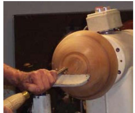
**Photo 11.** In this photo, the core from the previous bowl has been mounted on the lathe for truing up the outside and turning a new foot for this bowl.
