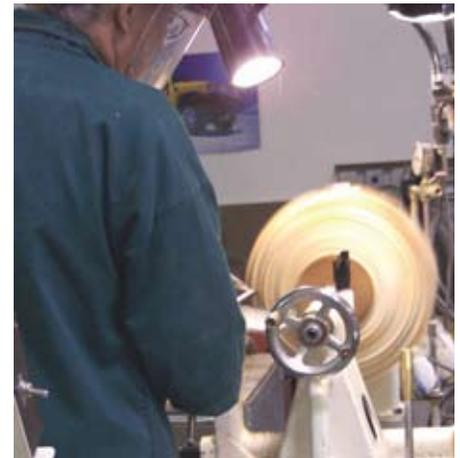
**Photo 2. In this photo Hal is defining the shape of the outside of the potential bowl. It is very important to turn the outside to near final shape before starting to core because this helps in the selection of which of the cutters to use for the first core. This is especially true if you are using the McNaughton Center Saver System.**
