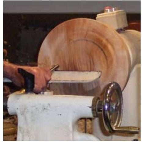
**Photo 5.** Truing the face of the bowl blank in preparation for coring. It is important for the face of the bowl to be smooth and flat for best coring operations.
