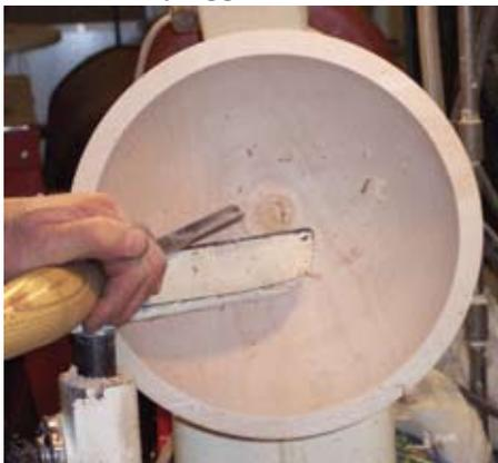
**Photo 21.** Carefully he makes the final cut to the center of the inside of the bowl. This is the cut in which you can tear out a chunk requiring additional passes to clean up the bottom, which can be very bad if you've already turned the wall thickness to the planned final thickness.
