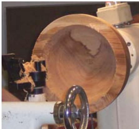
**Photo 9.** This photo was taken just after the core had been removed. Hal noted that he likes to clean up the inside of the bowl before removing it from the lathe and setting aside for drying.
