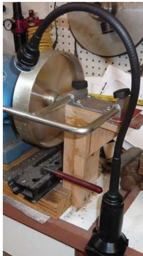
Figure 4. Work light being used to light the grinding wheel. This really provides a lot of light to see what you are doing when sharpening tools.
