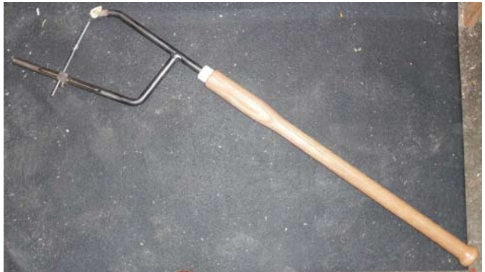
Figure 1. The Crabtree Hollowing Tool that Mildred and I tested has a 5/8" shaft and measures 39" from the tip of the support arm to the end of the handle. It is equipped with a small spring that helps determine wall thickness when hollowing.
