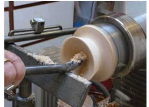
Figure 9. Practicing with the hollower for cutting the bottom of the vessel while I could see what the tool was doing.
