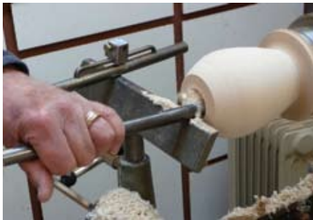
Figure 5. Beginning to hollow the vessel with the Crabtree Hollowing Tool.
