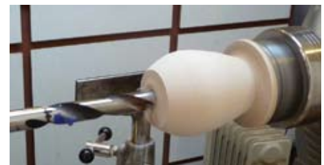
Figure 3. Enlarging the hole to about 7/8" with a Boeing Surplus drill.
