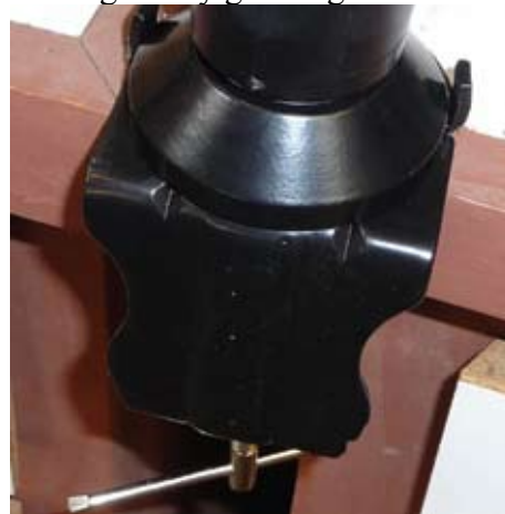
Figure 3. Close up of the metal clamp on mounting base for the lamp.
