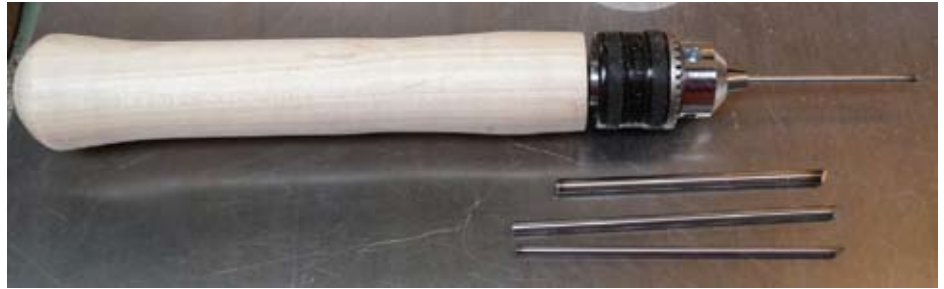
Figure 1. The Coving Tool comes with four different size coving cutters to make very small coves.
