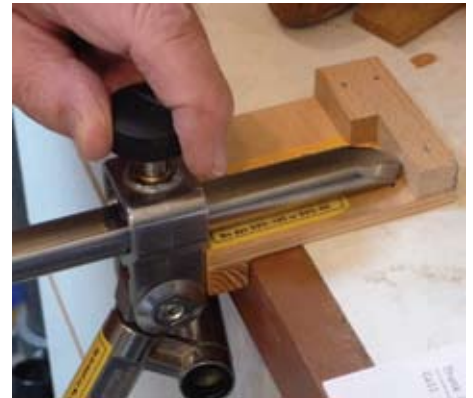
Figure 2. Setting the tool extension out of the Tormek tool holder.
