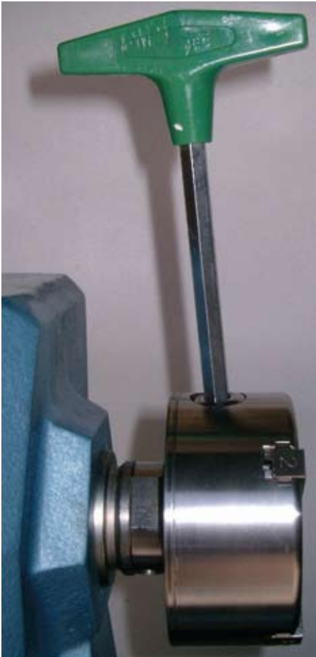
The chuck key is a regular metric size Allen key with a comfortable plastic T-handle.
