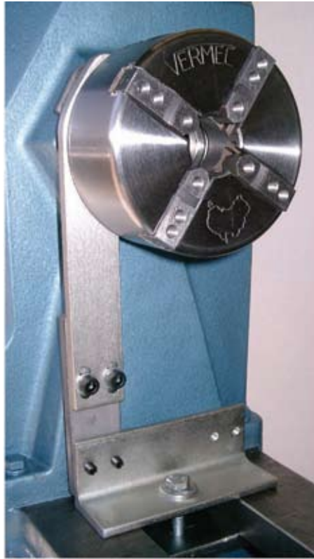
An optional item is an indexing fixture that has two pins to allow a wide range of indexing. I purchased this fixture also.
