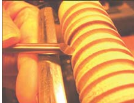
“Fig. 2-1: Refining the cove by moving left and right
