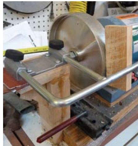
Figure 1. Mounting for a Tormek tool bar on my dry grinder with a 100 grit diamond wheel. The spacer block between the tool bar and the wheel is the same spacer block I use on the Tormek to set the wheel for doing the Ellsworth Grind on a 5/8" bowl gouge.
