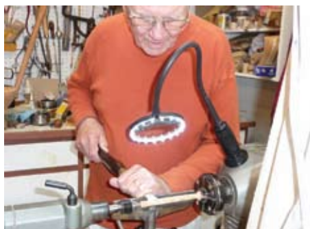
Figure 1. Work Light with the 5X magnifying lens being used while turning a pen blank.
