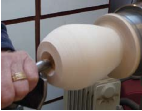
Figure 4. Enlarging the opening to make room for the tool to enter the opening.
