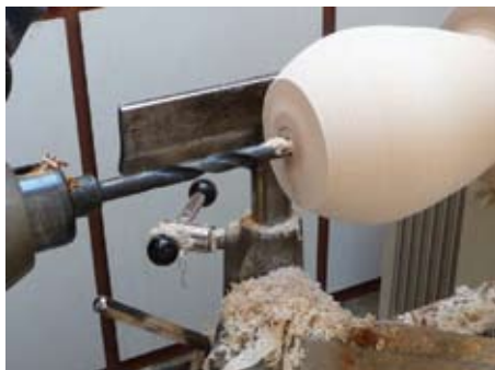
Figure 2. Drilling a 3/8" hole to depth with my new 3/8" drill with a Number 2 Morse Taper.
