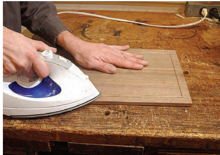
Ironing down the string. The glue may set before the inlay is in position. Heating the area with a household iron reactivates the glue for another try.
