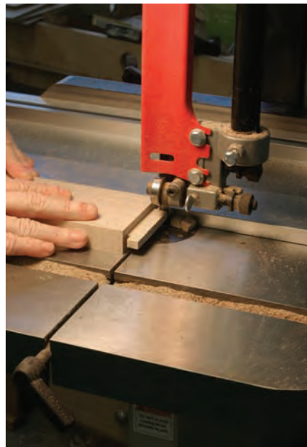
Careful now. Cut the remaining waste on the tenon at the band saw, being careful not to overshoot your mark. If you do, the resulting kerf will show on the front of the door.
