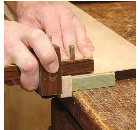
An efficient way to cut. With a simple jig and a marking gauge you can cut or rip string inlay easily.
