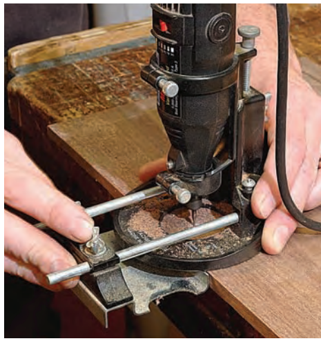
More power. You may want to speed the job along with a router or Dremel tool outfitted with a 1/16" end mill.
