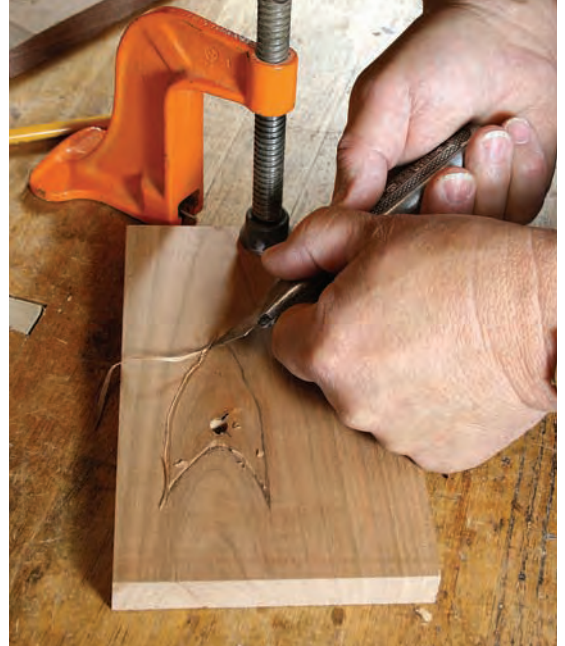
12 Relieve your knife line. Use a utility knife to make a relief cut all around the defective area in the scrap side.
