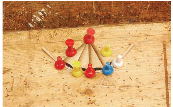
Push pin clamps. The curved stringing for the front edge of the fan is attached with white glue and held in position with push pins.
