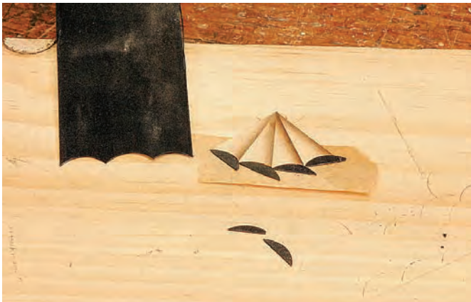
Tipping the ends. Black-dyed veneer pieces, cut with the same gouge, add another layer to the look of the fan.
