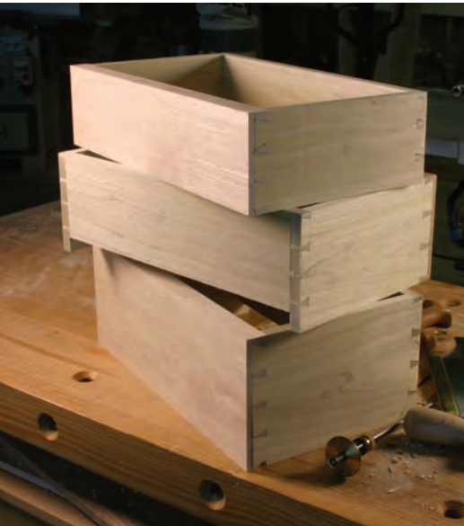
Stacked. Here, the finished drawers are stacked and waiting for drawer bottoms and the finish.
