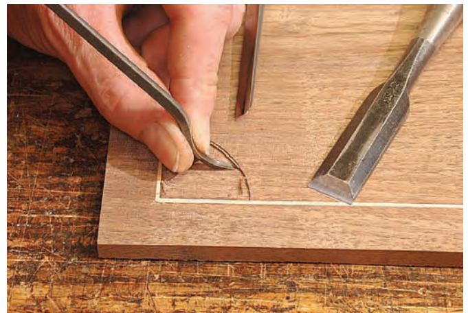
Preparing the recess. Once the recess is routed to the correct depth and close to the edges, remove the remaining waste with small chisels.
