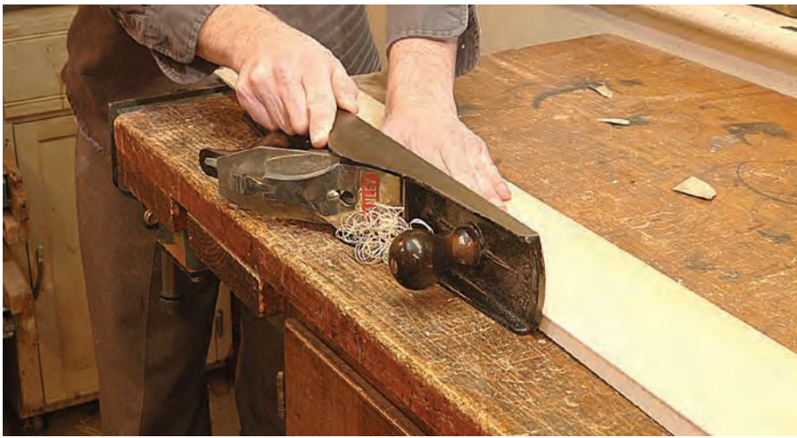
Edge cleaning. Shoot a straight edge onto the store-bought veneer before ripping the string.
