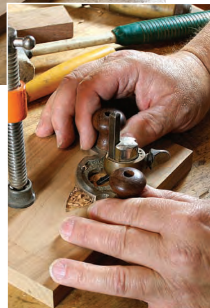
14 Hog out the waste. I use a butt-mortise plane (above) and a little router plane (right) to remove the bulk of the waste. The cutter on the router plane is about \frac{1}{4} " wide.
