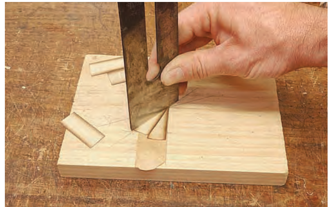
Building begins. After the plan of the fan is drawn full-size, use a plane iron to cut the shaded fan blades to size.
