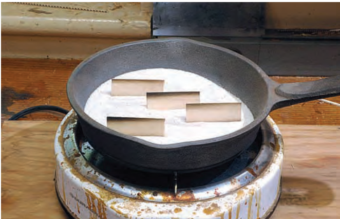
Shading takes skill(et). An iron skillet is the best way to shade the fan blades. Watch the process carefully to achieve consistent results.
