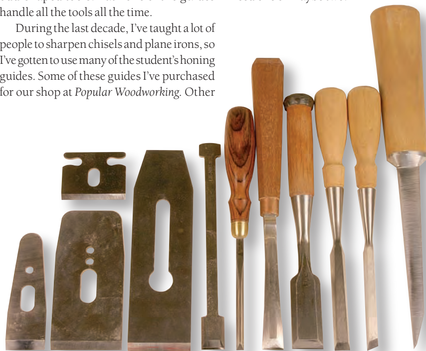
Many sizes and shapes. Here are some of the tools I sharpened (or attempted to sharpen) with the four honing guides. From the left: plane irons for a block plane, spokeshave, bevel-up smoothing plane, bevel-down smoothing plane and shoulder plane. The chisels include: a dovetail, fishtail, Japanese, bevel-edge, skew and mortising tool.
