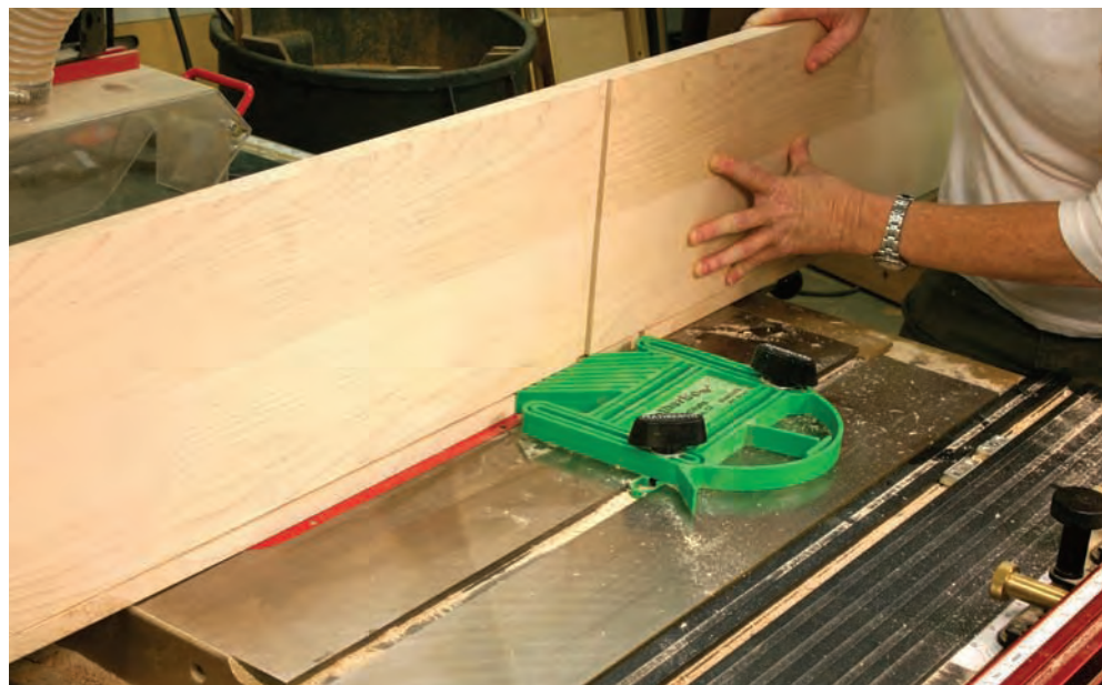
Two-step. This two-step rabbet cut is made more secure and safe by using a featherboard to help hold the workpiece.
