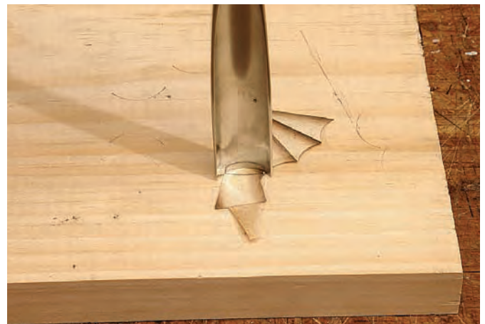
Gouge the ends. Use an appropriately sized gouge to create the scallop at the end of each blade.
