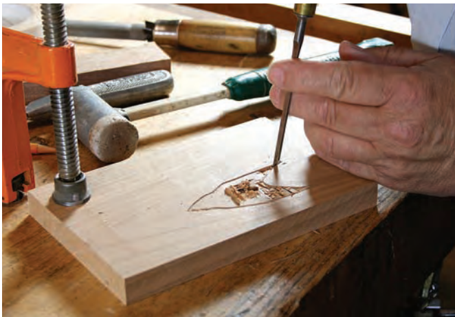
13 Chop and pare. Chop out the waste with a chisel. The size of the repair dictates the width of the chisel. Use a \frac{1}{8} " chisel in the tight corners. At tight points, lay the chisel on its side and use the point to remove material.
