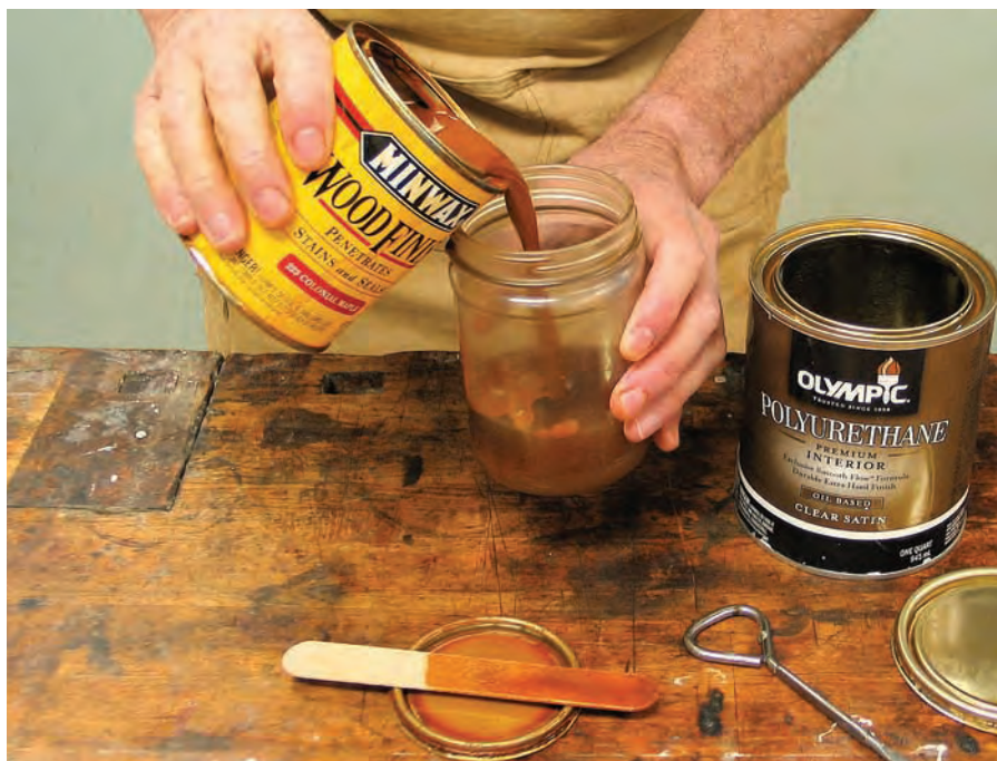
Mixing liquids. Just as all finishing products that thin with water can be mixed, so can all finishing products that thin with mineral spirits (paint thinner). Here I'm adding some stain of one brand to some polyurethane of another to make a "varnish stain," a stain that can be left a little thicker on the wood or over another coat of finish.
