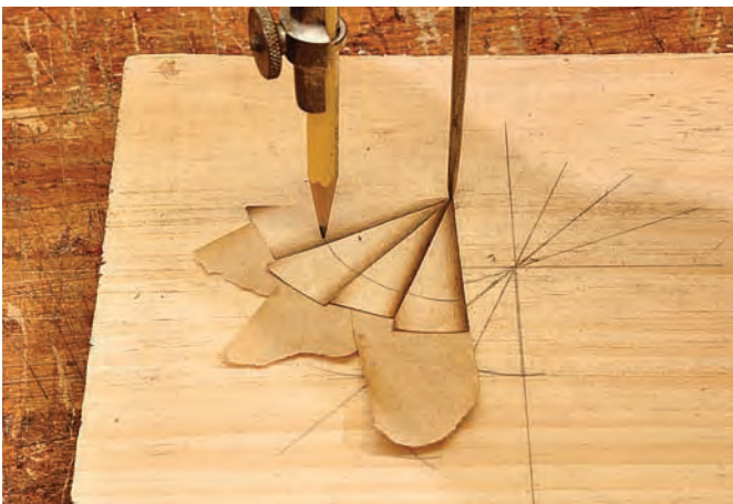
Mark the arc. A compass marks the outer edge of the fan, which is held together with veneer tape.
