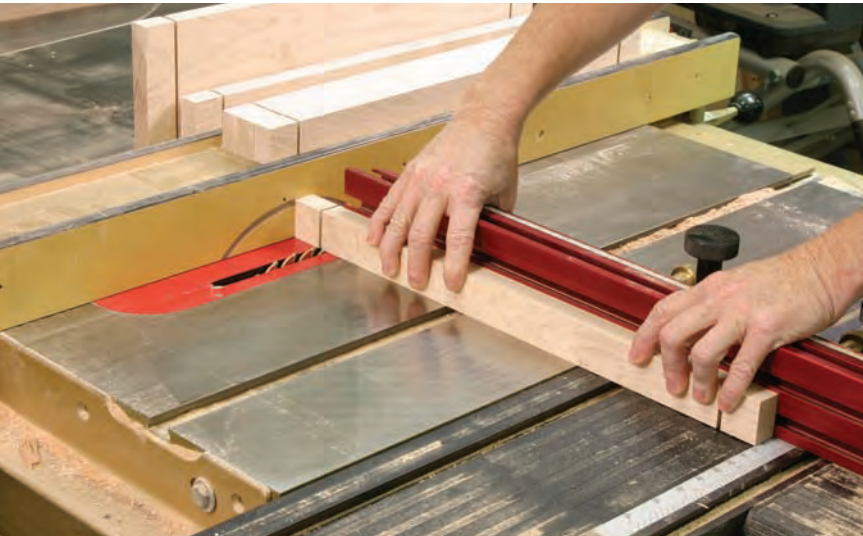
Rolling shoulder cuts. Make all four cuts on one end of each rail at the table saw, using a sled or sliding table.
