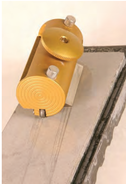
Roll with it. The SharpSkate hones your tools side-to-side, which allows you to work all the corners of your stones, even to work off the stone if you like.
