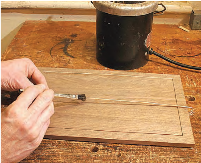
Inlay installation. Add hot hide glue to the stringing then fit the inlay into the recess. Use a veneer hammer if you need to persuade the stringing.
