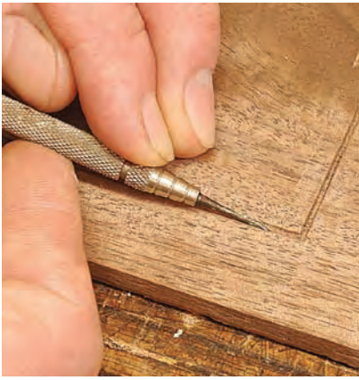
Flat bottoms. Remove the V-shaped bottom of the inlay area. A sharpened eyeglass screwdriver makes a great tiny chisel.
