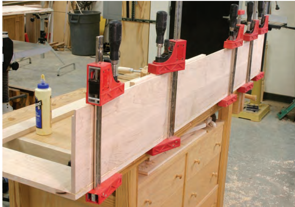
Taking sides. Make sure everything is lined up flush before tightening down the clamps. Secure the ends first, then adjust as necessary through the middle to compensate for any slight bowing.
