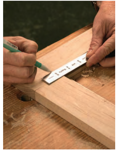
Square your corners. Use a 6" rule to extend the line of the rabbet, then clean the corner square with a chisel.
