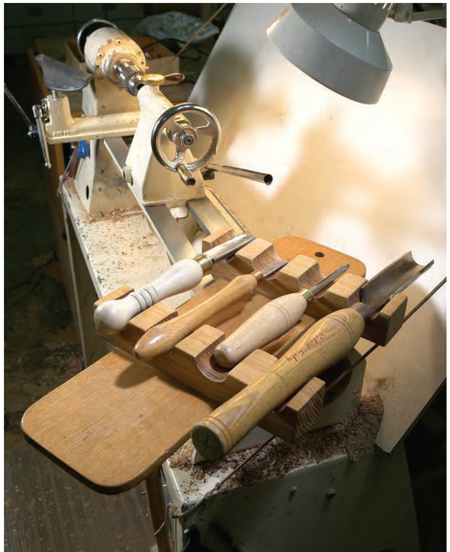
In easy reach. This is the tool holder I nearly always use now when I turn. It sits on the far right of my lathe bed. The tools are easy to see and pick up, and they stay in place when I put them down.
