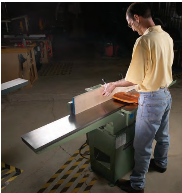
Bad stance. This is the wrong way to stand at the jointer. My mobility is greatly limited and I can trip myself.
