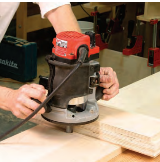
Shelf groove. Set up a straightedge jig to guide your router through your shelf-groove cut.
