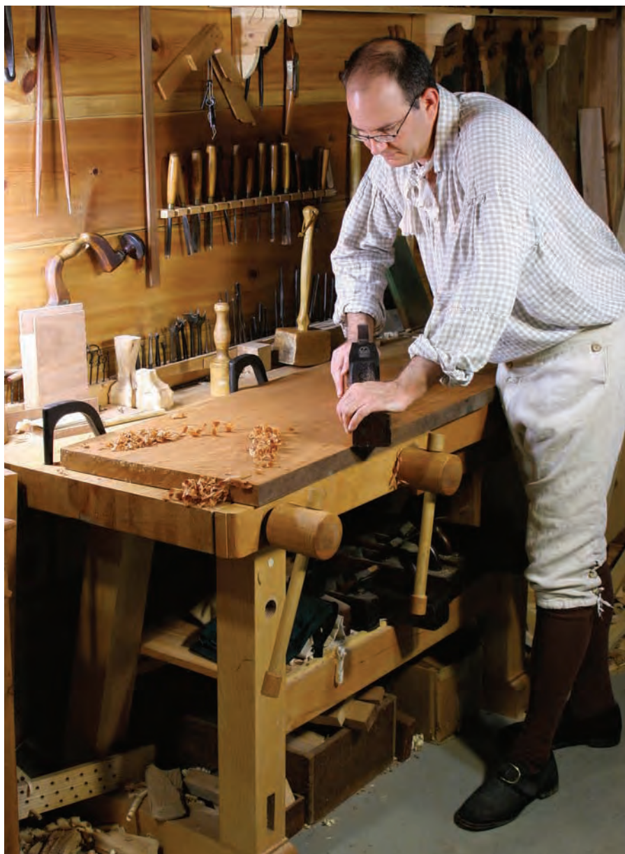
Eighteenth-century woodworking tools. This 20"-wide piece of mahogany will make a great tabletop when I get it flattened. My long try plane may not be the fastest tool for the job, but I sure am glad I have it. I could never justify purchasing a 24" stationary power planer because I come across stock like this infrequently. This plane allowed me to buy a piece of wood I probably couldn't work otherwise. Eighteenth-century woodworking tools can be restrictive in some ways. In this case, however, my try plane has opened up opportunities I wouldn't have had without it.
