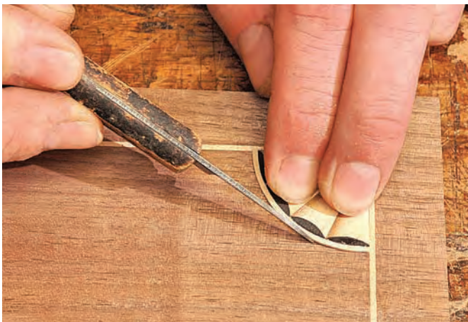
A fine line. Carefully cut a line for the fan inlay after the piece is trimmed and final shaped.
