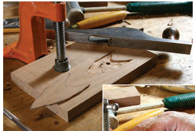
14 Hog out the waste. I use a butt-mortise plane (above) and a little router plane (right) to remove the bulk of the waste. The cutter on the router plane is about \frac{1}{4} " wide.
