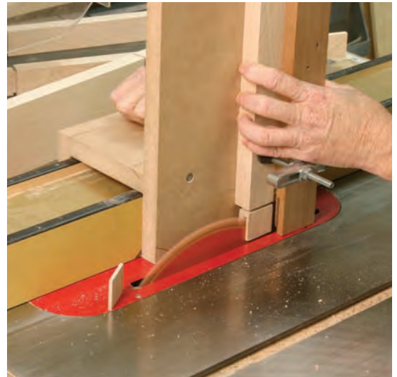
Tenon jig. This tenon jig keeps the workpiece secure as you cut off the cheeks of your tenons.
