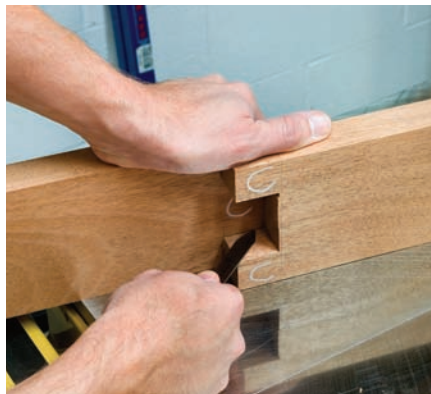
Marking, not measuring. Transferring the lines of the finger joints from one piece to the other guarantees the fingers will match.
