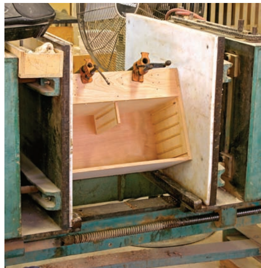
One mighty clamp. Custom presses are used to clamp assembled cases. Similar presses are used for assembling drawers.
