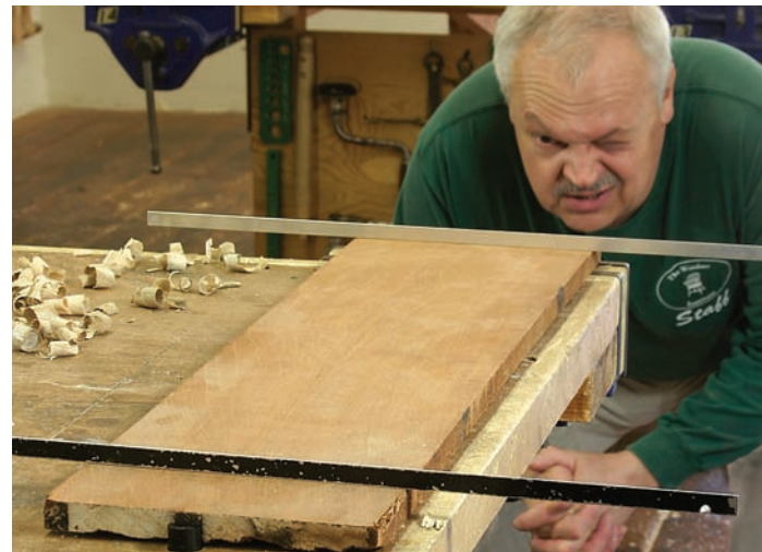
Sight lines. Winding sticks can be used to confirm if a board is flat — or to help identify high spots.
