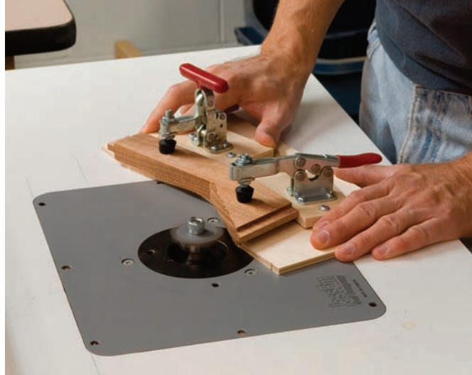
Grooving along. This fixture guides the sunburst stile against the bearing on the router bit and keeps hands at a safe distance from the cutter.
