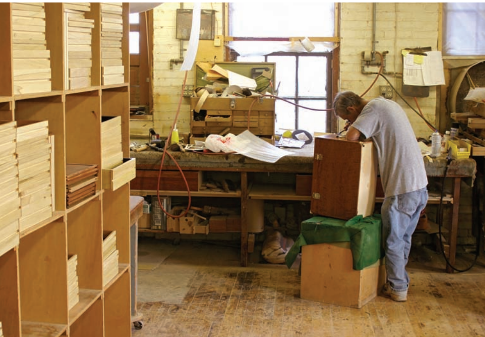
Still on the job. The fit of drawers in finished cases are checked a final time, and the finish is touched-up before packing. Employee Walter Rickard has worked for Gerstner for 19 years.
