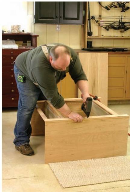
Get your face on. Check the fit of the face frame. If everything is correct, add a bead of glue to the case's front edge and position the frame on the case. You can add clamps if you like, but brads should hold the frame tight.
