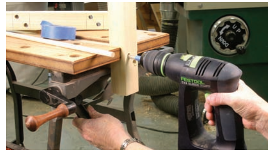
Drill straight. As you drill through the foot into the bottom of the upright, keep your drill level.
