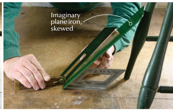
On the diagonal. As you can see in these pictures, moving slightly at a diagonal across a surface actually presents a lower angle of attack, and helps prevent tear-out.
