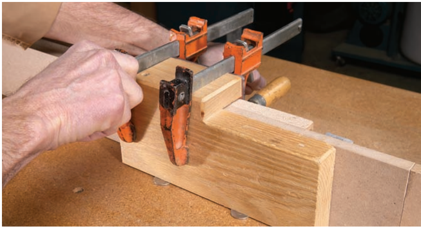
Two clamps, two coins. I always double-clamp my stop to keep it in place in case my work gets kicked by the saw. The coins (removed after clamping) raise the stop to help with dust removal.
