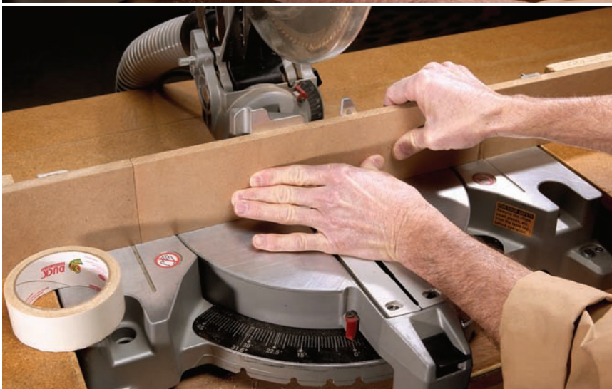
Stuck, secure and super-accurate. I install replaceable sub-fences on my miter saw to control tear-out and increase my accuracy. Here I'm installing one with exterior-grade carpet tape (top). Then I simply press it into place (bottom).
