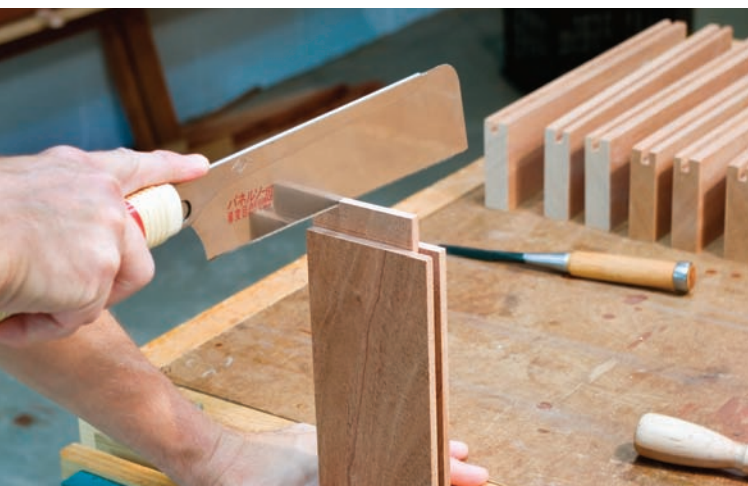
Handcut haunches. A haunch is cut in the tenon to fill the end of the groove, providing greater strength and a neater appearance.
