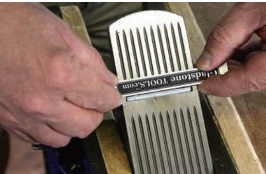
Almost imperceptible. A smooth plane has such a slight crest on the cutter that it's almost imperceptible, even with a straightedge held against it. This plane leaves a surface smooth to the touch.
