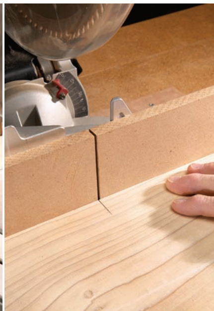
One slice to accuracy. With the sub-fence installed, I'll make a straight cut into it (left). Now I know exactly where my saw will cut when crosscutting my stock. I simply line up the mark on my board with the kef in the sub-fence (right).
