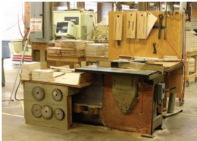
Purpose-built and still on the job. This custom-made machine cuts drawer sides to length, and puts a groove in each end with one stroke of a sliding table.
