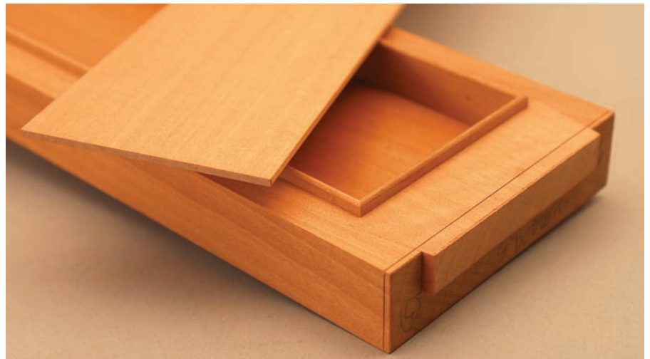
See the sawn details. Above is shown a sample of thin solid veneer. In this case it has been used for a small box lining in one of my student's work.
