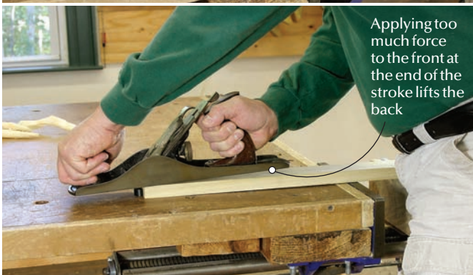
Rocking. Improper application and shifting of weight causes joint edges to bow, and flat surfaces to be out of uniform thickness, as shown in the two pictures above.
