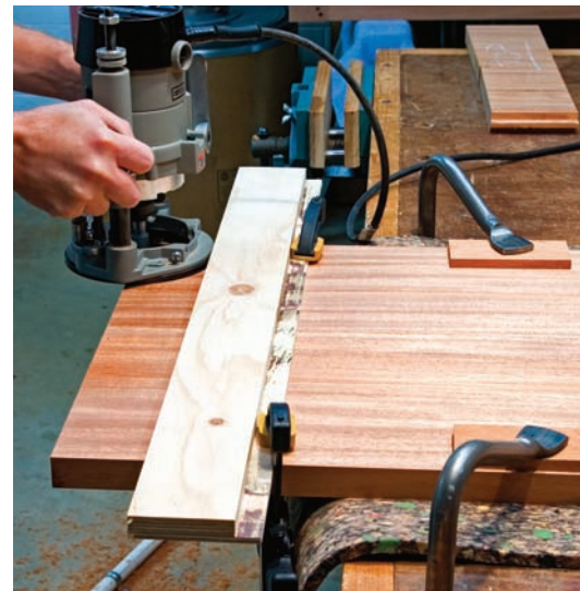
Tip of the tongue. The wide tongue is created with a \frac{3}{4} " router bit. The straightedge clamped across the top serves as a guide.
