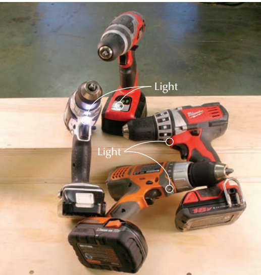
You can see in the dark. LEDs are common on many of the tested drills. Most are just above the trigger, but the more useful light, found only on the Skil, is mounted at the drill's base.
