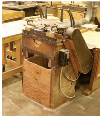
Purpose-built and still on the job. This custom-made machine cuts drawer sides to length, and puts a groove in each end with one stroke of a sliding table.
