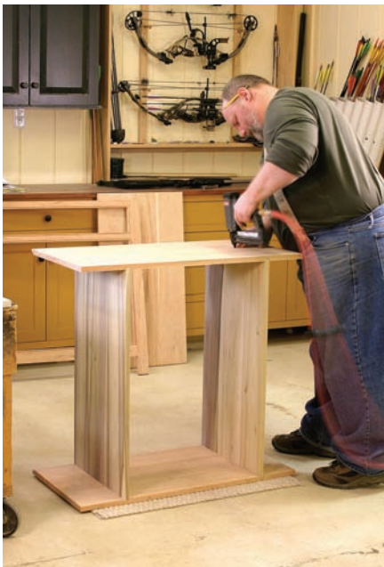
A simple connection. What could be easier than connecting the sides to the shelves with brads? Drawing a line at the center of the joint provides a nailing location and translates into efficient work.
