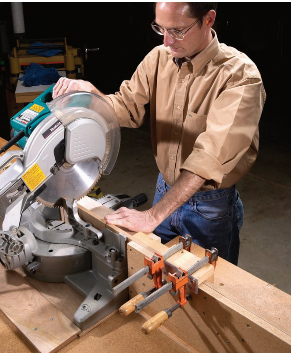
Ready for a good cut. Here is a proper setup for a good crosscut. Note that my stop has two clamps, which ensures it will stay put if the work gets kicked about.
