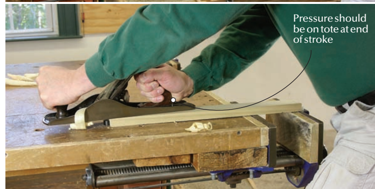
Left to right. To get a level surface, start with with pressure on the knob of your plane, apply pressure evenly through the middle of your pass, then shift the pressure to the tote as you come off the end of the board, as shown in the two photos above.
