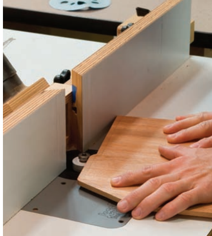
Rounding rabbets. The backs of the panels are rabbeted to fit the groove in the stiles and rails. Because of the cloudlift, a bearing-guided bit is used to follow the profile of the panel.
