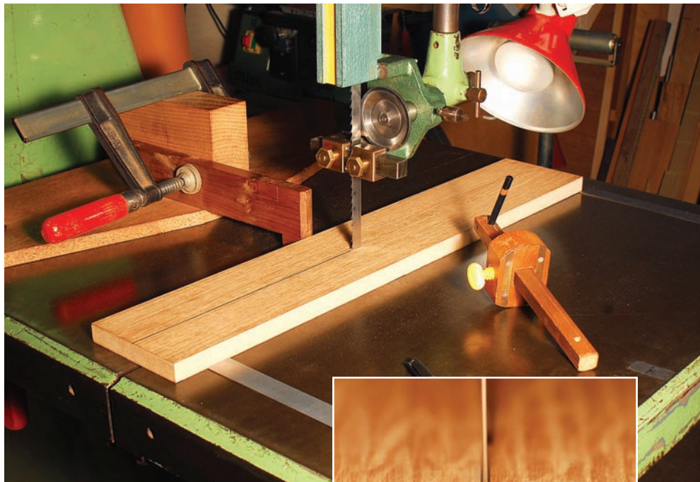
Getting the drift. Establish the correct feed angle with a point fence, a parallel-sided workpiece and a line from a pencil gauge. Experiment with the feed angle until the back of the blade is centered in the saw kerf (right).
