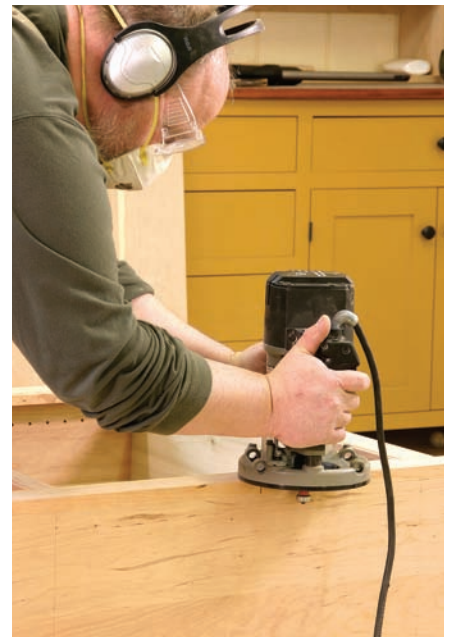
Trimming the fat. The extra 1/16" added to the face frame stiles ensures the frame overhangs the sides of the case. Any remaining material must be removed. A flush-trim router bit with a bottom-mount bearing is the perfect solution.
