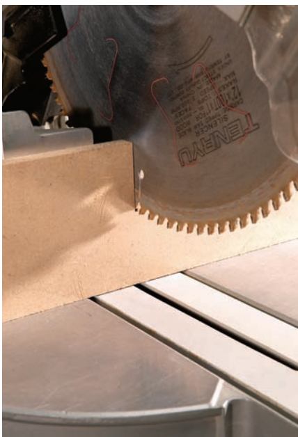
One slice to accuracy. With the sub-fence installed, I'll make a straight cut into it (left). Now I know exactly where my saw will cut when crosscutting my stock. I simply line up the mark on my board with the kef in the sub-fence (right).
