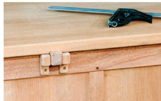
Handsome hinges. Shop-made wooden hinges, mortised to the top and screwed to the back, reflect the finger joints in the base.
