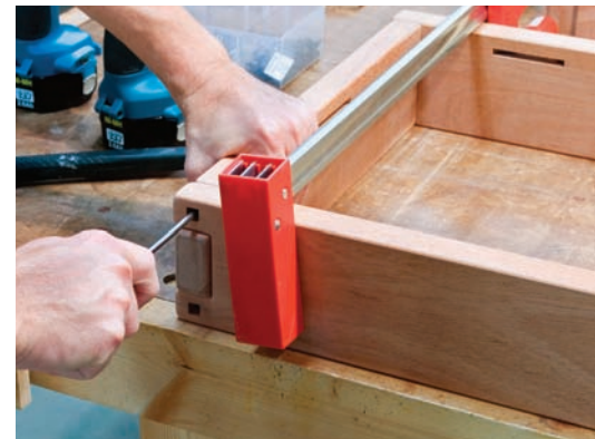
No glue on the fingers. The corners of the base are screwed together – a corner block will be glued in later from behind the joint.
