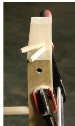
Drill straight. As you drill through the foot into the bottom of the upright, keep your drill level.
