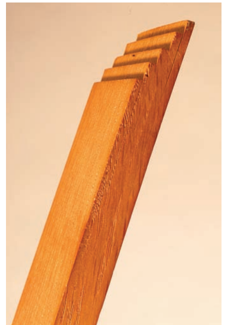
Cut then curved. This example of curved, tapered lamination in English oak shows how the glue lines can virtually disappear. They only become visible near the end, in the waste piece, where the clamping pressure was not adequate.
