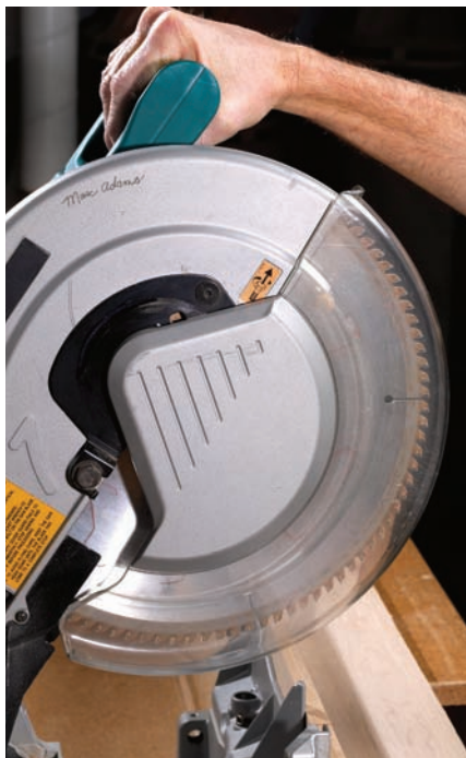
Lots of exposure. Since power miter saw manufacturers added the compound-cutting feature, the guards have had to expose the user to the blade more. Note how much blade is evident as the motor carriage is pulled down. It goes from fully covered (left) to fairly exposed (right).
