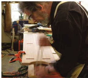
Getting in shape. After cutting the lower arch with a jigsaw, the curve is smoothed with a rasp.
