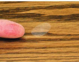
Sticky stage. Once the bubbles have popped out, you want the polyurethane to dry as fast as possible to get beyond the sticky stage (demonstrated here by a fingerprint in the finish) so dust nibs are kept to a minimum. Adding faster-evaporating naphtha to the finish doesn't speed the drying of this stage beyond what is accomplished simply by the thinning. You could just as well use mineral spirits.
