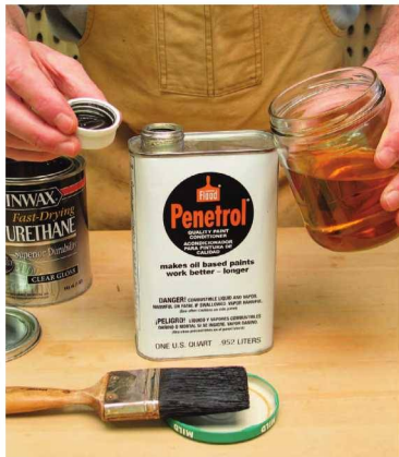
Penetrol. Adding Penetrol (a widely available additive for oil paint) to polyurethane slows its drying so dust has more time to settle and stick to the finish. Any possible gain in reduced brush marking is more than cancelled out by the added dust nibs.
