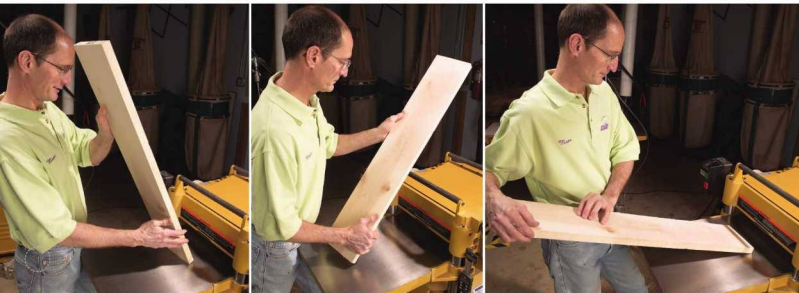
Flip after each pass. It's good practice to remove material from both faces of your work (once both faces are planed flat). To keep your board's grain direction oriented correctly, flip each board end-for-end after each pass.
