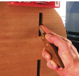
Marked in place. The tenons are marked directly from the mortises, ensuring that the locations match.
