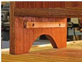
Simple enough. Maple runners below the bottom shelf support and guide the hidden drawer.
