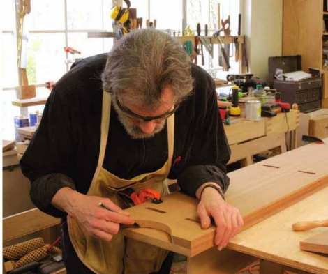
One side makes another. After the curves on one side are completed, the first side is used as a template to make the second side.
