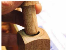
Square parts, turned tenon. The leg-to-foot joint should be snug with even shoulders all around.
