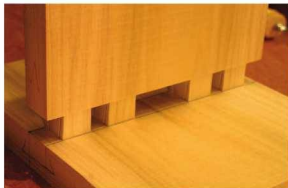
Test run. Do a dry fit (without wedges) to ensure the pieces fit snug, and clean up your cuts as necessary.
