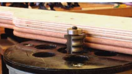
Along the curve. A plywood template is used to guide a reeding bit along the serpentine edge of the gallery.
