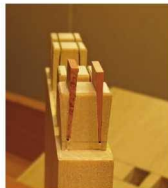
Don't split. The wedges spread the tenon to fill the flare of the mortise.
