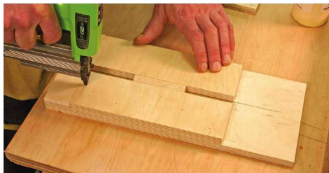
Built around the holes. This jig for the through-mortises is made by assembling small pieces to a backer. The openings are then cut with a router and a locating fence is added.
