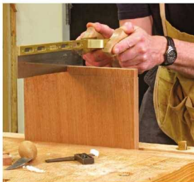
Ends second. The ends of the tenons are cut by hand, then the waste in between is removed.
