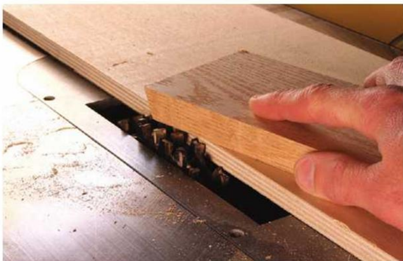
A brush with flushness. To set the dado stack so it is exactly as high as the top of the jig, rub a piece of your work over the knives. The knives should just brush the work.
