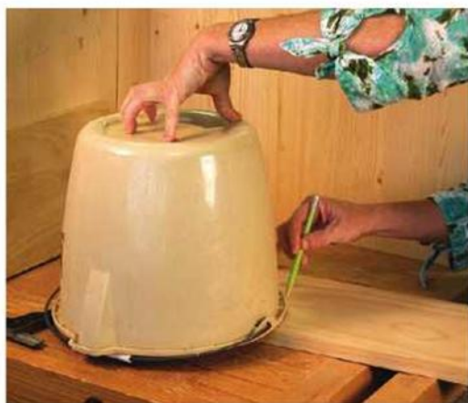
What's on hand. You don't need a compass to draw an arc. Just grab whatever's handy around the house. I used a bucket with an 11" diameter to its outer rim.
