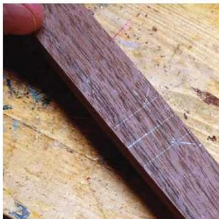
The miter’s mate. This photo shows the layout of the joint’s female part. The marks on the right edge of the moulding indicate the full width of the male moulding while the marks at the left-hand side of each diagonal indicate the width of the central raised portion of the male moulding. Staying clear of the layout lines, I cut the joint on my band saw.
