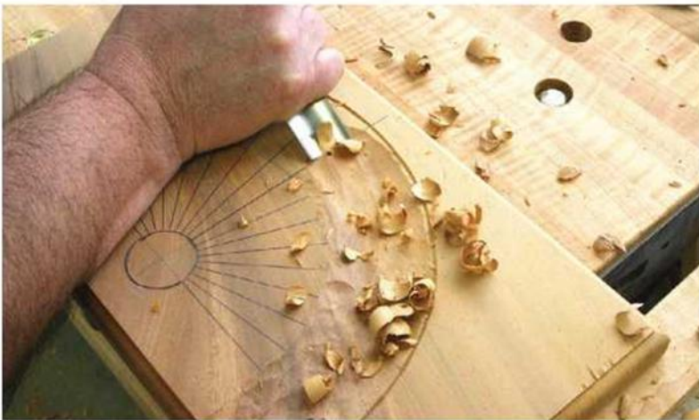
Work between the lines. The addition of the inside layout line, along with the depth-setting holes, allows you to create a level and symmetrical trough.
