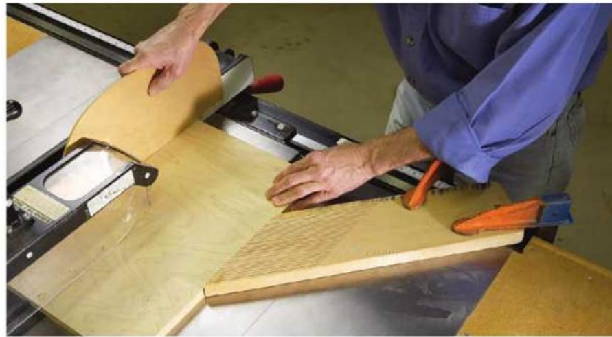
Better together. Here a push stick is used with a featherboard. The push stick keeps the work flat on the table and moving forward. The featherboard, located in front of the blade, presses the work against the fence.
