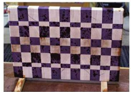
Travelin' through. The varnish travels through the grain and seeps out on the other side. Once it starts to soak through and you've coated both sides, let it dry in this position overnight.
