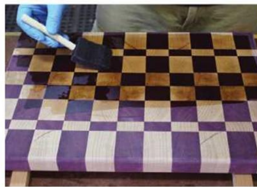
Quick work. The varnish quickly soaks into the end grain.
