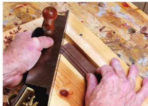
Shooting to size. I rough cut the miters on the male part with a saw, then finalized the miter with several strokes of a miter plane on a shooting board. The miter is finished when it just meets the central raised portion of the moulding.
