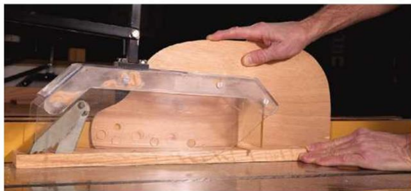
A good push stick. Here's one of my frequently used push sticks. It hooks over the back of the work and presses the work flat against the table.
