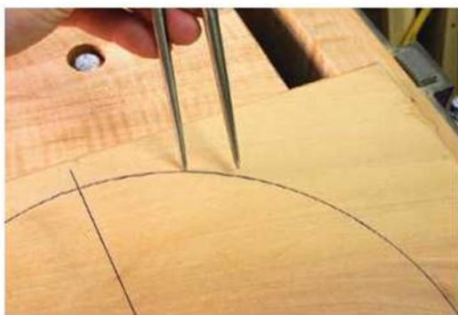
Stepping out. Symmetry is important, so it's best to lay out the ray sizes with a set of dividers.
