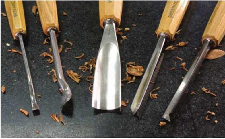
A short list. You don't need a tool chest full of carving tools to make this fan. Three gouges and two parting tools are all that's required.
