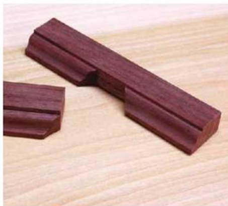
Double your precision. The partition mouldings enter the bottom moulding with the double-miter joint shown here. The same joint is used when the middle shelf mouldings enter the partition mouldings.
