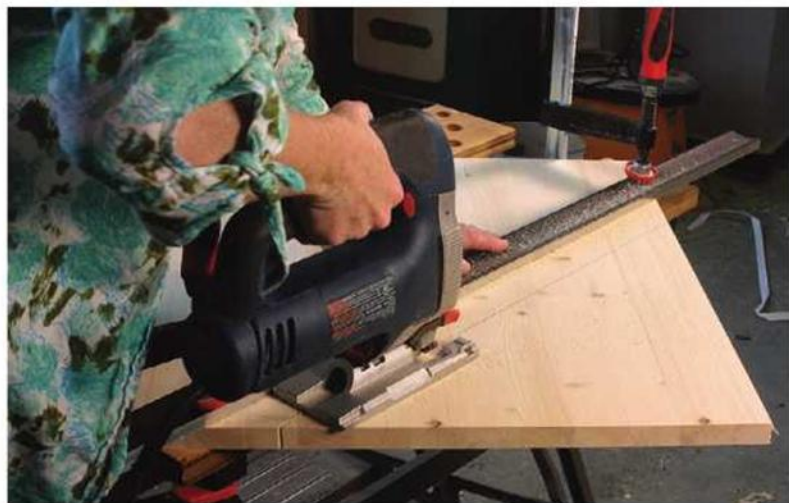
Straightedge jig. A straightedge with a beefy edge makes a good guide for making straight cuts with a jigsaw or circular saw.
