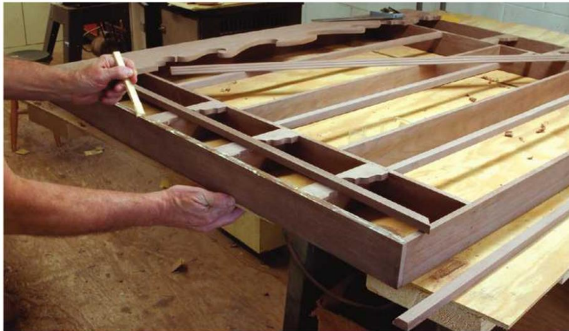
Where glue helps. Glue adds little strength to a dado joint so I assembled them unglued, but whenever I had a chance to glue side grain to side grain, I used glue as I’m doing here with this moulding.
