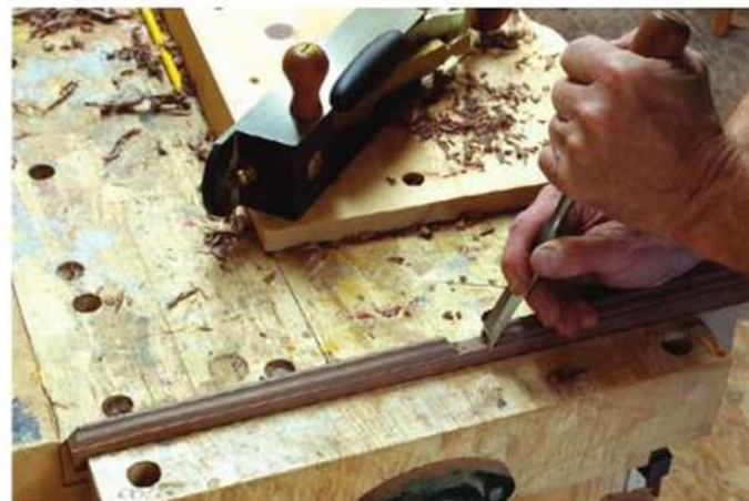
Pare to fit. I then fine-tuned the female part of the joint with a paring chisel, giving the part several test fittings.
