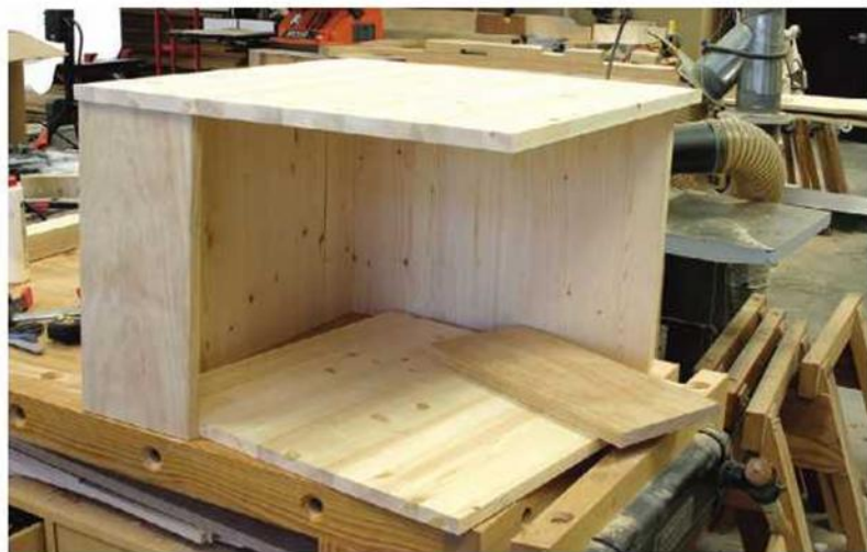
Cut to size. Cutting your top to size first allows you to easily fit everything that goes under it, even if you change the dimensions to suit your specifications.
