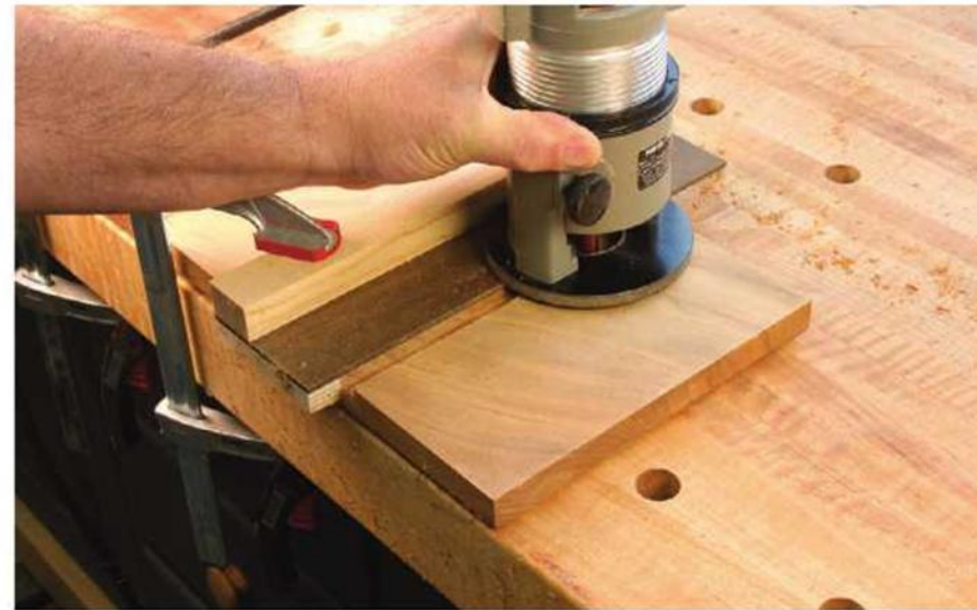
No guesswork needed. Once built, the jig is a snap to align with layout lines; hit the mark every time.
