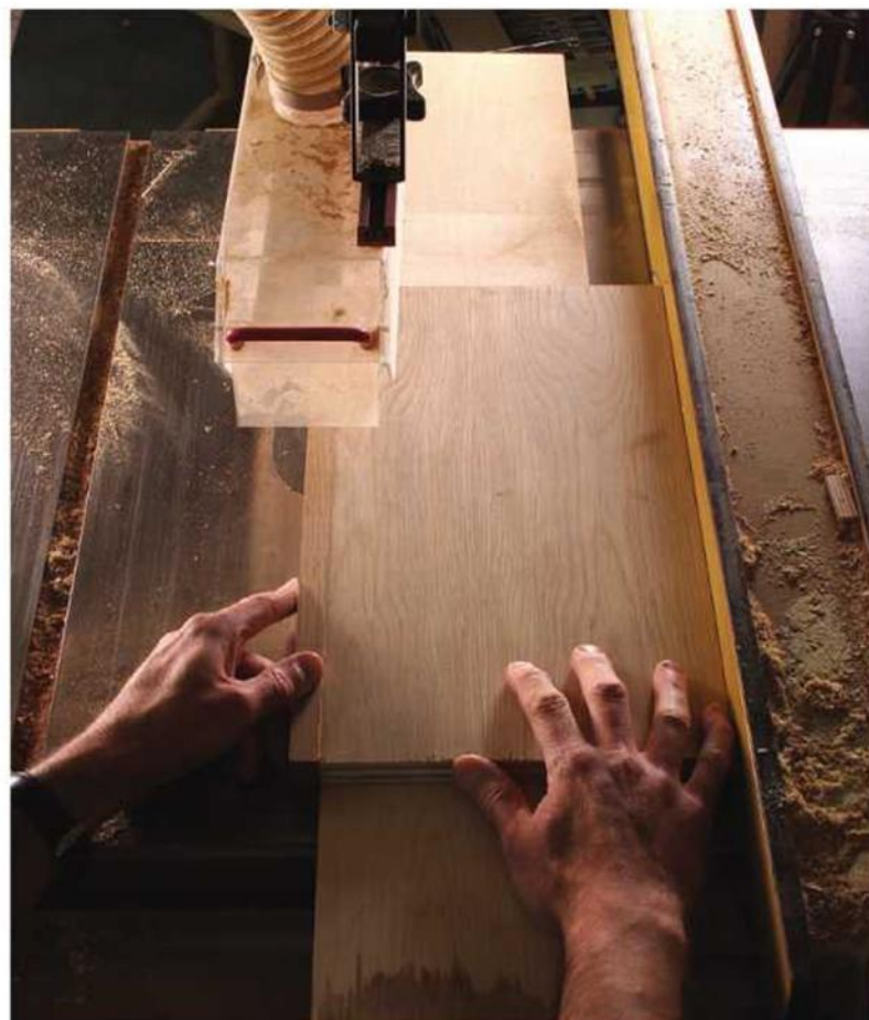
Safe and accurate. One of the things I really like about this jig is that you can push the work flat over the blades, plus you can use your basket guard for added safety.
