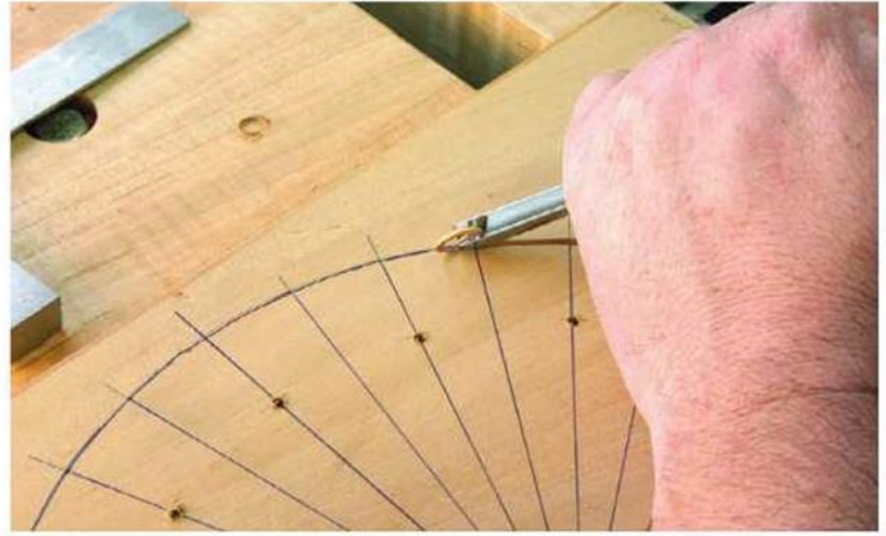
It's like driving a car. Steer your V-parting tool along the outer edge of the fan. How you turn your wrist determines the cut's path.
