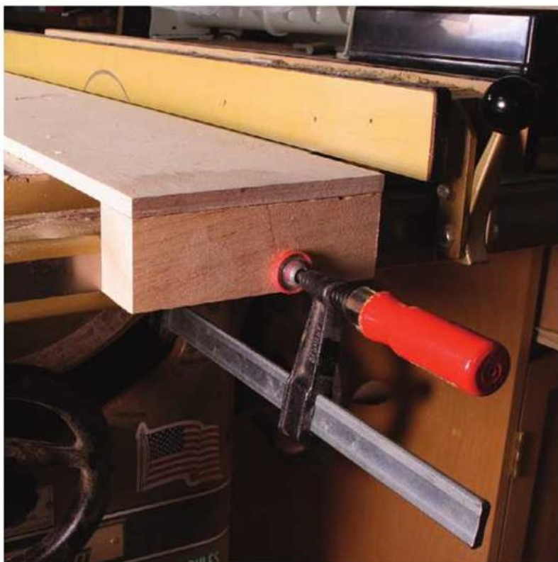
An overgrown bench hook. This jig works on the same principle as a bench hook, but it's essential to clamp the hook to your table saw's rail to be safe. You don't want it to move.
