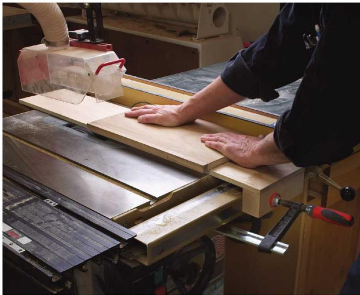
Just a little off the bottom. When you add solid-wood edging to plywood, trimming the solid wood flush to the plywood can be tricky or tedious. This simple jig (two bits of wood that are nailed and glued together) makes it simple and quick.
